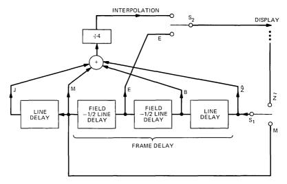
Fig. 7—Implementation of field interpolation.  $S_1$  is held in the down position during input of repeated fields and interpolated fields. No data are generated for them. One field period later,  $S_2$  is put in the up position to display interpolated fields and in the down position to display updated and repeated fields (see Fig. 1).
