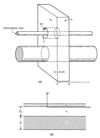
Fig. 7—(a) Schematic for the derivation of the general perturbation formula. The dielectric waveguide is perturbed by a small lossy rod. The closed surface S extends to infinity where the fields considered are assumed to vanish. (b) Application to the perturbation of H waves guided by a dielectric slab (k) by a lossy slab  $(k_m)$ .
