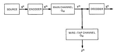
Fig. 2—Wire-tap channel (general case).
