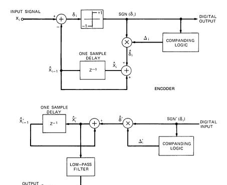
Fig. 1—Single-integration delta modulation.
