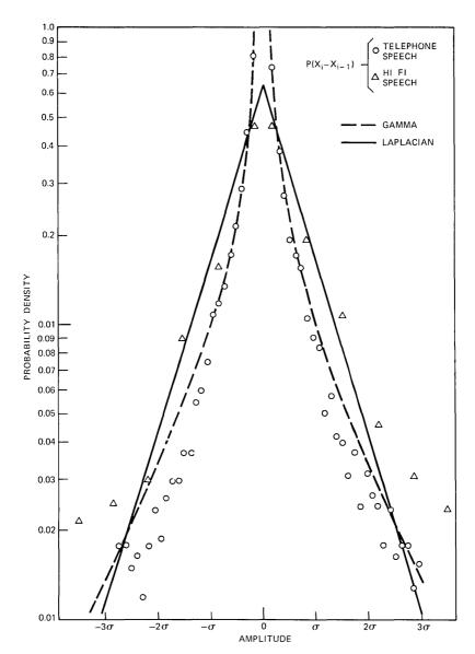
Fig. 3—The amplitude probability density function of  $(x_i - x_{i-1})$  as compared with the Laplacian and gamma distributions.
