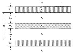
Fig. 1—Coupled dielectric slabs with thickness 2d and free wave number k. The cladding medium has free wave number k. Crosstalk can be reduced by introducing a metallic layer with free wave number  $k_m$  (almost purely imaginary) and thickness 2d.
