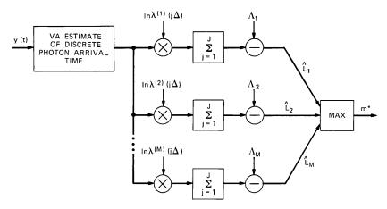
Fig. 11—Estimator detector type of weighted counter.
