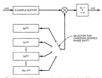
Fig. 2—A practical implementation of a variable phase shifter.
