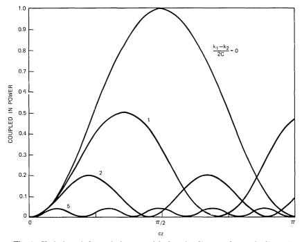
Fig. 4—Variation of the optical power picked up by fiber 2, where only fiber 1 is excited at z=0, as a function of the normalized axial distance. The axial wave numbers of the isolated fibers are assumed to be constant but different [parameter  $(k_1 - k_2)/2c$ ]. Note that the behavior for small cz is independent of  $k_1 - k_2$ .
