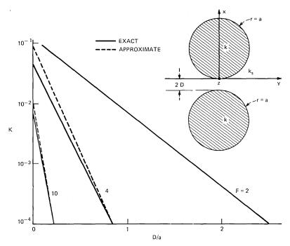
Fig. 3—Variation of the coupling between two dielectric rods of radii a as a function of their spacing (2D). The dimensions and free wave numbers are shown. The parameter K is defined as  $ca(1-k_s^2/k^2)^{-1}$ , and c is the coupling. The plain lines are from Snyder exact theory, and the dashed lines from the theory in Ref. 1, applied to large normalized frequencies F.
