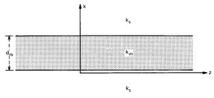
Fig. 6—Transmission of a metallic layer with thickness  $d_m$  and free wave number  $k_m$  under evanescent wave excitation (axial wave number  $k_z > k_*$ ). At large negative x, the field is assumed unperturbed by the layer.
