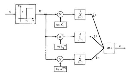
Fig. 3—Threshold-based weighted counter.
