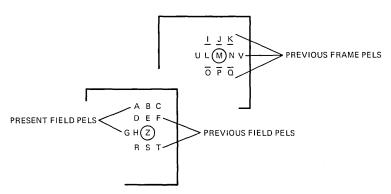
Fig. 1—Two successive television frames, interlacing assumed (two interlaced fields per frame). Pels Z and M are exactly one frame apart.
