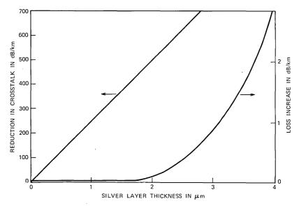
Fig. 2—Reduction in crosstalk and increase in fiber loss resulting from the introduction of a silver layer of thickness  $2d_m$  (free-space wavelength = 1  $\mu$ m). The dielectric slabs have a normalized frequency  $F \equiv (k^2 - k_s^2)^4 d = \pi/2$ . Their spacing is kept equal to 11  $\mu$ m. The loss varies with  $d_m$  only because of the change in the slab-layer spacing. In the absence of metallic layer, crosstalk is -20 dB/km.
