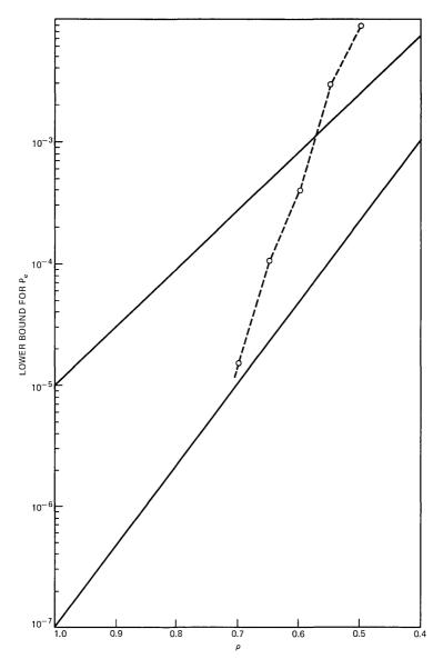
Fig. 2—Lower bounds on error rate vs signaling speed for two initial  $(\rho=1)$  cases. The solid curves are both matched filter bounds. The dashed curve is based on minimum-distance considerations and applies to the  $10^{-7}$  case. All curves are drawn for constant power.
