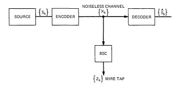
Fig. 1—Wire-tap channel (special case).
