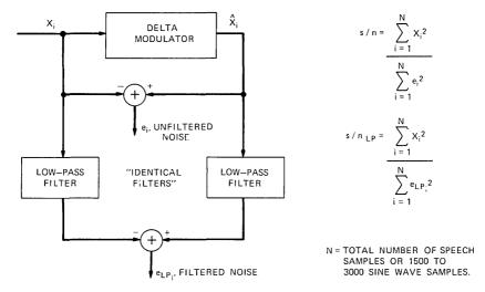
Fig. 2—Quantizing noise measurement.
