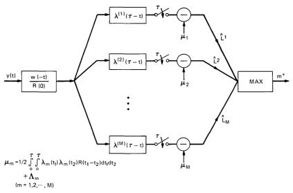
Fig. 5—Correlator filter for M-ary signaling.
