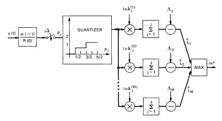
Fig. 10—Weighted counter with quantizer.
