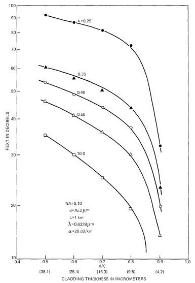
Fig. 15—FEXT vs. d/C (cladding thickness),  $d=76.2~\mu\mathrm{m},~\mathrm{NA}=0.10,~L=1~\mathrm{km},$   $\lambda=0.6328~\mu\mathrm{m},~\alpha=20~\mathrm{dB/km}.$
