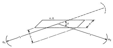
Fig. 3-Reflection from passive repeater.
