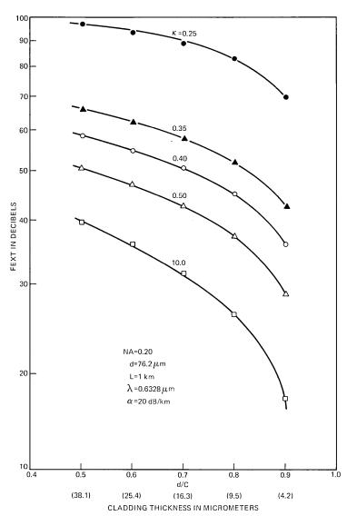
Fig. 17—FEXT vs. d/C (cladding thickness),  $d=76.2~\mu\mathrm{m},~\mathrm{NA}=0.20,~L=1~\mathrm{km},$   $\lambda=0.6328~\mu\mathrm{m},~\alpha=20~\mathrm{dB/km}.$
