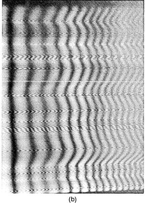
Fig. 3—Backscattered light patterns. (a) Complete pattern from 12.0-cm section of fiber. Slit in center allows for passage of incident light and bright spots in center are photographic artifacts. (b) Expansion of section of interest.
