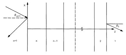
Fig. 22—Geometry used for calculation of transmission coefficients in multilayered dielectric media.
