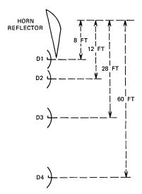
Fig. 30—Receiving antennas at Palmetto, Georgia in 1968. D1 to D4 are 4-foot-diameter parabolic reflectors.
