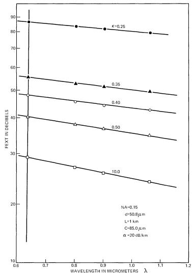
Fig. 21—Fext vs.  $\lambda$  (wavelength), L=1 km,  $d=50.8~\mu\text{m},~C=85~\mu\text{m},~\alpha=20$  dB/km, NA = 0.15,  $\kappa=0.25,~0.35,~0.40,~0.50,~10.0.$
