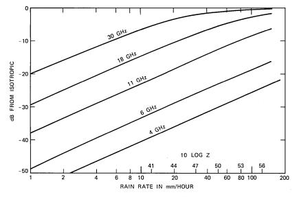
Fig. 2—Effective antenna gain  $G'_1$  during rain.
