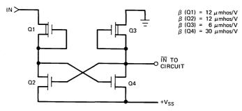
Fig. 7—Inverting level shifting input circuit.
