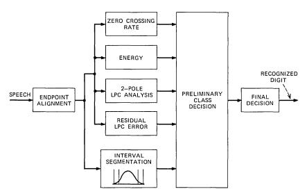
Fig. 1-Block diagram of the overall digit recognition system.
