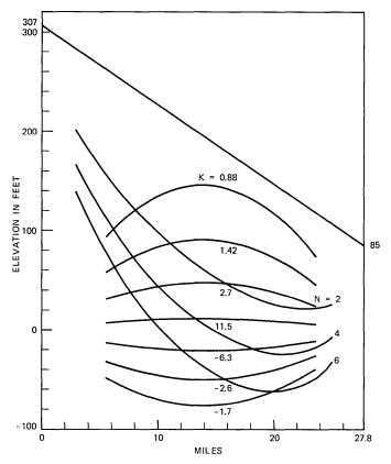
Fig. 20—Even Fresnel zone boundaries at 85-foot height for bottom receiving antenna at a frequency of 4 GHz.
