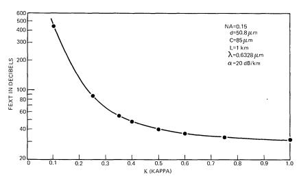
Fig. 20—Fext vs.  $\kappa$  (kappa), L=1 km,  $d=50.8~\mu\text{m},\,C=85~\mu\text{m},\,\alpha=20~\text{dB/km},\,\text{NA}=0.15,\,\lambda=0.6328~\mu\text{m}.$
