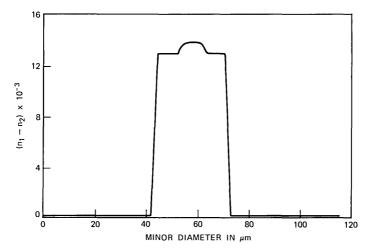
Fig. 1—Microinterferogram and index profile of cvp step-index fiber.
