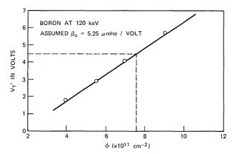
Fig. 6—Effective threshold vs. implant dose.
