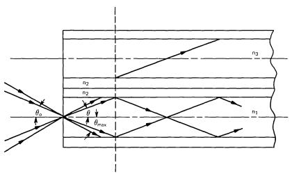
Fig. 3—Ray tracing of transmitted and crosstalk rays in adjacent optical fibers.
