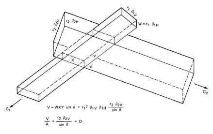
Fig. 4—Geometry of common volume.
