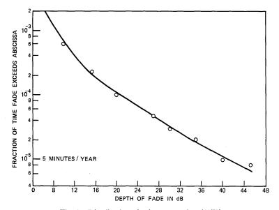
Fig. 6—Distribution of rain attenuation (1970).
