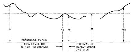
Fig. 25—Determination of terrain roughness.
