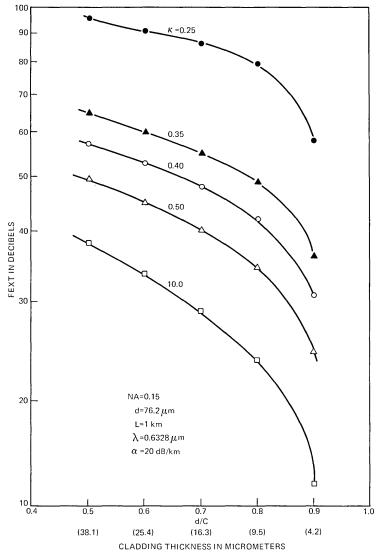
Fig. 16—FEXT vs. d/C (cladding thickness),  $d=76.2~\mu\mathrm{m},$  NA = 0.15,  $L=1~\mathrm{km},$   $\lambda=0.6328~\mu\mathrm{m},$   $\alpha=20~\mathrm{dB/km}.$
