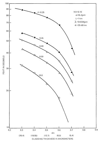
Fig. 9—fext vs. d/C (cladding thickness),  $d=25.4~\mu\text{m}$ , NA = 0.10, L=1~km,  $\lambda=0.6328~\mu\text{m}$ ,  $\alpha=20~\text{dB/km}$ .
