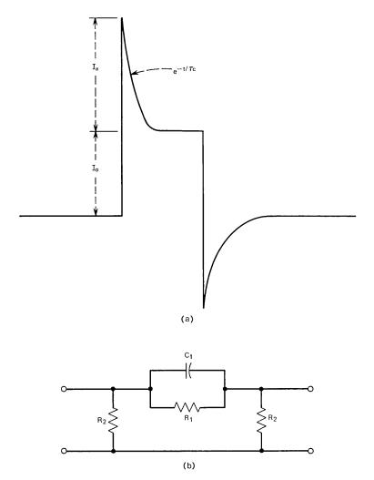
Fig. 6—(a) Current waveform for delay reduction of laser diodes. (b) The pulse shaping network used in the experiment.
