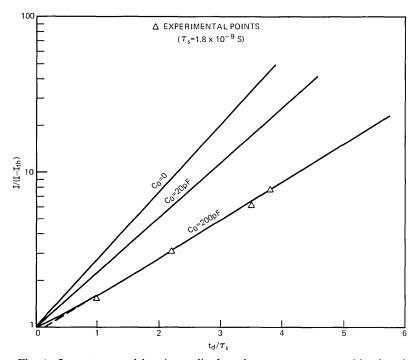
Fig. 4—Laser turn-on delay (normalized to the spontaneous recombination time  $\tau_*$ ) as a function of excitation currents above threshold for various zero-bias diode capacitances. Solid lines are calculated.
