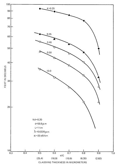
Fig. 14—FEXT vs. d/C (cladding thickness),  $d=50.8~\mu\text{m}$ , NA = 0.20, L=1~km,  $\lambda=0.6328~\mu\text{m}$ ,  $\alpha=20~\text{dB/km}$ .
