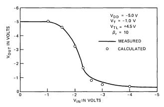
Fig. 4—Depletion-load inverter transfer curve.
