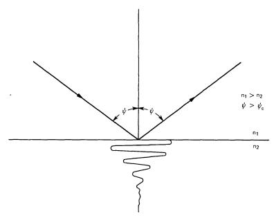
Fig. 4—Total internal reflection from plane dielectric boundary.
