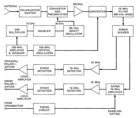
Fig. 2—60-GHz solid-state receiver with injection-locked local oscillator.
