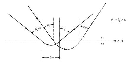
Fig. 5—Displacement of ray—the Goos-Hänchen shift.
