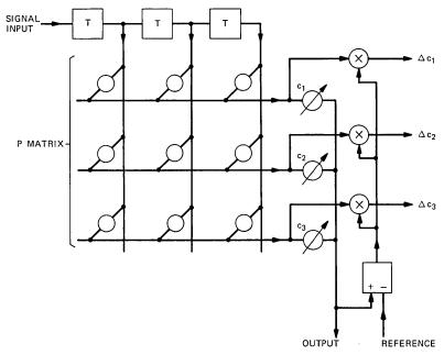
Fig. 3—Use of P matrix to obtain a modified equalizer structure.
