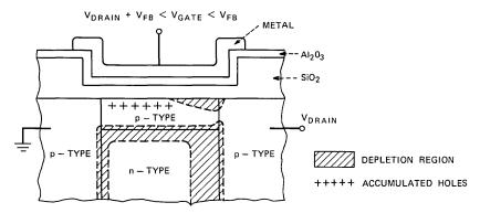
Fig. 5—Depletion igfet cross-sectional view.
