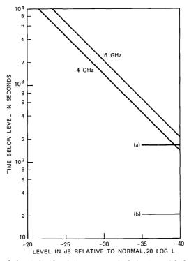
Fig. 5—Annual time below level (average case). Objectives: (a) short haul = 165 seconds/year, (b) long haul = 20 seconds/year.
