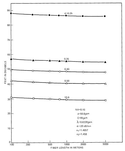
Fig. 19—fext vs. fiber length  $d=50.8~\mu\text{m},~C=85~\mu\text{m},~\alpha=20~\text{dB/km},~\text{NA}=0.15,~\lambda=0.6328~\mu\text{m},~\kappa=0.25,~0.35,~0.40,~0.50,~10.0.$
