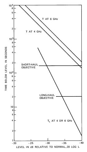
Fig. 8—Annual simultaneous time below level for 30-foot separation of antennas (continuation of average-case example from Fig. 5).
