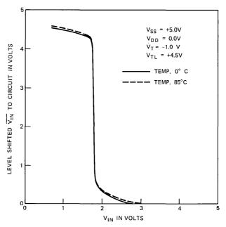
Fig. 8—Inverting level shifter transfer curves.
