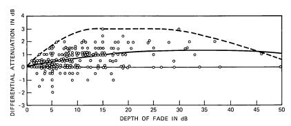
Fig. 10—Plot of measured differential attenuation as a function of fade depth.
