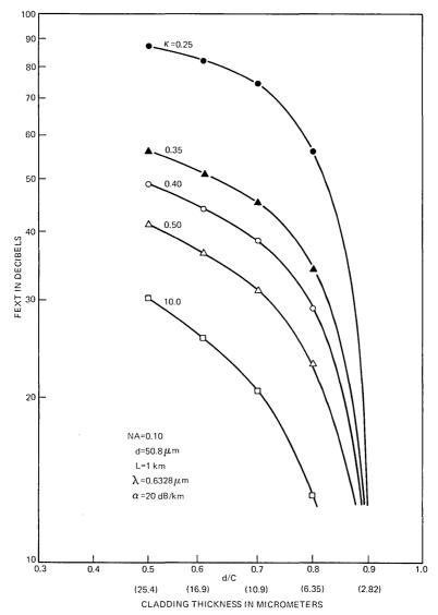
Fig. 12—fext vs. d/C (cladding thickness),  $d=50.8~\mu\text{m},~\text{NA}=0.10,~L=1~\text{km},~\lambda=0.6328~\mu\text{m},~\alpha=20~\text{dB/km}.$
