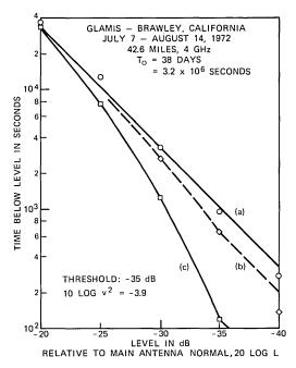
Fig. 12—Threshold switching, Glamis to Brawley, California. Reception at (a) Glamis, main antenna (unprotected), (b) Brawley, 15-foot separation, (c) Glamis, 30-foot separation.
