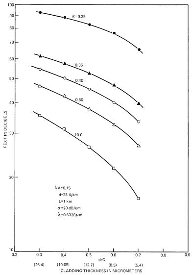
Fig. 10—fext vs. d/C (cladding thickness),  $d=25.4~\mu{\rm m},~{\rm NA}=0.15,~L=1~{\rm km},$   $\lambda=0.6328~\mu{\rm m},~\alpha=20~{\rm dB/km}.$
