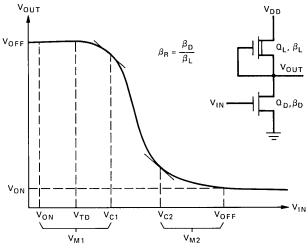
Fig. 2—Depletion load inverter.
