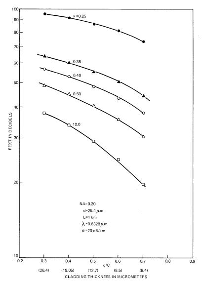
Fig. 11—FEXT vs. d/C (cladding thickness),  $d=25.4~\mu{\rm m},~{\rm NA}=0.20,~L=1~{\rm km},$   $\lambda=0.6328~\mu{\rm m},~\alpha=20~{\rm dB/km}.$
