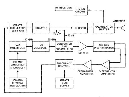
Fig. 3—60-GHz solid-state transmitter with frequency-controlled oscillator.
