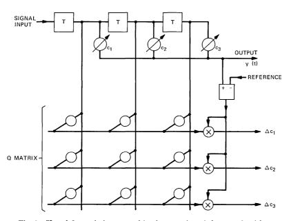
Fig. 2—Use of Q matrix in a second implementation of the new algorithm.
