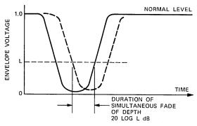
Fig. 6—Definition of simultaneous fade.
