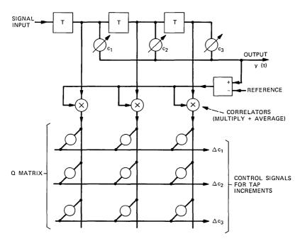
Fig. 1—Use of Q matrix in a first implementation of the new algorithm.
