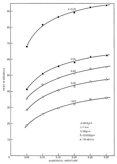
Fig. 18—FEXT vs. numerical aperture,  $d=50.8~\mu\text{m},~C=85~\mu\text{m},~\alpha=20~\text{dB/km},~L=1~\text{km},~\lambda=0.6328~\mu\text{m},~\kappa=0.25,~0.35,~0.4,~0.5,~10.0.$
