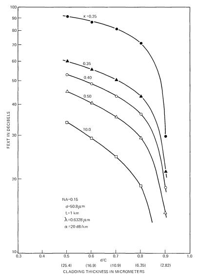
Fig. 13—Fext vs. d/C (cladding thickness),  $d=50.8~\mu{\rm m},~{\rm NA}=0.15,~L=1~{\rm km},$   $\lambda=0.6328~\mu{\rm m},~\alpha=20~{\rm dB/km}.$
