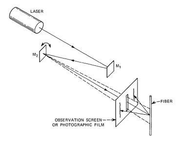
Fig. 2—Optical arrangement to determine core distortion function.
