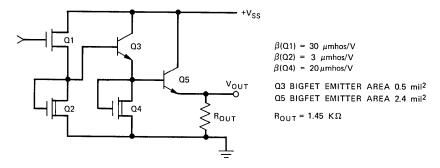
Fig. 9—BIGFET SIC output circuit.
