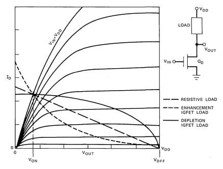
Fig. 1—Inverter load-line characteristics.
