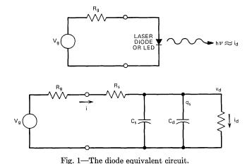
where the time constant  $\tau_s$  is the carrier spontaneous recombination time. This is equivalent to a capacitance,  $C_d$ , whose charge,  $q_d(t)$ , is equal to the stored charge and whose instantaneous charge-voltage relationship satisfies
