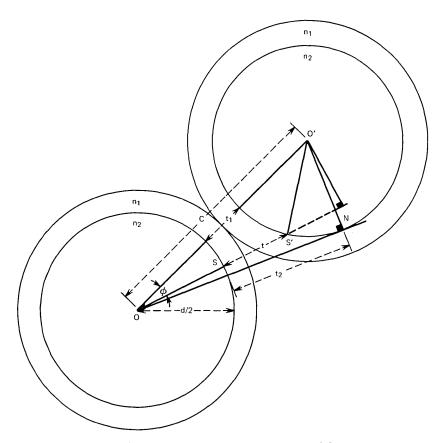
Fig. 8—Geometry of two adjacent round optical fibers.
