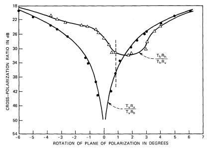
Fig. 4—Polarization discrimination characteristics of the operating system.
