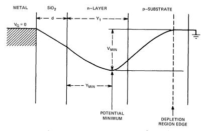
Fig. 2—Schematic potential diagram of a buried-channel CCD.
