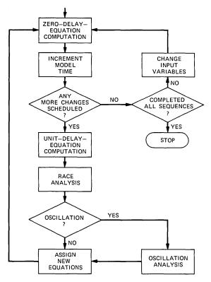
Fig. 7—Equation computation flow chart.
