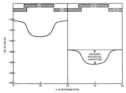
Fig. 5—Channel potential in a two-phase BCCD with all plates either at 0 or 15 volts. Parameters are  $d_1=0.3~\mu\text{m},~d_2=0.12~\mu\text{m},~Y_1=1.2~\mu\text{m},~Q_n=1.5\times10^{12}~\text{cm}^{-2},~N_A=5\times10^{14}~\text{cm}^{-3}.$
