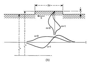
Fig. 2—(a) Whispering-gallery modes clinging to a circular boundary with effective radius  $\rho$  (= $a/\sin^2\theta$ ). The field ( $m=0,1,\cdots$ ) is described exactly by Bessel functions and approximately by Airy functions. (b) Cross section in a local r,  $\xi$  plane.
