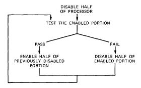
Fig. 1—Flow diagram of disabling process.
