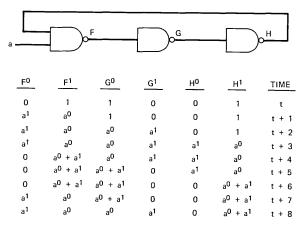
Fig. 6-Equation oscillation.
