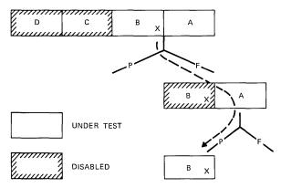
Fig. 2—Proposed method of fault location.
