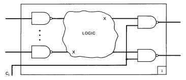
Fig. 4—Circuit-pack logic-disabling process.
