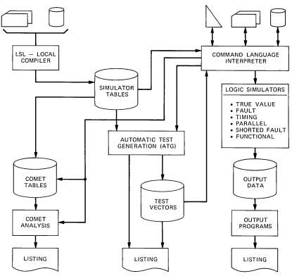
Fig. 1—Block diagram of LAMP system.
