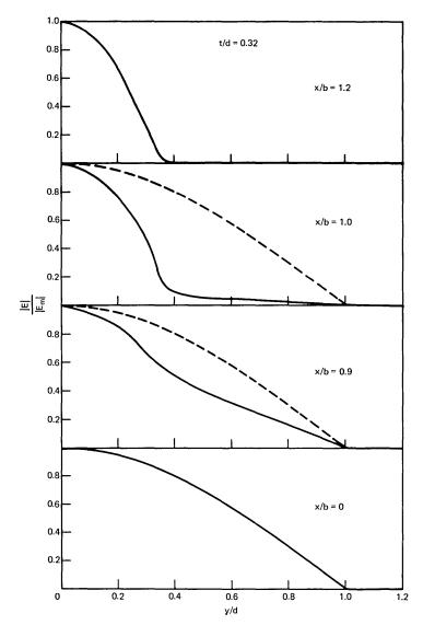
Fig. 4—Magnitude of the electric field vector relative to its maximum value at y=0 as a function of the normalized vertical dimension y/d. Solid and broken curves describe the single-material fiber with t/d=0.32 and t/d=0.
