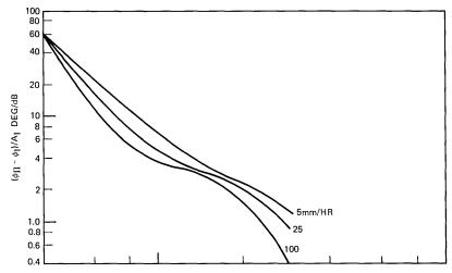
Fig. 4a—Normalized differential phase shift with respect to  $A_{\rm I}$  (4 to 30 GHz).
