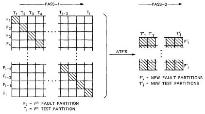
Fig. 5—Two-pass diagonal simulation.
