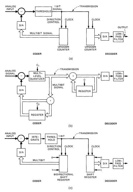
Fig. 1—Differential codecs employing digital integration. (a) Steps are counted in a delta modulator. (b) Steps are accumulated in a differential codec. (c) A shift register stores 1's in an interpolative codec.
