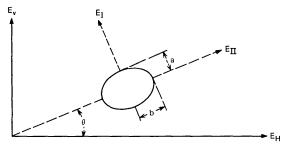
Fig. 1—Canted oblate spheroidal raindrop.
