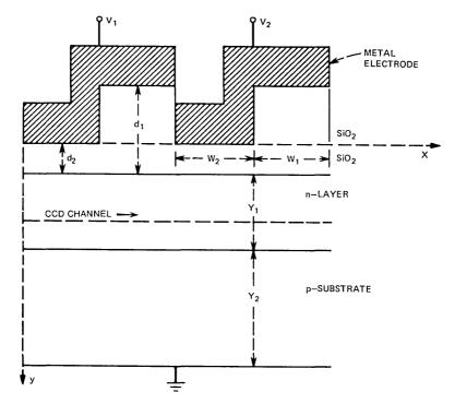
Fig. 3—Schematic diagram of a two-phase, stepped-oxide BCCD.
