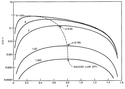
Fig. 2—Variation of the ratio of phase to group velocity in a dielectric slab for different relative permittivities, as a function of the characteristic angle  $\phi$ . The optimum points of operation for low pulse spreading in square-law tapered slabs are shown by a dashed line ( $\lambda = 1 \mu m$ ).
