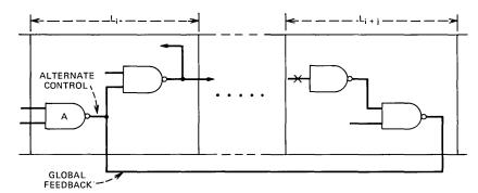
Fig. 8—Example of global feedback.
