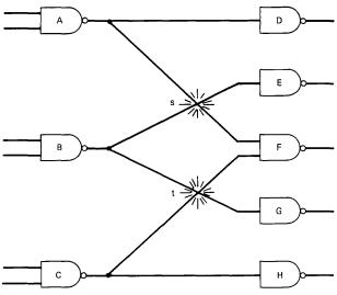
Fig. 6-Two shorted faults.
