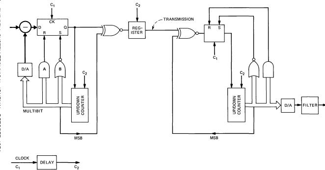
Fig. 2—Circuit that signals changes of magnitude.
