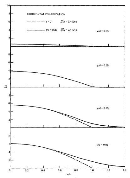
Fig. 3—Magnitude of the electric field vector shown as a function of the normalized horizontal dimension x/b. Solid curves describe the single-material fiber with t/d = 0.32, and broken curves apply to the fiber with t/d = 0.
