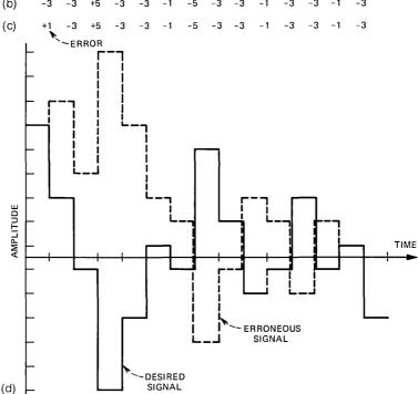
Fig. 6—Response of a multilevel differential codec having step sizes  $\pm 1$ ,  $\pm 3$ ,  $\pm 5$ . (a) Ordinary differential code. (b) The code that signals changes of magnitude. (c) The code with an error. (d) The correct and erroneous responses.
