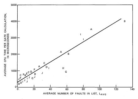
Fig. 7—Simulator time required to calculate gate output.
