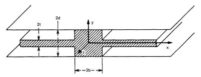
Fig. 2—For our analysis, the single-material fiber is placed between two perfectly conducting planes.
