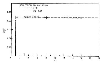
Fig. 8—Mode spectrum of the lowest-order single-material fiber mode in the region of its support slab with t/d=0.32. The short vertical broken line represents the mode content of the fiber with t=0.
