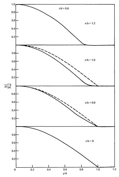
Fig. 6—Magnitude of the electric field vector relative to its maximum value at y=0 as a function of the normalized vertical dimension y/d. Solid and broken curves describe the single-material fiber with t/d=0.8 and t/d=0.
