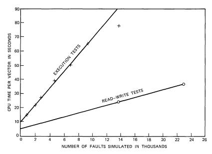
Fig. 8—Simulation times for typical processor diagnostics.
