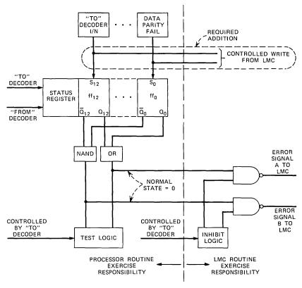
Fig. 12—Status register and its local-maintenance-center interface.
