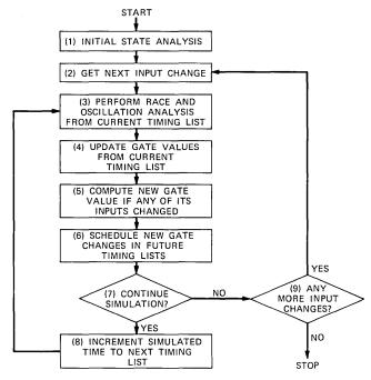
Fig. 1—Simplified simulation flow.
