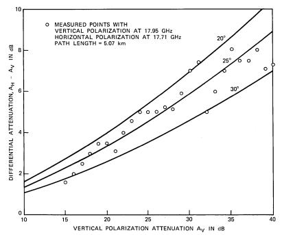
Fig. 5—Comparison between calculated and measured differential attenuation at 18 GHz.
