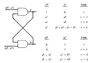
Fig. 4—Equations from F = 0, G = 1 state.
