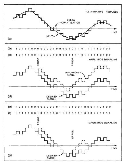
Fig. 3—code responses. (a) Representative input and output. (b) Delta modulator code. (c) Delta modulator code with two errors. (d) Delta modulator responses. (e) Code that signals magnitude change. (f) Code with two errors. (g) Output waveforms.
