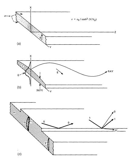
Fig. 1—Planar fibers. (a) Fiber with constant thickness and variation of the permittivity of the form  $1/\cosh^2(y)$ . (b) Tapered dielectric slab. The field is shown for the  $H_1$  slab mode. (c) Coupling between the various slab modes  $(H_1, H_2, \dots, E_1, E_2, \dots)$  cannot be neglected when the thickness 2d(y) varies abruptly. This coupling can eliminate the higher-order modes  $(H_2, E_2, \dots)$  for suitable dimensions (see Ref. 12).
