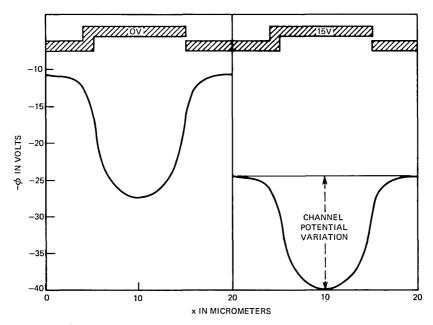
Fig. 6—Channel potential in a two-phase BCCD with all plates either at 0 or 15 volts. The parameters are  $d_1=0.6~\mu\mathrm{m},~d_2=0.12~\mu\mathrm{m},~Y_1=1.2~\mu\mathrm{m},~Q_n=1.5\times10^{12}~\mathrm{cm}^{-2},~N_A=5\times10^{14}~\mathrm{cm}^{-3}.$
