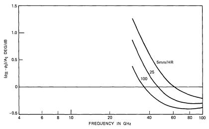
Fig. 4b—Normalized differential phase shift with respect to A<sub>I</sub> (30 to 100 GHz).
