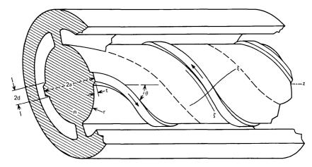
Fig. 1—Open view of the single-material, helicoidal fiber for two optical channels. The two optical beams propagate in the two ridges shown, with areas  $t \times 2d$ . The helicoidal motion is essential to maintain confinement. High-order modes are not confined. They radiate away to the envelope through the wings (only part of one is shown). The ratio period/diameter is much larger than that shown in the figure.
