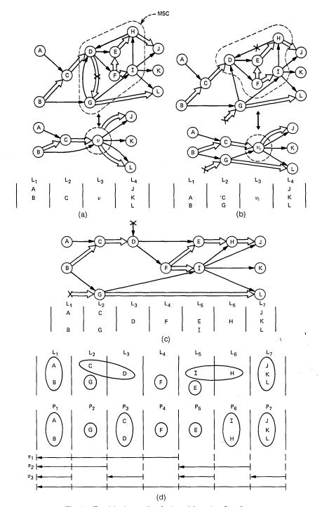
Fig. 7—Partitioning and ordering of functional nodes.
