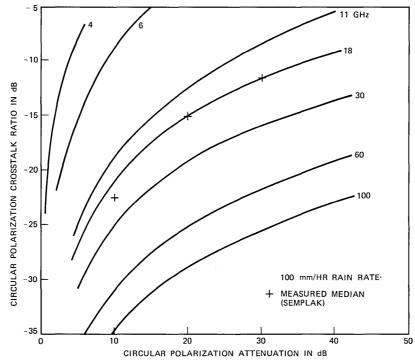
Fig. 12—Calculated rain-induced cross-polarization of circularly polarized waves.
