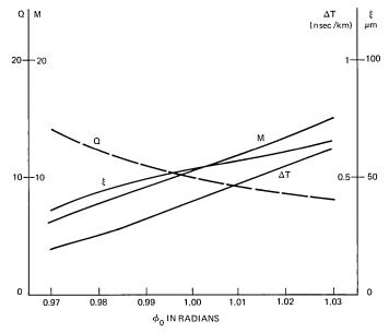
Fig. 5—Variation with the characteristic angle on axis  $\phi_o$  (or slab thickness on axis  $2d_o$ ) of the quality factor Q for  $\epsilon=1.02$  (n=1.01) and  $\phi=\phi_o-5\times 10^{-3}|y|$ . The variations of  $\xi$ , M, and  $\Delta T$  are also given. The ray period is 5.6 mm and  $\theta_o$  is equal to 4° for  $\phi_o=1$ .
