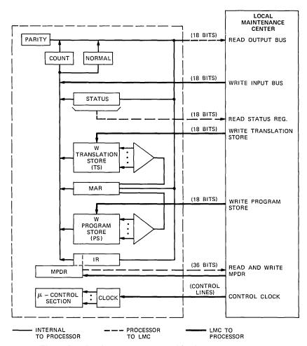
Fig. 9—Interface between processor and local-maintenance center.
