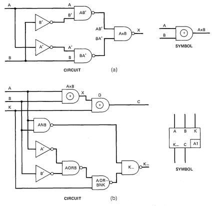
Fig. 2—(a) Exclusive-or circuit. (b) One-bit adder circuit.
