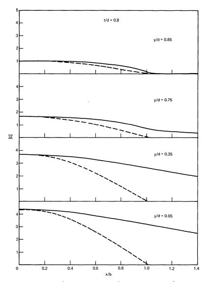
Fig. 5—Magnitude of the electric field vector shown as a function of the normalized horizontal dimension x/b. Solid curves describe the single-material fiber with t/d=0.8, and the broken curves apply to the fiber with t/d=0.
