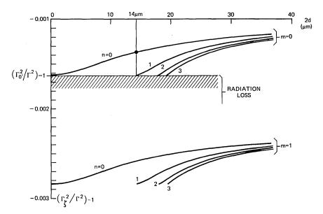
Fig. 3—Axial wave numbers  $\Gamma_{\xi mn}$  for various m and n modes (r and  $\xi$  coordinates). Radiation loss is suffered whenever  $\Gamma_{\zeta} < \Gamma_{0'}$ . The radiation zone is shaded. This figure shows that single-mode propagation is possible if the ridge width 2d is less than  $14 \ \mu m$  (for  $\lambda_0 = 1 \ \mu m$ , n = 1.45,  $t = 3.5 \ \mu m$ ,  $a = 50 \ \mu m$ , and  $\theta = 2.5^{\circ}$ ).
