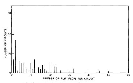
Fig. 14—Distribution of number of flip-flops per circuit.
