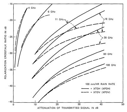
Fig. 10—Calculated rain-induced cross-polarization of horizontally and vertically polarized waves.
