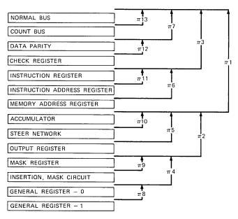
Fig. 14—Functional nodes included in simulation experiments.
