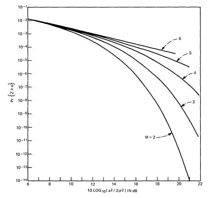
Fig. 8—Plots of Pr  $\{Z>a\}$  for n=2,  $10\log_{10}\left(a^2/\sum_{i=1}^M b_i^i\right)=8$  dB,  $b_1=\cdots=b_M$ , and for various values of M.
