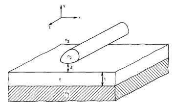
Fig. 4—Slab-loaded waveguide.
