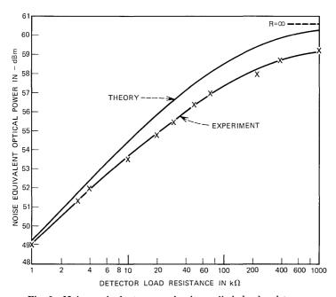
Fig. 8—Noise equivalent power circuit vs. diode load resistance.
