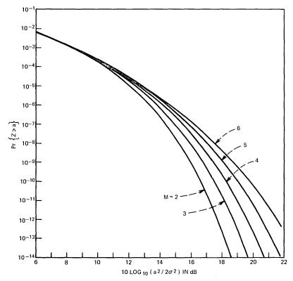
Fig. 12—Plots of Pr  $\{Z>a\}$  for n=3,  $10 \log_{10} (a^2/\sum_{i=1}^{M} b_i^2) = 10 \text{ dB}$ ,  $b_1=\cdots=b_M$ , and for various values of M.
