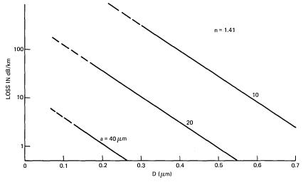
Fig. 5—Radiation loss in dB/km of the rod  $H_{01}$  mode in the slab as a function of spacing D with the rod radius a as a parameter, for  $n_{\text{rod}} = n_{\text{slab}} = 1.41$ . These curves are valid for large values of D.
