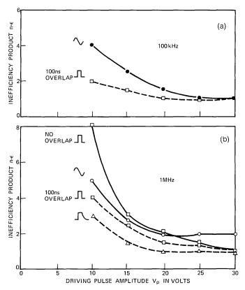
Fig. 11—Transfer inefficiency product as a function of driving pulse amplitude for various waveforms at (a) 100 kHz and (b) 1 MHz.
