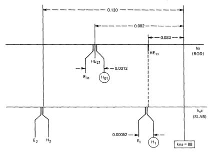
Fig. 4—Propagation constants (h) of the trapped modes of the rod and maximum value (h<sub>s</sub>) of the propagation constants of the radiation modes in the slab. It is assumed that n=1.41,  $\lambda=1~\mu\mathrm{m}$ , and  $a=10~\mu\mathrm{m}$ . The modes circled are those whose coupling is discussed in this paper.
