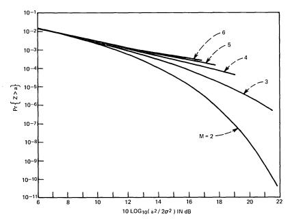
Fig. 10—Plots of Pr  $\{Z > a\}$  for n = 3,  $10 \log_{10} (a^2/\sum_{i=1}^{M} b_i^2) = 6 dB$ ,  $b_1 = \cdots = b_M$ , and for various values of M.
