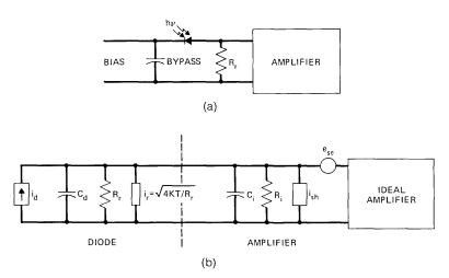
Fig. 1—(a) Input circuit. (b) Equivalent circuit.
