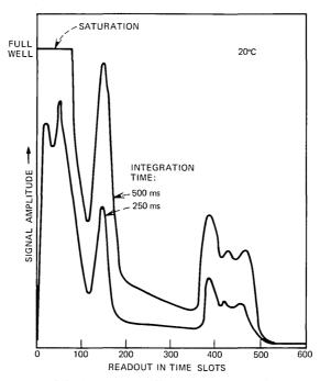
Fig. 16—Integrated dark current profile for two different integration times.
