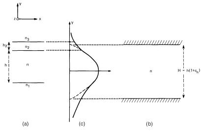
Fig. 12—(a) Two-layered slab. (b) Equivalent slab. (c) Field distributions  $(E_x$  and  $H_y$  or  $E_y$  and  $H_z$ ) in original slab (solid line) and in equivalent slab (dotted line).
