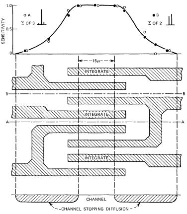
Fig. 18—Normalized light sensitivity measured with a narrow light spot in two different traces across the transfer channel.
