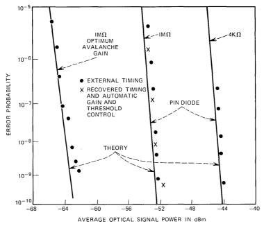
Fig. 11—Error probability vs. average optical signal power.
