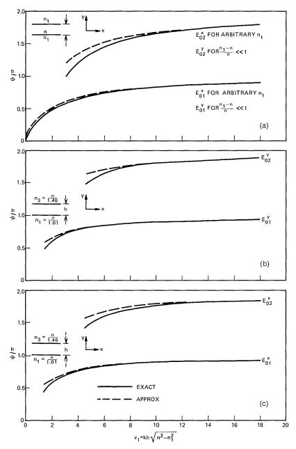
Fig. 13—Exact and approximate width of dielectric slabs. (a) Symmetric slab. (b) Asymmetric slab (polarization along y). (c) Asymmetric slab (polarization along x).
