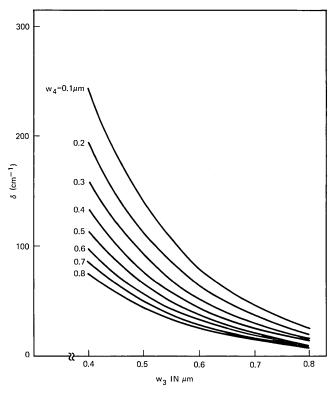
Fig. 2—The degenerate shift  $\delta$  as a function of half the distance between the two waveguides  $w_{\delta}$ , with the halfwidth  $w_{\delta}$  of guide IV as a parameter.
