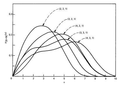
Fig. 1—Plots of p.d.f. of |S + N| for  $\sigma^2 = 1$ , M = 3, n = 2, and different sets of vector lengths  $(b_1, b_2, b_3)$ .
