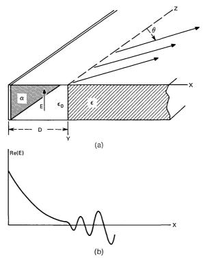
Fig. 1—(a) Reactive surface, with normalized susceptance  $\alpha$ , coupled to a semi-infinite dielectric with permittivity  $\epsilon = n^2 \epsilon_0$ . For H modes, the structure is assumed terminated in the y direction by electric walls. Radiation takes place at the Cerenkov angle  $\theta = \cos^{-1} \left[ (k^2 + \alpha^2)^{\frac{1}{2}} / kn \right]$ ,  $k = 2\pi/\lambda$ . (b) Variation of the field as a function of x.
