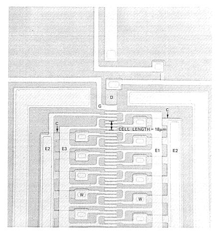
Fig. 1—One end of the linear 500-element 3-phase CCD. Shown are the three sets of transfer electrodes (E1, E2, and E3), the input diode (D), and the input gate (G). Electrodes E2 are alternately contacted to diffused crossunders (C) through contact windows (W) lying on either side of the transfer channel.
