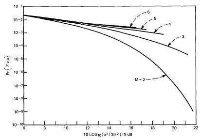
Fig. 7—Plots of Pr  $\{Z>a\}$  for n=2,  $10\log_{10}\left(a^2/\sum_{i=1}^M b_i^2\right)=6$  dB,  $b_1=\cdots=b_M$ , and for various values of M.
