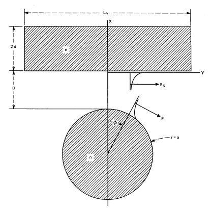
Fig. 3—Dielectric rod coupled to a dielectric slab. The rod field E is shown for the spurious  $H_{01}$  mode, and the slab mode is  $H_{1r}$  ( $\nu$  is a continuous index in the limit  $L_{\nu} \to \infty$ ). Coupling takes place at  $\phi \approx 0$ .
