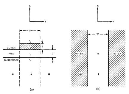
Fig. 1—Geometry of (a) strip-loaded film waveguide and (b) equivalent symmetrical waveguide.
