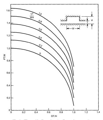
Fig. 8—Waveguide dimensions for  $E_{PQ}^{x,y}$  mode at cutoff.
