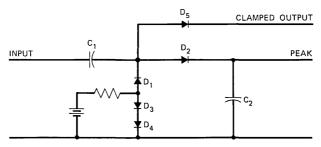
Fig. 5—Clamp and peak detector.
