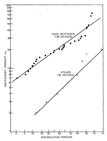
Fig. 19—Plot of  $n\epsilon$  distribution for all operating backsputter delineated devices and for a control batch with etched electrodes.
