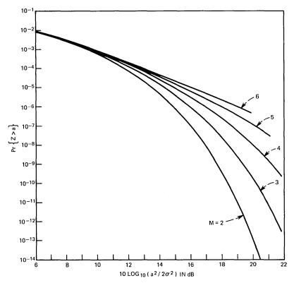
Fig. 11—Plots of Pr  $\{Z > a\}$  for n = 3,  $10 \log_{10} (a^2 / \sum_{i=1}^{M} b_i^2) = 8 dB$ ,  $b_1 = \cdots = b_M$ , and for various values of M.
