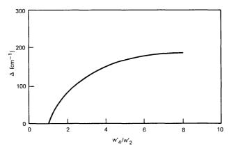
Fig. 4—The mismatching  $\Delta$  as a function of the ratio of the guide widths.
