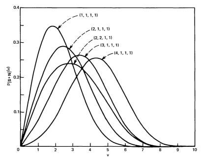
Fig. 2—Plots of p.d.f. of |S+N| for  $\sigma^2=1, M=4, n=2$ , and different sets of vector lengths  $(b_1, b_2, b_3, b_4)$ .
