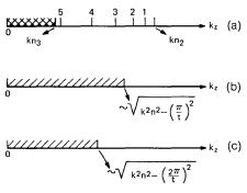
Fig. 5—Modal spectrum in: (a) isolated fiber of Fig. 4; (b) isolated slab of Fig. 4 (only for modes with one half period across t; (c) isolated slab of Fig. 4 (only for modes with two half periods across t).
