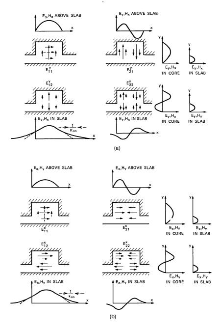
Fig. 7—Two families of modes. (a)  $E^{y}_{pq}$  modes and (b)  $E^{z}_{pq}$  modes.
