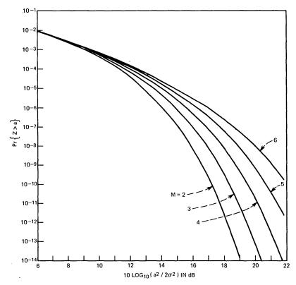
Fig. 9—Plots of Pr  $\{Z > a\}$  for n = 2,  $10 \log_{10} (a^2 / \sum_{i=1}^{M} b_i^2) = 10 \text{ dB}$ ,  $b_1 = \cdots = b_M$ , and for various values of M.
