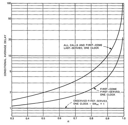
Fig. 2--Conditional average delay for M/M/1 vs occupancy.
