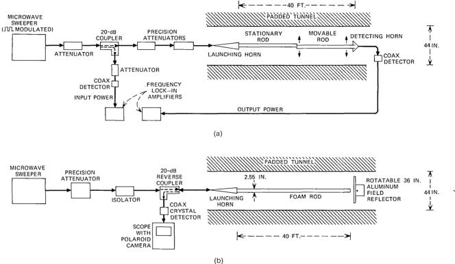
Fig. 3—Experimental arrangement used to corroborate analysis using microwave-guiding polyfoam rods. (a) Coupling vs axial displacement measurement configuration. (b) Coupling vs angular misalignment measurement configuration.
