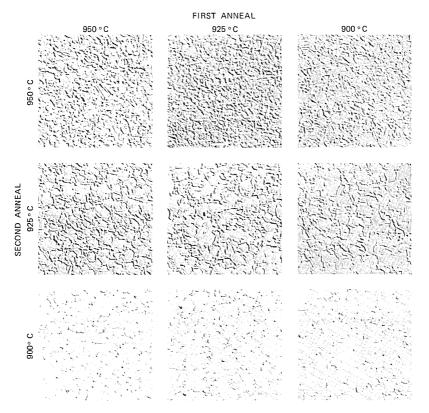
Fig. 7—Quenched microstructures of 2.5% V-0.53-mm Remendur wire; etched; DIC; 600X. First anneal indicates temperature of  $\frac{1}{2}$  hour anneal of 6.35-mm rod. Second anneal indicates temperature of  $\frac{1}{2}$  minute strand anneal of 0.53-mm wire.
