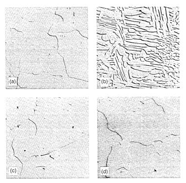
Fig. 4—Quenched microstructures of 2.5% V-6.35-mm Remendur rod in hot-rolled and various annealed conditions; etched; DIC; 600X. (a) Hot-rolled. (b) Annealed;  $\frac{1}{2}$  hour; 950°C. (c) Annealed;  $\frac{1}{2}$  hour; 925°C. (d) Annealed;  $\frac{1}{2}$  hour; 900°C.
