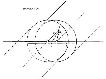
Fig. 1-Butt-joined fiber cores displaced by axial translation.
