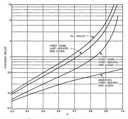
Fig. 3—Average delay for M/D/1 vs occupancy.
