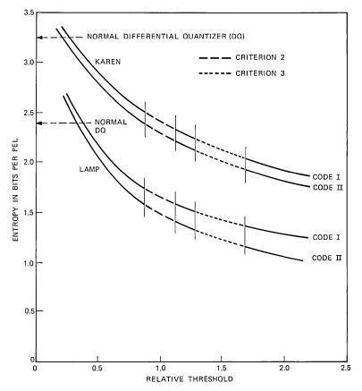
Fig. 7—Entropy of the free-running algorithm as a function of the threshold The measurements of entropy are made under the assumption of two different types of reversible code. The performance for the codes is very similar.
