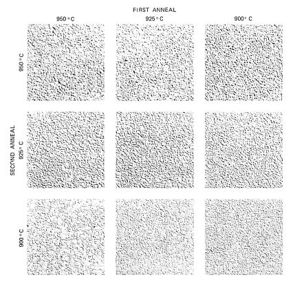
Fig. 8—Quenched microstructures of 3.0% V-0.53-mm Remendur wire; etched; DIC; 600X. First anneal indicates temperature of  $\frac{1}{2}$  hour anneal of 6.35-mm rod. Second anneal indicates temperature of  $\frac{1}{2}$  minute strand anneal of 0.53-mm wire.
