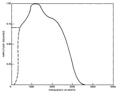
Fig. 2—Amplitude-squared characteristic of typical voiceband channel.
