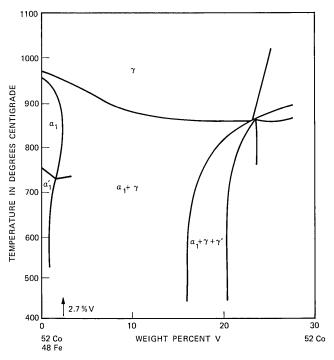
Fig. 3—Vertical section through Fe-Co-V ternary phase diagram, from the work of Köster and Schmid.<sup>1</sup>
