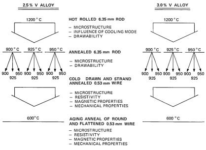
Fig. 2—Synopsis of Remendur processing experiment.
