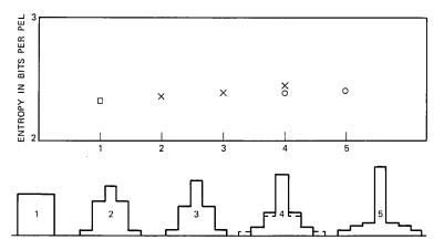
Fig. 9—Effect on entropy (code II) of varying the shape of the filter function. The width of the impulse response is:  $\square -3$  elements,  $\times -5$  elements,  $\bigcirc -7$  elements. Threshold decisions are very insensitive to the shape of the filter function.
