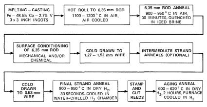
Fig. 1-Typical Remendur processing.
