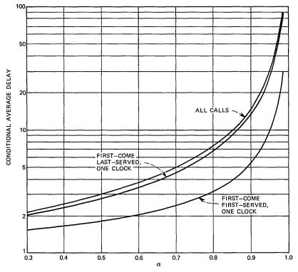
Fig. 5—Conditional average delay for  $M/\Gamma_{\frac{1}{2}}/1$  vs occupancy.
