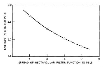
Fig. 10a—The effect on entropy (code II) of varying the width of the filter function. The overall spread of the function has a strong effect on entropy. Subject— Karen.
