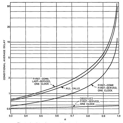
Fig. 4—Conditional average delay for M/D/1 vs occupancy.
