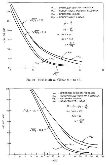
Fig. 11—MSE in dB vs  $\sqrt{2\beta}$  for E = 100 dB.
