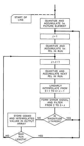
Fig. 6—Flow diagram for the element processing of the free-running interpolative algorithm. I denotes the last element in the previous run, J denotes the current length of the run being processed, and I + J denotes the element being currently processed.
