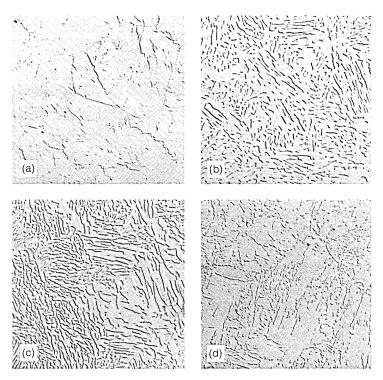
Fig. 5—Quenched microstructures of 3.0% V-6.35-mm Remendur rod in hot-rolled and various annealed conditions; etched; DIC; 600X. (a) Hot-rolled. (b) Annealed;  $\frac{1}{2}$  hour; 950°C. (c) Annealed;  $\frac{1}{2}$  hour; 925°C. (d) Annealed;  $\frac{1}{2}$  hour; 900°C.
