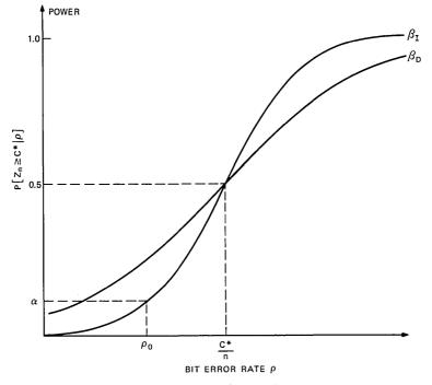
Fig. 1-Comparison of power functions.
