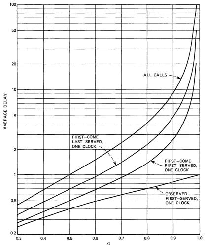
Fig. 1—Average delay for M/M/1 vs occupancy.
