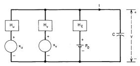
Fig. 2—Frequency converter with nonlinear capacitor C.
