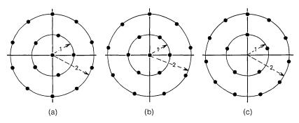
Fig. 10—New signal constellations: (a) 1–5–10,  $p_{\text{peak}}/p_{\text{av}} = 1.42$ ; (b) 1–6–9,  $p_{\text{peak}}/p_{\text{av}} = 1.525$ ; (c) 5–11,  $p_{\text{peak}}/p_{\text{av}} = 1.31$ .
