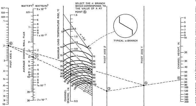
Fig. 10—Nomogram for evaluation of maximum wall temperature increase,  $r_H = 1$  (from Aung, Kessler, and Beitin<sup>7</sup>).
