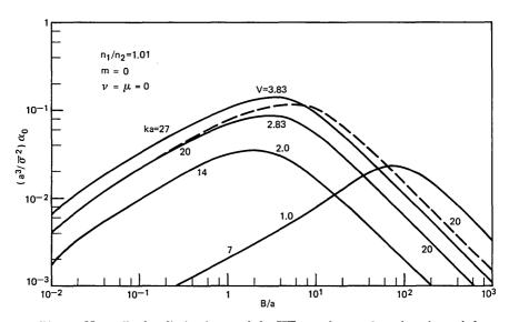
Fig. 2—Normalized radiation losses of the HE<sub>11</sub> mode,  $\nu = 0$ , as functions of the ratio of correlation length B to core radius a for different values of  $ka = 2\pi a/\lambda$  for pure diameter changes, m = 0.  $n_1/n_2 = 1.01$ . The dotted line results from using only "free space" radiation modes.
