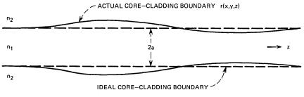
Fig. 1—Sketch of a fiber with distorted core-cladding interface.
