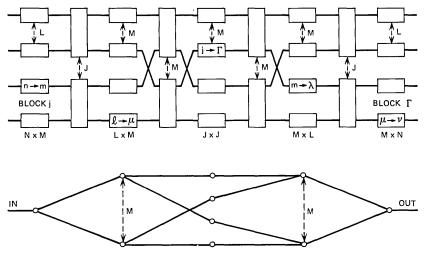
Fig. 5—Cross-connected five-stage network.
