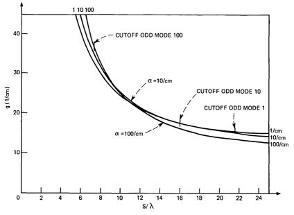
Fig. 10—Threshold gain as function of stripe widths for different attenuation  $\alpha$  in the side regions.  $\alpha_M = 12.5$ /cm.
