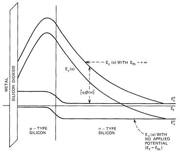
Fig. 8—Band diagram for buried-channel device.
