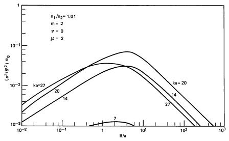
Fig. 3—HE<sub>11</sub> mode radiation losses caused by elliptical deformations, m = 2, of the core-cladding boundary.  $n_1/n_2 = 1.01$ .
