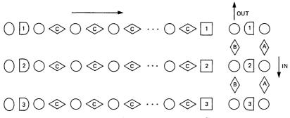
Fig. 10-Recirculating memory array for TSI gates.
