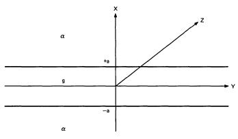
Fig. 1-Cross section of slab waveguide.
