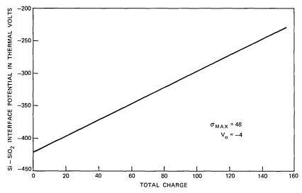
Fig. 7—Potential at the Si-SiO<sub>2</sub> interface versus total positive charge in a buriedchannel device with a Gaussian p-region doping profile and  $V_o = -4$  volts.
