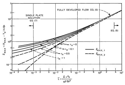
Fig. 3—Relation between dimensionless maximum wall temperature rise and the dimensionless parameter  $\tilde{L}$  (from Aung, et al.<sup>6</sup>).
