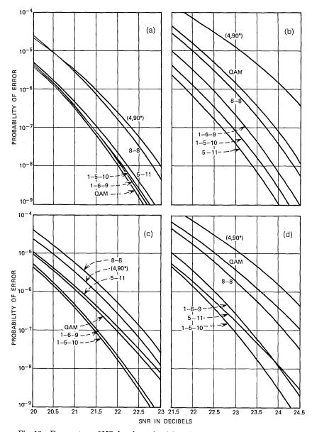
Fig. 13—Error rate vs SNR for channels with and without phase jitter; Gaussianoptimum receiver is assumed to have a phase-locked loop: (a) no jitter, average power constraint; (b) no jitter, peak power constraint; (c) rms jitter = 1.5 degrees, average power constraint; (d) rms jitter = 1.5 degrees, peak power constraint.
