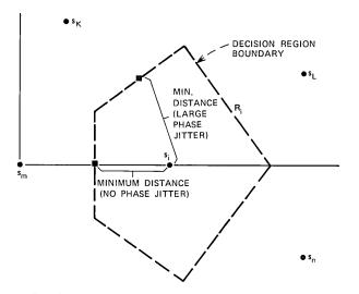
Fig. 7—Typical decision region about signal point  $s_i$ , with minimum distances to boundary shown for Gaussian noise alone (no phase jitter) and for large jitter (angular displacements highly likely).
