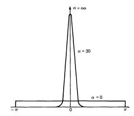
Fig. 5—Tikhonov phase jitter density  $p(\phi) = \exp(\alpha \cos \phi)/2\pi I_o(\alpha)$ .
