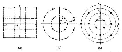
Fig. 9—Existing signal constellations: (a) quadrature amplitude modulation (QAM),  $p_{\text{peak}}/p_{\text{av}} = 1.8$ ; (b) modified AM-PM (8-8),  $p_{\text{peak}}/p_{\text{av}} = 1.43$ ; (c) circular constellation, (4, 90°)  $p_{\text{peak}}/p_{\text{av}} = 1.85$ .
