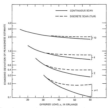
Fig. 6—Comparison of the standard deviation of peakedness estimates using discrete-scan and continuous-scan measurements of carried load on a 40-trunk group.
