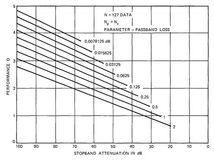
Fig. 11—Plots of *D* versus  $20 \log_{10} \delta_2$  for various values of the parameter  $20 \log_{10} (1/1 - \delta_p)$ , where  $\delta_p = 2\delta_1/(1 + \delta_1)$ , as calculated from the optimum non-linear fits to the data of Fig. 8 (N = 127).
