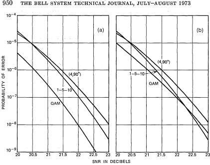
Fig. 15—Probability of error vs SNR for Gaussian-optimum receiver with "practical" decision region boundaries for the 1-5-10 constellation and with phase-locked loop: (a) no jitter, average power constraint; (b) rms jitter = 1.5 degrees, average power constraint.
