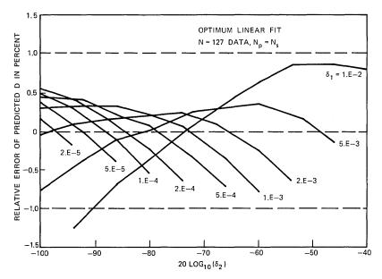
Fig. 9—The relative errors in fitting the data of Fig. 8 with a linear curve over the range  $\delta_1 \leq 0.01$ , for various values of  $\delta_1$  (N = 127).
