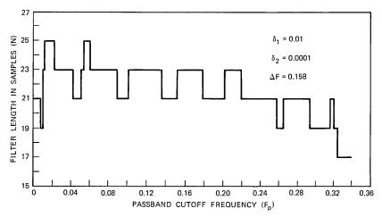
Fig. 14—Optimum values of N to meet given design specifications on  $\delta_1$ ,  $\delta_2$ , and  $\Delta F$ , as a function of  $F_p$ .
