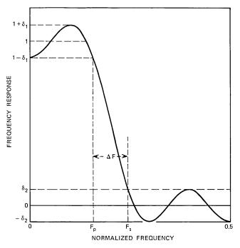
Fig. 1—Definition of low-pass filter parameters.
