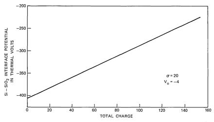
Fig. 4—Potential at the Si-SiO<sub>2</sub> interface versus total positive charge in a buriedchannel device with a uniform p-region and  $V_o = -4$  volts.
