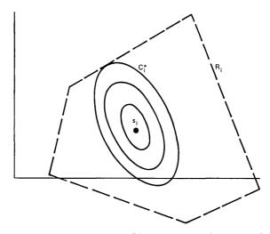
Fig. 8—Nested equidistance contours [distance defined by eq. (13)] about signal  $s_i$  in arbitrary decision region. Contour  $c_i^*$ , at distance  $d_i^*$ , defines  $d_i^*$  as the shortest distance to the boundary.
