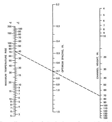
Fig. 13.—Nomogram for evaluation of optimum spacing,  $r_H = 1$  (from Aung, Kessler, and Beitin<sup>7</sup>).
