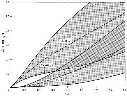
Fig. 2—Delay and time spread of the fiber output on axis and at an angle  $\theta = \Theta_{\infty}$ .
