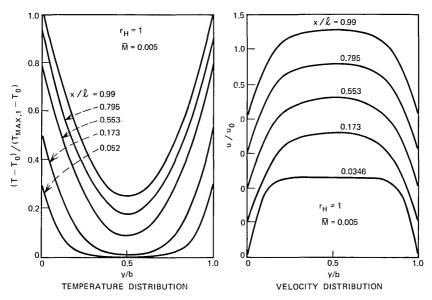
Fig. 5—Typical temperature and velocity distributions in a channel having developing flow.
