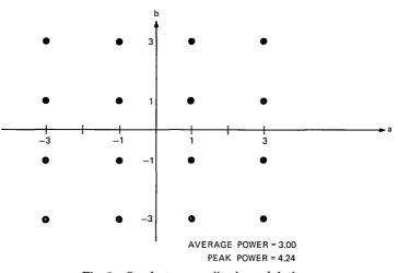
Fig. 3-Quadrature amplitude modulation.
