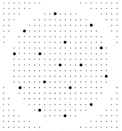
Fig. 19—Optimum signal constellation: Peak SNR = 27 dB, 1.5 degrees rms jitter (courtesy of B. W. Kernighan and S. Lin).
