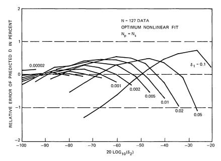
Fig. 10—The relative errors in fitting the data of Fig. 8 with a nonlinear curve over the range  $\delta_1 \leq 0.1$ , for various values of  $\delta_1$  (N = 127).
