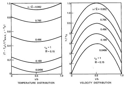
Fig. 4—Typical temperature and velocity distributions in a channel having nearly fully developed flow.
