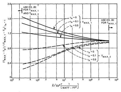
Fig. 9—Maximum wall temperature rise as a function of the quantity  $\ell/\tilde{q}b^{5}$ .
