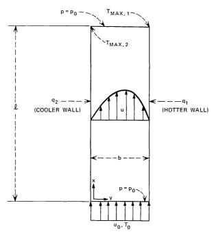
Fig. 2-Two-dimensional vertical channel model.
