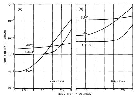
Fig. 14—Probability of error for receiver with "practical" decision region boundaries for the 1-5-10 constellation and with phase-locked loop: (a) average power constraint; (b) peak power constraint.
