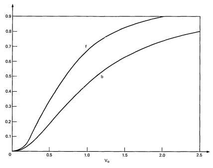
Fig. 6—b(v) for lowest-order even mode in a refractive slab guide and loss-weighing function  $f(v_0)$  for lowest-order even mode.
