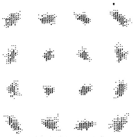
Fig. 4-Received signal points in a QAM system.
