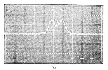
Fig. 8—Linear scan of nearfield distribution of stripe geometry lasers with stripe width of  $\sim 12 \ \mu m$ . One division  $\approx 3.7 \ \mu m$ . Current in both cases is  $\sim 20$  percent above threshold.
