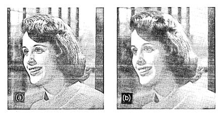
Fig. 1—(a) Original photograph; (b) Reconstruction of (a) via TAPEX, using 10 bits per picture-element.
