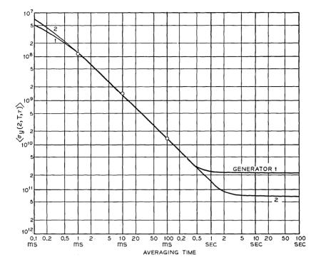
Fig. 7-Stability of two frequency generators, ten-foot cable.
