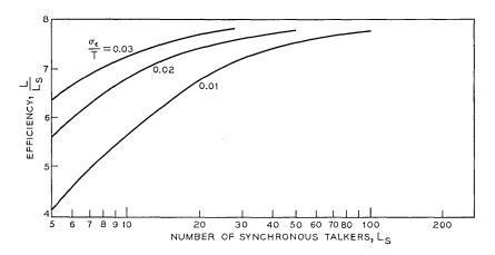
Fig. 6—Efficiency versus number of synchronous talkers for peak-to-average voltage ratio A = 8.
