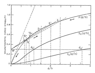
Fig. 10—Construction of solutions to the force equation in the presence of coercivity, l/h = 0.3,  $H/4\pi M_s = 0.2544$ ,  $H_c/4\pi M_s = 0.020$ .
