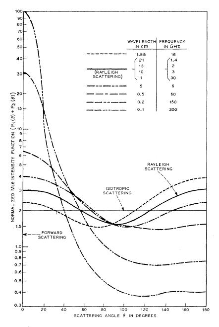
Fig. 3—Intensity versus scattering angle, rain rate = 50 mm/hr.
