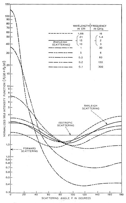
Fig. 2—Intensity versus scattering angle, rain rate = 100 mm/hr.
