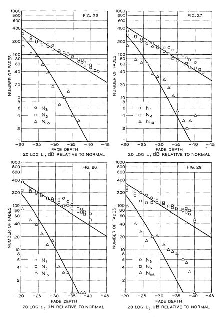
Fig. 26—Number of fades in test period (4-GHz band,  $\Delta f = 80$  MHz). Fig. 27—Number of fades in test period (4-GHz band,  $\Delta f = 100$  MHz). Fig. 28—Number of fades in test period (4-GHz band,  $\Delta f = 160$  MHz). Fig. 29—Number of fades in test period (4-GHz band,  $\Delta f = 160$  MHz).
