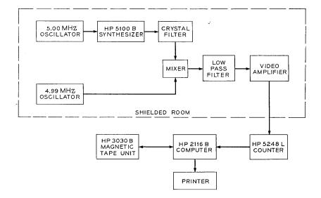
Fig. 3—Measurement system used for comparison of  $\langle \sigma_y(N, T, \tau) \rangle$  and  $\langle \sigma_y(2, T, \tau) \rangle$ .
