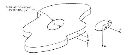
Fig. 1-Physical geometry and coordinate system for calculating spreading resistance.
