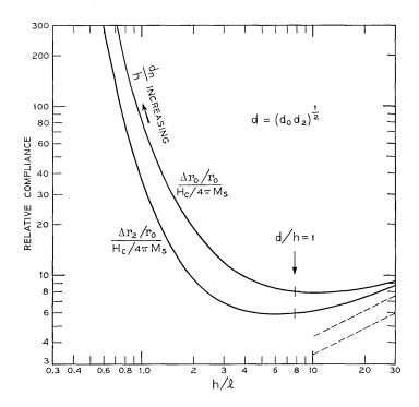
Fig. 13—Radial and elliptical relative compliance functions as a function of the thickness, h, measured in units of the characteristic length, l, for the bias condition  $d = (d_0d_2)^{\frac{1}{2}}$ .
