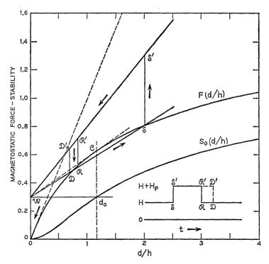
Fig. 11—Construction used in the pulsed bias field mobility method, l/h = 0.3,  $H/4\pi M_s = 0.254$ ,  $(H + H_F)/4\pi M_s = 0.500$ .
