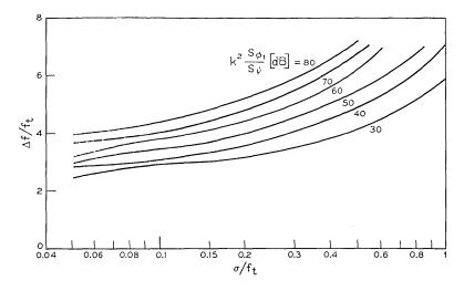
Fig. 6—Receiver filter only. Signal-to-noise from bandlimiting = 90 dB.
