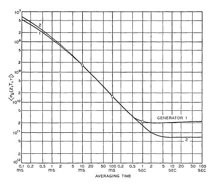
Fig. 8-Stability of two frequency generators, 200-foot cable.
