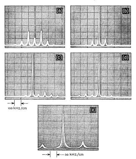
Fig. 2—Spectra of the injected signal and the oscillator output signal: (a) injected signal spectrum, (b) output signal with locking at  $\omega$ , (c) output signal with locking at  $\omega - \Omega$ , (d) output signal with locking at  $\omega + \Omega$ , and (e) output signal just before locking. ( $\theta \approx \pi/2 \sin \Omega t$ ,  $\Omega = 2\pi \times 100$  kHz,  $\Delta \omega_L \approx 2\pi \times 10$  kHz,  $F_0 = 35$  MHz)
