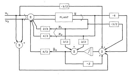
Fig. 6-Example of a controlled system.
