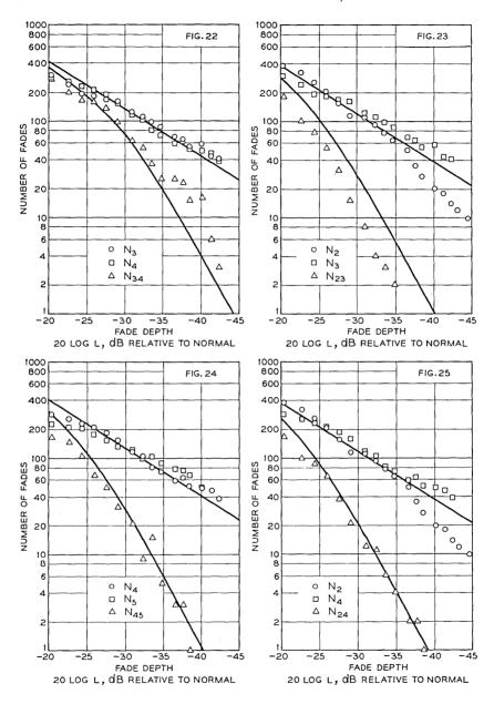
Fig. 22—Number of fades in test period (4-GHz band,  $\Delta f = 20$  MHz). Fig. 23—Number of fades in test period (4-GHz band,  $\Delta f = 60$  MHz). Fig. 24—Number of fades in test period (4-GHz band,  $\Delta f = 60$  MHz). Fig. 25—Number of fades in test period (4-GHz band,  $\Delta f = 80$  MHz).
