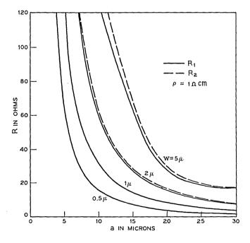
Fig. 6—Spreading resistances  $R_1$  and  $R_2$  for 1  $\Omega$  cm material.
