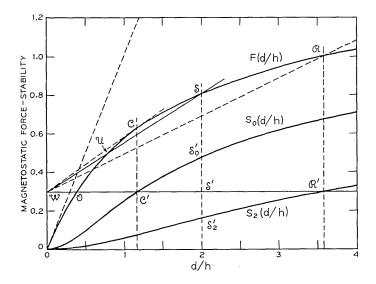
Fig. 2—Construction of solutions to the force equation for l/h = 0.3,  $d = d_0$ ,  $d = d_2$  and d = 2h.
