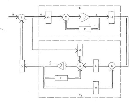
Fig. 3—The structure of a complete "controller."
