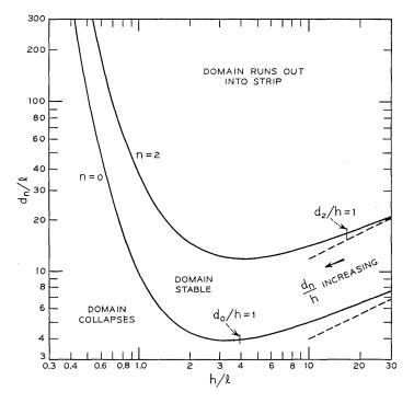
Fig. 4—Diameters of radial and elliptical metastability,  $d_0$  and  $d_2$ , in units of the characteristic length, l, as a function of the thickness, h, in units of l.
