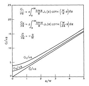
Fig. 4—Spreading conductances with and without fringing between disk and grounded back plane and between disk and grounded disk on back plane.
