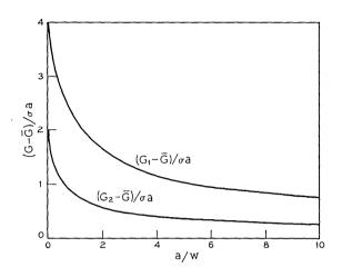
Fig. 5-Spreading conductance fringing components.
