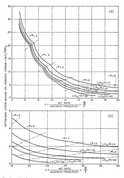
Fig. 3a and b—Performance curves. (Notes: 1. For analog implementation, use K = 1; delay = (L + 1) h. 2. For digital implementation, K = (T/Lh + 2)/(T/Lh + 1); delay = T + Lh. 3.  $\nu^*$  is the optimized number of bits per sample. 4. The optimum sampling rate is  $1/h = B/\nu^*$ .)
