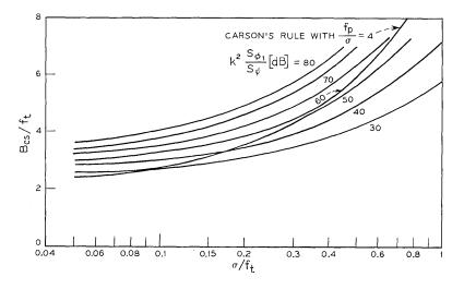
Fig. 8-Minimum channel spacing formula.
