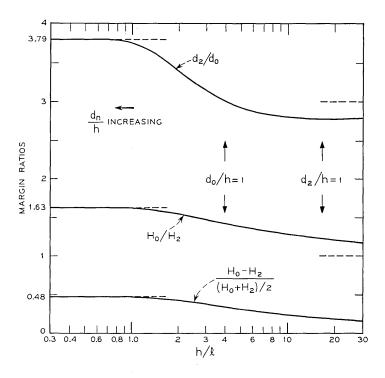
Fig. 5—Diameter and applied field margin ratios,  $d_2/d_0$ ,  $H_0/H_2$ , and  $2(H_0 - H_2)/(H_0 + H_2)$ , as functions of the thickness, h, measured in units of the characteristic length, l.
