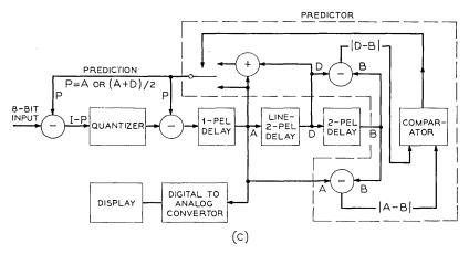
Fig. 4a—Diagram of apparatus used to evaluate coder (i) in which the value (A + D)/2 is used as a prediction of the current picture element. The displayed picture is equivalent to the received picture providing there are no channel errors. Fig. 4b—Apparatus used to evaluate coder (u) in which A + (D - B)/2 is
