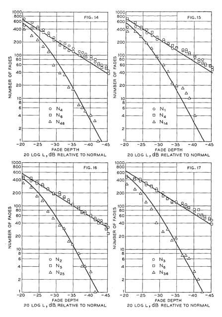
Fig. 14—Number of fades in test period (6-GHz band,  $\Delta f = 90$  MHz). Fig. 15—Number of fades in test period (6-GHz band,  $\Delta f = 120$  MHz). Fig. 16—Number of fades in test period (6-GHz band,  $\Delta f = 120$  MHz). Fig. 17—Number of fades in test period (6-GHz band,  $\Delta f = 120$  MHz).
