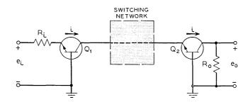
Fig. 1—Current transmission circuit for switching networks (assume  $\alpha \rightarrow 1$ ).
