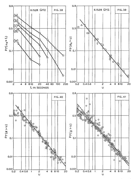
Fig. 38—Probability that duration of fade is longer than a given number of seconds for five fade depths [20 log L is: (a) -22.7 dB, (b) -27.6 dB, (c) -32.4 dB, (d) -37.6 dB, (e) -43.2 dB]. Fig. 39—Probability that duration of fade, normalized to its mean, is longer
