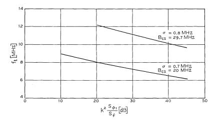
Fig. 9—Maximum top baseband frequency as a function of normalized adjacent channel interference noise.
