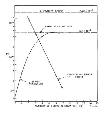
Fig. 2—Comparison of series expansion method with Chernoff Bound and exhaustive method. [SIN  $\pi t/T$ ]/( $\pi/T$ )t pulse, 5-pulse truncation approximation,  $t_0 = 0.05T$ , (S/N) = 24 dB.
