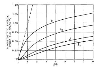
Fig. 3—The magnetostatic energy per unit wall length function, J, the magnetostatic force function, F, and the magnetostatic stability functions,  $S_0$  and  $S_2$ , as functions of the diameter-to-thickness ratio.
