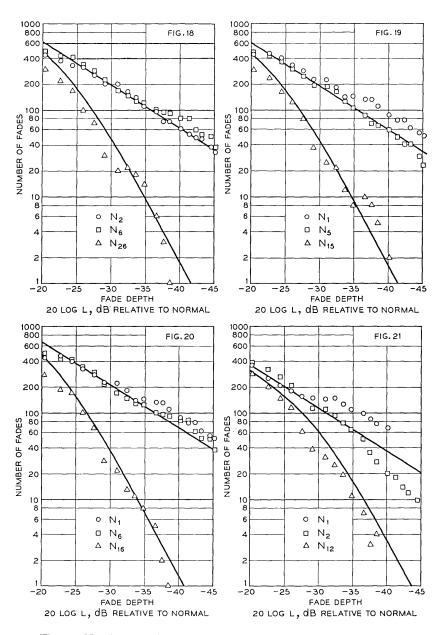
Fig. 18—Number of fades in test period (6-GHz band,  $\Delta f = 150$  MHz). Fig. 19—Number of fades in test period (6-GHz band,  $\Delta f = 180$  MHz). Fig. 20—Number of fades in test period (6-GHz band,  $\Delta f = 210$  MHz). Fig. 21—Number of fades in test period (4-GHz band,  $\Delta f = 20$  MHz).
