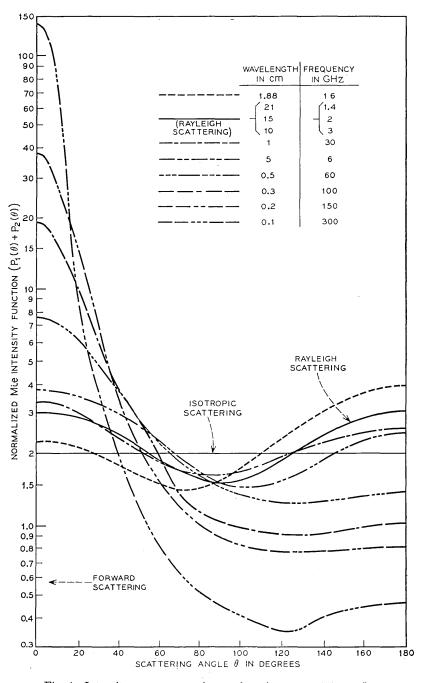
Fig. 1—Intensity versus scattering angle, rain rate = 150 mm/hr.
