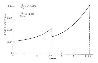
Fig. 8—Error spectrum for T = 1/2,  $\sigma_{\Delta}/T = 0.316$ . Undistorted spectrum is one for  $-\pi \leq \omega \leq \pi$ , and zero otherwise. S/N $_{\pi} = 18.5$  dB, S/N $_{2\pi} = 14$  dB.
