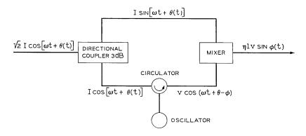
Fig. 1-Scheme of the digital demodulator for coherent phase detection.
