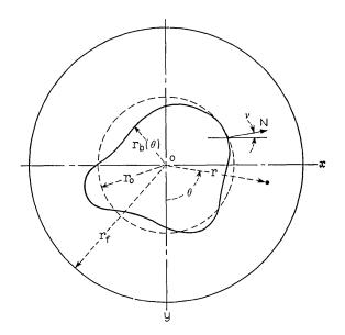
Fig. 9-Coordinate system used in consideration of anisotropic wall energy.
