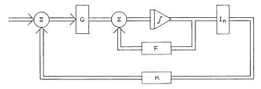
Fig. 2—Feedback control when the state is known.
