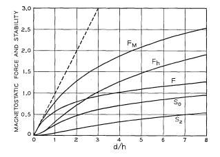
Fig. 4—The transverse magnetostatic force functions,  $F_M$ ,  $F_h$ , and  $F_H$  ( $F = F_H$ ) and the magnetostatic stability functions  $S_0$  and  $S_2$ , as functions of the diameter-to-thickness ratio.
