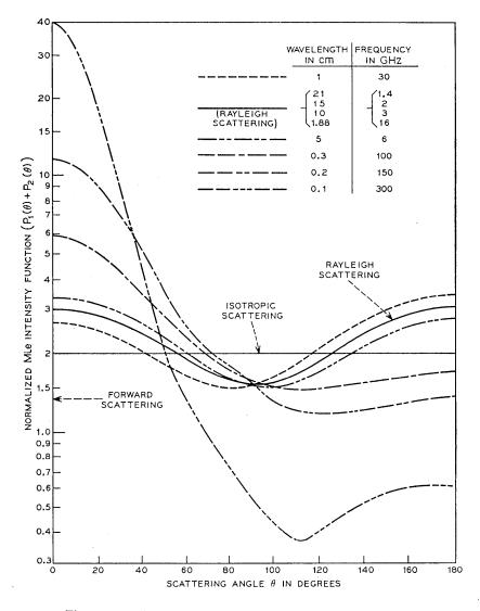
Fig. 4—Intensity versus scattering angle, rain rate = 1 mm/hr.
