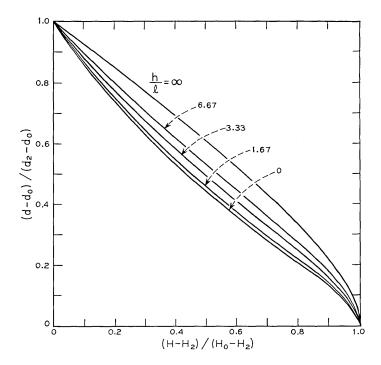
Fig. 8—Relative diameter,  $(d - d_0)/(d_2 - d_0)$ , as a function of relative applied field,  $(H - H_2)/(H_0 - H_2)$ , in the infinite plate for various values of the plate thickness, h, measured in units of the characteristic length, l.
