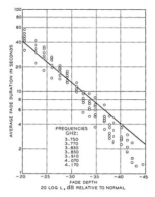
Fig. 5—Summary of the average fade durations of the seven single signals in the 4-GHz band (equation of theoretical line is  $\langle \alpha \rangle = 408 L$ ).
