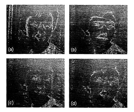
Fig. 5—Magnitude of the difference between a picture coded as 8-bit PCM and: (a) the reference coder; (b) coder (i) ([A + D]/2 is prediction); (c) coder (v) ([A + (D - B)/2] is prediction); (d) optional prediction coder of Fig. 4c.
