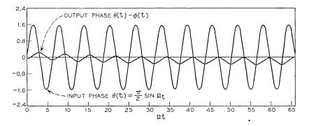
Fig. 3—Phase of the oscillator output signal for an injected signal phase modulated by  $\theta(t) = \pi/2 \sin \Omega t$ .  $[(\Delta \omega_L)/\Omega = 0.1, (\omega - \omega_0)/\Omega = -0.01, \theta_0 = \pi/2.]$
