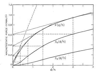
Fig. 3—Construction of the  $S_0(d/h)$  function as a sequence of collapse diameter solutions.
