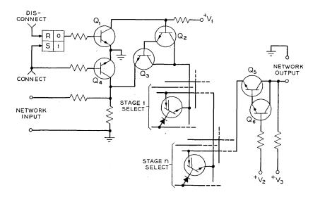
Fig. 2. — Thyristor network using current transmission.
