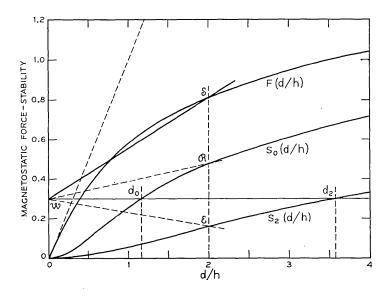
Fig. 12—Construction of the radial and elliptical relative compliance functions for l/h = 0.3, d/h = 2.
