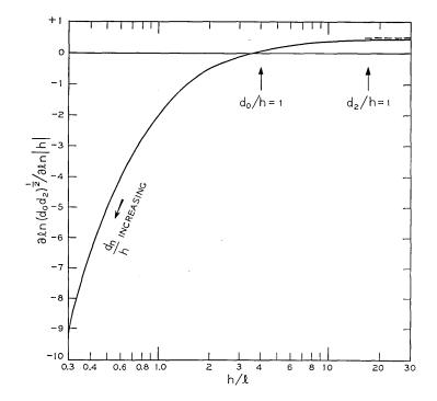
Fig. 6—Logarithmic derivative of the domain diameter with respect to plate thickness,  $\partial \ln d/\partial \ln |h|$ , for the bias condition  $d = (d_0 d_2)^{\frac{1}{2}}$  as a function of the plate thickness, h, measured in units of the characteristic length, l.
