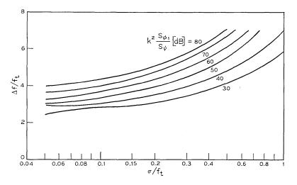
Fig. 4—Receiver filter only. Signal-to-noise from bandlimiting = 70 dB.
