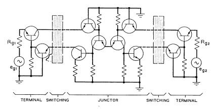
Fig. 4 — Combining two hybrid-transmission circuits in a switching network.
