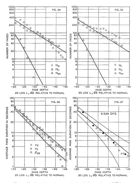
Fig. 34—Number of fades in test period (4-GHz band,  $\Delta f = 400$  MHz). Fig. 35—Number of fades in test period (4-GHz band,  $\Delta f = 420$  MHz). Fig. 36—Average durations of simultaneous fades of signals at 6.0045 and 6.0342 GHz (the lines are theoretical)
