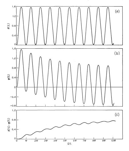
Fig. 4—Tracking angle and phase of the oscillator output signal for an injected signal phase modulated by  $\theta(t) = (\pi/2) \sin^2 \Omega t$  with  $(\Delta \omega_L)/\Omega = 0.1$ . (a) Phase of the input signal, (b) tracking angle, (c) phase of the oscillator output signal.
