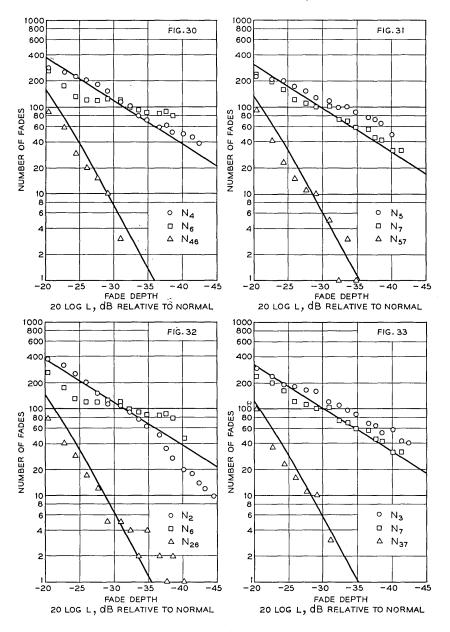
Fig. 30—Number of fades in test period (4-GHz band,  $\Delta f = 220$  MHz). Fig. 31—Number of fades in test period (4-GHz band,  $\Delta f = 260$  MHz). Fig. 32—Number of fades in test period (4-GHz band,  $\Delta f = 300$  MHz). Fig. 33—Number of fades in test period (4-GHz band,  $\Delta f = 340$  MHz).
