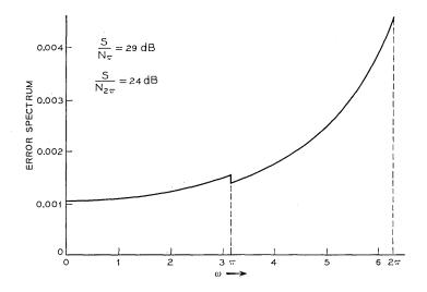
Fig. 9—Error spectrum for T = 1/2,  $\sigma_{\Delta}/T = 0.1$ . Undistorted spectrum is one for  $-\pi \leq \omega \leq \pi$ , and zero otherwise. S/N<sub> $\pi$ </sub> = 29 dB, S/N<sub>2 $\pi$ </sub> = 24 dB.
