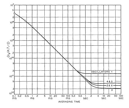
Fig. 6-Short-term stability of six precision oscillators.
