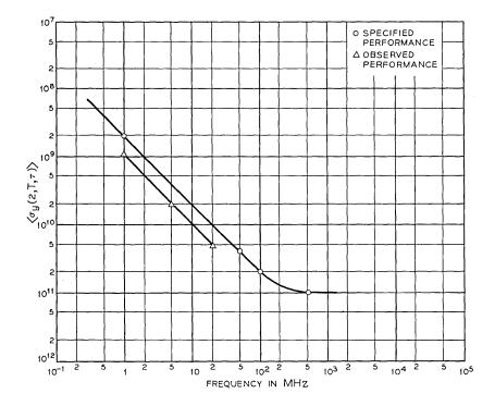
Fig. 9-Performance of frequency synthesizer, one-second averaging time.
