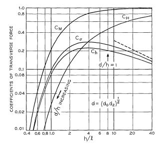
Fig. 5—The transverse force coefficients  $C_h$ ,  $C_H$ ,  $C_M$ , and  $C_\sigma$  for the bias condition  $d = (d_0 d_2)^{\frac{1}{2}}$ , as functions of the normalized thickness, h/l.
