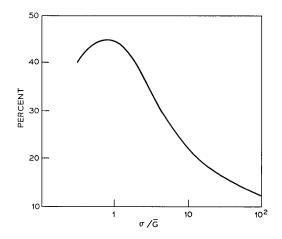
Fig. 7—Percent by which upper bound exceeds lower bound vs  $\sigma/\tilde{G}$  for unilateral gain diode. Percent =  $((\Lambda_U - \Lambda_L)/\Lambda_L) \times 100$ .
