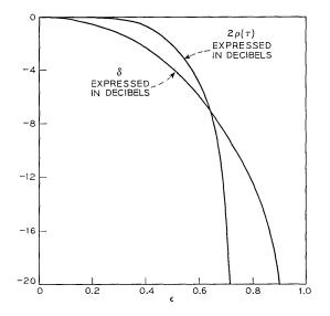
Fig. 8—Contrast ratio and pulse degradation as functions of epsilon.
