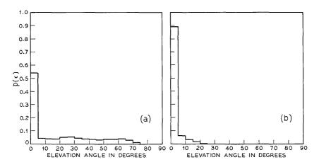
Fig. 12—Interference density vs. elevation angle into CCIR reference system centered at (a) 20° latitude and (b) 70° latitude. Satellite spacing =  $6^{\circ}$ .
