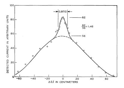
Fig. 6-Experimental results for a mode-locked He-Ne laser.
