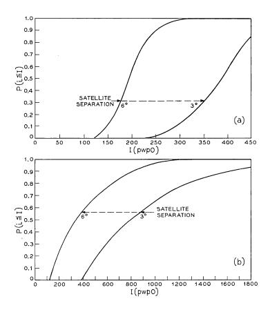
Fig. 10—Distribution of interference into CCIR reference systems centered at  $70^{\circ}$  latitude with (a)  $2^{\circ}$  pointing restriction, and (b) no restriction.
