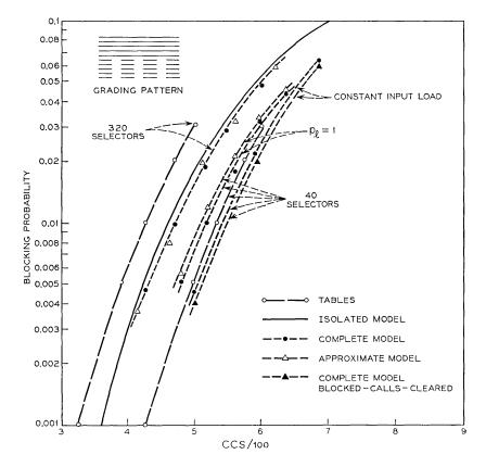
Fig. 3-Load-loss relations for a 25-trunk graded multiple.
