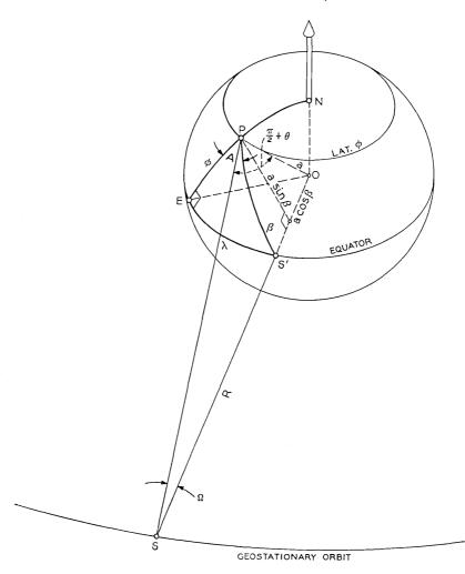
Fig. 2-Geometry of the geostationary orbit and a radio-relay station.
