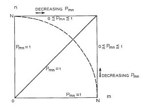
Fig. 11—Values of  $p_{mn}$  are shown projected onto the m-n plane. If  $N \to \infty$  then the  $N \times N$  square domain of definition for  $p_{mn}$  may be replaced by the dashed circle of radius N.
