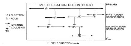
Fig. 1—Model of equal ionization device.
