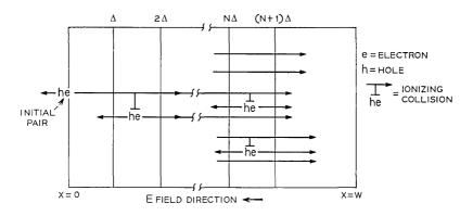
Fig. 2-Model of unilateral gain device.
