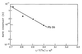
Fig. 14—Rate constant (k) on log scale vs 1/T (°K) for  $5-5/8'' \times 5-7/8'' \times 1/4''$  thick PbSb grids.
