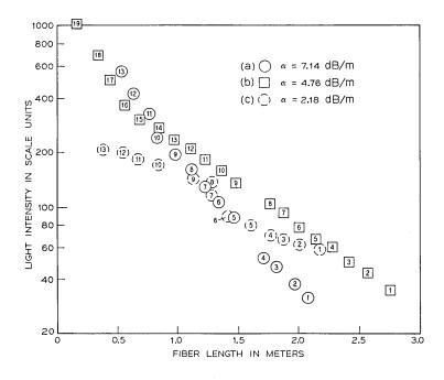
Fig. 8—(a, b) Transmission loss measurements along two different 13  $\mu$ m unclad fibers immersed in oil ( $\Delta = 2.44\%$ ). (c) Transmission loss measurements along a 3 $\mu$ m clad fiber.
