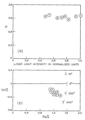
Fig. 7—The state of polarization of a  $28\mu m$  unclad fiber ( $L = 30 \text{ cm}, \Delta = 2.44\%$ ) analysed as a function of input power: (a) p vs normalized laser light power, (b)  $\bar{Q}$  is plotted in the complex plane with light power as the parameter. The points are numbered sequentially to correspond to the points of (a) reading from right to left.
