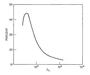
Fig. 8-Percent by which upper bound exceeds lower bound vs lower bound for unilateral gain diode.
