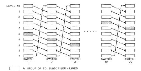
Fig. 10-Slipped multiple on terminal banks of line-finder switches.
