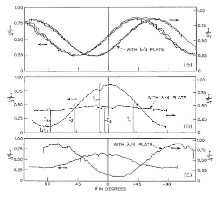
Fig. 6—Sample profiles of  $I/S_T$  vs  $\theta$  for partially polarized light leaving: (a)  $19\mu$ m clad fiber (L = 301 cm,  $\Delta = 0.824\%$ ), (b)  $28\mu$ m unclad fiber (L = 238 cm,  $\Delta = 2.44\%$ ), and (c)  $28\mu$ m unclad fiber (L = 197 cm,  $\Delta = 0.56\%$ ).
