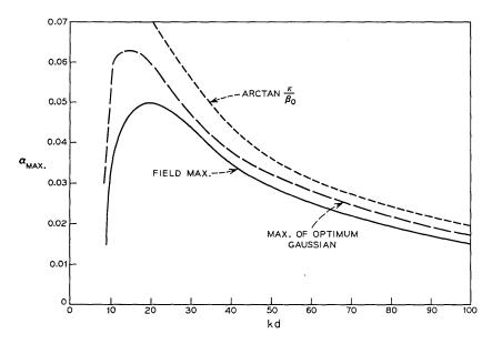
Fig. 5—Location of the peak of the radiation pattern. The solid curve indicates the maxima of the curves of Fig. 4; the dotted curve represents the direction of travel of the plane waves whose superposition comprise the guided mode; the dash-dotted curve indicates the location of the field maxima of the optimum gaussian distribution used to excite the waveguide.
