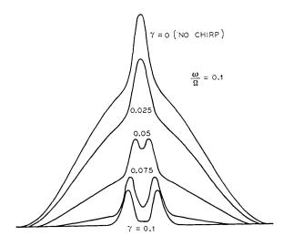
Fig. 4— $U(\tau)$  for a gaussian pulse with various amounts of chirp.
