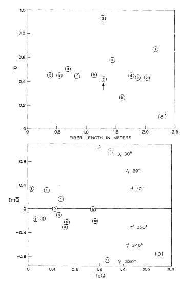
Fig. 10—Analyses of the states of polarization along a  $3\mu$ m clad fiber ( $\Delta = 0.824\%$ ): (a) p vs fiber length. The notation  $\uparrow$  refers to a bright spot indicative of a gross defect within the core or at the core cladding interface. (b) Q is plotted in the complex plane with fiber length as the parameter. The points are numbered sequentially to correspond to the points of (a) and Figure 8c reading from right to left.
