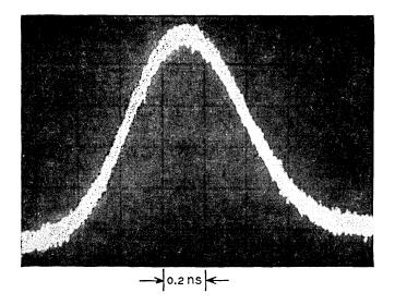
Fig. 7-Mode-locked pulse from He-Ne laser.
