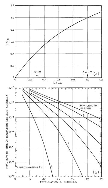
Fig. 3—(a) Attenuation as a function of hop length at constant probability using equation (2) with  $\rho = 0.543$ . (b) Probability distributions of rain attenuation with hop length as a parameter using approximating function B and equation (2) with  $\rho = 0.543$ .
