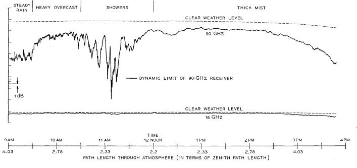
Fig. 2-Logarithmic record of 90-GHz and 16-GHz attenuation for December 8, 1969.
