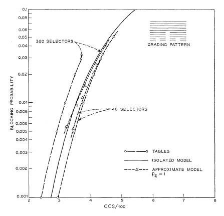
Fig. 7-Load-loss relations for a 19-trunk graded multiple.
