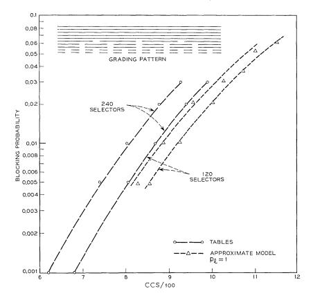
Fig. 9-Load-loss relations for a 45-trunk graded multiple.
