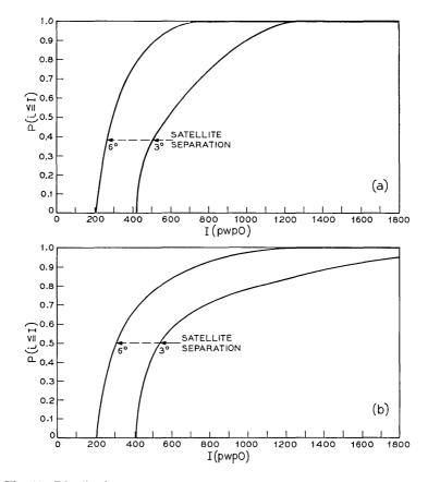
Fig. 11—Distribution of interference into 140-hop systems centered at  $40^{\circ}$  latitude with (a)  $2^{\circ}$  pointing restriction, and (b) no restriction.
