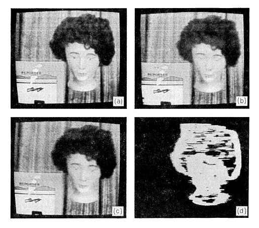
Fig. 3—(a) Fully sampled picture showing stationary head. (b) Fully sampled picture showing moving head. (c) Subsampled (2:1) picture using exchanged resolution. (d) Flags showing area deemed moving. Glossy prints of this figure may be obtained by writing to the authors.
