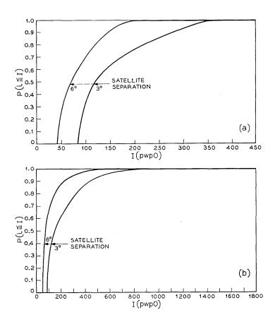
Fig. 6—Distribution of interference into CCIR reference system centered at 30° latitude with (a) 2° pointing restriction, and (b) no restriction.
