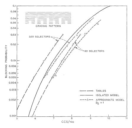
Fig. 8-Load-loss relations for a 37-trunk graded multiple.
