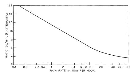
Fig. 3-Expected ratios of 90- to 16-GHz attenuation for different rain rates.
