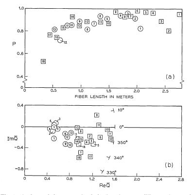
Fig. 9—Analyses of the states of polarization along two different  $13\mu$ m unclad fibers ( $\Delta = 2.44\%$ ): (a) p vs fiber length, and (b)  $\bar{Q}$  is plotted in the complex plane with fiber length as the parameter. The points are numbered sequentially to correspond to the points of (a) and Figure 8a, b reading from right to left.
