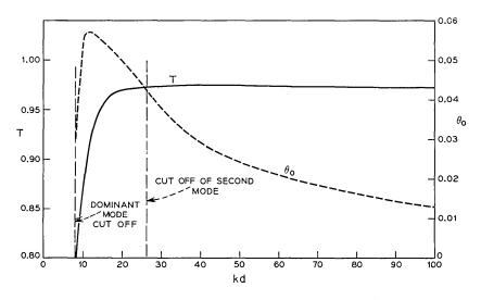
Fig. 7—Optimum transmission (excitation) coefficient T and optimum beam half width  $\theta_0$  of the exciting gaussian beam.
