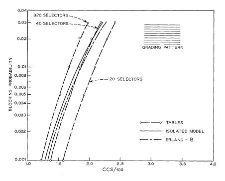
Fig. 5-Load-loss relations for the 11-trunk graded multiple.
