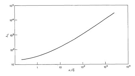
Fig. 6—Lower bound to required mean detected photons per pulse vs  $\sigma/\hat{G}$ .  $\sigma = \sqrt{N_0T}$ .
