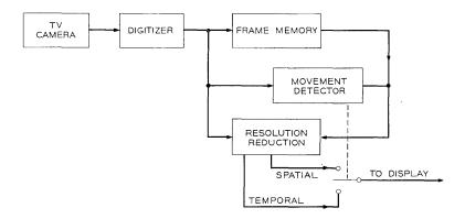
Fig. 1—System for resolution exchange.
