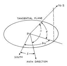
Fig. 3—Geometry determining the off-beam angle to a satellite.
