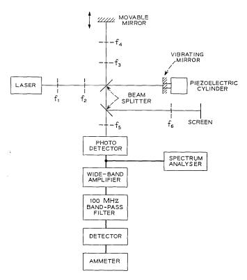
Fig. 1—Diagram of the BFD apparatus.
