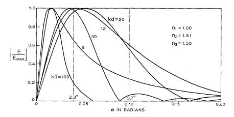
Fig. 4—Ratio of  $E_{\tau}$  over the peak value of the electric vector of the radiation field as a function of the angle in radians.  $n_1 = 1.00$ ,  $n_2 = 1.51$ ,  $n_3 = 1.50$ .
