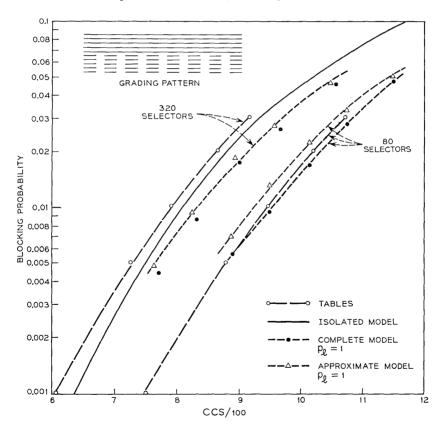
Fig. 4—Load-loss relations for a 45-trunk graded multiple.
