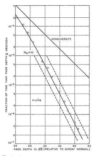
Fig. 16-GHz frequency diversity; 210-MHz separation,
