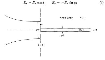
Fig. 1—Gaussian beam incident on the core of a dielectric fiber with refractive index n.
