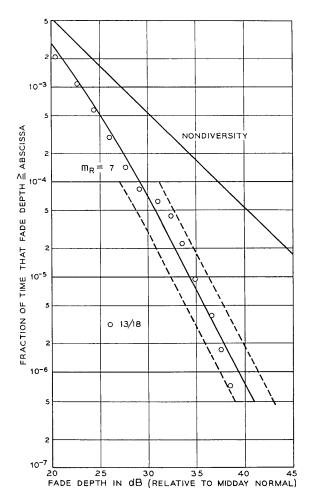
Fig. 14-6-GHz frequency diversity; 150-MHz separation.
