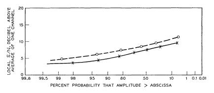
Fig. 8—CPD curves of a 2:4 array system. o, complex conjugate retransmission with maximal ratio reception; x, phase conjugate retransmission with equal gain reception.
