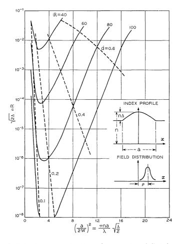
Fig. 3—Radiation loss in curved guides with truncated parabolic index profile.  $w = \sqrt{\frac{a\lambda}{\pi n\sqrt{8\Delta}}}$ ;  $d = \frac{2\rho}{a}$ ;  $\rho = \frac{a^2}{8\Delta R}$ .
