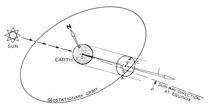
Fig. 13-Simplified geometry describing satellite eclipses.
