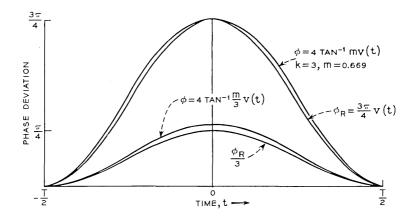
Fig. 6-Modulator input and output pulses.
