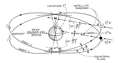
Fig. 8-Synchronous orbits phased for sun diversity.
