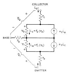
Fig. 3-Large signal dc transistor model.
