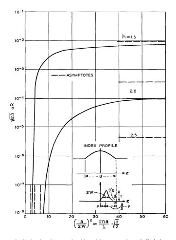
Fig. 5—Radiation loss in curved guides with truncated parabolic index profile.  $(\alpha/2) = \alpha$
