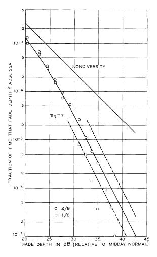
Fig. 18—4-GHz frequency diversity; 60-MHz separation.
