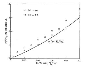
Fig. 2—The effect of the number of channels on the ratio of signal-to-second-order distortion.
