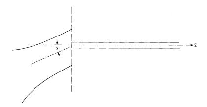
Fig. 3-Fiber excited by a tilted gaussian beam.
