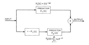
Fig. 3-Block diagram of the predictor for speech signals.
