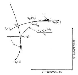
Fig. 12—An assumed fundamental admittance plane plot showing the angles  $\alpha_1$ ,  $\gamma_1$  and  $\theta_{10}$ . The device admittance is  $y_{11}(a_1)$  and the negative of the circuit admittance is  $-Y_1(\omega)$ . A similar diagram defines  $\alpha_2$ ,  $\gamma_2$  and  $\theta_{20}$  in the neighborhood of  $2\omega_0$ .
