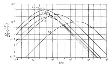
Fig. 9—Normalized radiation losses caused by random wall perturbations. The solid lines correspond to the dominant mode of the round guide, the dashed line represents the TE<sub>01</sub> mode of this waveguide. (n = 1.432.) The curve parameters are the values of ka.
