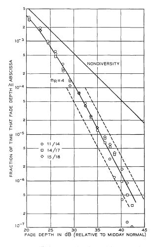
Fig. 12-6-GHz frequency diversity; 90-MHz separation.
