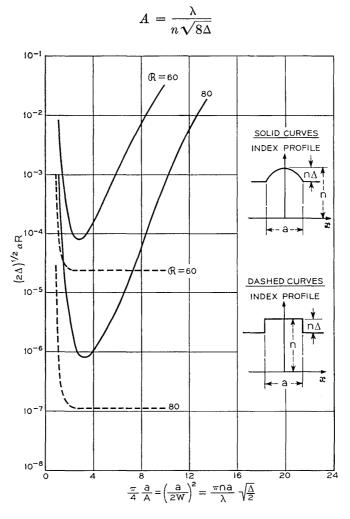
Fig. 4—Radiation loss in curved guides with truncated parabolic index profile (solid curves) and with rectangular index profile (dashed curves).
