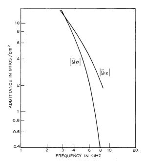
Fig. 8— $|\bar{y}_{12}|$  and  $|\bar{y}_{21}|$  versus frequency for  $V_1 = 10$  volts and  $V_2 = 1$  volt.
