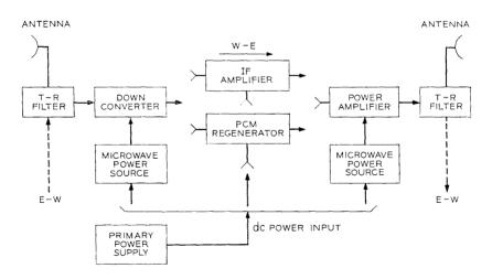
Fig. 9—Repeater of configuration for analog phase modulation or digital CPSK-PCM modulation.
