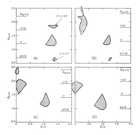
Fig. 16—Large-signal regions of stable  $\varphi_2$  versus  $\bar{\alpha}(\alpha_1 = \alpha_2 = \bar{\alpha})$  as obtained from the eigenvalues of the complete *B* matrix for the germanium oscillator example at (a) 3 GHz, (b) 4 GHz, (c) 5 GHz, and (d) 6 GHz; circuit variables  $D_1 = 50$ ,  $D_2 = 10$ ; diode variables  $V_1 = V_2 = 10$  volts,  $J_0 = 340$  A/cm<sup>2</sup>. This figure has  $\mu > 1$  everywhere except as noted.
