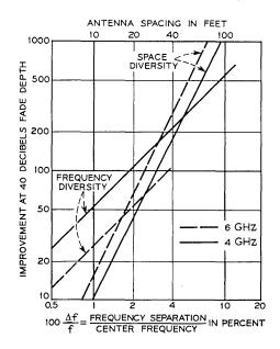
Fig. 33—Comparison of space and frequency diversity at a 40-dB fade depth.
