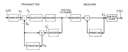
Fig. 1—Block diagram of a predictive coding system.
