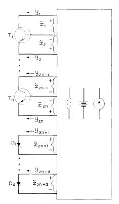
Fig. 1—Canonical form of a transistor network.
