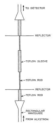
Fig. 4—Experimental resonant cavity set up to measure radiation losses of waveguide steps.
