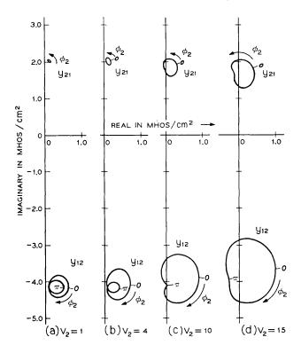
Fig. 5—Complex plane plot of  $y_{12}$  and  $y_{21}$  for  $V_1 = 10$  volts and  $V_2 = 2$ , 6, 10, 14 volts at 6 GHz, showing the relative insensitivity of  $y_{12}$  and  $y_{21}$  to changes in  $V_2$  and  $\varphi_2$  for moderate values of  $V_2$ .
