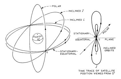
Fig. 4-Earth synchronous orbits and figure 8 patterns.
