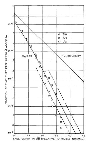
Fig. 19-4-GHz frequency diversity; 80-MHz separation.
