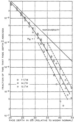
Fig. 10-6-GHz frequency diversity; 30-MHz separation.
