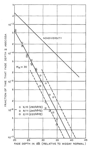
Fig. 22-4-GHz frequency diversity; 220/240/260-MHz separation.
