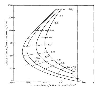
Fig. 2—The calculated large-signal single-frequency admittance of a 6-GHz germanium IMPATT diode at a bias current density  $J_0 = 340$  A/cm<sup>2</sup>.
