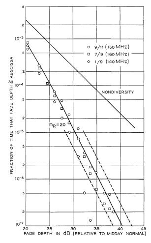
Fig. 21—4-GHz frequency diversity; 140/160-MHz separation.
