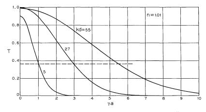
Fig. 7—Peak transmission coefficient T as a function of beam off-set.
