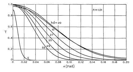
Fig. 8—Peak transmission coefficient as a function of tilt angle  $\alpha$ .
