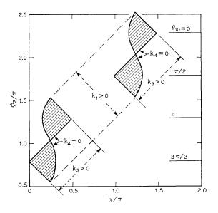
Fig. 13—Regions of stable  $\varphi_2$  versus  $\bar{\alpha}(\alpha_1 = \alpha_2 = \bar{\alpha})$  in the strongly coupled small-signal limit at 4 GHz;  $\mu \ll 1$ .
