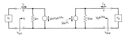
Fig. 1—Equivalent circuit of the IMPATT diode which includes nonzero voltages at two harmonically related frequencies. Port 1 is the fundamental port and port 2 is the second-harmonic port;  $y_{11}$  and  $y_{22}$  are the large-signal single-frequency diode admittances at the fundamental and second-harmonic frequencies, respectively.
