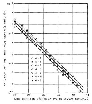
Fig. 6—Fade-depth distribution; 4-GHz channels.
