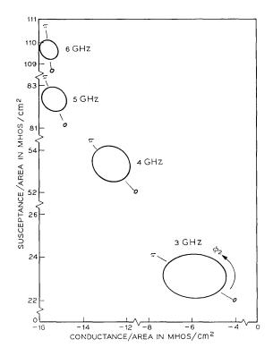
Fig. 3—The input admittance,  $Y_{in1}$ , at 3, 4, 5 and 6 GHz as it is modified by the presence of a second-harmonic voltage for  $V_1 = 10$  volts,  $V_2 = 1$  volt and  $J_0 = 340$  A/cm<sup>2</sup>.
