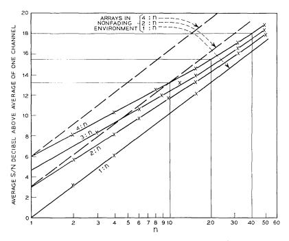
Fig. 4-Average S/N of complex conjugate retransmission arrays.
