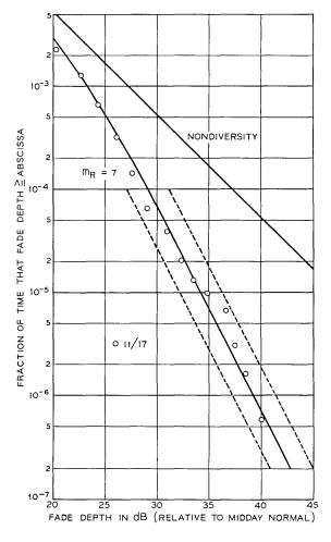
Fig. 15-6-GHz frequency diversity; 180-MHz separation.
