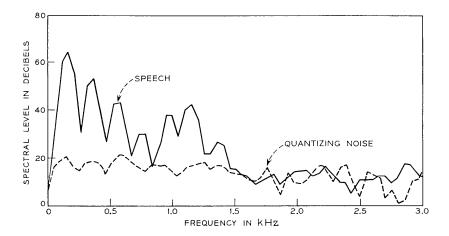
Fig. 6-Spectra of speech and quantizing noise.
