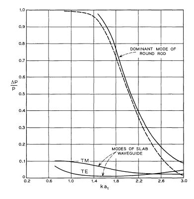
Fig. 2—Relative radiation loss caused by an abrupt step with  $a_2/a_1 = 0.5$  of the waveguide. The two curves labeled dominant mode of the round waveguide were obtained by the mode matching technique (dotted line) and by the radiation loss technique (solid line). The two curves at the bottom of the figure labeled TE and TM modes represent the step losses of the slab waveguide. The radius  $a_1$  (appearing in  $ka_1$ ) belongs to the larger waveguide section. Index of refraction n = 1.432.
