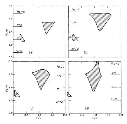
Fig. 15—Large-signal regions of stable  $\varphi_2$  versus  $\bar{\alpha}(\alpha_1 = \alpha_2 = \bar{\alpha})$  as obtained from the eigenvalues of the complete *B* matrix for the germanium oscillator example at (a) 3 GHz, (b) 4 GHz, (c) 5 GHz, and (d) 6 GHz; circuit variables  $D_1 = 50$ ,  $D_2 = 500$ ; diode variables  $V_1 = V_2 = 10$  volts,  $J_0 = 340$  A/cm<sup>2</sup>. This figure has  $\mu < 1$  everywhere.
