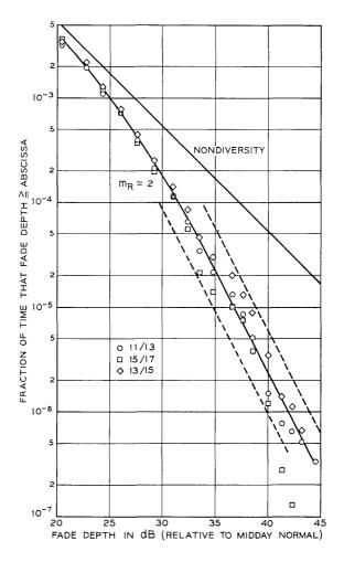
Fig. 11-6-GHz frequency diversity; 60-MHz separation.
