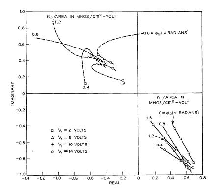
Fig. 6—Complex plane plot of  $K_1 = y_{12}/V_1$  and  $K_2 = y_{21}/V_1$  as a function of  $V_1$  for various values of second-harmonic phase  $\varphi_2$ , at 4 GHz.
