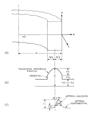
Fig. 1—(a) Two-dimensional truncated parabolic guide; (b) Refractive index profile; (c) Electric field distribution of the fundamental mode.
