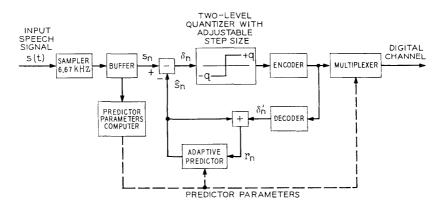
Fig. 4-Transmitter of the predictive coding system.
