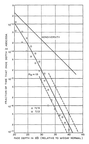
Fig. 20-4-GHz frequency diversity; 100-MHz separation.
