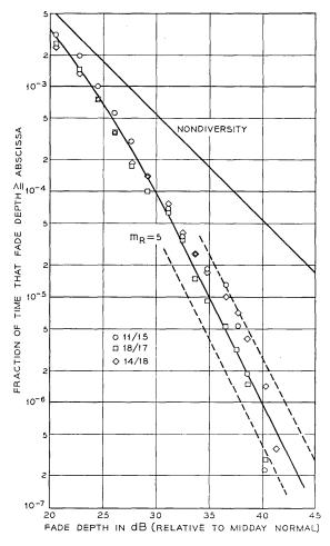
Fig. 13-6-GHz frequency diversity; 120-MHz separation.
