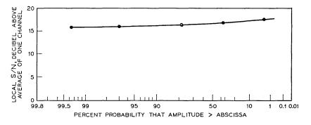
Fig. 7—CPD of a 4:32 array system. Complex conjugate retransmission maximal ratio diversity reception.
