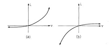
Fig. 4—General shape of the functions  $f_1$  and  $f_2$ ; (a) pnp transistor, (b) npn transistor.
