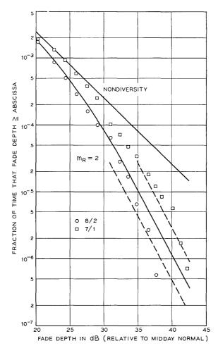
Fig. 17-4-GHz frequency diversity; 20-MHz separation.
