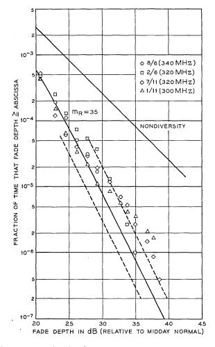
Fig. 23-4-GHz frequency diversity; 300/320/340-MHz separation.
