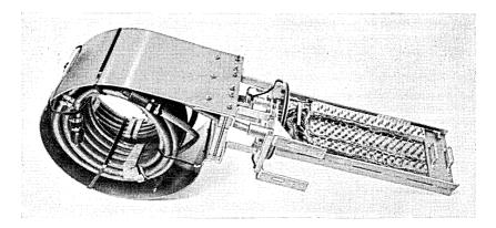
Fig. 21 — Cover plate and internal chassis for 472A1 apparatus case.
