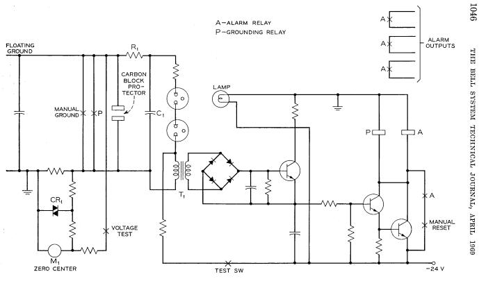
Fig. 2-Ground circuit simplified schematic.
