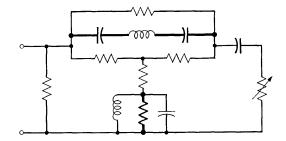
Fig. 32 — High frequency B equalizer Bode network.
