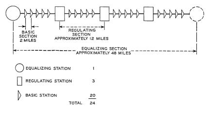
Fig. 12 — Equalizing section schematic.
