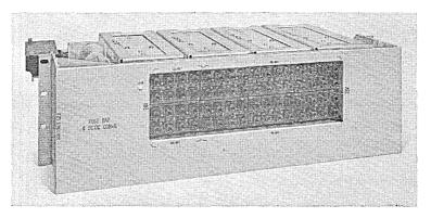
Fig. 41 — Fuse panel and converter assembly.
