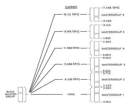
Fig. 1-Six-mastergroup line frequency spectrum.
