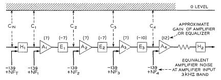
Fig. 9—Block Diagram of the A equalizer for noise figure calculations. Indicated are the equivalent noise sources and the approximate amplifier and network gains.
