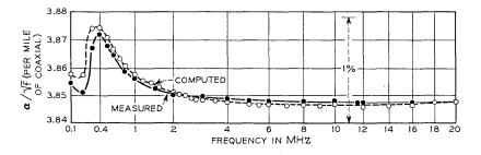
Fig. 3 — Attenuation divided by the square root of the frequency (per mile of coaxial). Derived from measurements on the installed Coax 20 at Chester, New Jersey  $(55^{\circ}F)$ .
