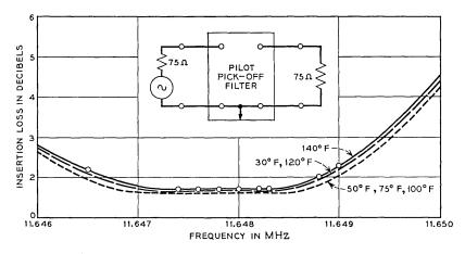
Fig. 33 — Inband temperature performance of pilot pick-off filter.
