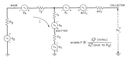
Fig. 10 — Equivalent circuit for noise figure calculation of a common emitter stage with series local feedback  $(R_E)$ .
