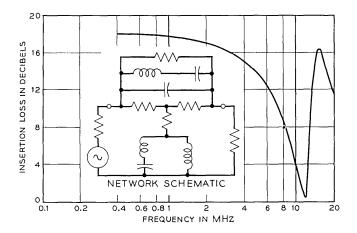
Fig. 31—Insertion loss characteristic and schematic diagram of  $11.648~\mathrm{MHz}$  notch filter.
