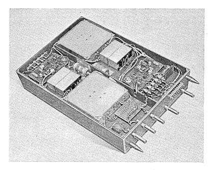
Fig. 25 — A equalizer assembly,
