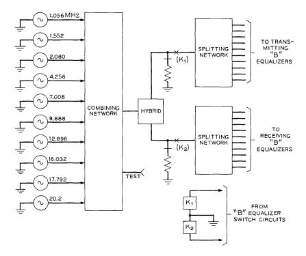
Fig. 35 - B test oscillator and oscillator connecting circuit.
