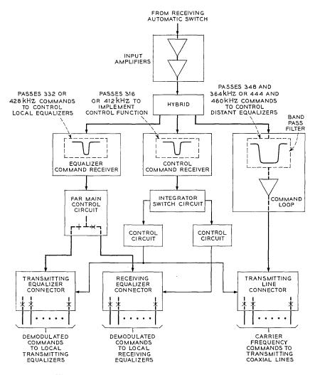
Fig. 5 - Loop-back circuit for unattended main station.
