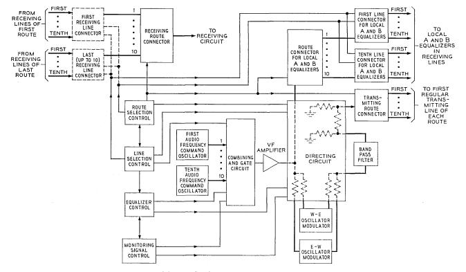
Fig. 3-Sending circuit block diagram.
