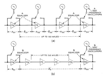
Fig. 7 — (a) A equalization; (b) B equalization.
