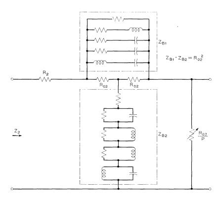
Fig. 29 - Schematic diagram of postregulator network.
