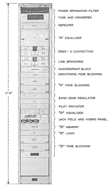
Fig. 45-Receiving bay equipment arrangement.
