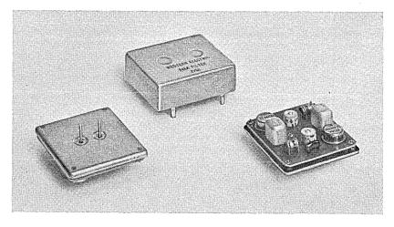
Fig. 34 — Mechanical construction of pilot pick-off filter.
