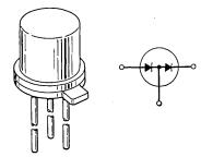
Fig. 6 — The device outline for the 459A diode. All dimensions are in inches.
