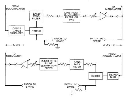
Fig. 20 - Mastergroup connector, MMX-1 to MMX-2 (two-way).
