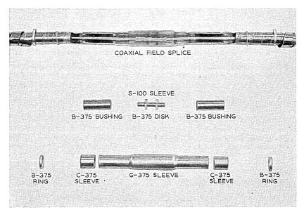
Fig. 9-Coaxial field splice.
