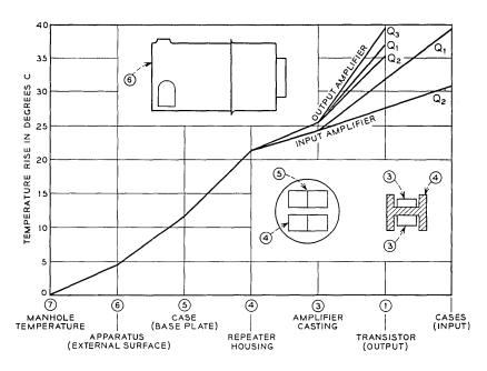
Fig. 5 - Temperature gradients for basic repeater installed in a manhole.
