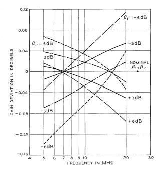
Fig. 10 — Calculated preamplifier gain deviations vs  $\beta$  of Q1 and Q2 transistors.
