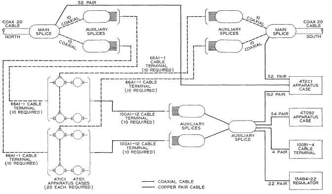
Fig. 15 — L-4 equalizing station schematic.
