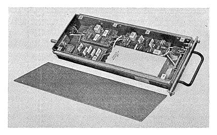
Fig. 27 — Command receiver assembly.
