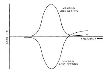
Fig. 17—Distorted network response before compensation. The distortion results chiefly from circuit parasities and has the effect of lowering the realized G relative to the design G.
