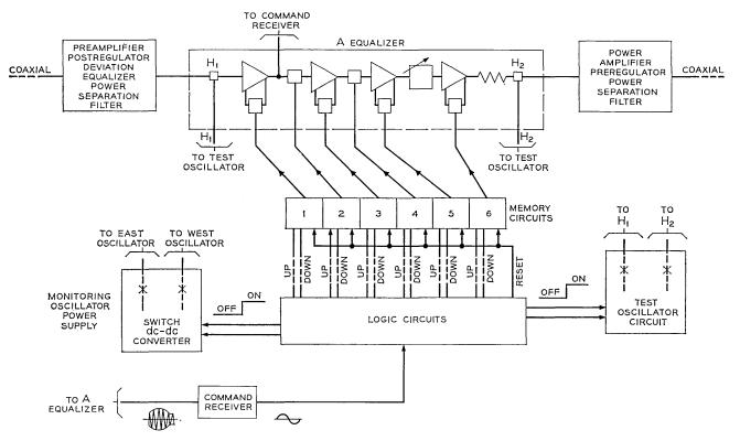
Fig. 1 - Functional block diagram of the equalizing repeater.
