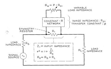
Fig. 23 — Series-type Bode regulator network.
