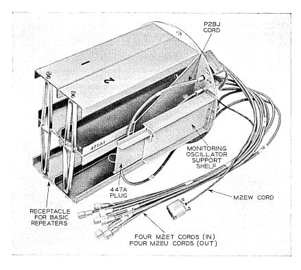
Fig. 19 --- Chassis for basic repeaters.
