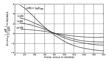
Fig. 8 — Calculated  $\mu\beta$  effect vs  $\mu\beta$  phase angle for various values of  $|\mu\beta|$ .
