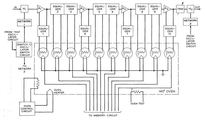
Fig. 30 — Block schematic of the B equalizer. For clarity only one oven and control circuit is shown. The B equalizer circuits are actually distributed among four plug-in modules and the rack-mounted shelf. Each module has its own oven and control circuit for the thermistors required by the equalizing networks in the module.
