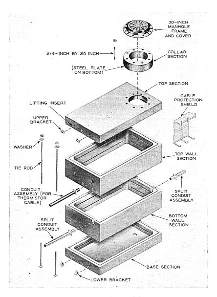
Fig. 16 — G manhole: exploded view.
