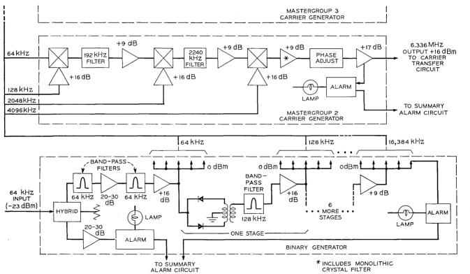
Fig. 6 — Carrier supply circuits.
