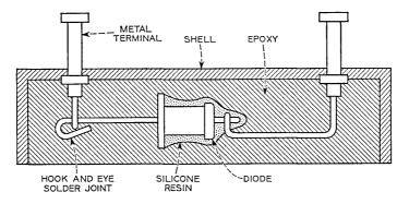
Fig. 5 — Schematic of assembly cross section.
