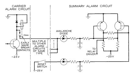
Fig. 9 — Typical alarm circuit.
