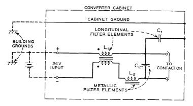
Fig. 5 — Input filter circuit.
