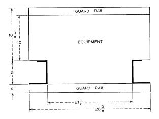
Fig. 38 - Plan view of a line bay.
