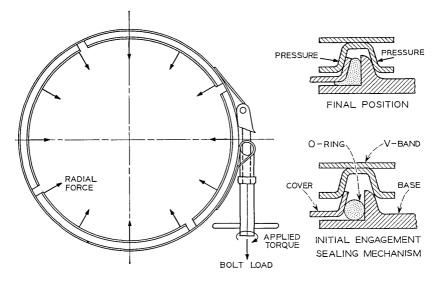
Fig. 18 - The O-ring-V-band sealing mechanism.
