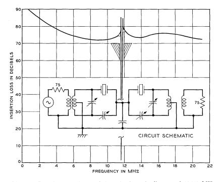
Fig. 32- Insertion loss characteristic and schematic diagram of  $11.648~\mathrm{MHz}$  crystal pilot pick-off filter.
