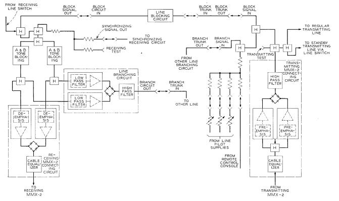
Fig. 16 — Line connecting circuits.
