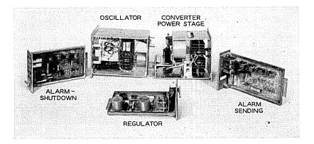
Fig. 8 - Converter plug-in packages,
