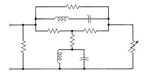
Fig. 15 — Ideal A equalizer Bode section.
