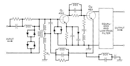
Fig. 6 — Schematic diagram of preamplifier (less bias circuitry).
