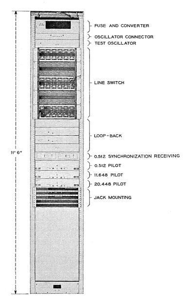
Fig. 48 — Control connecting bay equipment arrangement.
