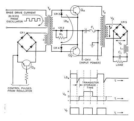
Fig. 3 — Power converter simplified schematic.
