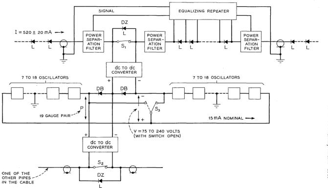
Fig. 6 - Monitoring oscillator power arrangements.
