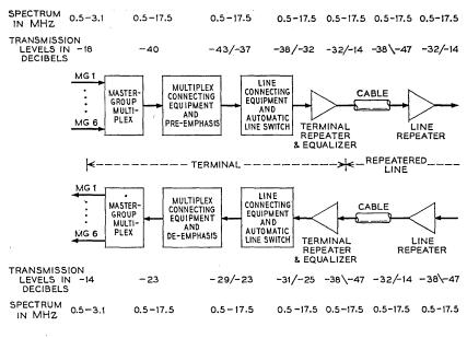
Fig. 6—L-4 transmission levels.
