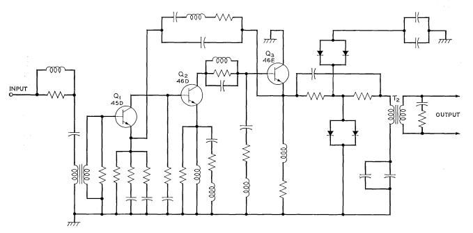
Fig. 11 — Schematic diagram of power amplifier (less bias circuitry).
