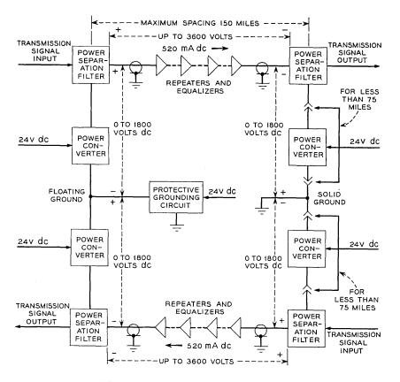
Fig. 1 — Power feed system block diagram.
