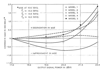
Fig. 13 — Change in third order modulation coefficient vs output signal power for power amplifier.
