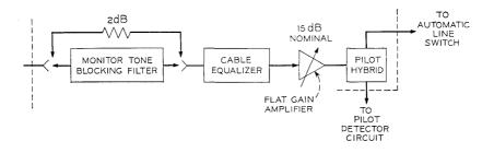
Fig. 37 — Block diagram of the monitoring tone blocking circuit. One of the pilot hybrid outputs is connected to the receiving line switch while the other goes to the switch initiating circuits.
