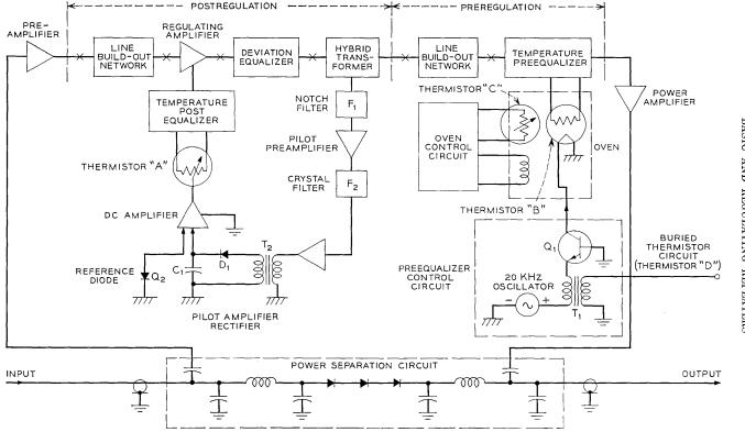
Fig. 19 — Complete block diagram of regulating repeater.
