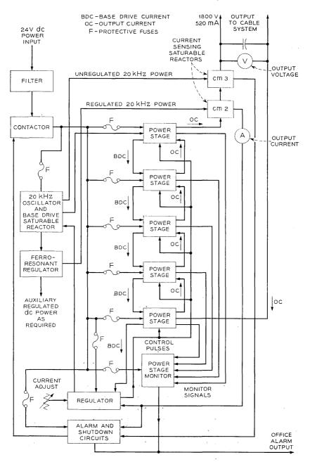
Fig. 4 - Power converter block diagram.
