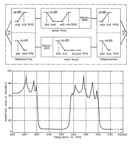
Fig. 18 — Command and line switching tone blocking filter.
