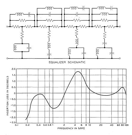
Fig. 26 — Deviation equalizer schematic diagram and requirements for a five-repeater regulating section.
