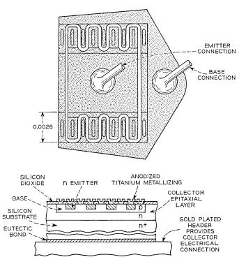
Fig. 1—The 45D transistor.
