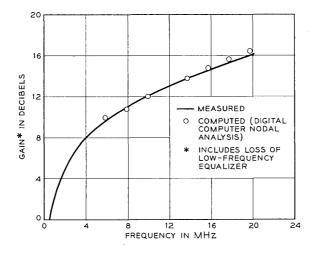
Fig. 9 - Measured and computed insertion gain of preamplifier.
