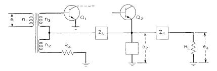
Fig. 7—Simplified schematic diagram of the equalizer amplifier.  $Z_3$  and  $Z_4$  would normally be realized by the adjustable impedance of equalizer networks.
