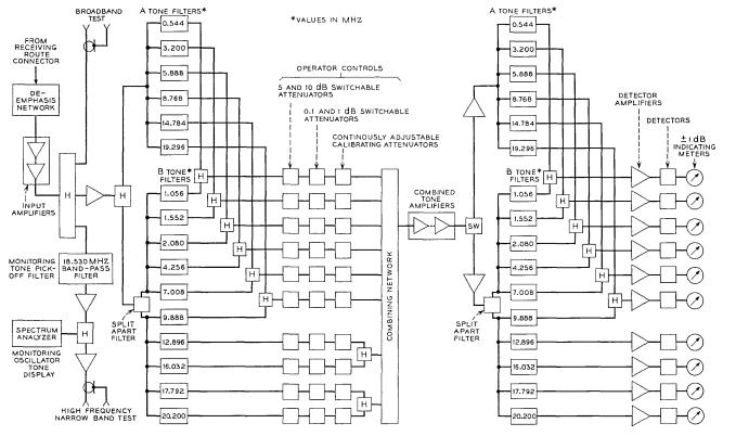
Fig. 4 - Receiving circuit block diagram.
