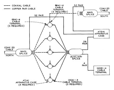
Fig. 13 — L-4 basic station schematic.
