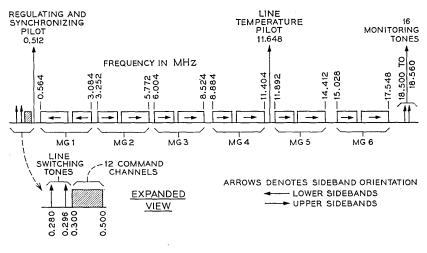
Fig. 1-L-4 frequency allocations.
