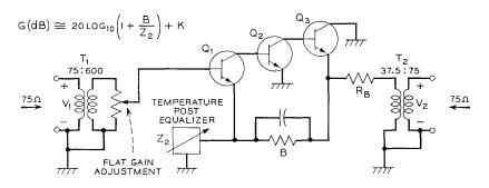
Fig. 27 — Simplified schematic diagram of regulating amplifier.
