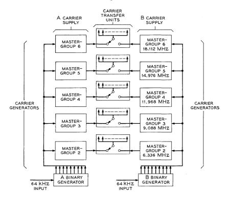
Fig. 7—Carrier supply arrangement.
