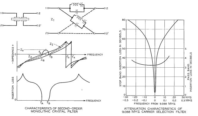
Fig. 15 - Monolithic crystal filter.
