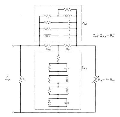
Fig. 24 - Preregulator network configuration.
