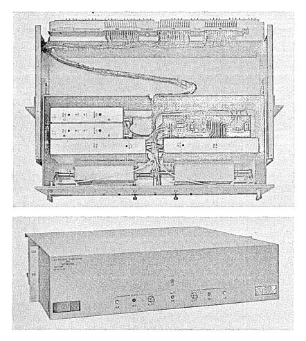
Fig.  $49-512~\mathrm{kHz}$  pilot stabilization and distribution unit. Top view (top) and front view.
