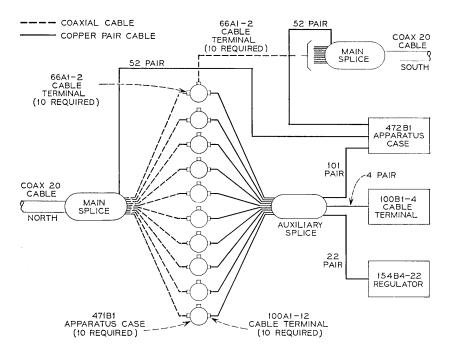
Fig. 14 — L-4 regulating station schematic.
