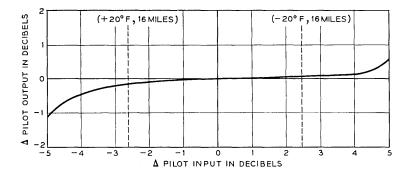
Fig. 37 — Regulating performance of pilot-controlled postregulator.
