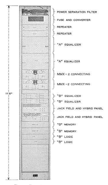
Fig. 39-Transmitting bay equipment arrangement.
