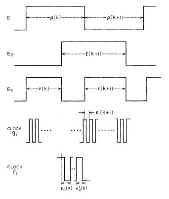
Fig. 9 — Waveforms for locked first order PLL showing how time jitter is caused by phase differences in clock signals.
