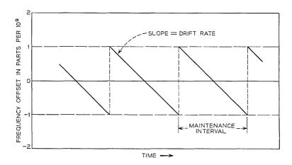
Fig. 13 — Maintenance of oscillator frequency accuracy by periodic corrections.
