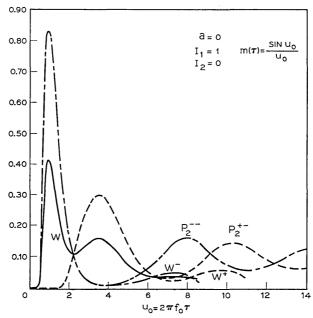
Fig. 5 (also Figs. 8, 11, 14, 17, and 20) — Plots of the probability functions  $P_2$ — $(u_0, I_1, I_2, a)$ ,  $W^-(u_0, I_1, I_2, a)$ ,  $W^-(u_0, I_1, I_2, a)$ ,  $W^+(u_0, I_1, I_2, a)$ , and  $W(u_0, I_1, I_3, a)$  associated with the crossings of the levels  $I_1$  and  $I_2$  by a stationary random process consisting of a sinusoidal signal of frequency  $f_0/2$  plus stationary gaussian noise with autocorrelation function  $m(\tau)$ . a denotes the signal-to-noise power ratio.
