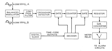
Fig. 10 — Difference frequency detector.
