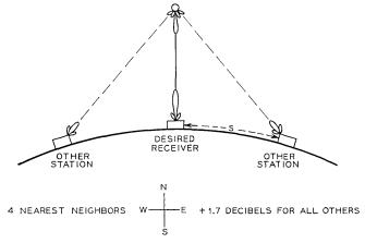
Fig. 7 — Interference at a satellite.
