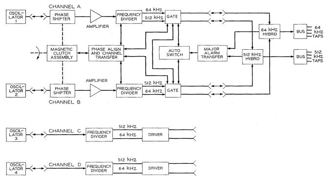
Fig. 1—Block diagram of principal circuits in reference frequency standard.
