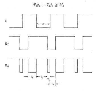
Fig. 12 — Waveforms for parasitic locked mode of second order PLL.
