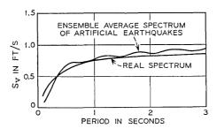
Fig. 10 — Comparison of velocity spectra of earthquakes,  $\lambda = 0.02$ .
