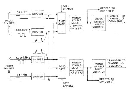
Fig. 6 — Phase align and channel transfer, phase coincidence circuit.
