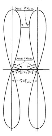
Fig. 16 — Geometry of adjacent 8's.  $\xi = \xi_{\min}$  for  $u_{\min} = v_{\min}$ ,  $v_{\min} = \text{closest}$  approach among N optimally packed satellites on each 8.
