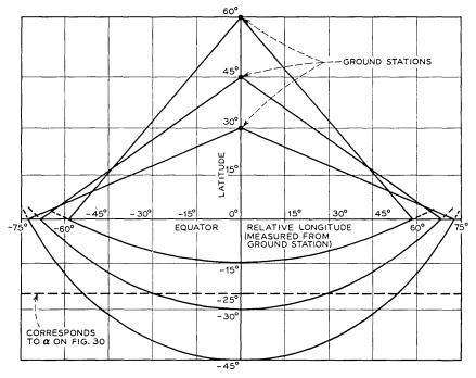
Fig. 31 — Region of visibility of a satellite from ground stations at representative north latitudes, assuming minimum elevation of 6.4° above the horizon. Same scale as Fig. 30, so that these curves give directly permitted 8's and equatorial satellites for representative paths on Fig. 30.
