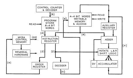
Fig. 2 — Prototype self-healing processor.
