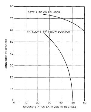
Fig. 32 — Maximum relative longitude from ground station for which satellite is visible 6.4° above the horizon.
