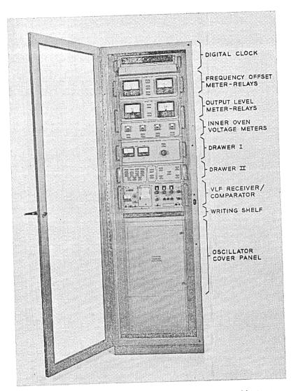
Fig. 14 — Front view of reference frequency standard cabinet.
