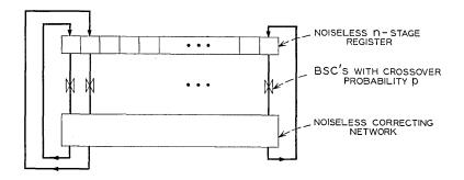
Fig. 3 — Noisy register with noiseless correcting network.
