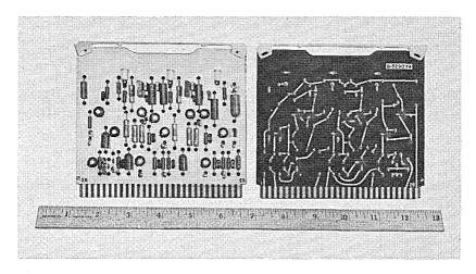
Fig. 18 — High speed plug-in card: (a) component side, (b) printed wiring side.
