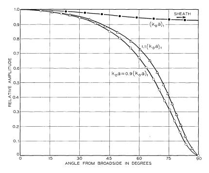
Fig. 5 —  $G(\theta)$  (normalized to unity at  $\theta = 0^{\circ}$ ) for values of  $k_{0}\alpha$  near  $(k_{0}a)_{1}$ ,  $G_{0}(k_{0}\sin\theta) \equiv 1$ ,  $\epsilon_{r} = 6.0$ .
