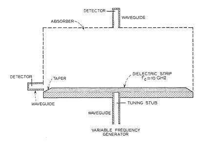
Fig. 6 — Apparatus for measuring broadside and end-fire radiation.
