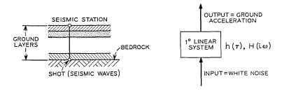
Fig. 6 — Ground layers represented by a linear system.
