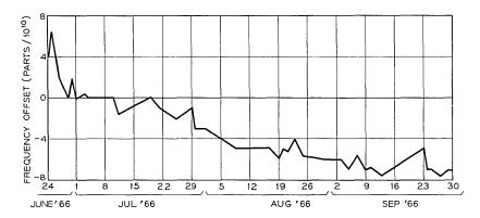
Fig. 3 — Typical precision oscillator drift characteristics.
