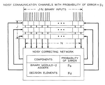
Fig. 7—Physical configuration of a memory based on a low-density parity-check decoder.
