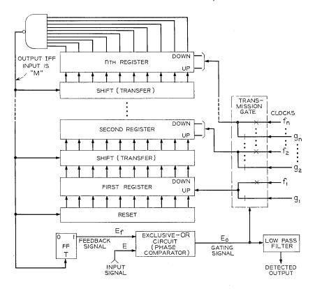
Fig. 1 — Block diagram of general digital PLL.
