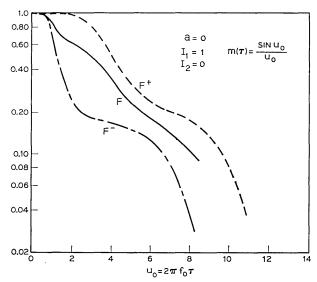
Fig. 7 (also Figs. 10, 13, 16, 19, and 22) — Plots of the probability functions  $F^+(u_0, I_1, I_2, a)$ ,  $F^-(u_0, I_1, I_2, a)$ , and  $F(u_0, I_1, I_2, a)$  associated with the crossings of the levels  $I_1$  and  $I_2$  by a stationary random process consisting of a sinusoidal signal of frequency  $f_0/2$  plus stationary gaussian noise with autocorrelation function  $m(\tau)$ , a denotes the signal-to-noise power ratio.
