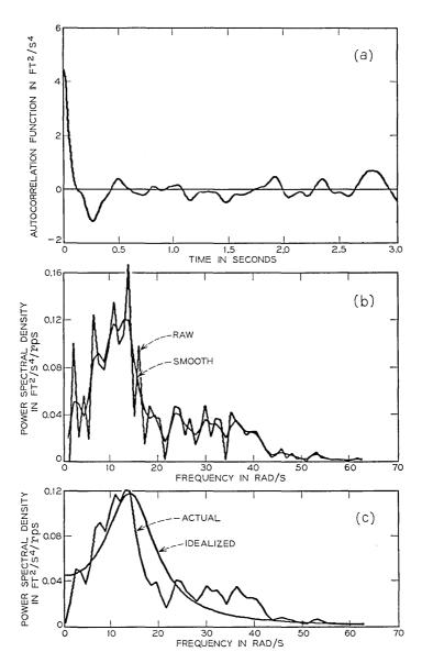
Fig. 4-N-S component of earthquake at El Centro, Calif., May 18, 1940. (a) Autocorrelation function. (b) Power spectral density function. (c) Comparison of actual and idealized power spectral density functions.
