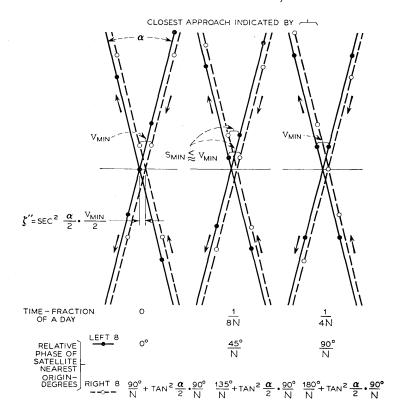
Fig. 24 — Central portion of two close-spaced interleaved 8's. Uniform phase spacing over 360° on each 8. N is odd, N large,  $\alpha=28^{\circ}$ . Tan²  $\alpha/2$  neglected in plotting satellites on right 8.
