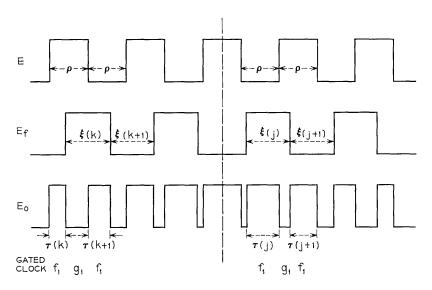
Fig. 6 - Input, feedback, and output waveforms of nonlocked first order PLL.
