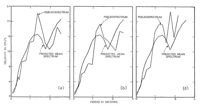
Fig. 14 — Comparisons of velocity response spectra,  $\lambda = 0.02$ .
