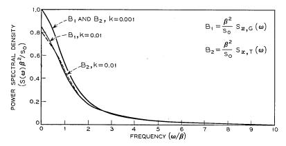
Fig. 3 — Power spectral density by equivalent linearization.
