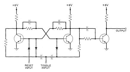
Fig. 5 - Binary flip-flop circuit.
