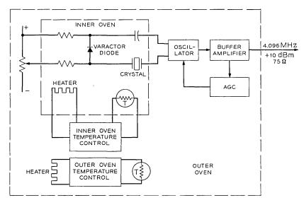
Fig. 2 — Precision oscillator block diagram.
