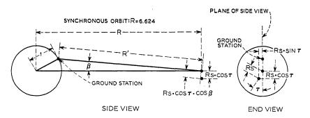
Fig. 35—Satellite separation as a function of ground station location. s = angular separation between satellites at center of earth. Distance between satellites (Rs) and its projections are true (not angular) lengths.
