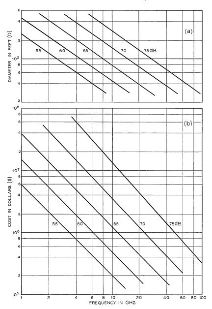
Fig. 8—(a) Diameter and (b) cost of minimum cost radome enclosed antennas for fixed gain and frequency vs frequency (Example 2).
