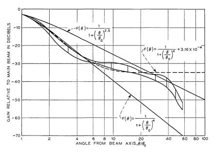
Fig. 4—Side lobe levels of microwave pole line periscope antenna. Beamwidth =  $2.5^{\circ}$ ,  $\theta_0 = 1.25^{\circ}$ . Vertical lines show range of envelope of side lobe levels for both polarizations.
