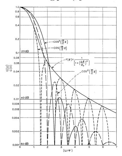
Fig. 5 — Calculated antenna pattern for  $\cos^n[(\pi/2)x]$  illumination of square aperture. a is aperture opening.  $\theta$  is angle with normal to aperture.  $u \equiv (\pi/\lambda)$   $a \sin \theta$ .
