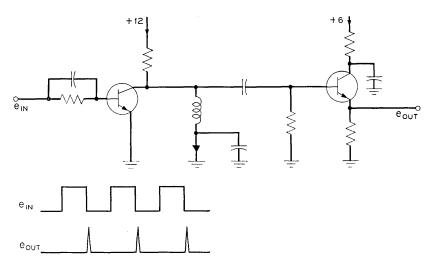
Fig. 7 - Shaper circuit.
