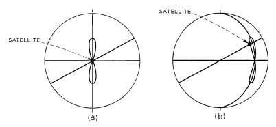
Fig. 5 — Figure 8 pattern. (a)  $c = 0^{\circ}$  as in Fig. 3; (b)  $c = 45^{\circ}$  as in Fig. 4.
