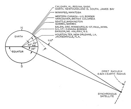
Fig. 1—Synchronous satellite on an inclined orbit; southernmost declination = inclination = 25°.
