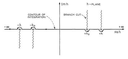
Fig. 3 — Definition of proper Riemann surface for evaluation of  $\beta_0 = (k_0^2 - h^2)^{1/2}$  and  $\beta = (k^2 - h^2)^{1/2}$ .
