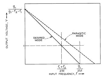
Fig. 13 — Comparison of parasitic and normal mode voltage versus frequency characteristic for second order PLL.
