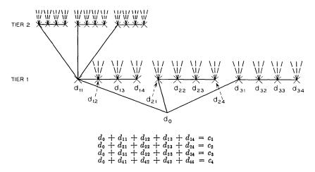
Fig. 6 — Two representations for the parity-check constraints involving  $d_0$ . At the top is one of the J parity-check set trees rising from  $d_0$ . Beneath it are the parity-check equations containing  $d_0$ .
