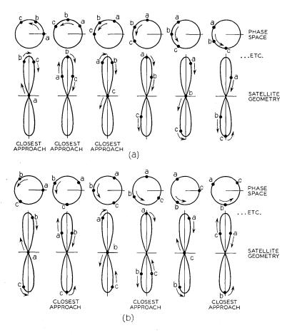
Fig. 15 — Satellite motion for N=3, optimum packing. Phase increment = 30°. Uniform phase spacing over (a) 180° and (b) 360°.
