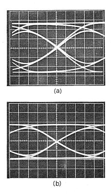
Fig. 14- First order PLL eye patterns for 300 baud random digital data. Lock range of (a) 400 Hz, (b) 600 Hz. Horizontal scale: 0.5 ms per cm.
