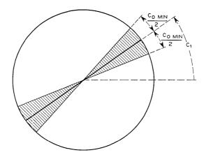
Fig. 12—Phase of a satellite with associated sector.  $c_{0 \text{ min}}$  given by equation 15.
