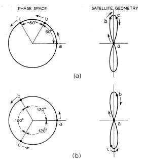
Fig. 14 — Optimum packing for N=3. Uniform phase spacing over (a) 180° and (b) 360°.
