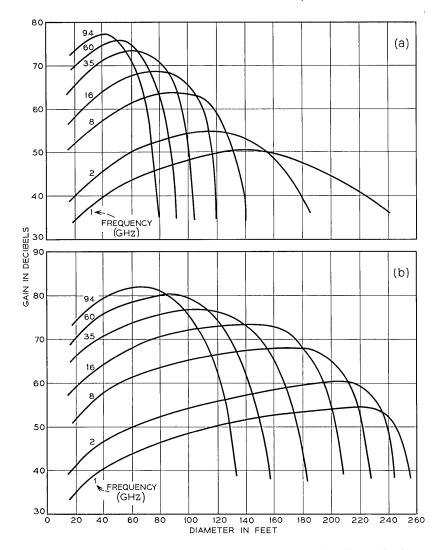
Fig. 9 — Gain vs diameter at several different frequencies with a fixed cost of (a) \$1,000,000, and (b) \$10,000,000 (Example 3).
