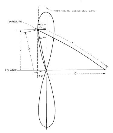
Fig. 6 — Enlarged 8 with relative geometric parameters.  $c = 45^{\circ}$ .
