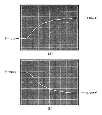
Fig. 5 — Output voltage response of first order PLL to input step frequency of (a) 1070 to 1270 Hz and (b) 1270 to 1070 Hz. Horizontal scale: 0.5 ms per cm.
