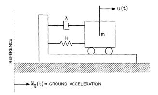
Fig. 3 - Linear mechanical system subjected to ground excitation.
