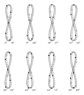
Fig. 25 — Satellite motion for two close-spaced, interleaved 8's. Phases indicated on respective 8's.  $N=5, \alpha=30^{\circ}$ , phase increment = 9°, relative phase between two 8's = 19.03°.
