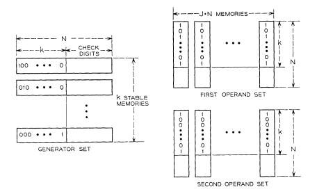
Fig. 2 — The generator set and typical operand sets. The digits are typical of the digits in each of the J noisy registers within the stable memory.
