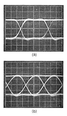
Fig. 16 — Second order PLL eye patterns for (a) 150 baud and (b) 300 baud random digital data. Horizontal scale: 1 ms per cm.
