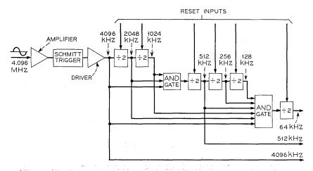
Fig. 4 — Frequency divider circuit.
