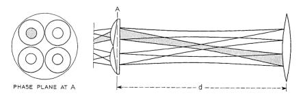
Fig. 7—A distribution of the phase spots that minimizes distortion.
