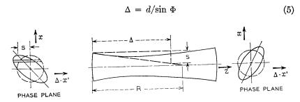
Fig. 3 — The phase spot for a beam entering with a curved phase front.
