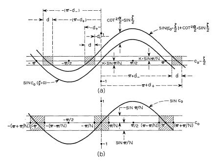
Fig. 18—Forbidden region for relative phase between satellites on different 8's (equation 37). N=9. (a) General case.  $\cot^2\alpha/2\cdot\sin\zeta/2=0.5$  (separation about half that for two 8's just touching), K=0.6. Enlarged portion of upper curve, containing forbidden region to left of origin, shown in Fig. 19. (b) Limiting case (single 8).  $\zeta=0$ , K=1. This curve is the same as the lower curve of (a).
