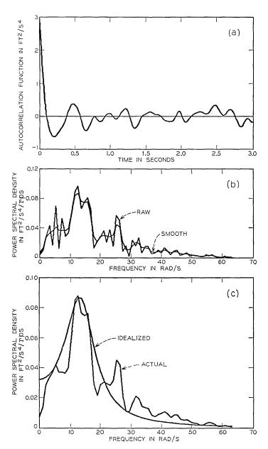
Fig. 5—E-W component of earthquake, El Centro, Calif., May 18, 1940. (a) Autocorrelation function. (b) Power spectral density function. (c) Comparison of actual and idealized power spectral density functions.
