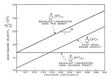
Fig. 2 — Comparison of mean square velocity nonlinear system subjected to random noise.
