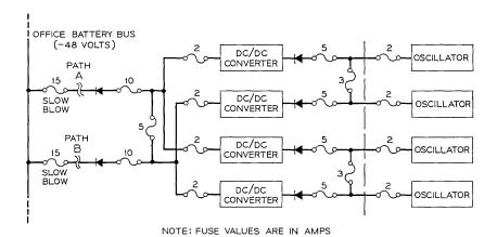
Fig. 8 — Oscillator power supply circuit.
