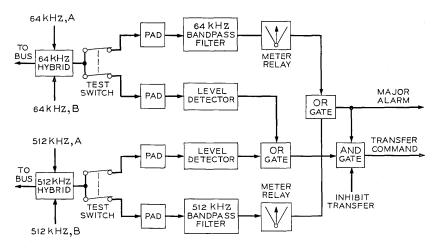
Fig. 9 - Major alarm transfer circuit.
