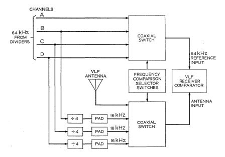
Fig. 11 — VLF receiver-comparator mode-select circuits.
