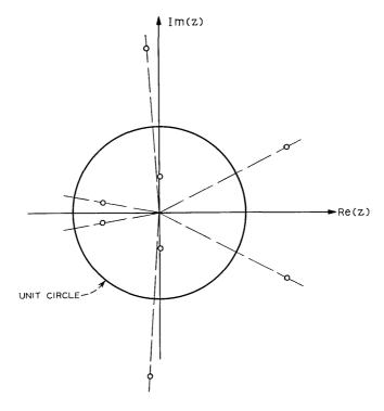
Fig. 7 — Root locations of pulse page 563 of Ref. 5.  $B(z) = 15z^8 - 20z^7 + 40z^6 - 60z^5 + 0z^4 + 115z^3 + 60z^2 + 20z + 10$   $\theta_1, \; \theta_1^* = 0.404 \; \angle \; \pm 89.8 \; ^{\circ} \theta_2, \; \theta_2^* = 0.652 \; \angle \; \pm 169.9 \; ^{\circ} \phi_1, \; \phi_1^* = 1.642 \; \angle \; \pm 27.7 \; ^{\circ} \phi_2, \; \phi_2^* = 1.894 \; \angle \; \pm 94.4 \; ^{\circ}.$
