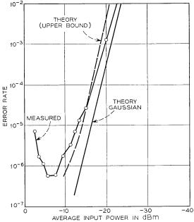
Fig. 3—Comparison of experimental and theoretical error rates for one link of noncompandored transmission. Theory neglects overload distortion. Instantaneous input power of +6 dBm is the onset of overload.
