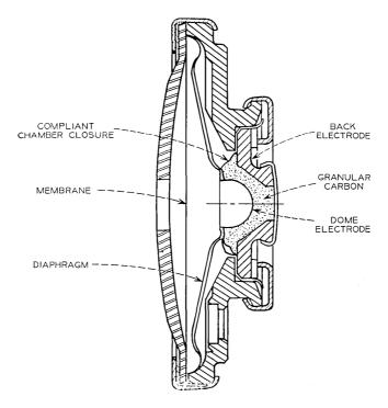
Fig. 1 — Cross section of T1 transmitter.
