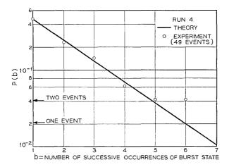
Fig. 4 — Burst statistics for T1 digital transmission line.
