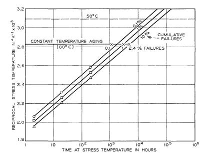
Fig. 7 — Loci of constant percentile cumulative failure in time and temperature for unprotected wires aged in air.
