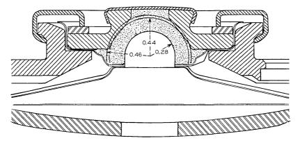
Fig. 5 — Approximation of carbon chamber by hemispherical cavity. Indicated radii are in cm.
