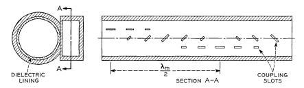
Fig. 3 —  $TE^{\circ}_{10}$ - $TE^{\circ}_{01}$  coupler using unequal phase constants in the rectangular and round waveguides.
