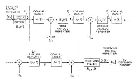
Fig. 1 — A hybrid coaxial cable digital transmission system.
