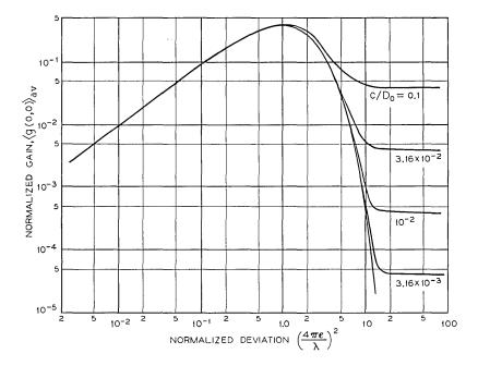
Fig. 2 - Normalized antenna gain.
