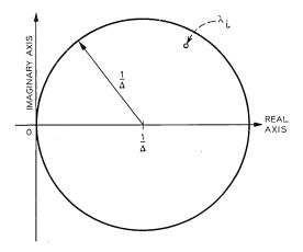
Fig. 8 — Necessary relation of  $\Delta$  to location of eigenvalue in complex plane.
