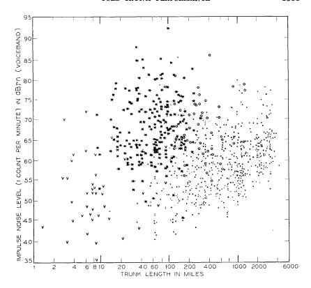
Fig. 6—Scatter diagram of impulse noise level versus trunk length. v = voice-frequency trunks; \* = trunks containing only compandored carrier; o = trunks containing both compandored and noncompandored carrier; · = trunks containing only noncompandored carrier.
