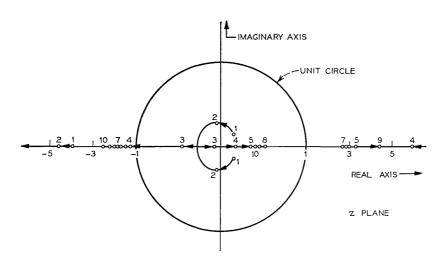
Fig. 4 — Root loci for pulse of Fig. 3. Scale inside circle is magnified four times.
