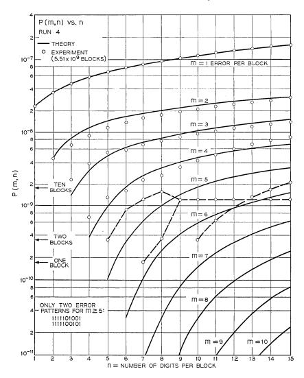
Fig. 5—Block error statistics (digits per block) for T1 digital transmission line.
