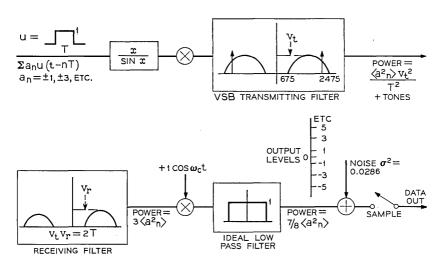
Fig. 2—Model of back-to-back transmission of VSB modem. The noise added at baseband represents imperfections of the modem.
