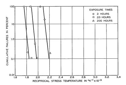
Fig. 8 — Failure distribution in temperature for protected wires.
