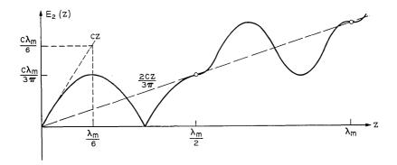
Fig. 5 — Undriven-wave amplitude versus distance for "third harmonic" in square-wave coupling.
