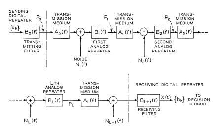
Fig. 1—A general hybrid digital transmission system.
