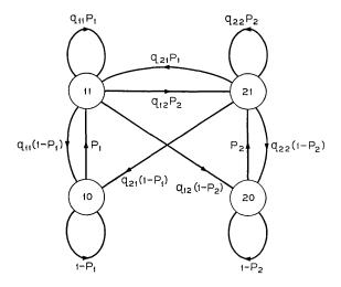
Fig. 2 — State diagram of binary regenerative channel.
