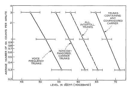
Fig. 7 — Average impulse noise levels at receive switch with 90 percent confidence intervals.
