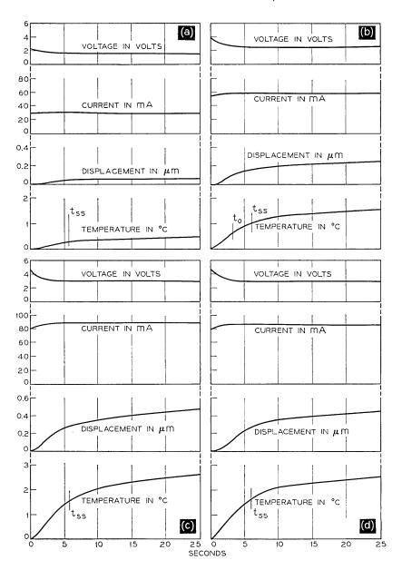
Figure 10. — Transient response of an excited T1 telephone transmitter. (a) Run 1,  $\langle IV \rangle_{av\ transient} = 0.056W$ ; (b) run 2,  $\langle IV \rangle_{av\ transient} = 0.156W$ ; (c) run 3,  $\langle IV \rangle_{av\ transient} = 0.264W$ ; (d) run 4,  $\langle IV \rangle_{av\ transient} = 0.264W$ .
