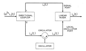
Fig. 1 — Injection-locked-oscillator FM receiver.
