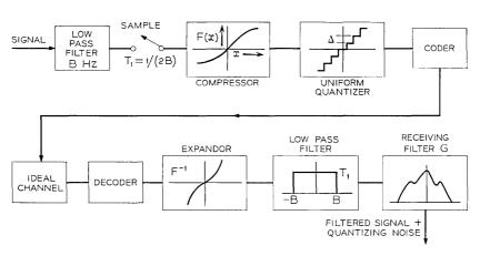
Fig. 1 — Essential elements of quantized transmission scheme.
