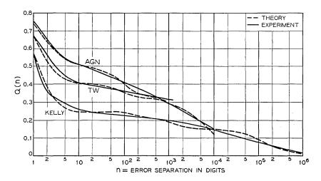
Fig. 7 — Error separation statistics for switched telephone network.
