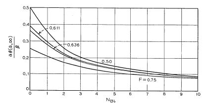
Fig. 6 — Dome electrode maximum temperature rise vs  $N_{B^{\pm}}.$  (F=0.636 for standard T1 transmitter.)
