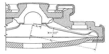
Fig. 3 — Coordinate system for heat flow along the conical diaphragm.
