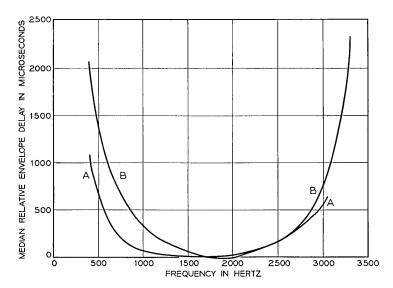
Fig. 12 — Median relative envelope delay for (a) short (0 to 62.5 miles) and (b) long (2000 to 4000 miles) intertoil trunks.
