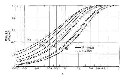
Fig. 8 — Transient temperature rise of the dome electrode for various  $N_{Bi}$  and two values of F.
