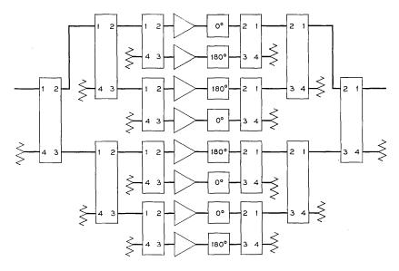
Fig. 3 — Eight way quadrature divider with amplifiers.
