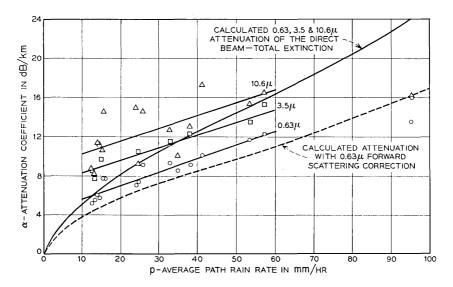
Fig. 19 — Measured attenuation coefficients of a rain storm for a 2.6 km path.
