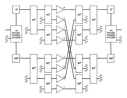
Fig. 5—Hybrid array of in-phase and quadrature couplers: doubled for way divider to form eight element amplifier.
