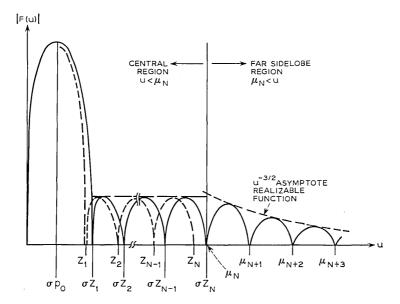
Fig. 5 — Construction of asymptotic difference pattern.
