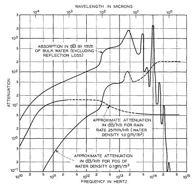
Fig. 26 — Attenuation due to liquid water in various forms as function of frequency.
