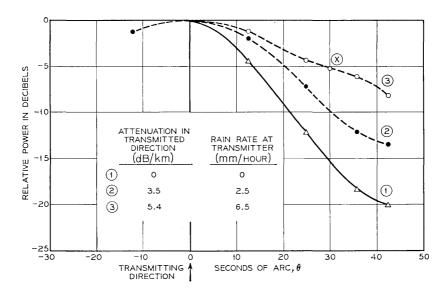
Fig. 23 — Beam broadening caused by rain.
