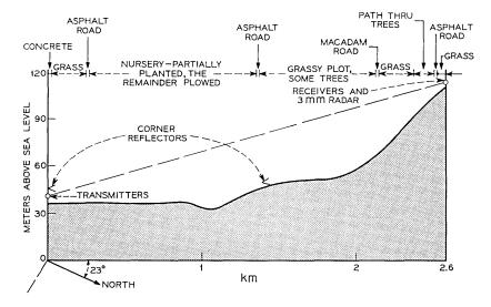
Fig. 12 — Profile of transmission path.
