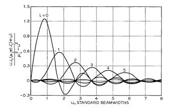
Fig. 2 — Bessel series pattern function terms.
