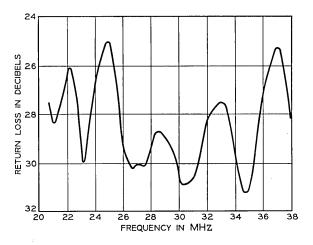
Fig. 52 — Output return loss of 30 Mc amplifier.
