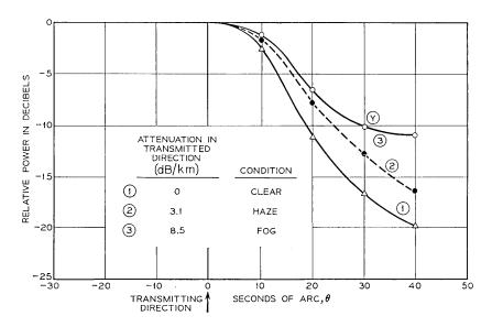
Fig. 25 — Beam broadening caused by fog.
