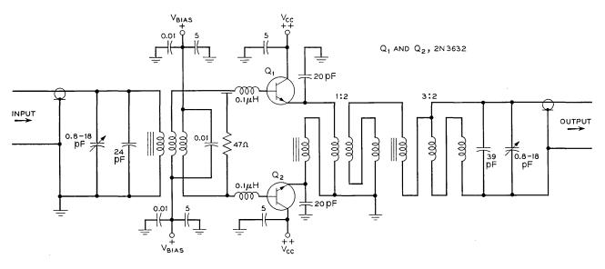
Fig. 40 — Class B push-pull amplifier for 30 Mc system (20-40 Mc, class A-B, push-pull, 7.5 watts linear).
