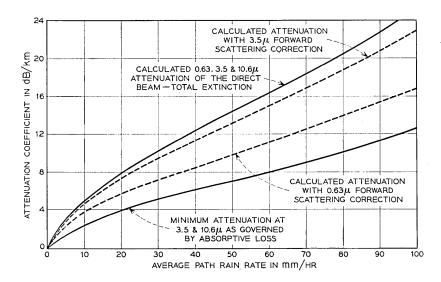
Fig. 8 — Rain attenuation coefficient for a 2.6 km path.
