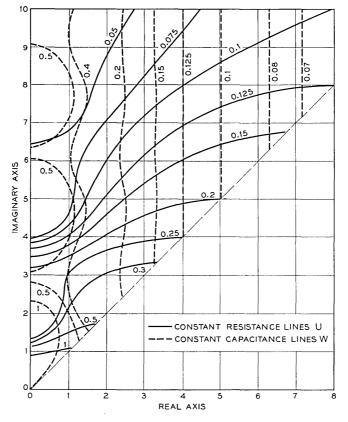
Fig. 5 — The values of U and W for complex poles at  $\vartheta = x + jy$  when  $z_s = \infty$ .
