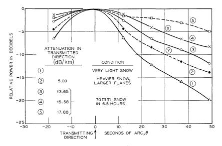
Fig. 24 — Beam broadening caused by snow.
