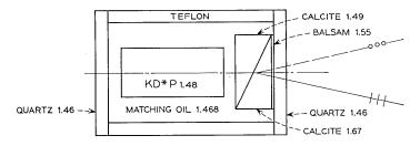
Fig. 2—Optical switch with numbers giving the refractive indices for light polarized in the plane of the figure.
