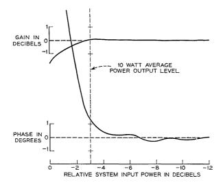
Fig. 23 — System gain and phase at 75Mc as a function of input power.
