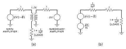
Fig. 21 — Thevenin equivalents of subsidiary amplifier feed into main amplifier output circuit.
