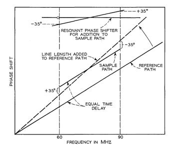
Fig. 36 — Phase equalization of reference loop.
