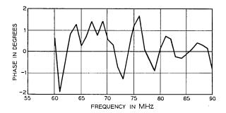
Fig. 26 — Phase deviation from linear phase vs. frequency behavior (Constant time delay). Average time delay  $= 2.5 \mu \text{sec}$ .
