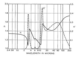
Fig. 2 — Complex refractive index (n - in') of ice.
