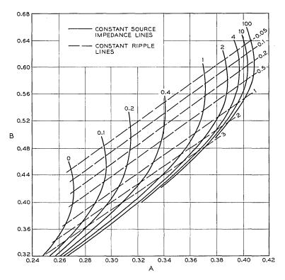
Fig. 10 — The distributed load low-pass filter design chart.
