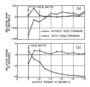
Fig. 51 — Gain (a) and Phase (b) Variation at 35 Mc.
