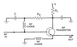
Fig. 44 — Conventional transistor biasing arrangement with DC stabilization.
