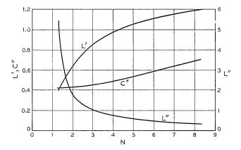
Fig. 19 — Component values for equivalent transformer.
