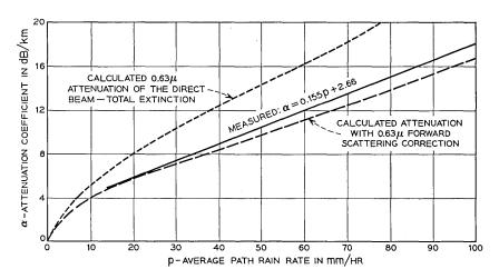
Fig. 17 — Measured rain attenuation coefficients of  $0.63\mu$  for a 2.6 km path; standard deviation is  $\pm 2.8$  dB per km at a rain rate of 50 mm/hr.
