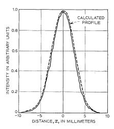
Fig. 7—Intensity scan across the guide cross-section for light after one round trip in the 3-section line.
