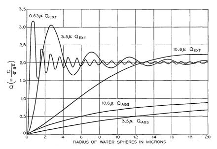
Fig. 3 — Approximate extinction and absorption cross sections.
