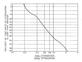
Fig. 14 — A distribution for the ratio of attenuation by light fog at  $3.5\mu$  and  $0.63\mu$ .
