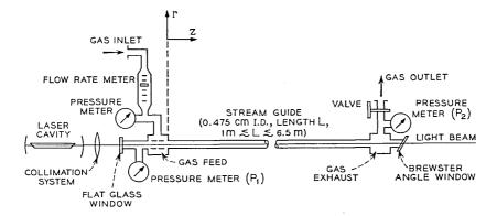
Fig. 1—Experimental setup for measurements with the stream guide.
