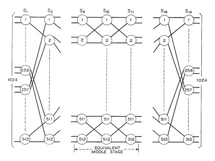
Fig. 5 — Beneš type 1024 terminal network of  $\beta$  elements.
