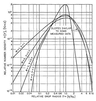
Fig. 5 — Drop size distribution of fog models.  $n(r) = Ar^a \exp[(-\alpha/\gamma)r^{\gamma}] A = (N/a_m) (\alpha/\gamma)^{(a+1)/\gamma} \gamma/\Gamma[\alpha+1)/\gamma]$ , and  $a_m = \text{radius of drops with maximum number density.}$
