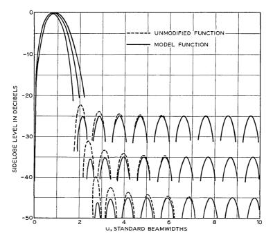
Fig. 3—Model difference pattern compared with unmodified function for sidelobe levels of 25, 35, and 45 dB.
