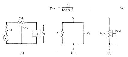
Fig. 2 — The basic low-pass filter circuit.
