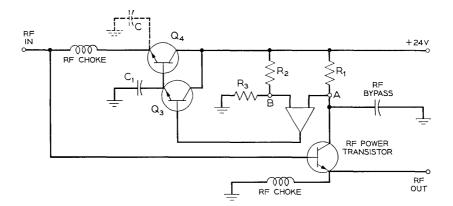
Fig. 42 — Active clamp schematic.
