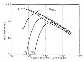
Fig. 12 — Difference pattern relative directivity,  $\eta$ .
