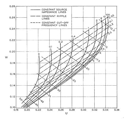
Fig. 7 — The lumped load low-pass filter design chart.
