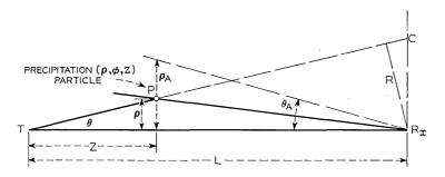
Fig. 9 — Geometry for forward scattering.
