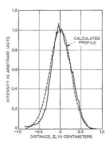
Fig. 9 — Intensity scan across the guide cross-section for light after 150 round trips in the 3-section guide.
