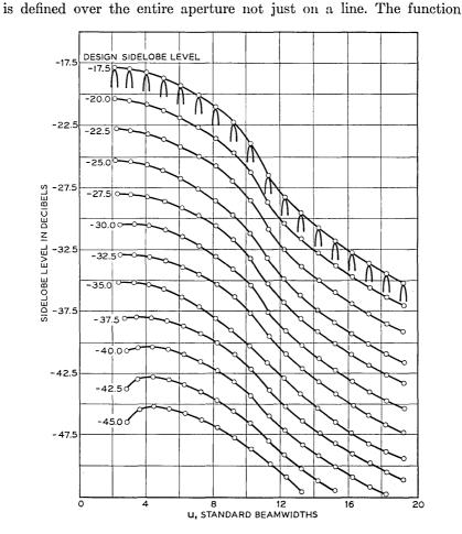
Fig. 8 — Sidelobe envelope of pattern functions for N = 10.
