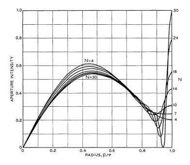
Fig. 7 — Circular aperture functions for -30 dB sidelobe level.
