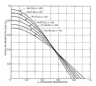
Fig. 14 — Normalized angular sensitivity function,  $K(u)/K_0$ .
