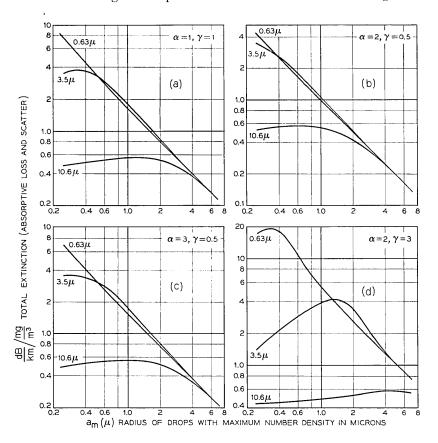
Fig. 6 — Extinction of coefficients for various fog models.
