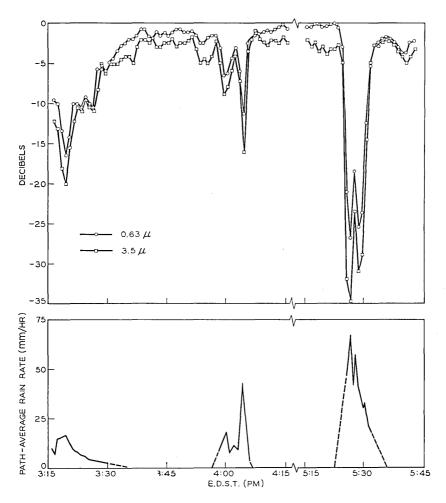
Fig. 16 — Measurement of  $2.6~\rm km$  transmission loss in rain showers on September  $24,\,1965.\,0$  dB-signal level in clear weather.
