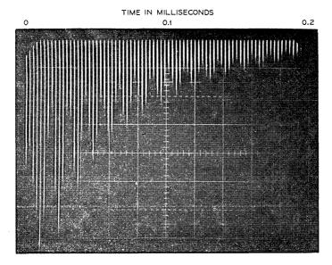
Fig. 10 — Pulse train from the 3-section line after one lens was misaligned.
