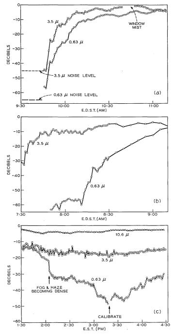
Fig. 13 - Measurement of  $2.6~{\rm km}$  transmission loss in light fog.  $0~{\rm dB\text{-}signal}$  level in clear weather.
