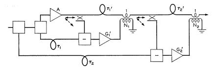
Fig. 11 — Two loop feed-forward network.
