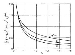
Fig. 5 — The statistical response of beam position relative to the sensor when lenses and sensors are disturbed simultaneously.
