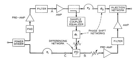
Fig. 22 — 75Mc feed forward system.
