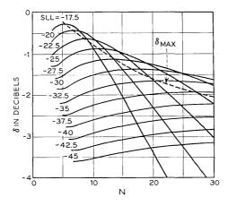
Fig. 13 — Difference pattern relative angular sensitivity,  $\delta$ .
