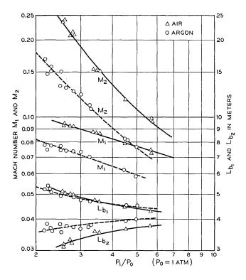
Fig. 2—Experimental Mach number and theoretical period of the beam size variation  $L_{b_1}$  and  $L_{b_2}$  (according to equation 3) at the beginning and the end of the pipe as a function of the initial pressure  $p_1/p_0$  for air and argon (temperature 22 °C). The experimental period of the beam size variation was constant and corresponded to the total length of the pipe (6.42m).
