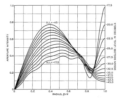
Fig. 6 — Circular aperture functions for N = 10.
