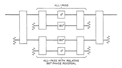
Fig. 2 — All-pass four way quadrature power divider.
