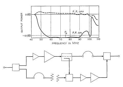
Fig. 39 — System output with reference line open, feed forward switched on and off.
