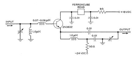
Fig. 31 — 60-90 Mc class A, 6.0-7.0 dB gain, 1.25 watt linear power stage.
