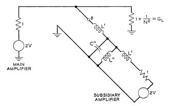
Fig. 20 — Shunt error injection using transformer network equivalent.
