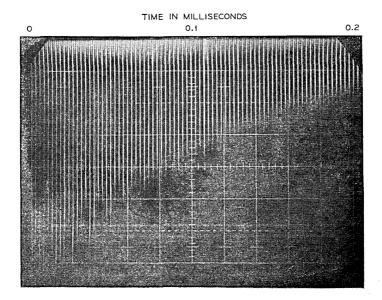
Fig. 5 — Pulse train from the 3-section line with the amplifier working.
