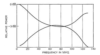
Fig. 28 — Coupling characteristics of 2 section coupler.
