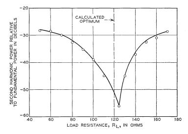
Fig. 3 — Experimental null in second harmonic distortion as a function of  $R_{L_2}$  using a Western Electric 20J transistor with  $V_o = 30$  volts,  $I_o = 100$  milliamperes, and  $R_s = 500$  ohms.
