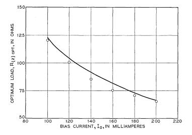
Fig. 10 — Measured (plotted points) and computed values (curve) of  $R_{(2)opt}$  as a function of bias current,  $I_o$ , using a Western Electric 20J transistor with  $R_{\bullet} = 500$  ohms and  $V_o = 25$  volts.
