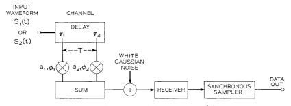
Fig. 1- Data transmission system model.
