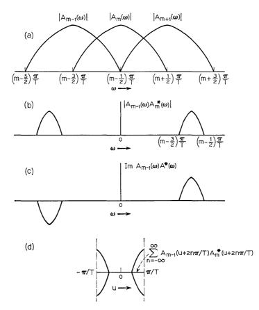
Fig. 7— (a) Spectra of transmitters which affect  $m^{\text{th}}$  output. (b) Magnitude of  $A_{m-1}(\omega)A_m^*(\omega)$ . (c) Required  $A_{m-1}(\omega)A_m^*(\omega)$ . (d) Demonstration that above  $A_{m-1}(\omega)A_m^*(\omega)$  satisfies constraint for periodic zeros.
