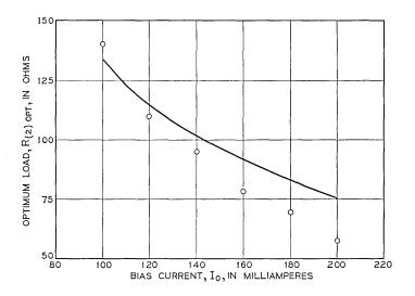
Fig. 9 — Measured (plotted points) and computed values (curve) of  $R_{(2)opt}$  as a function of bias current,  $I_o$ , using a Western Electric 20J transistor with  $R_o = 500$  ohms and  $V_o = 29$  volts.
