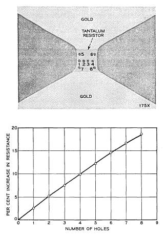
Fig. 12 — Resistor trimming by spot material removal.
