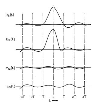
Fig. 5-Required time domain responses for distortionless transmission.
