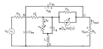
Fig. 1—High frequency nonlinear model.
