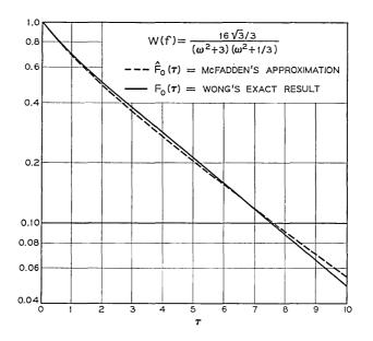
Fig. 2—Comparison of approximate and exact results for  $F_{*}(\tau)$ , the probability that a zero-crossing interval lasts longer than  $\tau$ .
