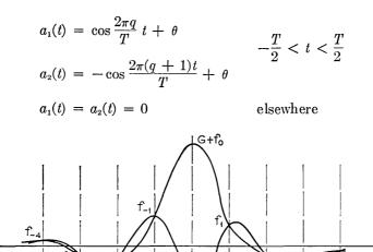
Fig. 10-Possible time domain responses for distortionless PSM system.
