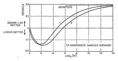
Fig. 6 — Comparison of linear and square-law detectors,  $P_{FA} = 5.10^{-4}$ .
