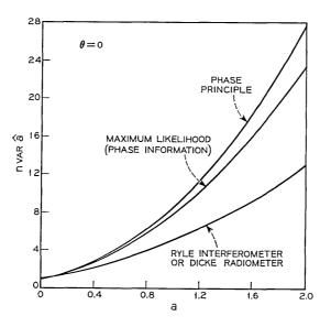
Fig. 5 — Theoretical accuracies of Ryle interferometer, Dicke radiometer, phase principle, and maximum likelihood principle (using only phase information) for measuring the spectral shape of a discrete radio source. Both the Ryle interferometer and the Dicke radiometer require some amplitude information.
