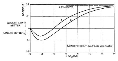
Fig. 7 — Comparison of linear and square-law detectors,  $P_{FA} = 0.09$ .
