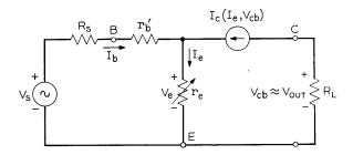
Fig. 6 — Low frequency nonlinear model.
