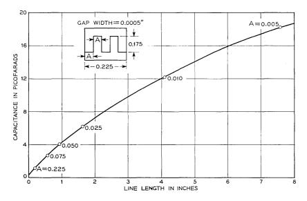
Fig. 11—Capacitance of serpentine gap capacitors as a function of total length of gap.
