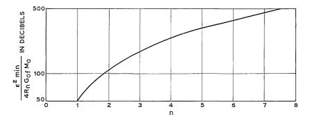
Fig. 8 — A typical plot when Butterworth polynomials are used to approximate the ideal noise performance characteristic. Even though n is a discrete variable the plot is given for all  $n \ge 1$ .
