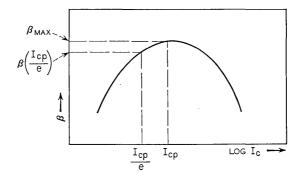
Fig. 8 — Current gain nonlinearity as a function of the bias current,  $I_c$ .
