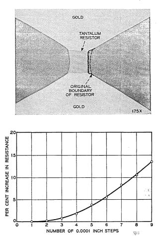
Fig. 13 - Resistor trimming by edge material removal.
