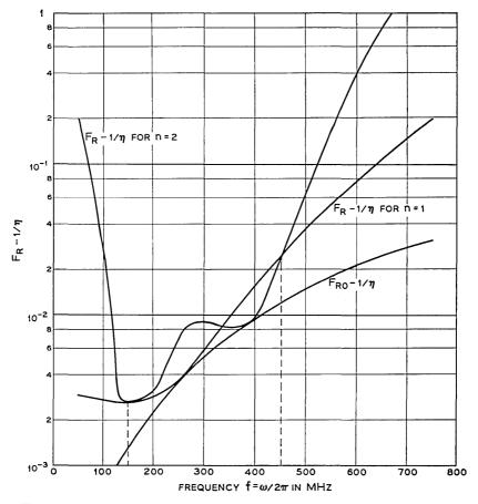
Fig. 10 — Noise factor  $F_R$  as a function of  $\omega$  for Chebyshev approximations of order n = 1,2. It is assumed that  $f_o = 31.83$  GHz,  $\eta = 0.70$ ,  $T_o = 290^{\circ}$ K,  $I_o = 500 \ \mu\alpha$ ,  $F_o = 2.0833$ , and  $\epsilon^2 = 1$ .
