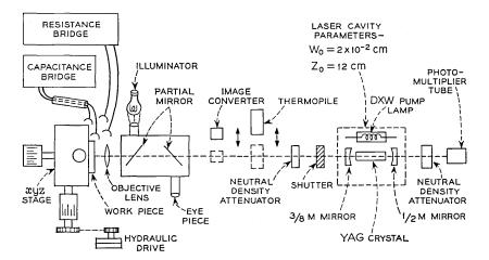
Fig. 1—Schematic diagram of laser machining apparatus.
