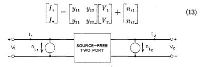
Fig. 3 — Separation of two port with internal noise sources into a source-free two port.
