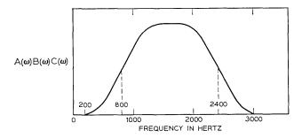
Fig. 13 — Zero stuffing spectrum for voiceband transmission.
