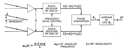
Fig. 1—Simplified implementation of a phase principle for measuring location or spectral shape of a discrete radio source. When source is located at  $d \sin \theta = \lambda/4$ ,  $\eta^{\dagger} \doteq 0$ . When source is located at  $\theta = 0$ , receivers scan in frequency and  $\eta^{\dagger}$  traces out a measure of spectral shape.
