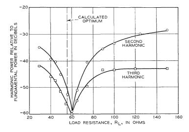
Fig. 11 — Simultaneous null in second and third harmonics as a function of load,  $R_L$ , with the same transistor and  $R_*$  as in Figs. 9 and 10. Here  $V_* = 29$  volts and  $I_* = 240$  mA.
