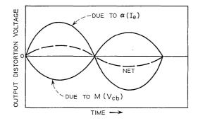
Fig. 2 — Cancellation of distortion components.
