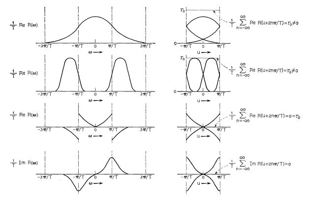
Fig. 1 — Such constraints on  $R(\omega)$  that  $r(qT) = 0, q \neq 0$ .
