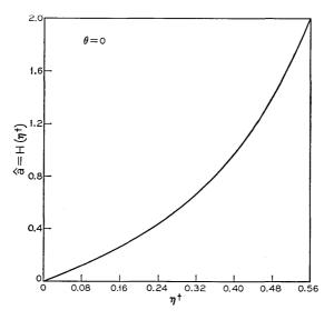
Fig. 4 — The theoretical calibration curve associated with the phase principle for measuring spectral shape of a discrete radio source. The receivers scan in frequency and  $\hat{a}$  traces out the spectral shape.
