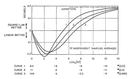
Fig. 5—Comparison of linear and square-law detectors. S/N (dB) in filter bandwidth, for  $P_D = (*)$ ,  $P_{FA} = 10^{-6}$ .
