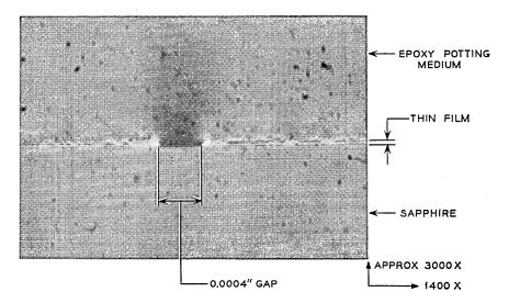
Fig. 4 — Cross section through gap machined in 3000 Å gold film showing the affected zone in the sapphire substrate.
