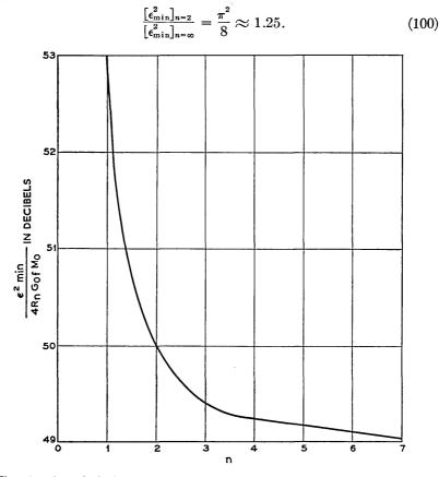
Fig. 11—A typical plot when Chebyshev polynomials are used to approximate the ideal noise performance characteristic. Even though n is a discrete variable the plot is given for all  $n \ge 1$ .
