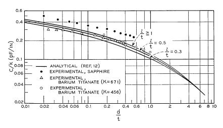
Fig. 6 — Capacitance of gap capacitors as a function of gap width. Comparison of analytical and experimental results.
