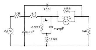
Fig. 4 — Linear model for  $I_e = 150$  mA,  $V_{cb} = 10V$ . With the indicated element values, this model matches the measured *h*-parameters shown in Fig. 5. The quality of the match at this bias point ( $I_e = 150$  mA,  $V_{cb} = 10V$ ) is typical.
