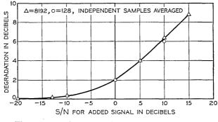
Fig. 4 — Degradation resulting from added CW signal.
