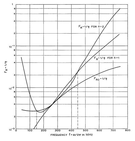
Fig. 7—Butterworth approximations of order n = 1,2. It is assumed that  $f_o = 31.83$  GHz,  $\eta = 0.70$ ,  $T_a = 290^{\circ}$ K,  $I_o = 500 \ \mu\alpha$ ,  $F_o = 2.0833$ , and  $\epsilon^2 = 1$ .
