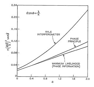
Fig. 3—Theoretical accuracies of Ryle interferometer, phase principle, and maximum likelihood principle (using only phase information) for measuring the angular location of a discrete radio source.
