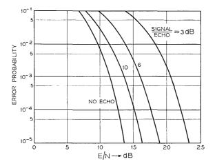
Fig. 6 — Error performance in single echo channel.
