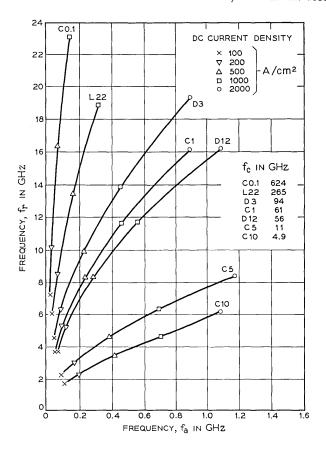
Fig. 6—Locus of poles of F as function of current density in the complex frequency plane. Note unequal scales of real and imaginary axes.
