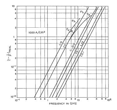
Fig. 3—Real part of 1 - 1/F as function of frequency for various structures. Current density 1000 amps/cm<sup>2</sup>.
