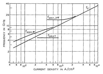
Fig. 18 — Frequency at which  $g_{\text{max}}$  occurs and  $f_r$  for diode R1.
