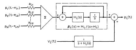
Fig. 3. — Simplified model of station i for the associated linear system.
