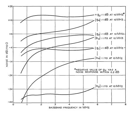
Fig. 7 — AM/PM intermodulation noise (k = 1.0 radian).
