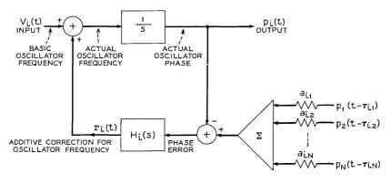
Fig. 2 — Model of station i of the associated linear system.
