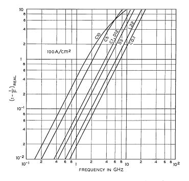
Fig. 2 — Real part of 1 - 1/F as function of frequency for various structures. Current density 100 amps/cm<sup>2</sup>.
