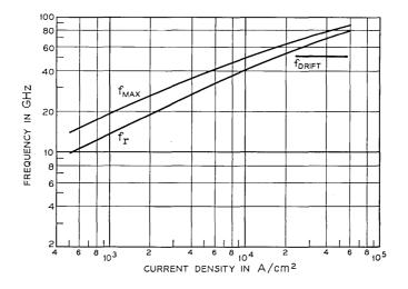
Fig. 16 — Frequency at which  $g_{\text{max}}$  occurs and  $f_r$  for diode D3.
