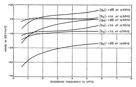
Fig. 6-Intermodulation noise due to transmission deviations.
