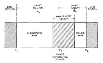
Fig. 1 — Schematic of IMPATT diode.
