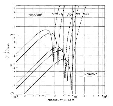
Fig. 4—Imaginary part of 1 - 1/F as function of frequency for various structures. Current density 100 amps/cm<sup>2</sup>. The vertical bars indicate  $f_{\rm crit}$ .
