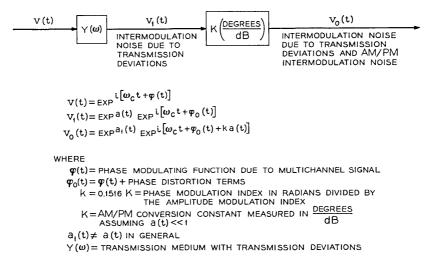
Fig. 1— Model illustrating sources of intermodulation noise due to transmission deviations and AM/PM conversion.
