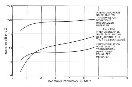
Fig. 11 — Representative radio system noise response.
