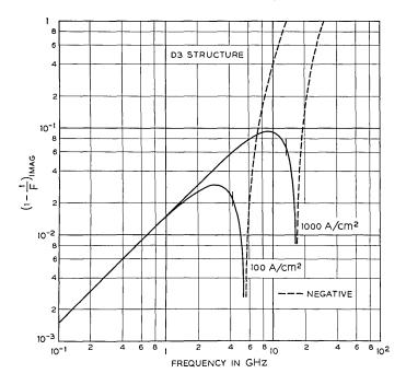
Fig. 5 — Imaginary part of 1 - 1/F as a function of current density for diode D3 at 100 and 1000 amps/cm<sup>2</sup>.
