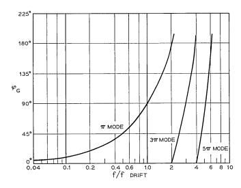
Fig. 8 — Negative of drift delay phase.
