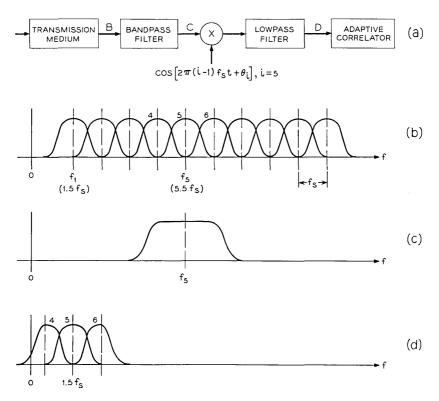
Fig. 6 — Reception of the signals in channel 5.
