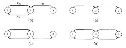
Fig. 4 - A system graph and three control graphs. (a) system graph; (b) inadequately connected control graph; (c) weakly connected control graph; (d) strongly connected control graph.
