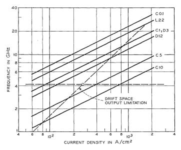
Fig. 19-Illustration of Read diode design considerations.
