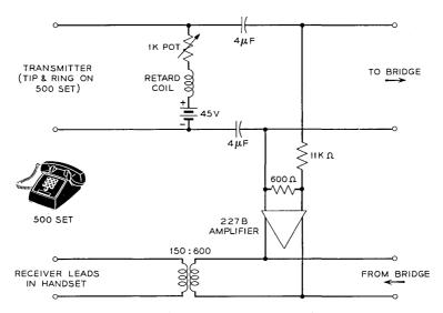
Fig. 4 — Modification of 500 type telephone set.
