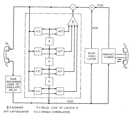
Fig. 1-System for demonstration of automatic transversal echo suppressor.
