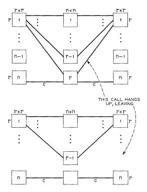
Fig. 3—Blocking state of A reached in r + 2 steps (only links in use indicated).
