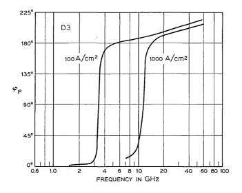
Fig. 7 — Phase of F for diode D3 at 100 and 1000 amps/cm<sup>2</sup>.
