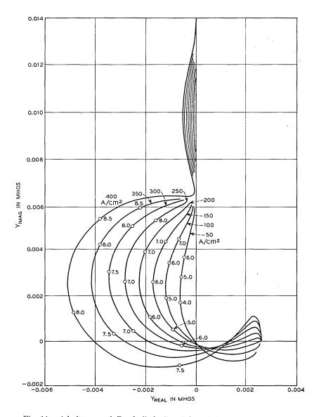
Fig. 14 — Admittance of Read diode R1. Selected frequencies, in GHz, are marked off on each curve.
