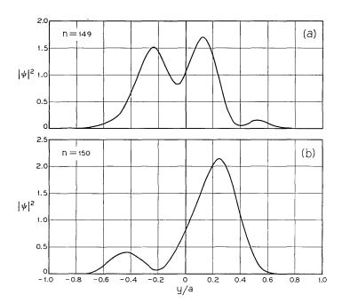
Fig. — 5 Field distortion after 150 lenses.  $P\,=\,0.956.$
