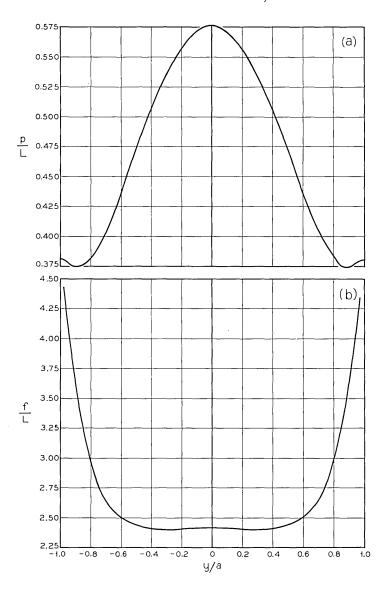
Fig. 2—(a) The principal surface p of the gas lens normalized with respect to the tube length L as a function of y/a. (b) The focal length f of the gas lens normalized with respect to the tube length L as a function of y/a.
