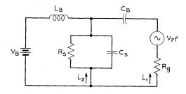
Fig. 18 — Equivalent circuit for biased operation.
