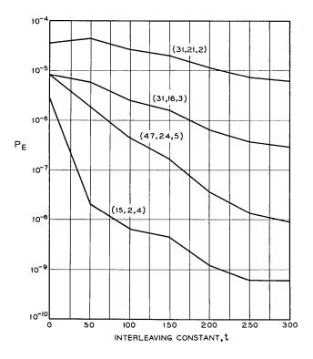
Fig. 4 — Error rate vs interleaving constant.
