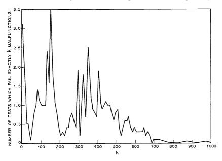
Fig. 3 — The number of tests which fail exactly k malfunctions, that is, the number of columns of the matrix with exactly k 1's in them. Curve has been smoothed by grouping 10 or 50 values of k.
