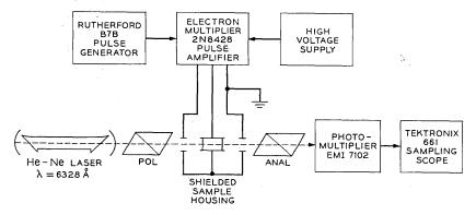
Fig. 11 — Experimental apparatus for unbiased pulse measurements.
