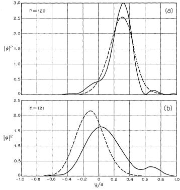
Fig. 8 — Field distortion of the field in the apertured lens after traversing 120 lenses. Solid curves represent the warped thin lens, P=0.976. Dotted curves represent a fictitious plane lens with the same focal length aberration, P=1.000.
