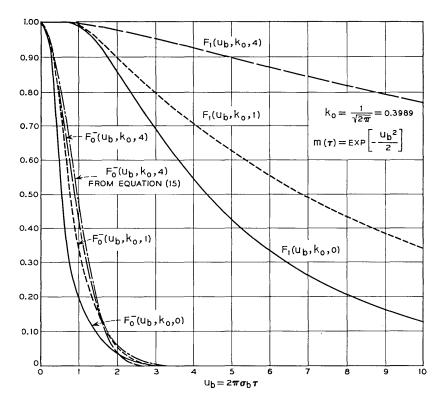
Fig.  $10 - F_0^-(u_b, k_0, a)$  is the probability that the duration of a fade of the Rayleigh process below the normalized level  $k_0$  lasts longer than  $u_b$ .  $F_1(u_b, k_0, a)$  is the probability that the interval between fades of the Rayleigh process below the normalized level  $k_0$  lasts longer than  $u_b$ .
