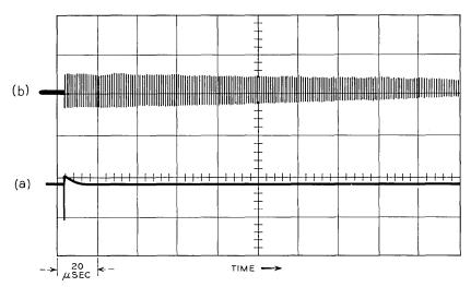
Fig. 13 — Ringing in light modulation at intermediate pulse widths (several  $\mu$ sec).
