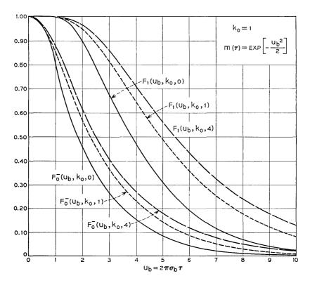
Fig.  $4 - F_0^-(u_b, k_0, a)$  is the probability that the duration of a fade of the Rayleigh process below the normalized level  $k_0$  lasts longer than  $u_b$ .  $F_1(u_b, k_0, a)$  is the probability that the interval between fades of the Rayleigh process below the normalized level  $k_0$  lasts longer than  $u_b$ .
