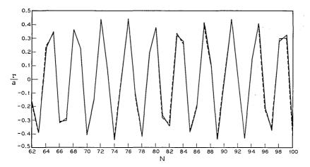
Fig. 4 — Comparison of ray trajectories through gas lenses and equivalent thin lenses. n = lens number, a = radius of gas lens, D = lens spacing,  $f_o = \text{focal}$  length of rays close to the optical axis, L = length of gas lens. D/a = 1200,  $D/f_o = 2.16$ , L/a = 50.
