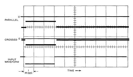
Fig. 12 — Very low frequency light modulation response.
