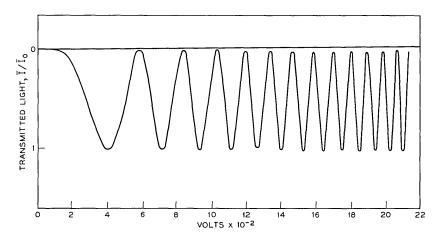
Fig. 3 — Light transmitted by KTN polarization switch as function of applied voltage.
