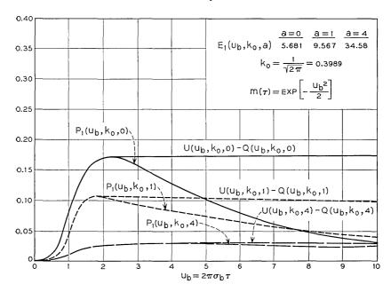
Fig.  $9 - P_1(u_b, k_0, a)$  is the probability density of the interval between fades of the Rayleigh process below the normalized level  $k_0$ . The autocorrelation function of the Gaussian process involved in the definition of the Rayleigh process is  $m(\tau)$  and the signal-to-clutter power ratio equals "a".
