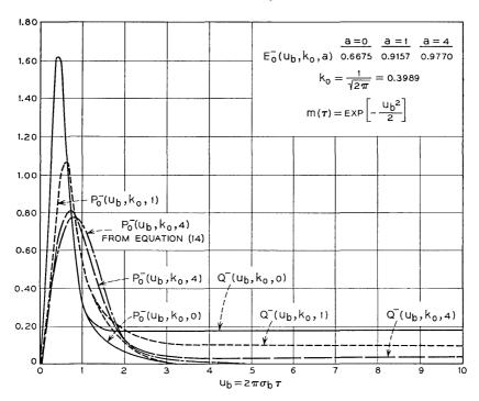
Fig. 8 —  $P_0^-(u_b, k_0, a)$  is the probability density of the duration of a fade of the Rayleigh process below the normalized level  $k_0$ . The autocorrelation function of the Gaussian process involved in the definition of the Rayleigh process is  $m(\tau)$  and the signal-to-clutter power ratio equals "a."
