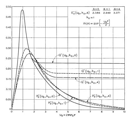
Fig.  $2-P_0^-(u_b\,,\,k_0\,,\,a)$  is the probability density of the duration of a fade of the Rayleigh process below the normalized level  $k_0$ . The autocorrelation function of the Gaussian process involved in the definition of the Rayleigh process is  $m(\tau)$  and the signal-to-clutter power ratio equals "a."
