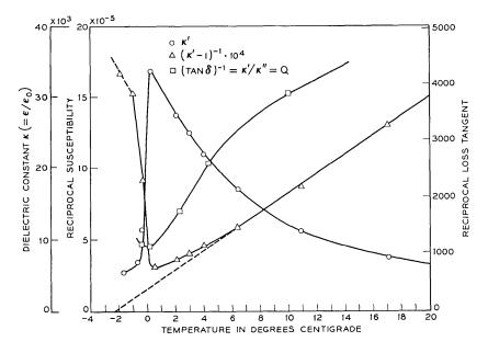
Fig. 5 — Dielectric behavior of KTN as a function of temperature.
