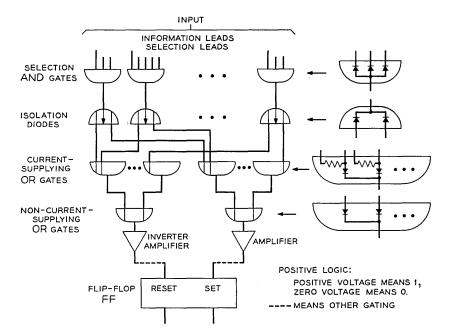
Fig. 8 — Simplified block diagram for flip-flop reading circuit.
