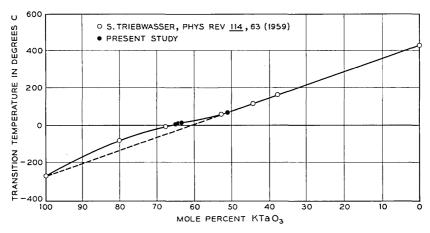
Fig. 7 — Compositional dependence of phase transition temperature in  $KTa_x$   $Nb_{1-x}O_3$  system.
