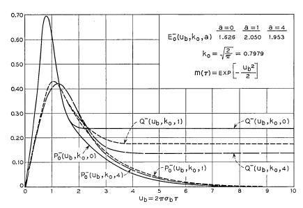
Fig.  $5 - P_0^-(u_b, k_0, a)$  is the probability density of the duration of a fade of the Rayleigh process below the normalized level  $k_0$ . The autocorrelation function of the Gaussian process involved in the definition of the Rayleigh process is  $m(\tau)$  and the signal-to-clutter power ratio equals "a".
