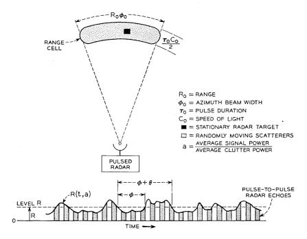
Fig. 1 — A model for studying the duration of fades associated with signal plus clutter. R(t,a) represents the envelope of the pulse-to-pulse radar echoes from the range cell. At the level R,  $\phi$  and  $\phi + \theta$  represent the duration of a fade and the interval between fades, respectively.
