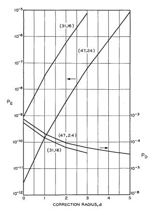
Fig. 1 — Error rates vs correction radius (no interleaving).
