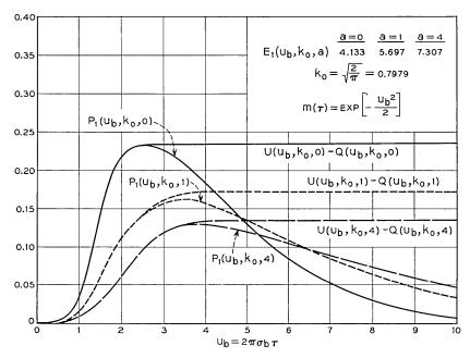
Fig.  $6 - P_1(u_b, k_0, a)$  is the probability density of the interval between fades of the Rayleigh process below the normalized level  $k_0$ . The autocorrelation function of the Gaussian process involved in the definition of the Rayleigh process is  $m(\tau)$  and the signal-to-clutter power ratio equals "a".
