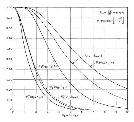
Fig. 7 —  $F_0^-(u_b, k_0, a)$  is the probability that the duration of a fade of the Rayleigh process below the normalized level  $k_0$  lasts longer than  $u_b$ .  $F_1(u_b, k_0, a)$  is the probability that the interval between fades of the Rayleigh process below the normalized level  $k_0$  lasts longer than  $u_b$ .
