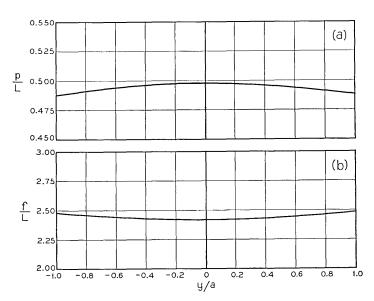
Fig. 12 — (a) Principal surface of gas lens of Fig. 11. (b) Focal length of gas lens of Fig. 11.
