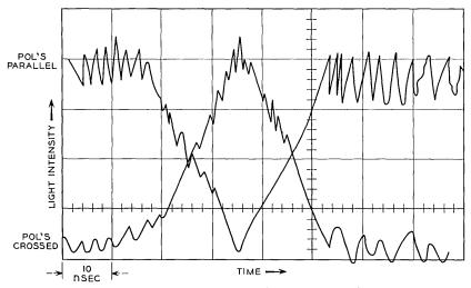
Fig. 16 — Clamped electro-optic pulse modulation.
