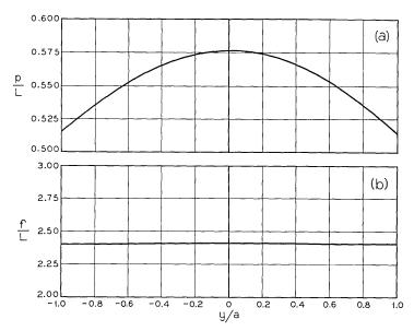
Fig. 7—(a) Principal surface of the apertured lens. (b) Focal length of the apertured lens.
