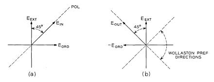
Fig. 2 — Retardation of plane of polarization by half-wave plate.
