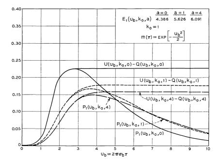
Fig.  $3 - P_1(u_b, k_0, a)$  is the probability density of the interval between fades of the Rayleigh process below the normalized level  $k_0$ . The autocorrelation function of the Gaussian process involved in the definition of the Rayleigh process is  $m(\tau)$  and the signal-to-clutter power ratio equals "a."
