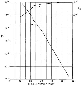
Fig. 3 — Error rates of double error-correcting  $\{n, \lceil (n+1)/2 \rceil \}$  codes.
