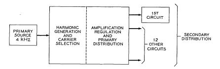
Fig. 19 — Carrier-supply — general plan.
