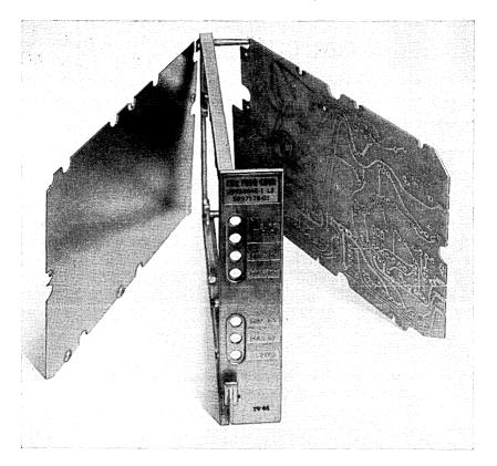
Fig. 7 — Basic frame, printed wiring board, and shield.
