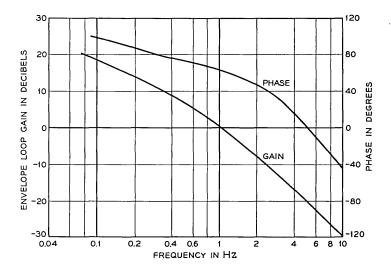
Fig. 11 — Envelope open loop phase and gain characteristic of double channel regulator.
