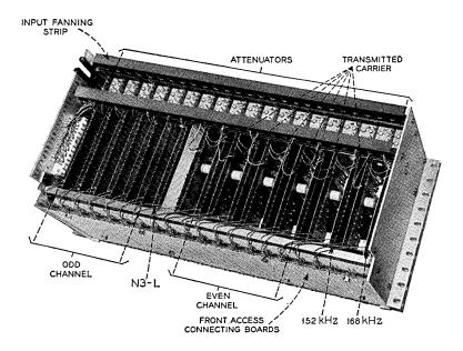
Fig. 25 — Secondary carrier distribution panel (rear view).
