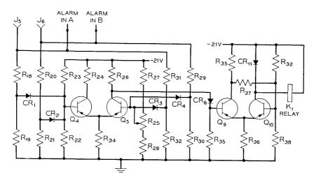
Fig. 28 - Monitoring circuit.
