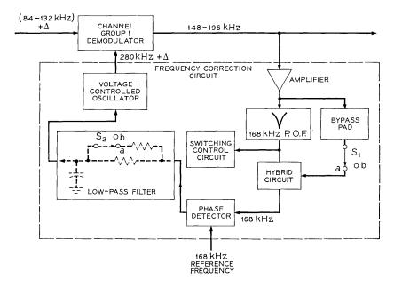
Fig. 14 — Block diagram of frequency correction circuit.
