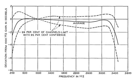
Fig. 5 — N3 channel VF gain-frequency characteristic.
