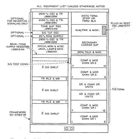
Fig. 5-J99300D N3 carrier 24-channel packaged terminal frame (7 feet high) with patching jacks.
