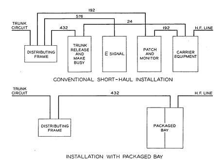
Fig. 3 — Comparison of installer cabling — number of conductors.
