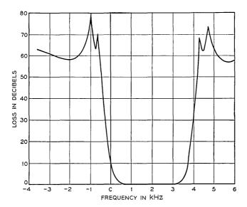
Fig. 4 — N3 channel filter discrimination.
