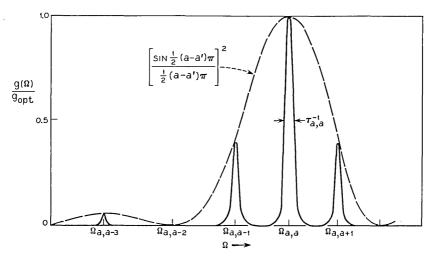
Fig. 4 — A plot of  $g(\Omega)$ , the enhancement factor, as a function of frequency, for the condition  $\Psi=0$  and L=L'.
