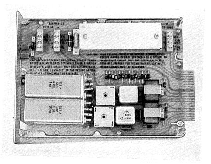
Fig. 17—Line terminating unit.
