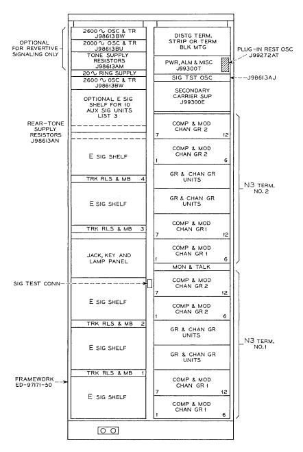
Fig.  $4-J99300\Lambda$  N3 carrier 48-channel packaged terminal frame (11 feet, 6 inches high) with patching jacks.
