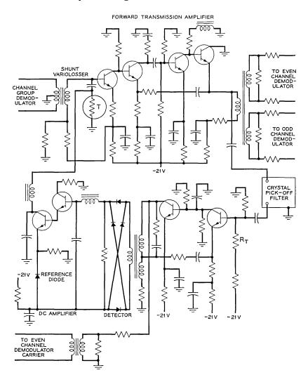
Fig. 8 — Double-channel regulator.
