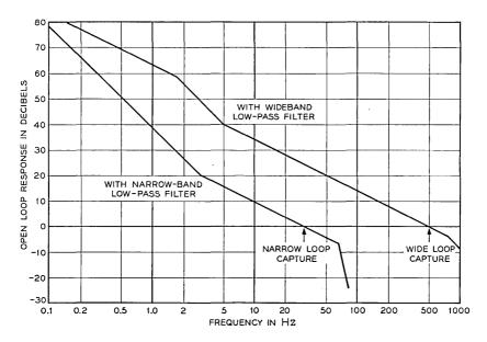
Fig. 15 — Open loop response of correction circuit.
