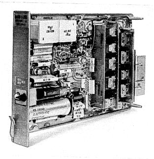
Fig. 14 - Alarm and restoral unit.
