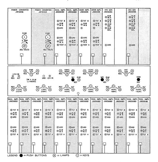
Fig. 24 — Switch and alarm panel in relation to plug-in units (alternate plug-in positions shown shaded).
