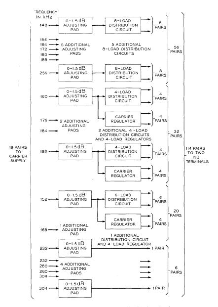
Fig. 30 — Secondary carrier distribution circuit.
