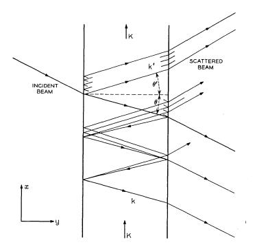
Fig. 1 — Schematic arrangement for acoustic scattering of light in an optically resonant geometry. In this case the acoustic wave travels parallel to the mirror planes.
