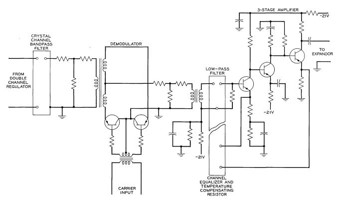
Fig. 5 — Channel demodulator circuit.
