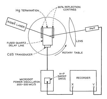
Fig. 5 — Experimental apparatus for studying acoustic scattering in a Fabry-Perot resonator.
