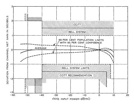
Fig. 7 — N3 channel compandor tracking characteristic.
