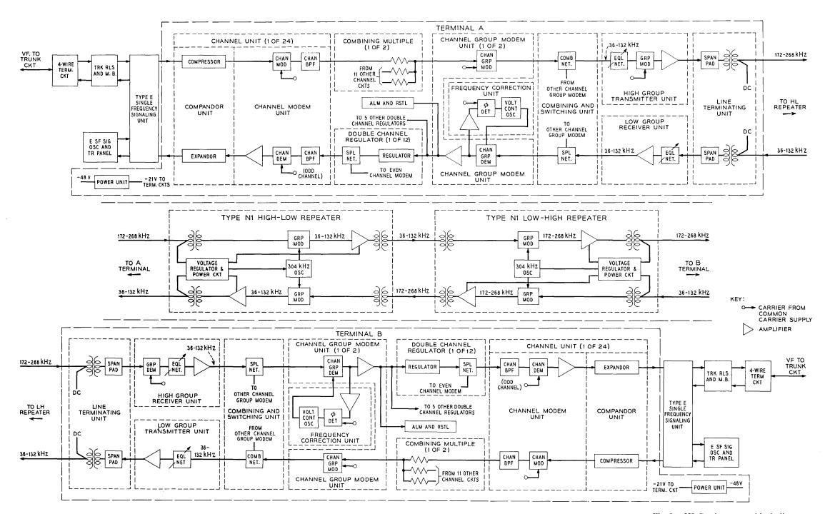
Fig. 2 — N3 Carrier system block diagram.
