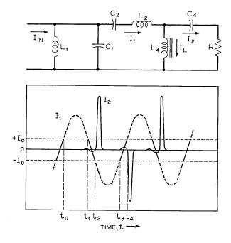
Fig. 24 — Typical pulse waveforms.
