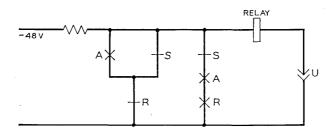
Fig. 31 — Relay control circuit.
