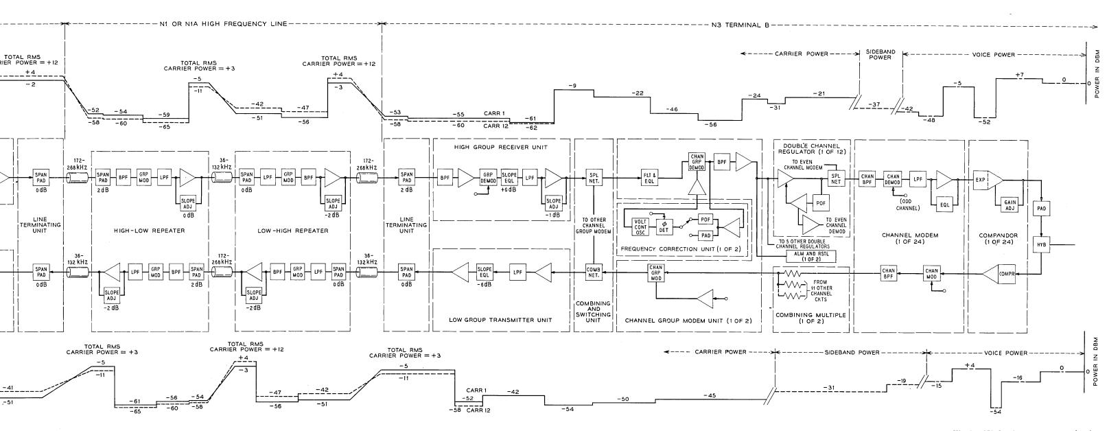
Fig. 3 — N3 Carrier system power levels.
