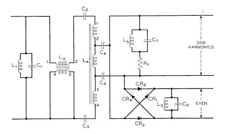
Fig. 23 — Harmonic generator circuit.
