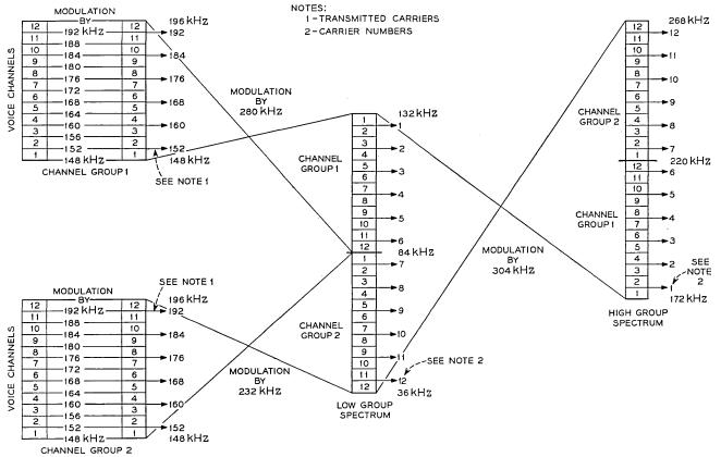
Fig. 1 — N3 carrier system frequency allocation.
