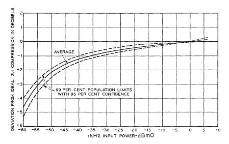
Fig. 8 — N3 channel compressor tracking characteristic.
