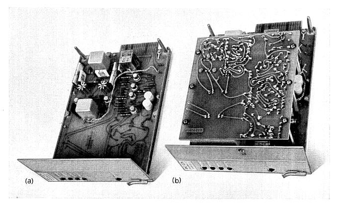
Fig. 21 — 4-kHz generator plug-in unit. ((a) for use with external source; (b) with 61A oscillator mounted in place.)
