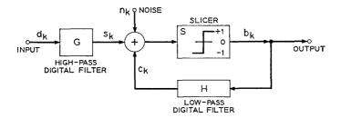
Fig. 1—Binary pulse regenerator with low-frequency restoration.
