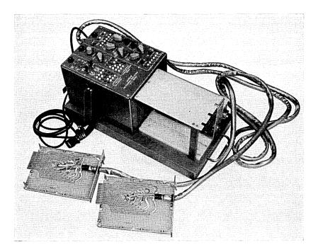
Fig. 19 — Plug-in unit terminal test stand.
