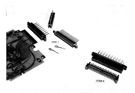
Fig. 9 — Plug-in unit connectors.
