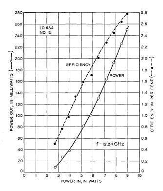
Fig. 1 — Output power and efficiency vs input power.
