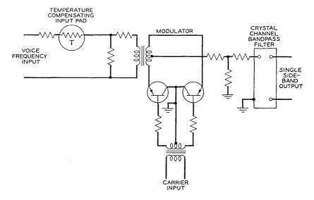
Fig. 3 — Channel modulator circuit.
