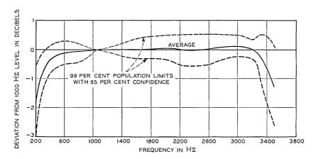
Fig. 6 — N3 channel sideband gain-frequency characteristic.
