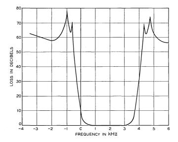
Fig. 4 — Measured insertion loss N3 channel band filter.
