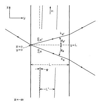
Fig. 3 - Scattering interaction geometry for coupled-mode calculation.
