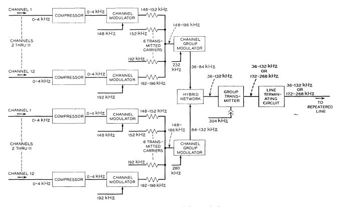
Fig. 1 — N3 transmitting terminal.
