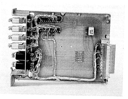
Fig. 16 — Combining and switching unit.
