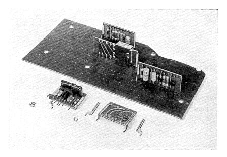
Fig. 10 — Slave board technique for obtaining high component density.
