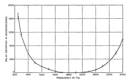
Fig. 9 — N3 channel delay distortion characteristic.
