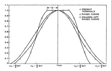
Fig. 6 — Envelopes of amplitude spectra.
