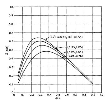
Fig. 3 —  $\sum (\frac{1}{2})$  vs  $\theta/\pi$  for l/L=0.25 and four values of the parameter D/L. 1014
