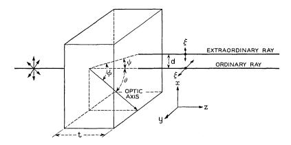
Fig. 13 — Angles and directions in uniaxial crystal,
