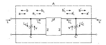
Fig. 1 — Basic configuration of the unilateral parametric amplifier.
