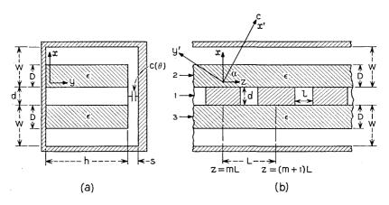
Fig. 1 — Comb structure loaded with ruby. The c axis of ruby makes an angle  $\alpha$  with the z direction.
