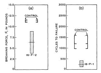
Fig. 19 — Inferior weld test, test number 16: (a) destructive strength — inferior welds show 55 per cent of the strength of good welds, based on the means of the distributions; (b) bending fatigue life (without insulation, lightly loaded bending) — inferior welds show 17 per cent of the bending fatigue life of good connections, based on the means of the distributions.
