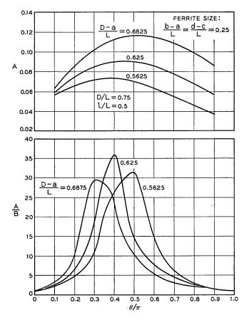
Fig. 13 — A and A/B vs  $\theta/\pi$ : D/L = 0.75, l/L = 0.5; ferrite size, (b-a)/L = (d-c)/L = 0.25  $(0.02 \times 0.02 \text{ inch})$ .
