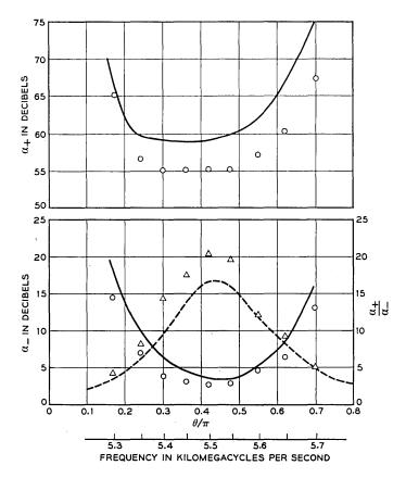
Fig. 17 — Measured and calculated forward and reverse absorption. Ferrite disks =  $0.03 \times 0.03 \times 0.002$  inch (35 pieces). L=0.08 inch, D=0.06 inch, l=0.04 inch,  $\alpha=0.009$  inch,  $\Delta H=251$  oe,  $4\pi M=1750$  oe. Solid lines are the calculated  $\alpha_{\pm}$  and the circled points are measured. Broken line is the calculated  $\alpha_{+}/\alpha_{-}$  and the triangles are measured points.
