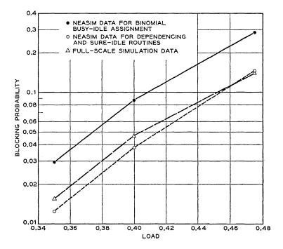
Fig. 12 — Comparison of NEASIM results (with and without dependencing and sure-idles) with full-scale simulation data for a realistically complex network.
