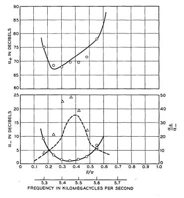
Fig. 16 — Measured and calculated forward and reverse absorption. Ferrite size:  $0.02 \times 0.02 \times 0.02$  inch (71 pieces). L=0.08 inch, D=0.06 inch, l=0.04 inch, a=0.01 inch,  $\Delta H=223$  oe,  $4\pi M=1750$  oe. Solid lines are the calculated  $\alpha_{\pm}$  and the circled points are measured. Broken line is the calculated  $\alpha_{+}/\alpha_{-}$  and the triangles are measured points,
