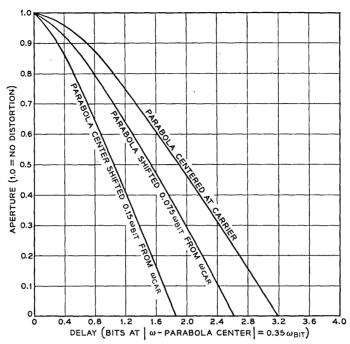
Fig. 17 — Apertures for parabolic delay; aperture = 0 indicates system makes errors with no noise.
