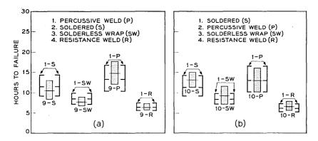
Fig. 11 — Vibration fatigue life and orders of merit after corrosion tests. (a) Test number 9 (three months); (b) test number 10 (six months).
