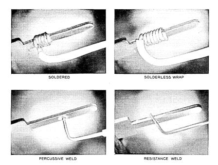
Fig. 3 — Typical examples of general wiring connections.
