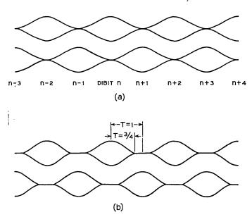
Fig. 5 — Envelope shaping: (a) full raised-cosine shaping, (b) modified shaping used in present data terminals.
