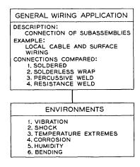
Fig. 1 — Test program for permanent connection comparison.
