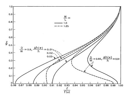
Fig. 7 —  $\omega$ - $\beta$  diagram for different W/L and  $\Delta h(\pi)/h$ . D/W=0.9, L-l=l=d.
