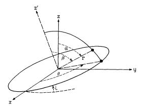
Fig. 3 — Orbital spherical coordinate system.
