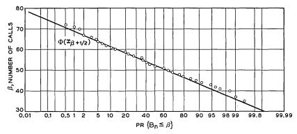
Fig. 8 — Cumulative distribution for GRAPH of Fig. 3 ( $p = p_2 = 0.5$ ) in a run of 201,600 calls in which the number of blocked calls was noted for every 1,008 calls run. The points are experimental data; the line is the theoretical distribution,  $\Phi(x_{\beta+1})$
