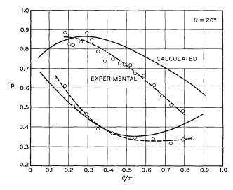
Fig. 9 — A comparison of the theoretical and experimental results for a ruby with  $\alpha=20^\circ$ . The solid line is the theoretical curve and the points are the experimental measurements.
