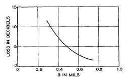
Fig. 6 — Loss vs radius of aperture at f/15 and 6943 Å.
