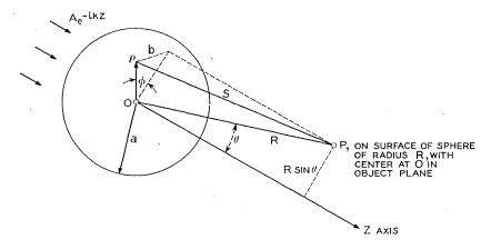
Fig. 15 — Angles and dimensions used to determine  $E(\theta)$ .
