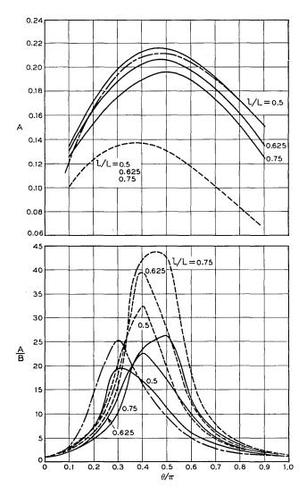
Fig. 14 — A and A/B vs  $\theta/\pi$ : ferrite size, (b-a)/L=(d-c)/L=0.375 (0.03  $\times$  0.03 inch); solid line, D/L=0.75, (D-a)/L=0.6875 (a=0.005 inch); dashed line, D/L=1.0, (D-a)/L=0.8125 (a=0.015 inch); irregular dashed line, D/L=1.0, (D-a)/L=0.9375 (a=0.005 inch); l/L=0.5.
