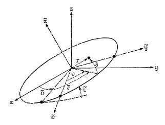
Fig. 4 — Rotating spherical orbital coordinates.
