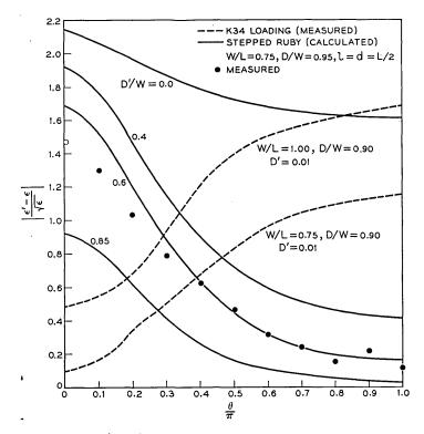
Fig. 11 —  $\left| \frac{\epsilon' - \epsilon}{\sqrt{\epsilon}} \right|$  vs  $\theta/\pi$  for ruby shaping and K34 loading.
