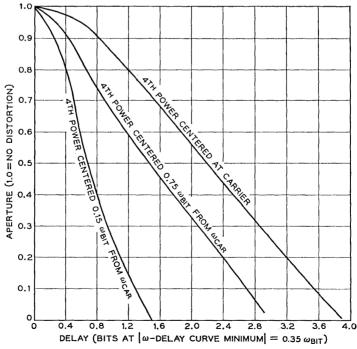
Fig. 18 — Aperture vs delay for fourth-power delays.
