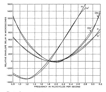
Fig. 16 — Representations of some typical lines by sinusoidal approximations (primes are approximations). K=2 links K carrier, K=3 links K=3
