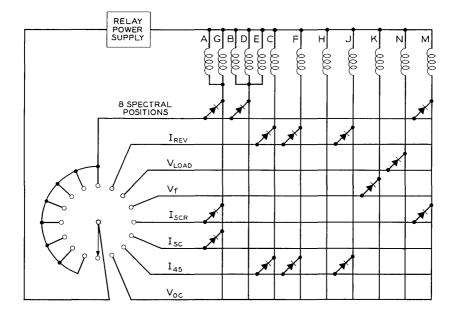
Fig. 7 — Diode matrix for activation of relays.
