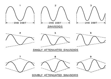
Fig. 4 — Noise waveshapes; all shapes are shown prior to detection but subsequent to transmission.
