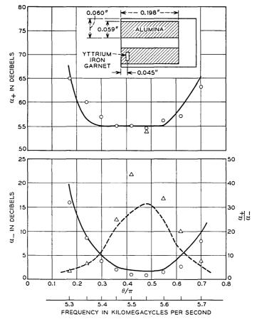
Fig. 15 — Measured and calculated forward and reverse losses. Ferrite disks  $0.02 \times 0.02 \times 0.02$  inch (71 pieces). L=0.08 inch, D=0.06 inch, l=0.04 inch, a=0.016 inch,  $\Delta H=223$  oe,  $4\pi M=1750$  oe. Solid lines are the calculated  $\alpha_{\pm}$  and the circled points are measured. Broken line is the calculated  $\alpha_{+}/\alpha_{-}$  and the triangles are measured points.
