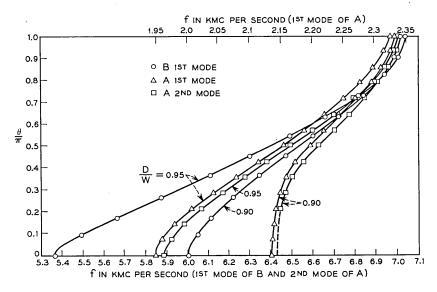
Fig. 13 — Comparisons of the first and the second passbands of the loaded comb structures. The fingers are  $0.040 \times 0.040$  inch in cross section and l = 0.040 inch.
