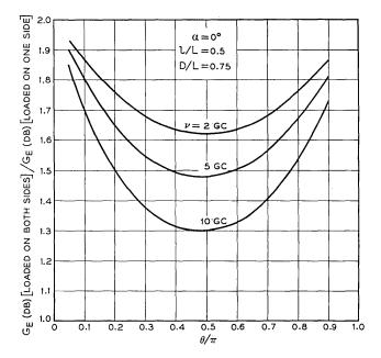
Fig. 7 — The ratio of the electronic gain (in db) of a maser when loaded on both sides to that when loaded on one side. The structures are otherwise identical, with  $\alpha = 0^{\circ}$ , l/L = 0.5, D/L = 0.75.
