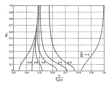
Fig. 6 — Calculated  $\omega$ - $\beta$  diagram as the thickness of the dielectric is changed. It is assumed that L-l=l=d, W/L=1.25,  $K(\pi)C(\pi)c/h=0.05$ , and  $\epsilon=9$ . The frequency scale is normalized to  $f_0(\pi)$ , the frequency at  $\theta=\pi$  for the empty comb.
