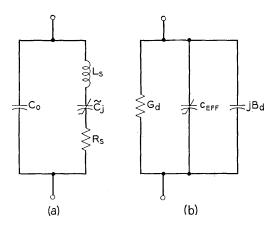
Fig. 7 — Equivalent circuits of a variable capacitance diode.
