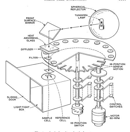
Fig. 4 — Optical and mechanical system.
