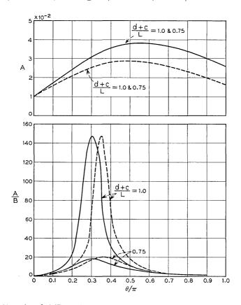
Fig. 11 — A and A/B vs  $\theta/\pi$  for the following parameters: D/L = 0.75, l/L = 0.5; ferrite size, (b-a)/L = (d-c)/L = 0.125 (0.01  $\times$  0.01 inch); solid curves for (D-a)/L = 0.6875 (a = 0.005 inch); broken curves for (D-a)/L = 0.625 (a = 0.01 inch).
