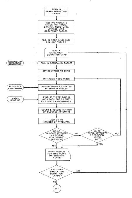
Fig. 5 — Flow diagram for the NEASIM program.
