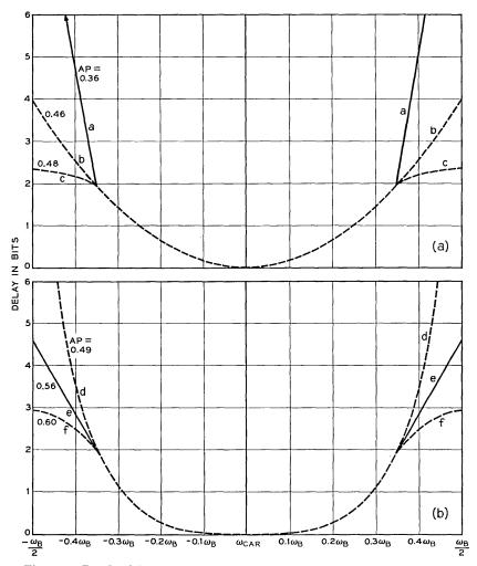
Fig. 22 — Bandwidth requirements, all curves symmetric about  $\omega_{\text{car}}$ : (a) quadratic delay,(b) fourth-power delay.
