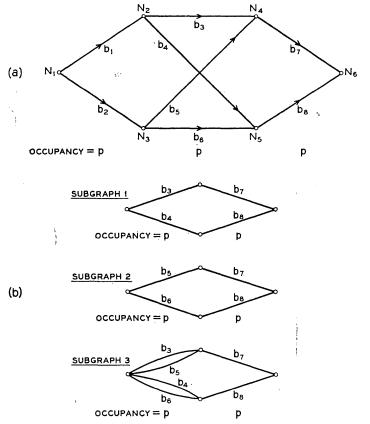
Fig. 2 — (a) GRAPH of the network of Fig. 1, with occupancy p on each of the branches. (b) The subgraphs of the GRAPH.
