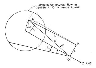
Fig. 16 — Angles and dimensions used to determine  $E(\rho)$ .
