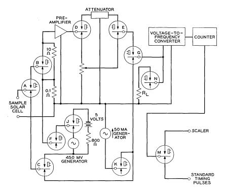
Fig. 6 — Switching of signal paths.
