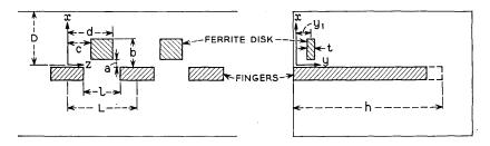
Fig. 10 — Ferrite disk isolators imbedded in the comb structure.
