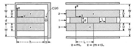
Fig. 1 — Cross sections of the comb structure.
