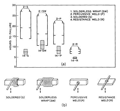
Fig. 17 — (a) Vibration fatigue life with configuration omitting 90° bend in the lead-off wire, test number 14 (with insulation); order of merit, based on vibration fatigue life. (b) Vibration configuration omitting 90° bend.
