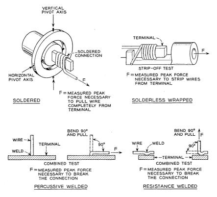
Fig. 23 — Destructive tests.
