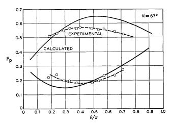
Fig. 8 — A comparison of the theoretical and experimental results for a ruby with  $\alpha=67^{\circ}$ . The solid line is the theoretical curve and the points are the experimental measurements.
