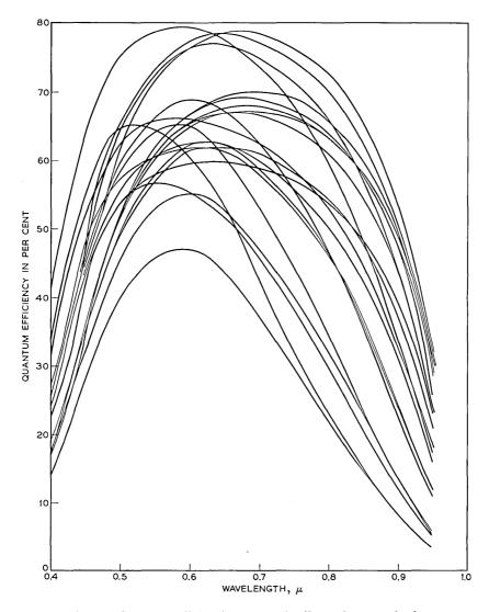
Fig. 2 — Quantum efficiencies of set of cells used as standards.
