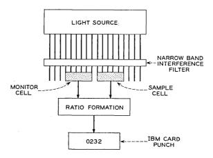
Fig. 1 — Method of measuring ratio of quantum efficiencies.
