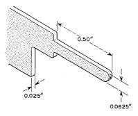
Fig. 22 — General wiring terminal; material is nickel-silver.
