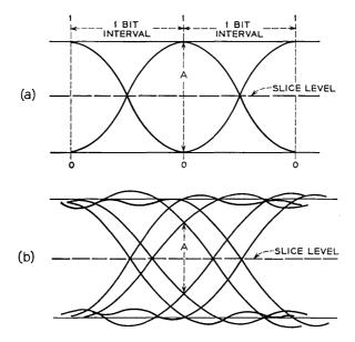
Fig. 7 — Eye patterns. (a) Undistorted eye: tracings result from patterns 000, 001, 010, 011, 110, and 111; A is eye aperture normalized for undistorted eye to 1.0. (b) Distorted eye: figure shows some tracings; total eye formed from all possible three-bit intervals.
