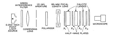
Fig. 8 — Pictorial diagram of four-unit deflection system.
