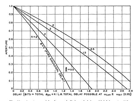
Fig. 20 — Aperture vs delay for parabolic bounded sinusoidal delays,  $\theta = 90^{\circ}$ .
