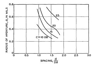
Fig. 5 — Radius of aperture vs center-to-center spacing at constant crosstalk, f/15 and 6943 Å.
