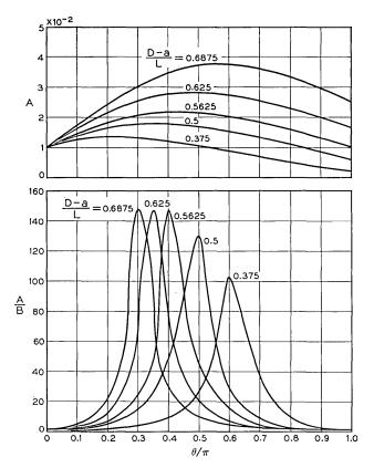
Fig. 12 — A and A/B vs  $\theta/\pi$  for the following parameters: D/L = 0.75, l/L = 0.5; ferrite size, (b-a)/L = (d-c)/L = 0.125 (0.01  $\times$  0.01 inch); (d+c)/L = 1.0 (ferrite on an axis midway between the adjacent fingers).
