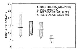
Fig. 21 — General wiring fatigue life summary (with insulation); order of merit, based on vibration fatigue life.
