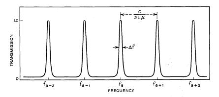
Fig. 2 — Transmission vs frequency for a Fabry-Perot etalon.
