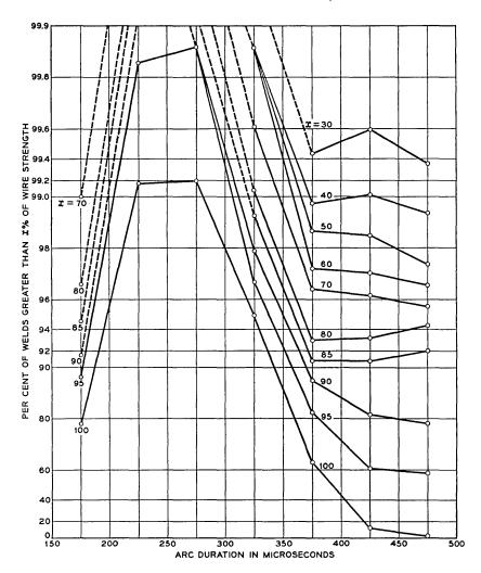
Fig. 6 — Results of test No. 1, weld strength vs are duration: 24-gauge copper wire, nickel-silver terminal, capacitance 2300  $\mu f$ , resistance 0.04 ohm, diagonal-cut wire tip, variable wire velocity.
