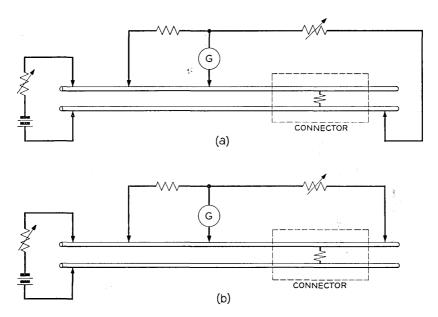
Fig. 4 — Modified Kelvin bridge. Circuit (a) is used to measure the resistance of the top lead wire in to the point of contact, plus the resistance between the two wires. Circuit (b) measures merely the lead wire resistance. The contact resistance is calculated from these two measurements.
