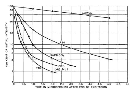
Fig. 9 — Form of decay of various fast-decay phosphors.
