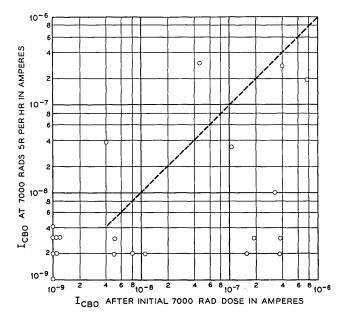
Fig. 26. — Correlation of change in  $I_{CBO}$  after a screening dose at 8  $\times$  10<sup>5</sup> rads/hr with subsequent changes at 5 rads/hr.
