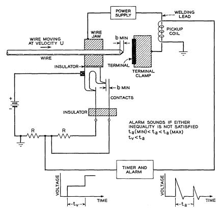
Fig. 5 — Wiring schematic of monitoring circuit.
