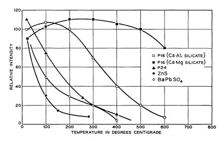
Fig. 11 — Temperature dependence of emission intensity for various fast-decay phosphors.
