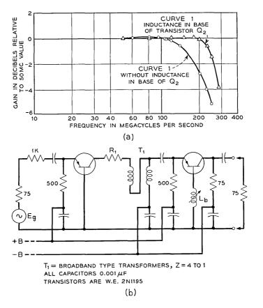
Fig. 2 — (a) Measured responses of series peaking circuit, (b) circuit used to measure interstage series peaking response.
