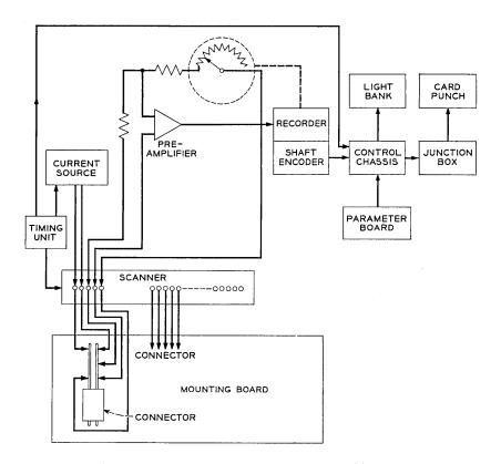
Fig. 6 — Block diagram of automated bridge.
