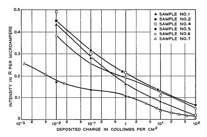
Fig. 7 — Aging of emission intensity of various P16 samples.
