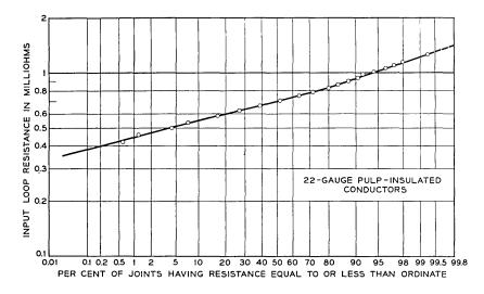
Fig. 13 — Initial resistance distribution of 100 B Wire Connector joints.
