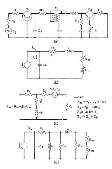
Fig. 1 — (a) Typical interstage circuit, (b) equivalent circuit for the interstage, (c) equivalent circuit for computation of input impedance, (d) equivalent interstage circuit including losses.
