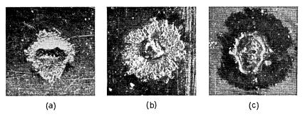
Fig. 2—Appearance of weld breaks: (a) Excessively short arc durations do not provide sufficient melting energy and result in a weak weld due to the reduced area of fusion. (b) Arc durations within the optimum range result in a strong weld. (c) Excessively long arc durations allow excessive heat conduction losses and result in a weak weld due to premature solidification.
