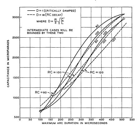
Fig. 4 — Computed curves for  $t_{a(\max)}$ : 24-gauge copper wire, nickel-silver terminal, welding voltage 50v,  $V_1=20\mathrm{v}$ ,  $V_2=10\mathrm{v}$ , K=7 watt(sec.)<sup>3</sup>.
