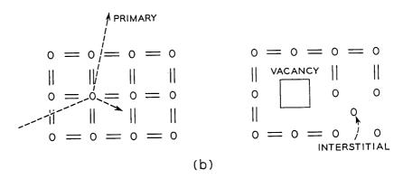
Fig. 1. — (a) Production of hole-electron pairs by collision of a charged particle with electrons of a semiconductor. (b) Production of lattice defects by collision of particles with the nuclei of a semiconductor.
