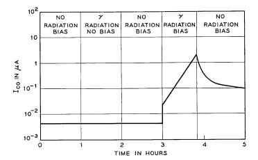
Fig. 2. — The response of  $I_{CBO}$  of a diffused silicon transistor to either radiation or bias alone or to both together. Radiation dose rate  $8.5 \times 10^5$  rads/hr.
