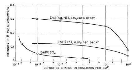
Fig. 8 — Aging of emission intensity of ZnO(Zn), BaPbSO<sub>4</sub>, and ZnS(Ag,Ni) phosphors.
