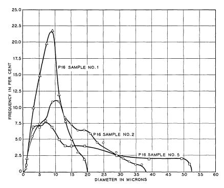
Fig. 3 — Particle size distribution of three representative P16 phosphors.
