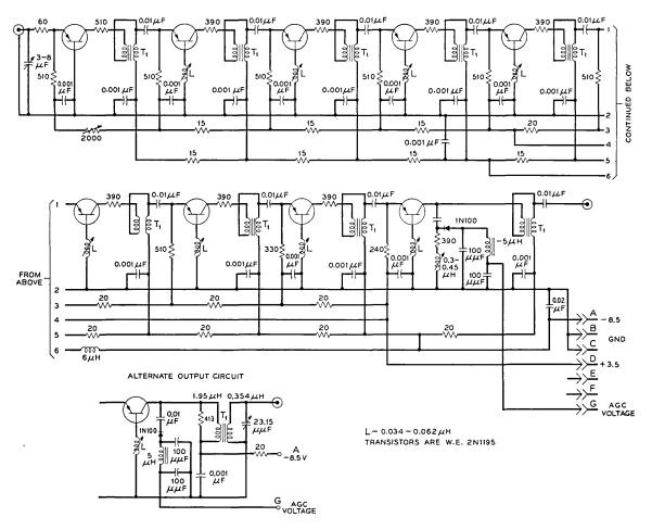
Fig. 5 — IF amplifier schematic.
