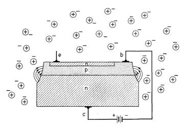
Fig. 4. — A model of a reverse-biased transistor in a gas atmosphere ionized by radiation.
