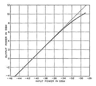
Fig. 8 — Compression characteristic for amplifier of Fig. 5.
