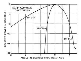
Fig. 8 — Typical free-space patterns of parabolic antennas (750 mc).
