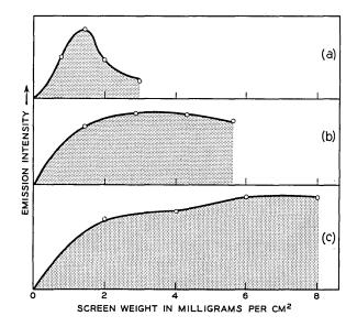
Fig. 2 — Luminescent intensity versus screen weight for three representative phosphors: (a) P16 sample \$1, (b) P16 sample \$2, (c) P15. Samples used for obtaining curves (a) and (b) have different particle size as shown in Fig. 3.
