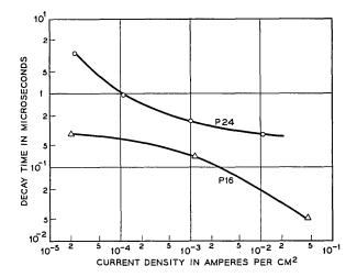
Fig. 10 — Decay time of a representative P16 and P24 sample as a function of the excitation level (as determined by the exciting current density).
