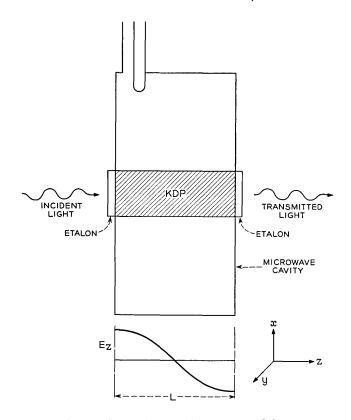
Fig. 1 — Schematic of Fabry-Perot modulator.
