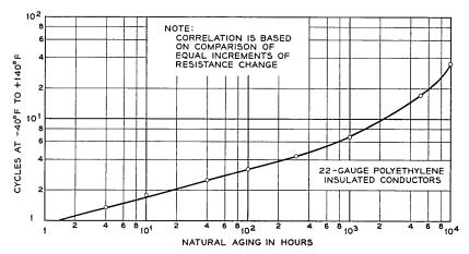
Fig. 12 — Correlation of  $-40^{\circ}$ F to  $+140^{\circ}$ F temperature cycles to natural aging.
