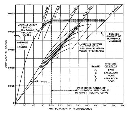
Fig. 8 — Graphical representation of over-all test program.
