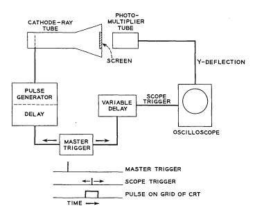
Fig. 1 — Schematic of the circuit for measuring decay times of fast-decay cathode-ray tube phosphors.
