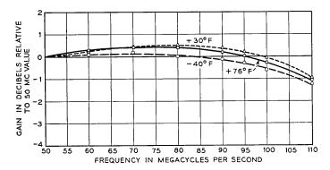
Fig. 10 — Frequency response vs temperature of IF amplifier.
