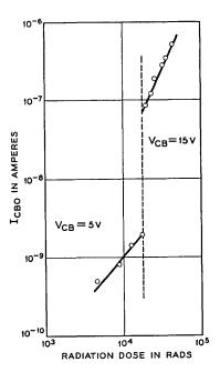
Fig. 10. — Influence of change in collector bias on degradation of  $I_{CBO}$  . Dose rate 8.5  $\times$  10<sup>5</sup> rads/hr.
