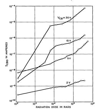
Fig. 11. — Dependence of degradation in  $I_{CBO}$  on collector bias.
