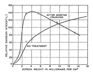
Fig. 4 — Effect of mechanical treatment of a P24 phosphor on its emission intensity and optimum screen weight.
