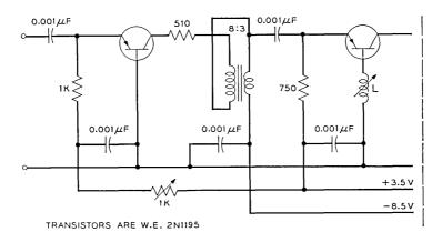
Fig. 12 — Input circuit for low noise figure.
