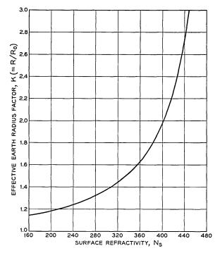
Fig. 3 — Effective earth-radius factor vs refractivity at surface.
