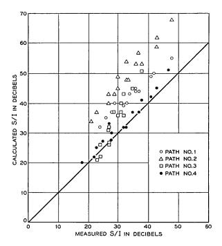
Fig. 12 — Calculated single-echo S/I vs average measured (unadjusted) S/I.
