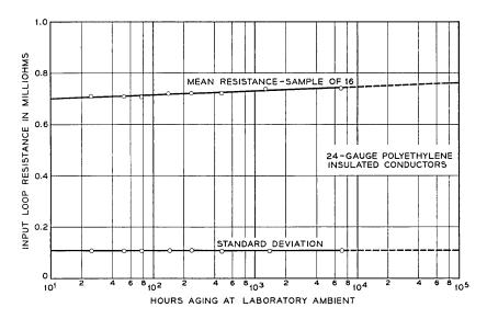
Fig. 14 — Performance of B Wire Connector joints under natural aging.
