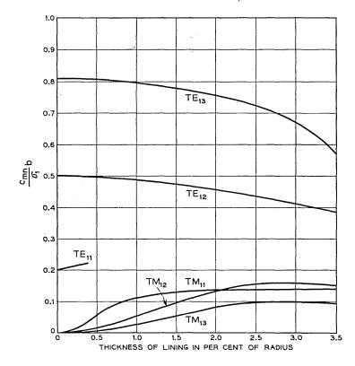
Fig. 15 — Coefficients  $c_{mn}$  of coupling between TE<sub>01</sub> and TE<sub>1n</sub> and TM<sub>1n</sub> in axially offset lined waveguide.  $b/\lambda = 4.70$ ,  $\epsilon_r = 2.5$ .
