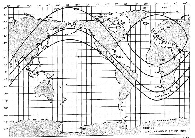
Fig. 17 — Qualities of service from a West-European point for a system of 24 satellites in 6000-mile orbits (12 polar and 12  $28^{\circ}$ -inclined).
