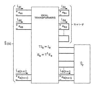
Fig. 4 — Realization of  $\hat{\mathbf{S}}(s)$  when the normal rank of  $[\mathbf{1}_{n+1} + \hat{\mathbf{S}}(s)]$  is r. where
