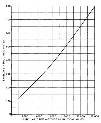
Fig. 2 — Satellite period vs circular orbit altitude. The period of elliptical orbits is found by using a circular orbit altitude which is the average of the apogee height and the perigee height of the elliptical orbit.
