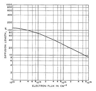
Fig. 8 — Degradation of diffusion length vs electron flux.
