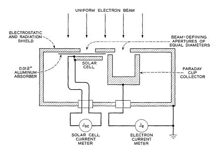
Fig. 6 — Schematic representation of the double-aperture vacuum Faraday cup for measuring  $J_{sc}/J_{e}$ .
