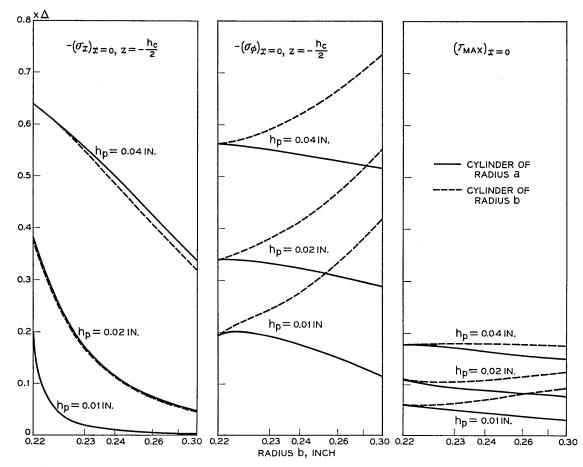
Fig. 6 — Stresses at the junctions of radially unbalanced seals. The values for both cylinders are shown as the radius, b, of the balancing seal is varied.
