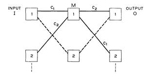
Fig. 4 — Calls  $c_1$  and  $c_2$  over path via  $M_1$ .
