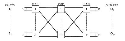
Fig. 1 — Three-stage Clos network N(m,n,r).
