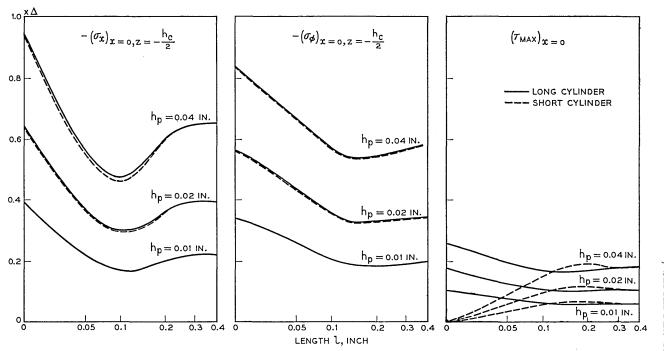
Fig. 8 — Stresses at the junctions of axially unbalanced seals. The values for both cylinders are shown as the length, l, of the intermedate cylinder is varied.
