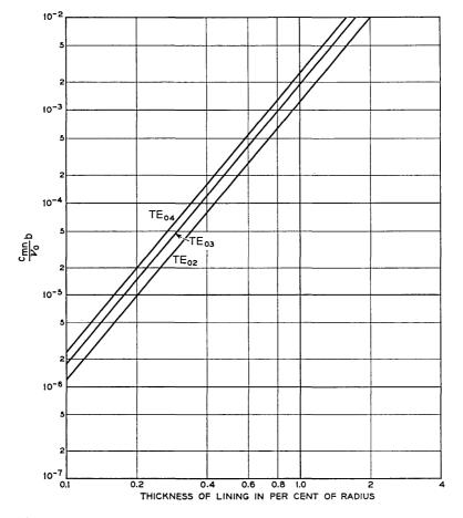
Fig. 10 — Coefficients  $c_{mn}$  of coupling between TE<sub>01</sub> and TE<sub>0n</sub> waves at lining imperfections of circular symmetry.  $b/\lambda = 4.70$ ,  $\epsilon_r = 2.5$ .
