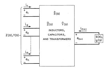
Fig. 3 — Most general structure defining Z(s) and Y(s).
