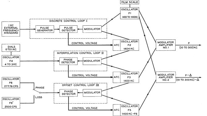
Fig. 6 - Block diagram of standard controlled heterodyne oscillator (SCHO).
