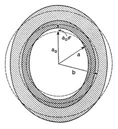
Fig. 14 — Lined waveguide with cross-sectional deformation.
