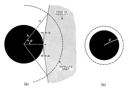
Fig. 4 — Satellite visibility geometry: (a) Plane view of the cone of visibility for a ground station at A.  $\alpha$  is the minimum usable elevation angle. (b) Circle of visibility. A satellite of altitude *H* would be more than  $\alpha$  degrees above the horizon at the ground station whenever it is over this circular region centered on the ground station.
