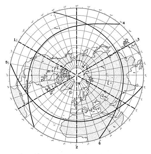
Fig. 15 — Orientation of the orbit planes of the 24-satellite system. The dotted lines are the intersections of the polar planes with the surface of the earth, and the solid lines are the intersections of the  $28^{\circ}$  planes with the earth's surface. The planes are numbered at the ascending nodes of the orbits.
