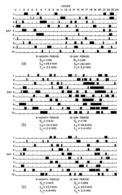
Fig. 23 — London-Johannesburg service: (a) Representative service furnished by the uniformly spaced system shown in Fig. 15. (b) Service during the poorest 10-day period from the 6-month simulation of the bunched system shown in Fig. 20. (c) Service during the period shown in Fig. 23(b) if four satellites in a 28° plane were added to the bunched system.
