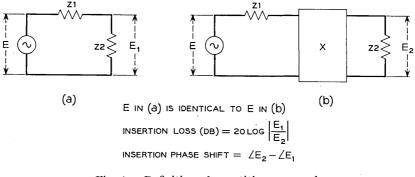
Fig. 1 — Definition of quantities measured.
