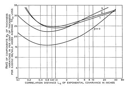
Fig. 12 — TE<sub>01</sub> loss in lined waveguide with random lining imperfections of exponential covariance: 2-inch inside diameter at 55.5 kmc, lining  $\epsilon_r = 2.5$ ,  $\delta = 0.5$  per cent.
