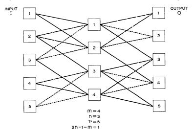
Fig. 6 — Network showing that  $I_1$  and  $O_5$  cannot be connected without moving a call on one of  $I_1$  ,  $O_5$  .
