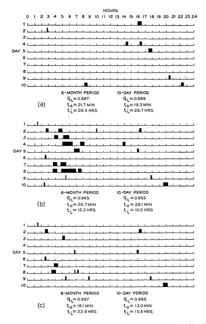
Fig. 22 — Seattle-Hawaii service: (a) Representative service furnished by the uniformly spaced system shown in Fig. 15. (b) Service during the poorest 10-day period from the 6-month simulation of the bunched system shown in Fig. 20. (c) Service during the period shown in Fig. 22(b) if four satellites in a 28° plane were added to the bunched system.
