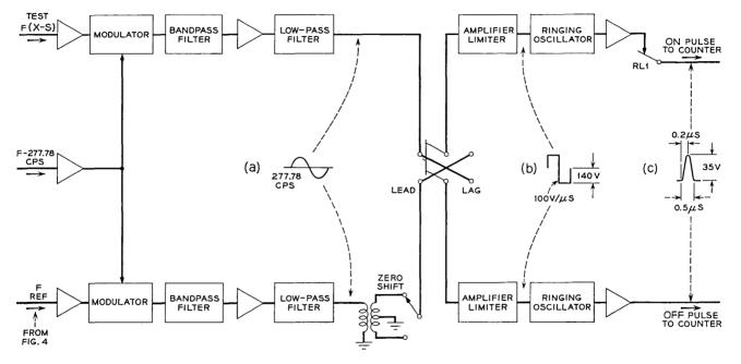
Fig. 7 — Block diagram of phase detector.
