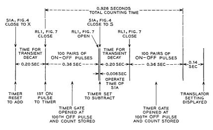
Fig. 8 — Time diagram of phase measurement circuit operation.
