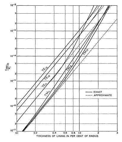
Fig. 6 — Coefficients  $c_{mn}$  of coupling between TE<sub>01</sub> and TE<sub>1n</sub> and TM<sub>1n</sub> waves at lining imperfections of order  $p = 1. b/\lambda = 4.70$ ,  $\epsilon_r = 2.5$ .
