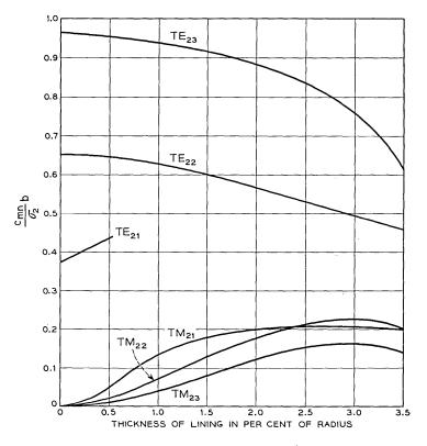
Fig. 16 — Coefficients  $c_{mn}$  of coupling between TE<sub>01</sub> and TE<sub>2n</sub> and TM<sub>2n</sub> in lined waveguide with elliptical deformation.  $b/\lambda = 4.70$ ,  $\epsilon_r = 2.5$ .
