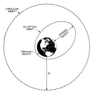
Fig. 1 — Elliptical and circular orbits.
