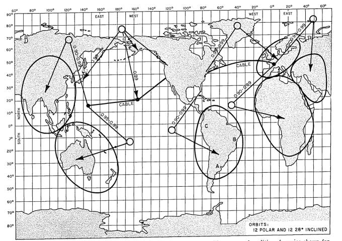
Fig. 18 — A world-wide network which uses satellites and submarine cables. The ranges of qualities of service shown for each region would be provided by 24 satellites in 6000-mile orbits (12 polar and 12  $28^{\circ}$ -inclined).
