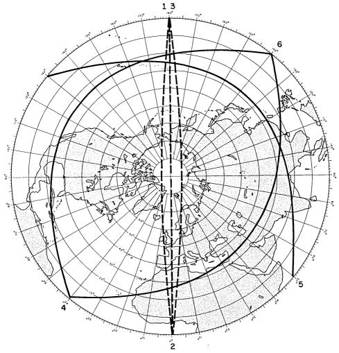
Fig. 20 — Orientation of the orbit planes of the 24-satellite system for a severe case of plane bunching. This bunching would occur after six years if a certain combination of  $5^{\circ}$  errors were made in the inclinations of four of the planes.
