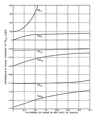
Fig. 2 — Phase constants of TE<sub>1n</sub> and TM<sub>1n</sub> modes in lined waveguide.  $b/\lambda = 4.70$ ,  $\epsilon_r = 2.5$ .
