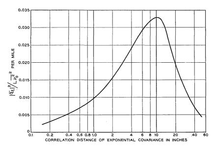
Fig. 13 — TE<sub>01</sub> — pulse distortion in lined waveguide with random imperfections of the lining. Mode conversion causes a reconversion tail of rms amplitude  $\sqrt{|\bar{q}_t|^2}$  to follow the pulse.  $b/\lambda = 4.70$ ,  $\epsilon_r = 2.5$ ,  $\delta = 1$  per cent.
