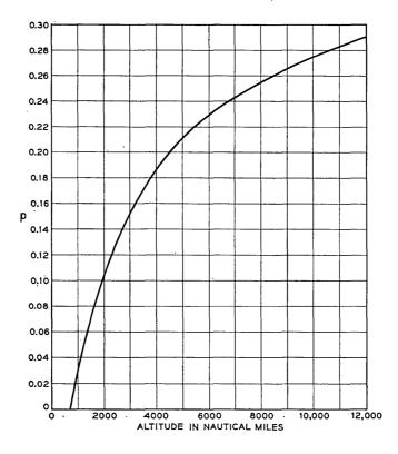
Fig. 6 — Fraction of time (p) a satellite in a circular polar orbit of altitude H is visible to Maine and London.  $\alpha = 7.5^{\circ}$ .
