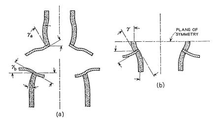
Fig. 5 — Exaggerated picture of deflections produced by discontinuity forces and moments acting at joints.
