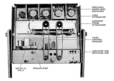
Fig. 9 — Comparison unit, showing the ganged level control.
