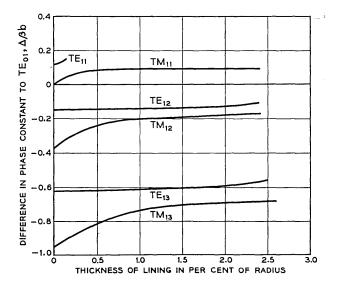
Fig. 5 — Phase constants of TE<sub>1n</sub> and TM<sub>1n</sub> modes in lined waveguide.  $b/\lambda = 7.62$ ,  $\epsilon_r = 2.5$ .
