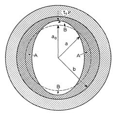
Fig. 1 -Round waveguide with lining of varying thickness.
