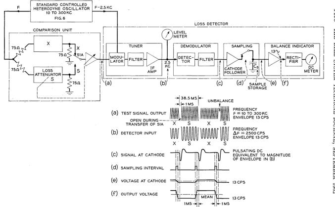
Fig. 3 — Block diagram of loss measurement circuits.
