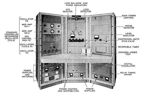
Fig. 5 — The assembled loss and phase measuring set.
