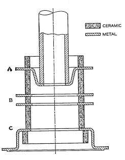
Fig. 1 - A cross-sectional view of a representative ceramic-metal electron tube envelope.
