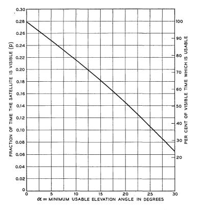
Fig. 7 — The effect of the minimum elevation angle on the usefulness of a satellite in a 6000-mile polar orbit. Ground stations at Maine and London.
