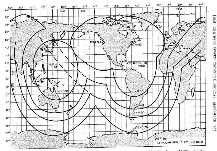
Fig. 16 — Qualities of service from U. S. points for a system of 24 satellites in 6000-mile orbits (12 polar and 12 28°-inclined).
