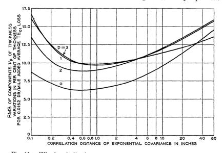
Fig. 11 — TE<sub>01</sub> loss in lined waveguide with random lining imperfections of exponential covariance: 2-inch inside diameter, at 55.5 kmc, lining  $\epsilon_r = 2.5$ ,  $\delta = 1$  per cent.
