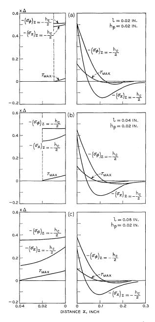
Fig. 9 — Stress distributions showing the effect of varying the length, l, of the intermediate cylinder in an axially unbalanced seal. Note the difference in scale for long (right side) and short (left side) cylinders.
