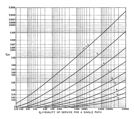
Fig. 9 — Fraction of time  $q_m$  that m or more satellites are visible. In a system with multiple paths between two ground stations  $q_m$  is the quality of service on a path with priority m. The number of satellites needed to furnish  $q_m$  is found by entering Fig. 8 with  $q_1$  and p.
