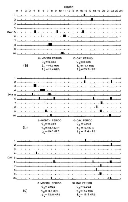
Fig. 21 — Maine-London service: (a) Representative service furnished by the uniformly spaced system shown in Fig. 15. (b) Service during the poorest 10-day period from the 6-month simulation of the bunched system shown in Fig. 20. (c) Service during the period shown in Fig. 21(b) if four satellites in a 28° plane were added to the bunched system.
