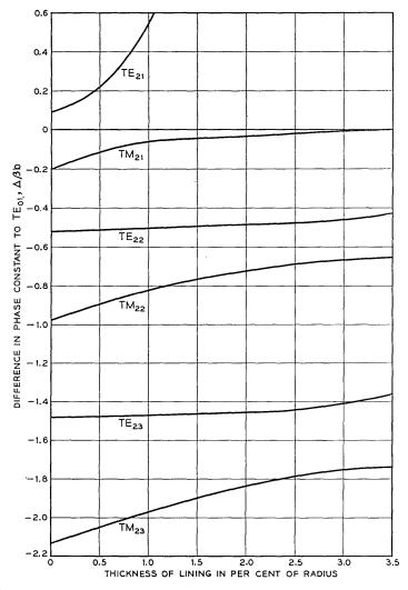
Fig. 3 — Phase constants of TE<sub>2n</sub> and TM<sub>2n</sub> modes in lined waveguide.  $b/\lambda = 4.70$ ,  $\epsilon_r = 2.5$ .
