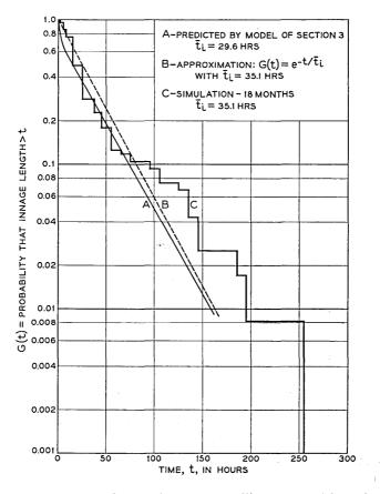
Fig. 1 — Innage length distribution for 18-satellite system with random polar orbits (Maine-Western Europe).
