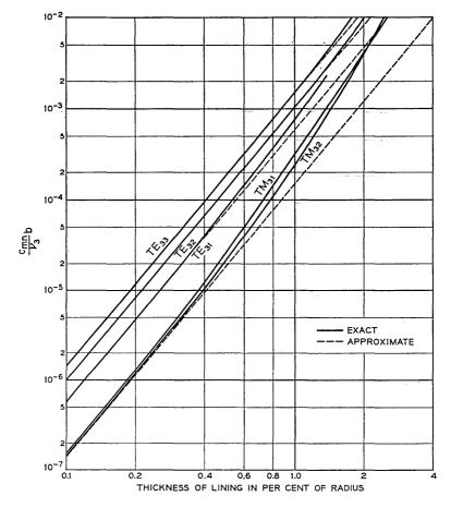
Fig. 8 — Coefficients  $c_{mn}$  of coupling between TE<sub>01</sub> and TE<sub>3n</sub> and TM<sub>3n</sub> waves at lining imperfections of order p = 3.  $b/\lambda = 4.70$ ,  $\epsilon_r = 2.5$ .
