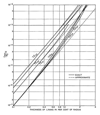
Fig. 7 — Coefficients  $c_{mn}$  of coupling between TE<sub>01</sub> and TE<sub>2n</sub> and TM<sub>2n</sub> waves at lining imperfections of order  $p = 2. b/\lambda = 4.70$ ,  $\epsilon_r = 2.5$ .
