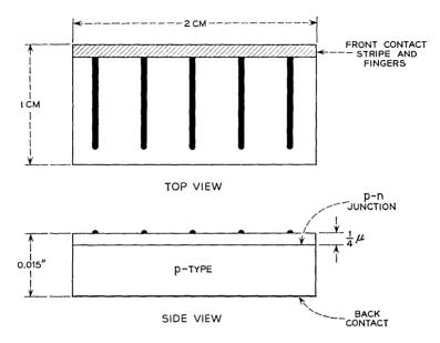
Fig. 1 — Schematic representation of the silicon solar cell.
