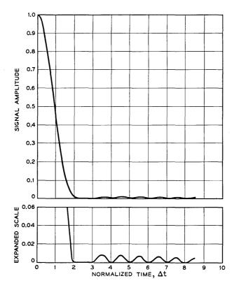
Fig. 26 — Quadratic phase distortion effects, weighted pulse,  $\varphi = 0$ .
