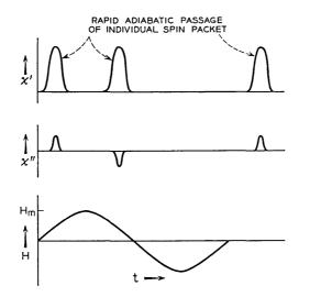
Fig. 27 — Signals from one spin packet, case 5; the spins do not relax between consecutive field modulation cycles, so  $\chi'$  does not change sign, while  $\chi''$ , which is due to nonperfect adiabaticity, changes sign.
