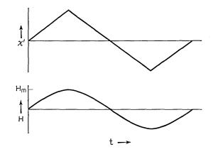
Fig. 34 — Scope trace of signal of case 7: a stationary state is established; the spin packets at the center of the field modulation cycle are burnt out, while those at the extrema yield an adiabatic rapid passage signal.
