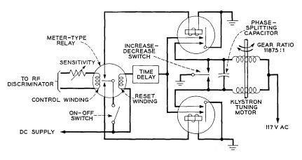
Fig. 14 — Functional schematic of the transmitter AFC circuit.
