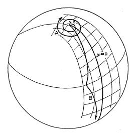
Fig. 10 — Locus of the magnetization vector for almost sudden (A) and almost adiabatic, (B), transitions for infinite relaxation times. (N.P. = North pole;  $\varphi$  = the polar angle.)
