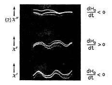
Fig. 39 — Experimental scope traces corresponding to case 8 (compare with Fig. 36): the  $\chi''$  trace is probably a spurious  $\chi'$  signal; the signal here is weak, so the signal-to-noise ratio is not good.
