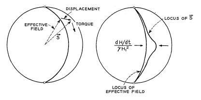
Fig. 50 — The locus of the magnetization vector for an almost adiabatic rapid passage.
