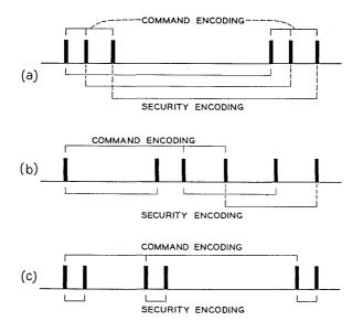
Fig. 3 — Methods for combining security and command codes: (a) short command codes, long security codes: (b) interleaved security and command codes; (c) long command codes, short security codes.
