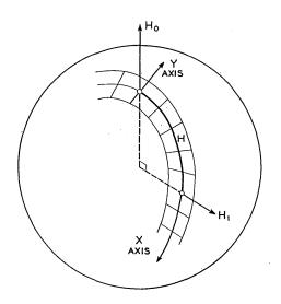
Fig. 47 — Almost-cartesian coordinate net covering a part of a sphere. regions are "narrow" (see Fig. 47). In this coordinate system,
