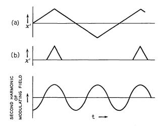
Fig. 44 — Demonstration of the strong harmonic content of "fresh" signals: (a)  $\chi'$  of case 7 (stale); (b)  $\chi'$  of case 8 (fresh). Note that the "stale" signal possesses only odd harmonics of the magnetic field modulation frequency, while the "fresh" signal possesses a strong second harmonic component.
