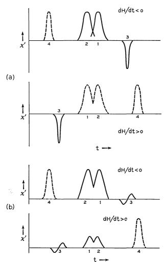
Fig. 7 — (a) The  $\chi'$  signal expected from the system with energy levels shown in Fig. 5, when *all* transitions (including those of the forbidden lines), are adiabatic; line 4 is assumed to be *strictly* forbidden, while line 3 is not; there is *no* simple symmetry under  $dH/dt \rightarrow -dH/dt$ . (b) The  $\chi'$  signal from the system with the energy level diagram shown in Fig. 5, when line 3 is *not* passed adiabatically.
