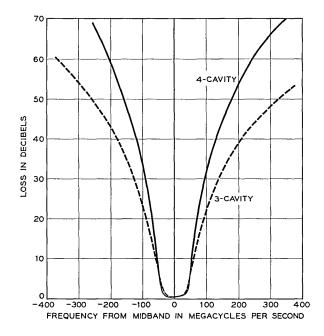
Fig. 11 — Representative transmission characteristics of the  ${\tt RF}$  receiver bandpass filters.
