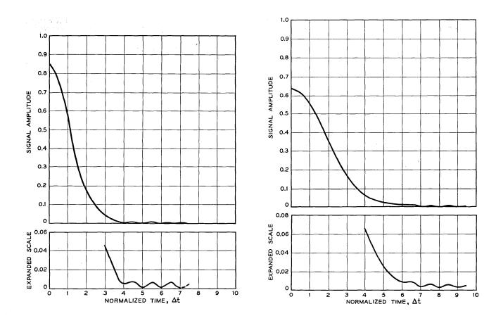
Fig. 31 — Quadratic phase distortion effects, weighted pulse,  $\varphi = \pi$ .
