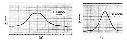
Fig. 24 — (a)  $\chi'$  for mixture of cases 1 and 2; with P.S.D., 0° phase shift between modulating field and reference voltage [compare with Fig. 19(b)]. (b) Same as (a), but  $\chi'$  signal 90° out-of-phase with modulating field.
