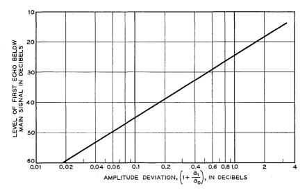
Fig. 12 — Amplitude of echo with amplitude distortion.
