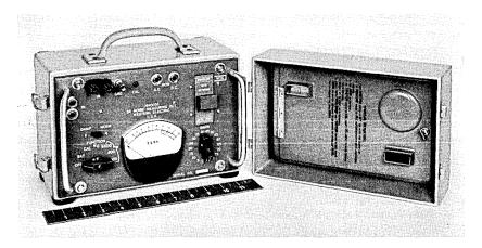
Fig. 6 — The 3A Noise Measuring Set.
