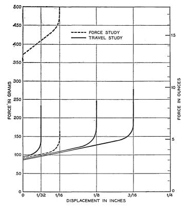
Fig. 6 — The idealized force-displacement curves of the two conditions compared in the study of forces, and the three conditions compared in the study of button travel. These curves are based on essentially static measurements of the universal pushbutton switches.
