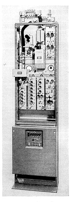
Fig. 34 — TJ transmitter-receiver bay.
