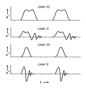
Fig. 54 — Expected  $\chi'$  and  $\chi''$  scope traces of case 11; wiggles are observed when  $\gamma H_1 \langle \langle \langle \omega_m H_m \rangle$ , and  $\omega_m T_2$  is not very small compared with unity.
