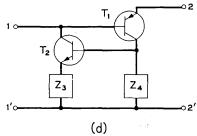
Fig. 14 — Transistor realizations of the converter.
