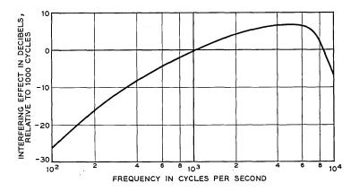
Fig. 3 - Response vs. frequency of standard 5-kc program circuit weighting.
