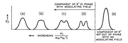
Fig. 19 — Expected recorder traces for rapid (adiabatic or nonadiabatic) passage, with a field modulation period long compared with, or of the same order, as  $T_1$ : (a) large  $H_1$ , small  $H_m$ ; (b) and (c) intermediate values of  $H_1$ ,  $H_m$ ; (d) Small  $H_1$ , large  $H_m$ . (These four are the component of  $\chi'_f$  in-phase with the field modulation.) (e) Component of  $\chi'_f$  90° out-of-phase with the field modulation.
