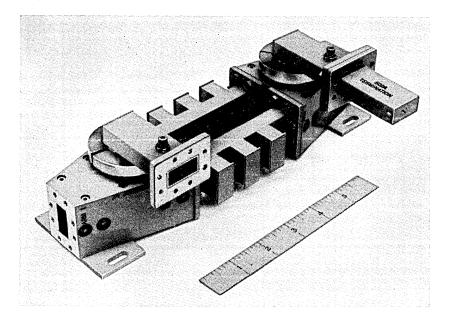
Fig. 4 — Channel separation-combining network.
