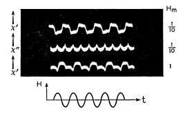
Fig. 16 — Experimental scope traces for case 2. Top trace,  $\chi'$  signal, almost ideal case "2"; center trace,  $\chi''$  signal due to slow passage near the extrema of the modulation cycle; bottom trace,  $\chi'$  signal, when the adiabatic condition is slightly violated.
