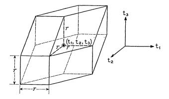
Fig. 7 — Polytope containing all decodable messages for n = 4.
