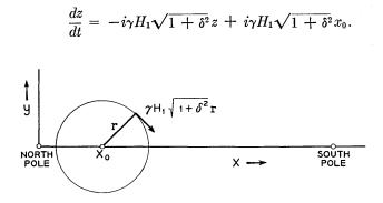
Fig. 48 — Diagram illustrating the differential equation satisfied (approximately) by the magnetization vector.
