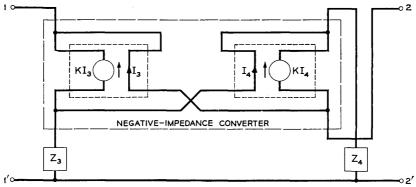
Fig. 4 — Alternate idealized realization of the converter.
