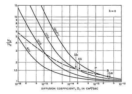
Fig. 4 — Calculated ratios of impurity surface concentration to body concentration  $(N_s/N_0)$  produced by parabolic oxidation of silicon with zero segregation coefficient. The arrows indicate the surface concentrations predicted for the impurities indicated at 1100°C. The dashed line corresponds to the surface concentrations predicted for antimony at various temperatures.
