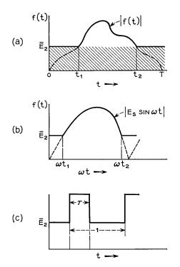
Fig. 8 — (a) Voltage across  $R_1$  and  $R_2$  with f(t) into the detector; (b) sine wave into the detector; (c) rectangular wave into the detector.
