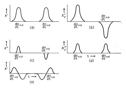
Fig. 4 — Some typical traces observed when the system does not relax between  $\chi''$ , no P.S.D. (rapid, not perfectly adiabatic, passage); (d)  $\chi''$ , with P.S.D.; (e)  $\chi''$ , with P.S.D., very rapid sweep. Again, notice the symmetry properties which are different from those occurring when the system relaxes between sweeps.
