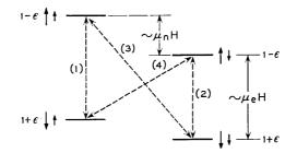
Fig. 5 — Energy-level diagram of an electron-nucleus system in a magnetic field (the nuclear spin is supposed to be  $\frac{1}{2}$ ). Lines (1) and (2) are "allowed," while lines (3), (4) are "forbidden," but not strictly.
