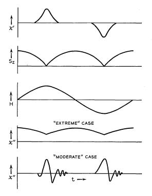
Fig. 40 — Expected scope traces of case 10:  $\chi'$  depends critically upon variations of  $S_z$ ; these may be due to "burnout," or the derivative of the line shape; here, variations due to burnout are postulated.
