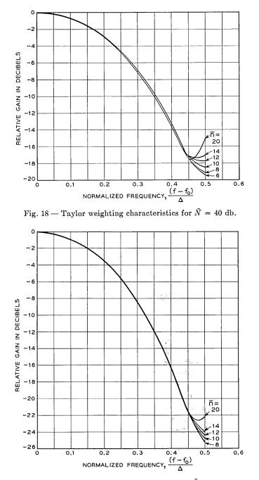
Fig. 19 — Taylor weighting characteristics for  $\bar{N}$  = 47.5 db.
