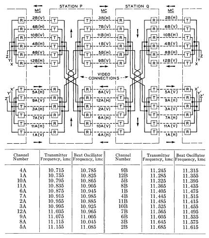
Fig. 2 — TJ frequency assignment plan.
