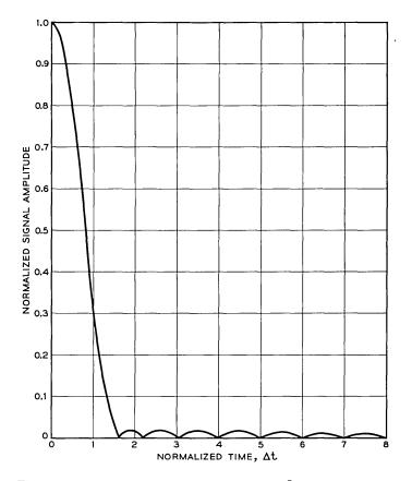
Fig. 21 — Taylor weighting pulse envelope for  $\bar{N} = 34$  db,  $\bar{n} = 5$ .
