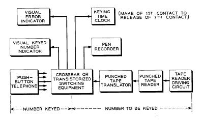
Fig. 2 — Schematic drawing of equipment for measuring and recording keying performance.
