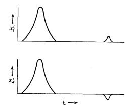
Fig. 37 — Expected recorder traces of case 8 signals: the line is burnt while sweeping through, consecutive sweeps yield weaker lines; their sign depends upon  $T_1$ , the time between consecutive sweeps, and the extent to which the line is "burnt out."
