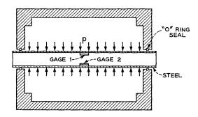
Fig. 2 — Experimental arrangement for calibration.
