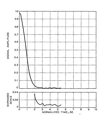
Fig. 29 — Quadratic phase distortion effects, weighted pulse,  $\varphi = \pi/4$ .
