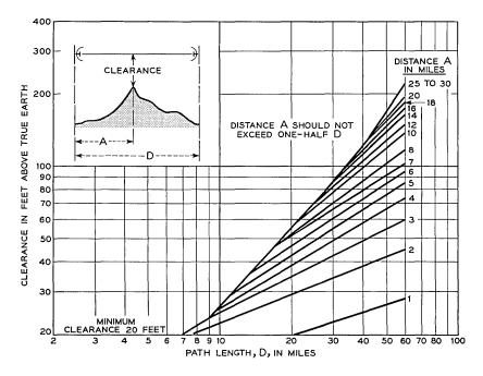
Fig. 42 — TJ radio path clearance requirements.
