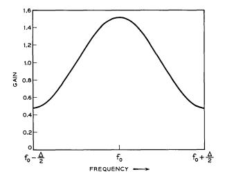
Fig. 14 - Network amplitude response.
