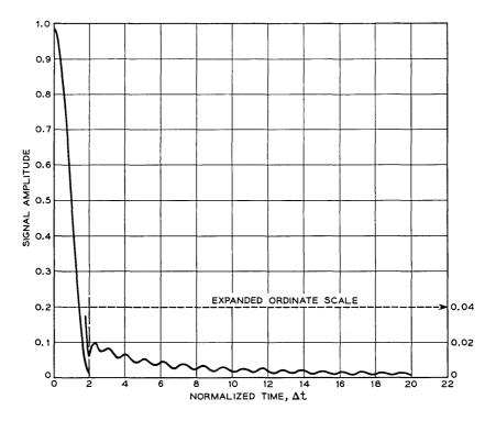
Fig. 37 — Weighting effects on Doppler-shifted signals.
