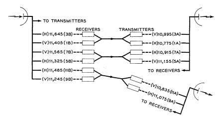
Fig. 43 — Typical frequency assignments at TJ branching point.
