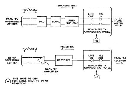
Fig. 33 — Video terminal connecting circuit.
