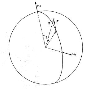
Fig. 46 - Position of magnetization vector in space.
