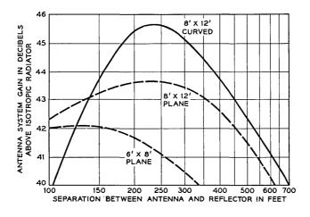
Fig. 30 — Gain of periscopic antenna system.
