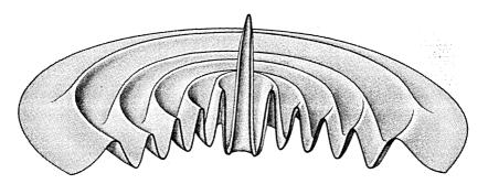
Fig. 6 — Cut-away of three-dimensional projected view of complete ambiguity amplitude  $\rho(t,\Omega)$  when n = 10.
