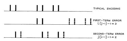
Fig. 2 — First- and second-term error for 2 | 3 code.
