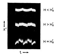
Fig.  $21 - \chi'$  scope traces of rapid, nonadiabatic passage of a line, when  $T_1$  is very short compared with the field modulation cycle, at the center of the line (bottom trace), and on both sides of it (top and center traces).
