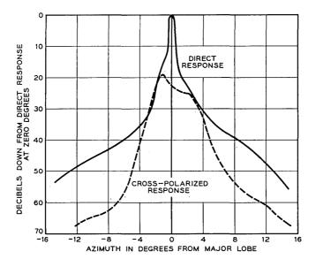
Fig. 29 —  $\pm 15^{\circ}$  radiation patten of the TJ 10-foot antenna.
