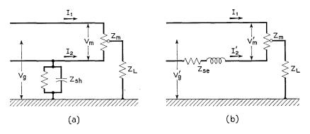
Fig. 10 — Equivalent circuit representations for (a) shunt and (b) series unbalance. For shunt unbalance, 20  $\log_{10}(V_m/V_g) = 20 \log_{10}(Z_m/4Z_{sh}) =$  balance ratio in decibels; for series unbalance, 20  $\log_{10}(V'_m/V'_g) = 20 \log_{10}(Z_{se}/4Z_L) =$  balance ratio in decibels.
