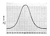
Fig. 25 — The component of  $\chi'_{f}$  in-phase with the modulating field, with higher microwave power than that used to obtain Fig. 24(a); the higher power yields a "cleaner" trace [compare with Fig. 19(a)].
