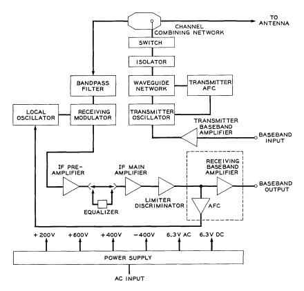
Fig. 3 — Block schematic of the TJ transmitter-receiver bay.
