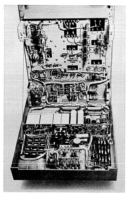
Fig. 37 — Internal view of TJ radio power supply.
