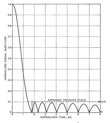
Fig. 23 — Taylor weighting pulse envelope for  $\bar{N} = 40$  db,  $\bar{n} = 6$ .
