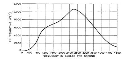
Fig. 8 — Proposed new TIF weighting curve, W(f) = Kw(f)M(f), where K is such that W(1000 cycles) = 5000;  $w(f) = 10^{db(f)/10}$  is the C-message weighting and M(f) = f/1000 to approximate the coupling distortion between power and telephone circuits.
