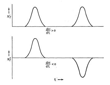
Fig. 55 — Expected recorder traces of case 11 (system relaxes between sweeps); the true line shape may be observed, sometimes even if  $H_m$  is not small compared with  $\Delta H$  (the width of the nonburnt region must then be small). Compare with Figs. 42(a) and (b).
