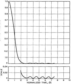
Fig. 28 — Quadratic phase distortion effects, weighted pulse,  $\varphi = \pi/6$ .
