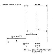
Fig. 3 — Coordinates and notations used in the analysis of the impurity redistribution phenomenon.
