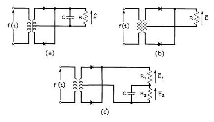
Fig. 7 — (a) Peak detection; (b) average detection; (c) "quasi-rms" detection.
