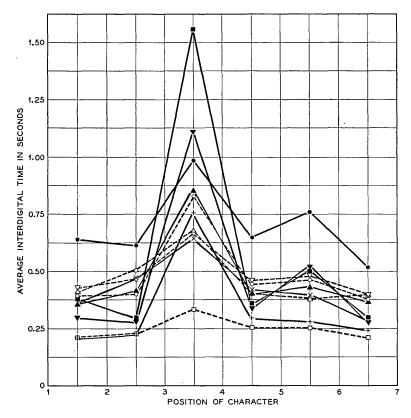
Fig. 8 — Average interdigital intervals for individual subjects keying sevencharacter numbers. The interdigital intervals were measured from the breaking of one electrical contact to the making of the next contact. (These results were obtained for all-numeral dialing; data for letter-and-numeral dialing are similar but less definitive than those shown in the figure.)
