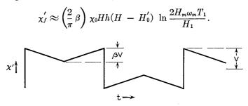
Fig. 20. — An idealized  $\chi'$  scope trace of case 3, used to estimate the amplitude of the signal.
