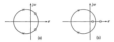
Fig. 11 — Construction of the extremum points of  $Z(\sigma)$ .
