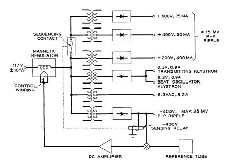
Fig. 16 — Power supply block schematic.
