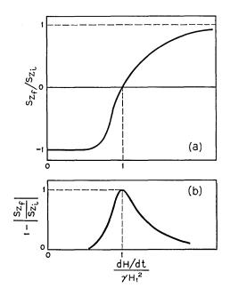
Fig. 11 — Loss of magnetization per passage due to nonadiabaticity (or nonsuddeness), qualitative only. In an adiabatic transition,  $S_z \rightarrow -S_z$ ; in a sudden transition,  $S_z \rightarrow S_z$ ; in both cases, there is no loss of  $|S_z|$ . In an intermediate transition, there is a loss in  $|S_z|$ ;  $S_{z_1}$  and  $S_{z_f}$  are the initial and final values of  $S_z$ , respectively.
