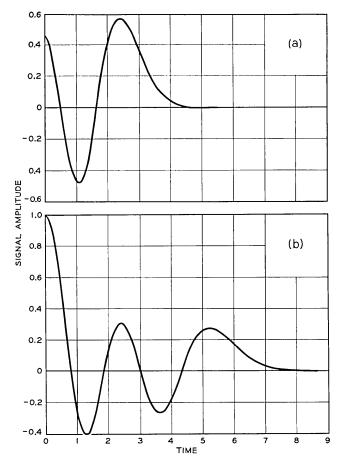
Fig. 3 — Envelope of (a) transmitted signal and (b) matched-filter response when n = 4.
