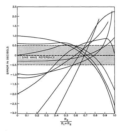
Fig. 11 — "Quasi-rms" detector error for several functions.
