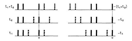
Fig. 4 - Six false security codes for a three-pulse code.
