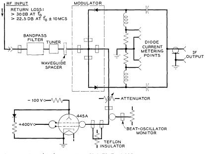
OVER-ALL LOSS (MAX) RF INPUT TO IF OUTPUT = 9.0 DB MAXIMUM NF AT TUNER INPUT = 15.0 DB
