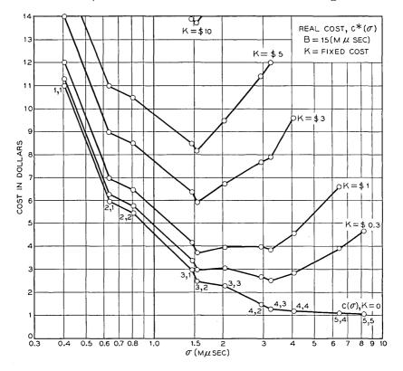
Fig. 4 — Real cost per section of a ten-section, one-microsecond, lumped-constant delay line as a function of the standard deviation of the delay per section and for various values of the fixed cost K. The delay tolerances are  $\pm B = \pm 15$  mµsec.
