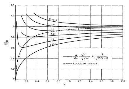
Fig. 4 — Reduction of attenuation in a magnetically loaded line in terms of the normalized dimension parameter v and the normalized magnetic loss parameter k. For each fixed k, the value of v yielding minimum attenuation is shown.
