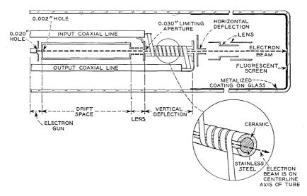
Fig. 5 — Cross section of broadband oscilloscope tube — Model IV.
