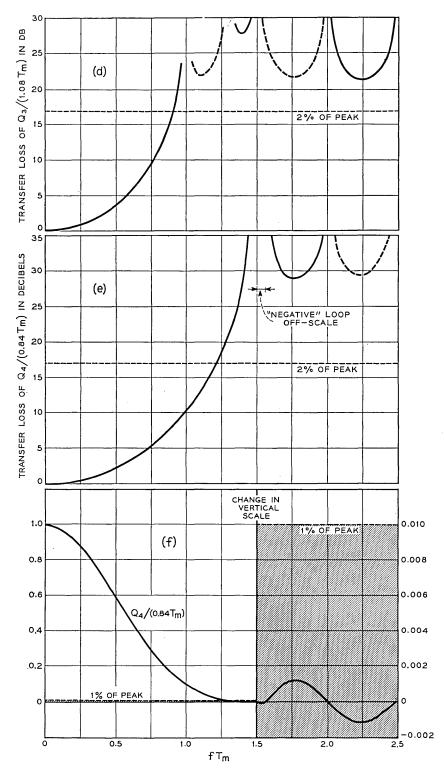
Fig. 15(d)(e)(f) — Transfer loss of spectral windows  $Q_3$ ,  $Q_4$  in db and power transfer ratio of spectral window  $Q_4$ .
