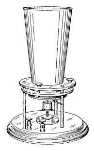
Fig. 4 — Liquid transmitter used by Bell on March 10, 1876.
