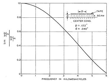
Fig. 3 — Transit time versus frequency for a beam in the presence of parallel plates.
