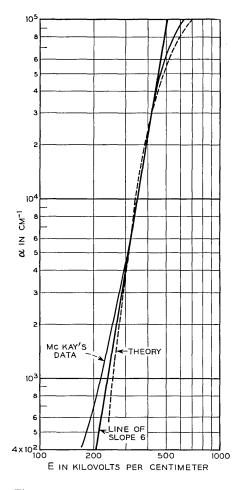
Fig. 3 — Ionization rate vs electric field.
