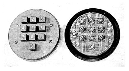
Fig. 8 — Front and rear views of a pushbutton crosspoint switch.
