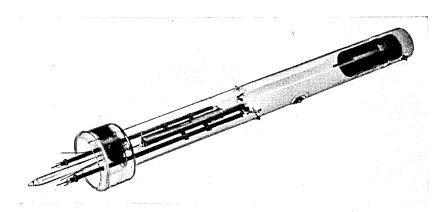
Fig. 1 — Photograph of broadband oscilloscope tube — Model III.
