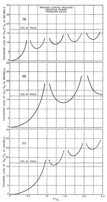
Fig. 15(a)(b)(c) — Transfer loss of spectral windows  $Q_0$ ,  $Q_1$ ,  $Q_2$  in db.
