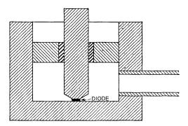
Fig. 2 — Diode mounted in microwave cavity.
