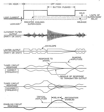
Fig. 12 — Waveforms illustrating operations at a pulse receiver in pushbutton calling.
