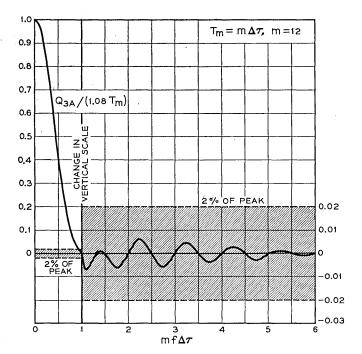
Fig. 19 — Aliased spectral window  $Q_{3A}$  for m = 12.
