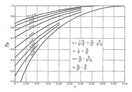
Fig. 5 — Maximum reduction of attenuation in a magnetically loaded line in terms of the magnetic loss parameter k and the dielectric loss parameter m of the magnetic material.
