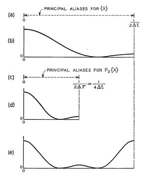
Fig. 20 — Transmission curves for a simple example of smoothing and decimation.
