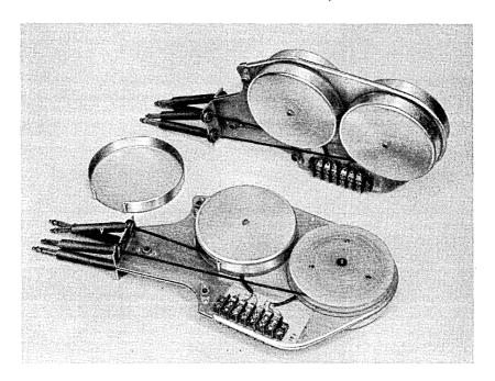
Fig. 10 — Cord reel assembly showing the switchboard cords in the retracted position. This assembly provides access to two cord circuits.
