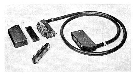
Fig. 11 — Patching cable assembly showing the method of terminating the cable on the 52-pin connectors. The connector in the lower left-hand corner is the mating connector which mounts in each unit and to which the patching cable connects.
