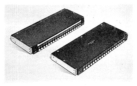
Fig. 13 — Trunk and line packs each containing twenty jack and lamp appearances. The pack on the left is a trunk pack, that on the right a line pack. Connection is made via two 52-pin connectors not shown here but mounted on the rear of each pack.
