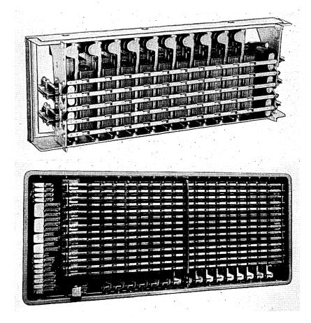
Fig. 17 — Top: Crossbar switch, present date design by the Swedish Telecommunications Administration. (By courtesy of Swedish Board of Telecommunications.) Bottom: "Pentaconta" crossbar (France). (By courtesy of International Telephone and Telegraph Co.)
