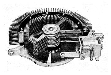
Fig. 16 — A rotary selector (Belgium). (By courtesy of International Telephone and Telegraph Co.)
