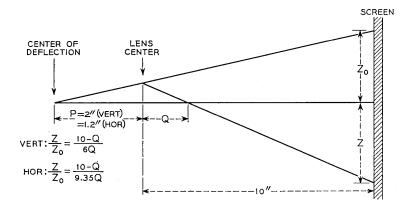
Fig. 6 — Method for determining magnification.
