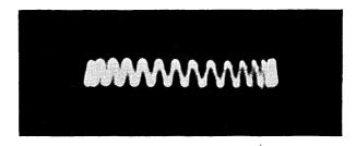
Fig. 10 — Photograph of 800 mc sine wave.
