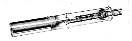
Fig. 4 — Photograph of broadband oscilloscope tube — Model IV.
