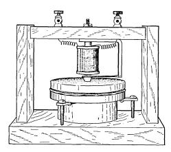
Fig. 2 — "Gallows frame" transmitter of Alexander Graham Bell, June 3, 1875.
