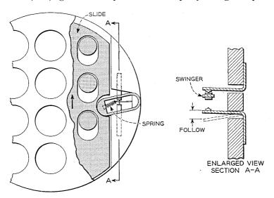
Fig. 9 — Switch detail, showing the slide plate and follow arrangement for toggle contact K1.
