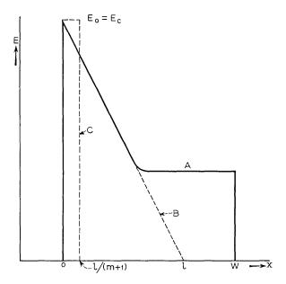
Fig. 4 — Field distribution at breakdown.
