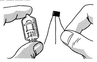
Fig. 21 — Comparative sizes of vacuum tube (left) and transistor.
