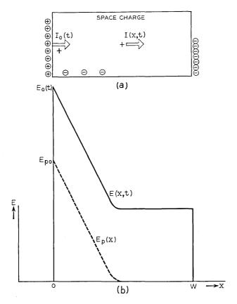
Fig. 7 — Current (a) and field (b) in the space-charge region.
