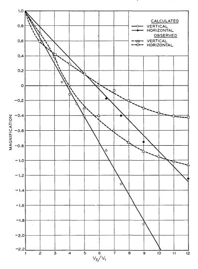
Fig. 7 — Magnification versus  $V_2/V_1$ , for cross-over lens with non-aluminized screen.
