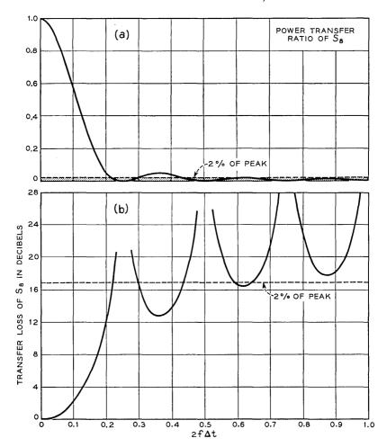
Fig. 21 — Transmission curves for  $S_8$ .
