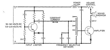
Fig. 3 — Simplified circuit schematic of the tone ringer.
