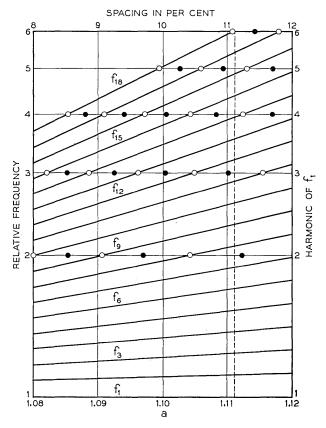
Fig. 2 — Interlacing of harmonics in geometric series of frequencies.
