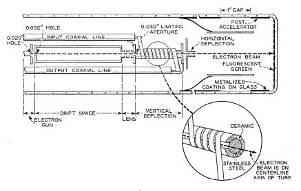
Fig. 2 — Cross section of broadband oscilloscope tube — Model III.
