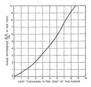
Fig. 2(a) — Change in phase constant of the TM<sub>11</sub> wave in the dielectric-coated waveguide.  $\epsilon = 2.5$ ;  $a/\lambda = 1.03$ .
