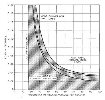
Fig. 5 – 90° normal mode bend of  $\frac{7}{8}$ -inch I.D. copper pipe with a dielectric coat 0.0075 inch thick ( $\epsilon' = 2.5$ ,  $\epsilon'' = 2.5 \times 10^{-3}$ ), designed for optimum performance at  $\lambda = 5.4$  mm (55.5 kmc).
