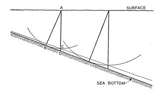
Fig. 1 — Slope correction of echo soundings.
