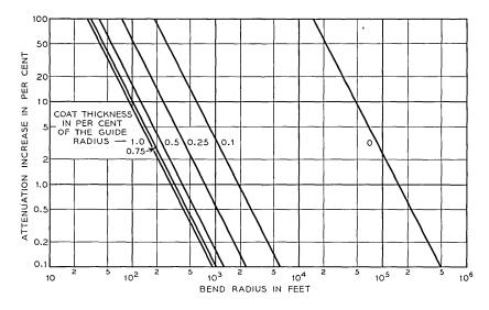
Fig. 4 — Increase in TE<sub>01</sub> attenuation of a dielectric-coated guide in a uniform bend. 2a = 2 inches;  $\epsilon = 2.5$ ;  $\lambda = 5.4$  mm.
