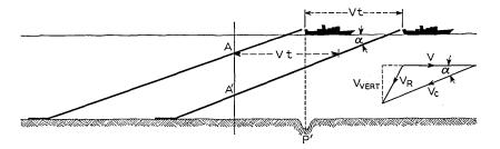
Fig. 7 - Illustration of vertical cable sinking rates.
