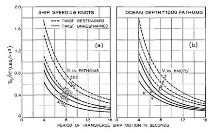
Fig. 34 - Variation of the transverse ship motion tension of cable No. 2 with the period of ship motion.
