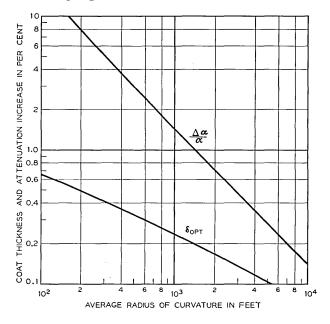
Fig. 7 — Optimum coat thickness and increase in TE<sub>01</sub> attenuation of a dielectric-coated guide with random deviations from straightness. 2a = 2 inches;  $\lambda = 5.4$  mm;  $\epsilon = 2.5$ .
