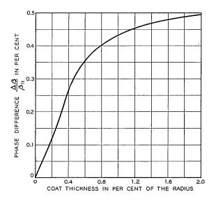
Fig. 2(c) — Change in phase constant of the TM<sub>11</sub> wave in the dielectric-coated waveguide.  $\epsilon = 2.5$ ;  $a/\lambda = 4.70$ .
