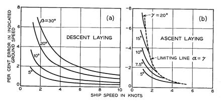
Fig. 25 — Error during descent and ascent laying of 12-gauge piano wire.
