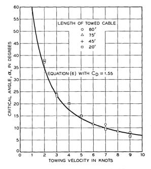
Fig. 3 — Experimental and theoretical variation of critical angle with towing velocity for cable No. 2.
