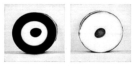
Fig. 14 — Cross-section of Poly(Vinyl Chloride) rod showing sulfiding due to sulfate-reducing marine bacteria. Bottom end was in sediment — top in water. Exposed at Daytona Beach for two years. Original magnification 1.6X.
