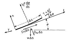
Fig. 9 — Diagram of forces acting on a cable element.
