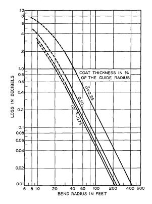
Fig. 3 — Maximum conversion loss of the TE<sub>01</sub> wave in a uniform bend of the dielectric-coated waveguide. 2a = 2 inches;  $\lambda = 5.4$  mm;  $\epsilon = 2.5$ .
