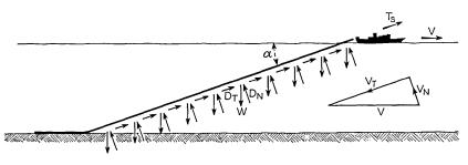
Fig. 1 -Forces acting on a cable in normal laying.
