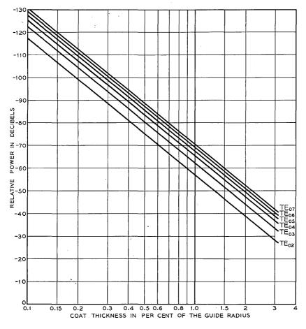
Fig. 8 — Higher circular electric waves at a transition from plain waveguide to the dielectric-coated guide.  $\epsilon = 2.5$ ;  $a/\lambda = 4.70$ .
