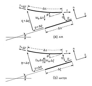
Fig. 33 - Diagram of forces acting on a cable element in air and in water.
