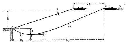
Fig. 35 — Coordinates for the analysis of tension rise when a cable is completely suspended.
