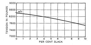
Fig. 23 — Variation of shipboard tension with per cent slack for laying cable No. 2 at a ship speed of 6-knots in a depth of two thousand fathoms.
