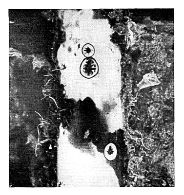
Fig. 13 — Sulfiding of Poly(Vinyl Chloride) plastic test rod beneath barnacles. The black, circular border and center area represent sulfiding at points of exceptionally close contact. Original magnification 2X. Photo by J. B. DeCoste.
