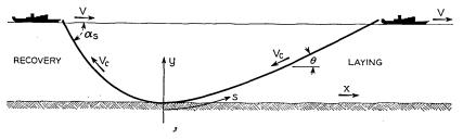
Fig. 8 — Definition of coordinates for the two-dimensional stationary model.
