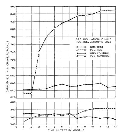
Fig. 6 — Capacitance changes resulting from exposure of GR-S (51-92) and Poly (Vinyl Chloride) (BTL 172-54) insulated conductors in sea water and sediment.
