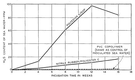
Fig. 4 — Examples of  $H_2S$  production by marine bacteria in anaerobic sea water test with Poly(Vinyl Chloride) plastics as carbon source.
