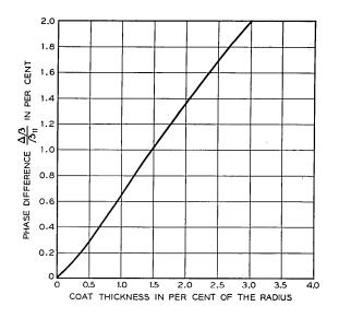
Fig. 2(b) — Change in phase constant of the TM<sub>11</sub> wave in the dielectric-coated waveguide.  $\epsilon = 2.5$ ;  $a/\lambda = 2.06$ .
