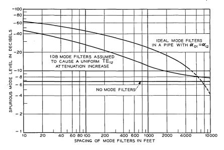
Fig. 3 — Spurious mode level of TE<sub>01</sub>-TE<sub>12</sub> coupling in serpentine bends with mode filters; 2-inch I.D.  $2\frac{3}{8}$ -inch O.D.,  $\lambda = 5.4$  mm. Serpentine bends are caused by equally spaced supports and the elasticity of the copper pipe. The supporting distance is a multiple of the beat-wavelength between TE<sub>01</sub> and TE<sub>12</sub>.
