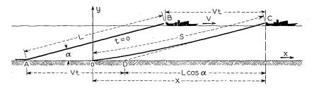
Fig. 11 - Cable geometry at a time t after the onset of negative slack.
