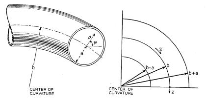
Fig. 1 -Coordinates used in circular bend in circular waveguide.
