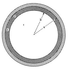
FIG. 1 — The dielectric-coated waveguide;  $\rho = b/a$ ,  $\delta = 1 - \rho = (a - b)/a$ .
