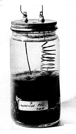
Fig. 5 — General setup of conductor test showing a coil half in sediment and half in sea water.
