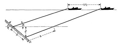
Fig. 20 — Kinematics of straight-line descent laying.
