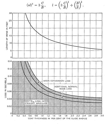
Fig. 4 — 90° normal mode bend of  $\frac{7}{5}$ -inch I.D. copper pipe with a dielectric coat of  $\epsilon' = 2.5$ ,  $\epsilon'' = 2.5 \times 10^{-3}$ . Optimum design for 5.4-mm wavelength.
