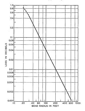
Fig. 6 — Bend conversion loss in a dielectric-coated guide of optimum design according to equation (28). 2a = 2 inches;  $\delta = 1.25\%$ ;  $\epsilon = 2.5$ ;  $\lambda = 5.4$  mm.
