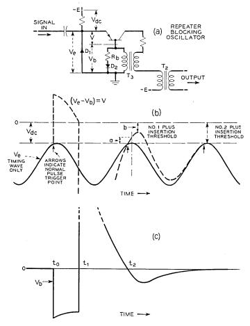
Fig. 10 — (a) Circuit diagram of blocking oscillator showing various components of the effective bias. (b) The effective bias as a function of time. (c) Inhibiting voltage  $V_b$  produced by a regenerated pulse.
