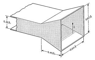
Fig. 6 - Feed horn dimensions.
