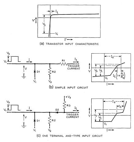
Fig. 7 — Input trigger circuits.
