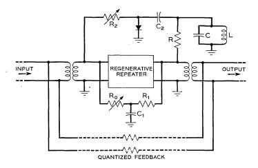
Fig. 4 — Method for maintaining the dc values of timing wave.
