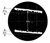
Fig. 3 — Picture of field effect-photoconductivity pattern, as observed on oscilloscope. Dark curve at the bottom.
