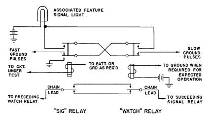
Fig. 9 — Chain circuit showing watching relay function.
