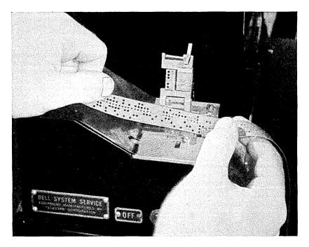
Fig. 15 — Perforated tape being inserted in reader.
