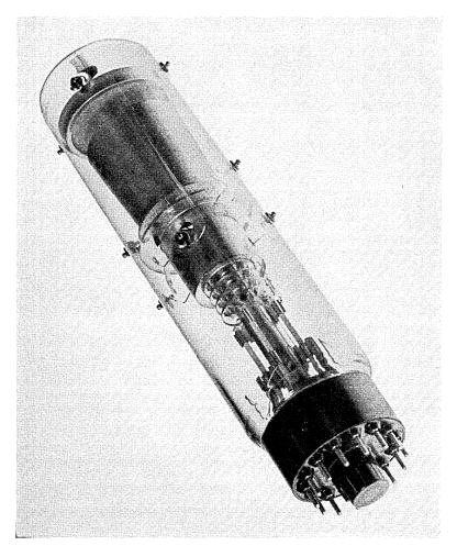
Fig. 19 — Electrostatic storage tube.
