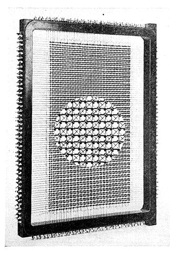
Fig. 18 — Magnetic core array (Courtesy of IBM).
