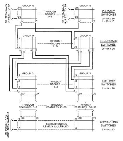
Fig. 12 - Switching plan.
