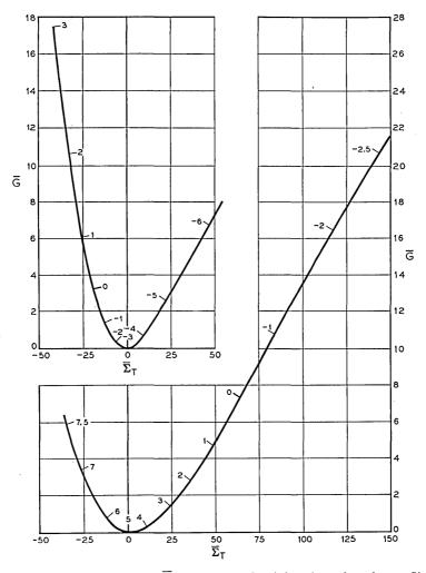
Fig. 5 — Curves showing  $\Delta \overline{G}$  (surface conductivity, in units of  $e\mu_p n_i \mathcal{L}$ ) and  $\Sigma$  surface charge, in units of  $en_i \mathcal{L}$ ) for the 22.6 ohm-cm sample (upper curve) and for the 8.1 ohm-cm sample (lower curve). Values of Y, deduced from the surface conductivity, are indicated on the curves.
