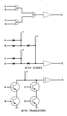
Fig. 26 — A logic function with diodes or transistors.
