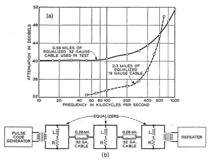
Fig. 5(a) — Equalized characteristics of 19 and 32 gauge line.
