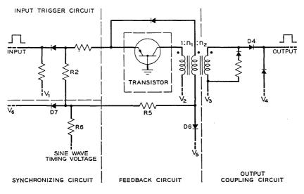
Fig. 11 — Shunt connection of output and feedback.
