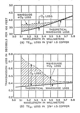
Fig. 7 —  $TE_{01}$  transmission losses.
