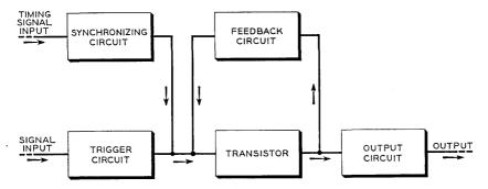
Fig. 2 — Regenerative amplifier block diagram.
