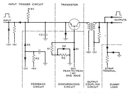
Fig. 4 — Negative resistance feedback amplifier.
