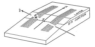
Fig. 3 — Schematic view of a scribed *p-n* junction. <sup>6</sup> V. A. Johnson and K. Lark-Horowitz, Phys. Rev., **69**, p. 259, 1946.
