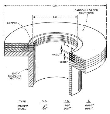
Fig. 9 - Structure of spaced-disk mode filter.
