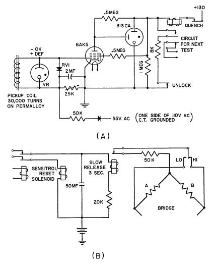
Fig. 7 — Circuits used in relay coil test set. (a), direction of winding, simplified schematic; (b) anti-stall, simplified schematic.
