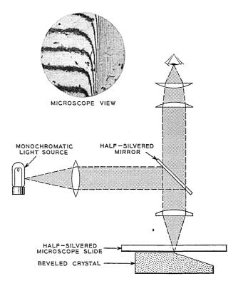
Fig. 5 — Diagrammatic view of the light path in the interferometer.
