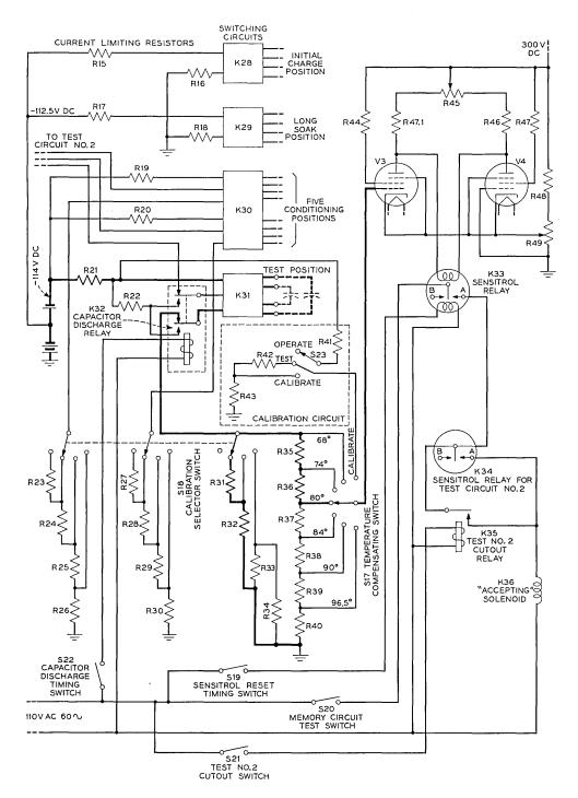
Fig. 12 — Simplified schematic of insulation resistance test circuits. 1196
