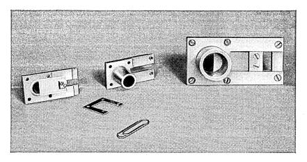
Fig. 5 - Structure of waveguide switch.
