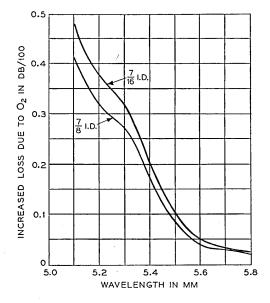
Fig. 6 — TE<sub>01</sub> transmission loss in waveguides due to oxygen absorption. • A. B. Crawford and D. C. Hogg, Measurement of Atmospheric Attenuation at Millimeter Wavelengths, B.S.T.J., **35**, pp. 907-917, July, 1956.
