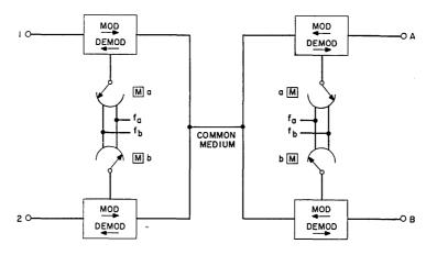
Fig. 7(b) — Frequency division switching.
