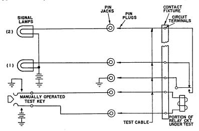
Fig. 2 — Simplified circuit sketch for manual test operation.
