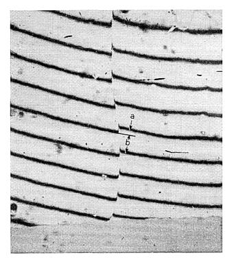
Fig. 10 — Evaluation of the interference fringe pattern of a shallow step in a surface.
