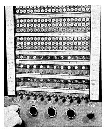
Fig. 10 — Lower portion of lamp display panel.
