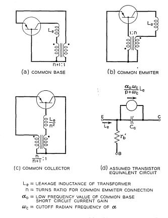
Fig. 6 — Transformer coupled blocking oscillator circuits.
