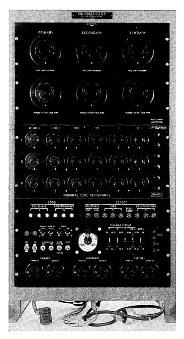
Fig. 5 — Relay coil test set control panel. \$\$1142\$
