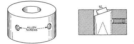
Fig. 1 - Jig for lapping a bevel.
