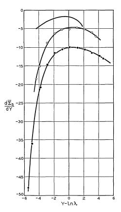
Fig. 6 — Differential charge in fast states versus surface potential. The graphs show  $(\partial \Sigma_s / \partial Y)$  plotted against  $Y - \ln \lambda$ . Dots: p-type; circles: n-type. A typical result of Brown and Montgomery, using 28 ohm-cm p-type germanium, is also shown.
