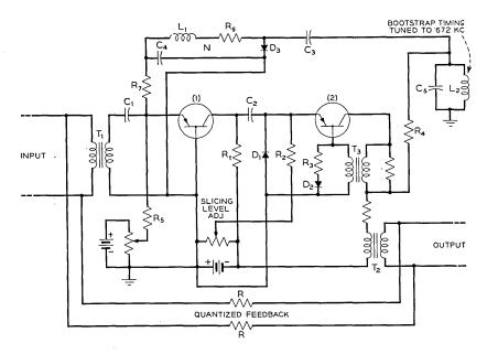
Fig. 3 — Circuit diagram of the regenerative repeater.
