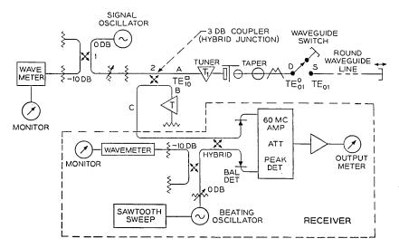
Fig. 3 — Schematic of measuring equipment.
