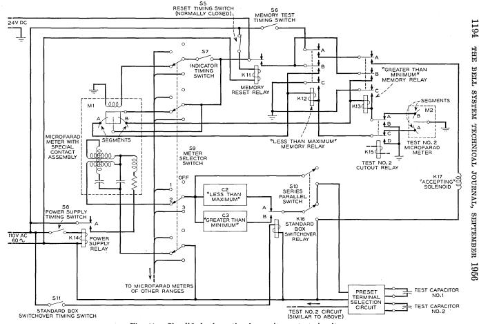
Fig. 11 - Simplified schematic of capacitance test circuits.
