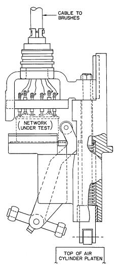
Fig. 3 — Test fixture, loaded.
