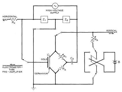
Fig. 2 — Electrical circuit.
