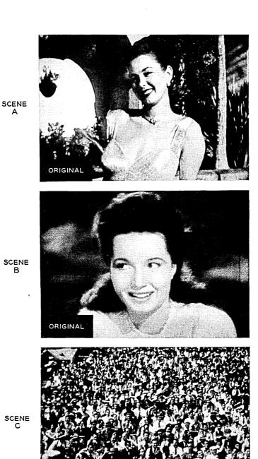
Fig. 14—Three pictures as photographed from the face of a kinescope. Scene "A" is a picture of average complexity. Scene "B" is a simple, rather soft picture. Scene "C" is a complex, highly detailed picture. Roughly, these pictures represent the gamut of pictures normally expected to be transmitted.
