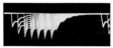
Fig. 23. Output of Shannon-Rack decoder for a signal giving 100% modulation.
