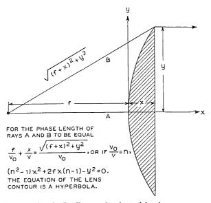
Fig. 17—Profile equation for a delay lens,
