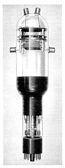
Fig. 4-Experimental seven-digit coding tube.
