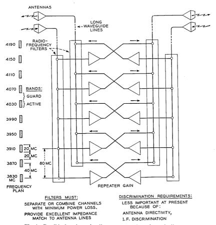
Fig. 1—Possible five-channel radio repeater station schematic diagram.
