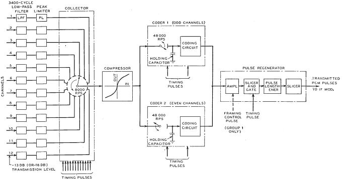
Fig. 7. PCM transmitter for a 12-channel group.
