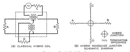
Fig. 4—a. Classical hybrid coil. b. Hybrid junction schematic diagram.
