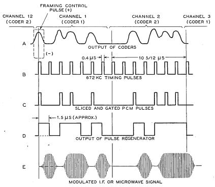
Fig. 8. Waveforms of the pulse regenerator.
