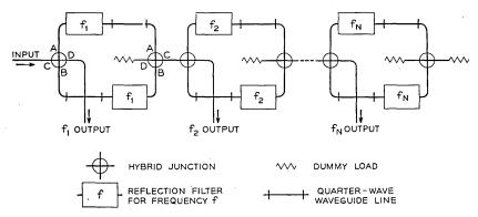
Fig. 5-N Channel branching filter.
