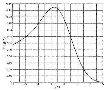
Fig. 3—Probability density of sine wave plus noise. When rms  $I_N << Q$  and I is near Q,  $p_1(y) \sim a^{-1/2}F(y-a)$ ,  $y-a=(I-Q)/({\rm rms}\ I_N)$ . See Fig. 1 for notation.
