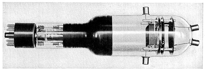
Fig. 16. Coding tube. This new electron device transforms speech samples into pulse codes.
