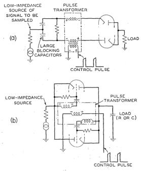
Fig. 12. Diode and triode sampling circuits.
