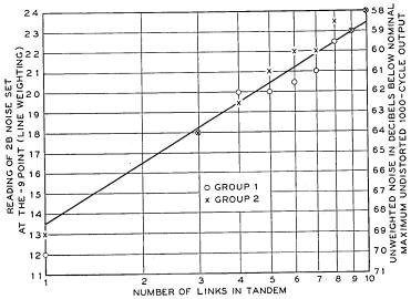
Fig. 27. Noise measurements on idle PCM channels.
