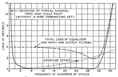
Fig. 11. Equalization for the aperture effect.
