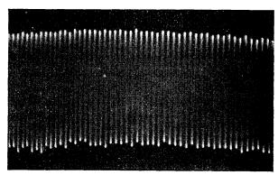
Fig. 7—Variation of quantizing current with beam deflection.
