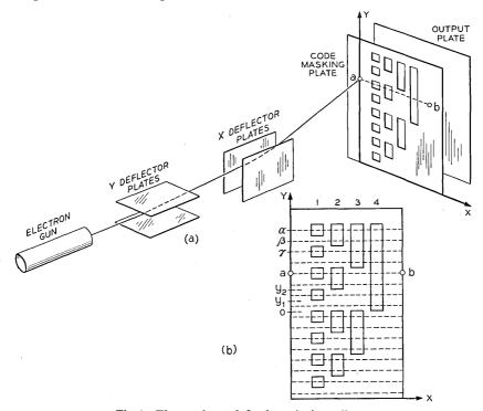
Fig. 1—Electron beam deflection tube for coding.
