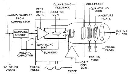
Fig. 18. Functional schematic of the coder.
