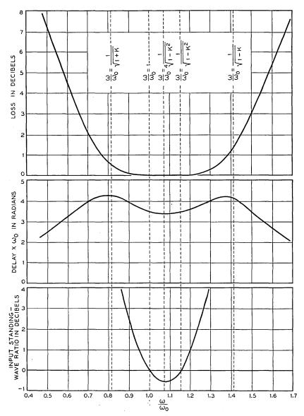
Fig. 2.—Loss, delay, and input standing-wave ratio versus relative frequency for the matched transformer for k=0.5. Loss and delay curves also apply to the case of the mis-matched transformer for k=0.632.
