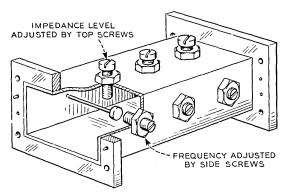
Fig. 8-Waveguide band reflection filter.
