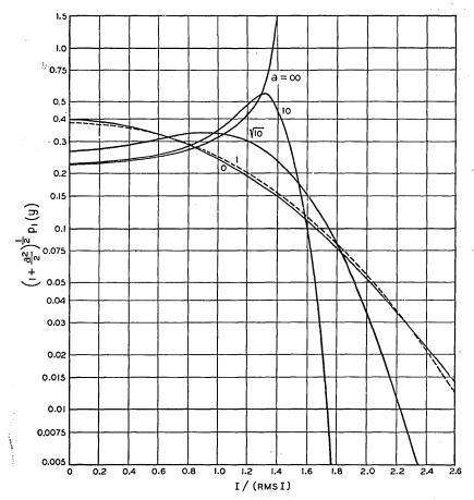
Fig. 1-Probability density of sine wave plus noise.
