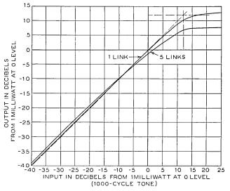
Fig. 26. Input-output characteristics of PCM channels.
