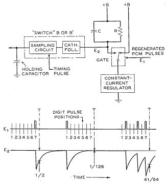
Fig. 21. Shannon decoding circuit and waveforms.
