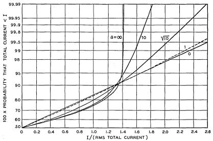
Fig. 2—Cumulative distribution of sine wave plus noise. Ordinate =  $100 \int_{-\infty}^{\infty} p_1(y_1) dy_1$ . See Fig. 1 for notation.
