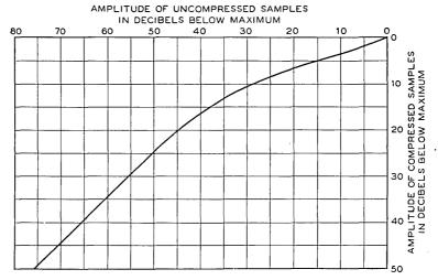
Fig. 14. Characteristic of the instantaneous compressor.
