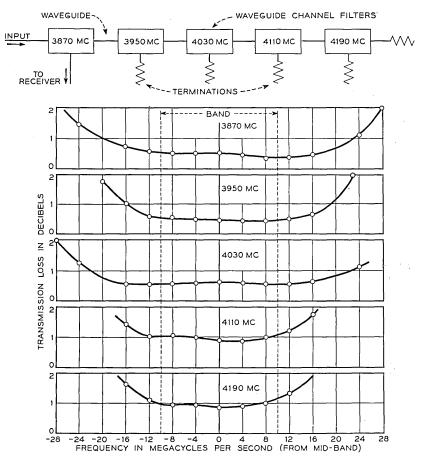
Fig. 11—Transmission loss of hybrid branching filter.
