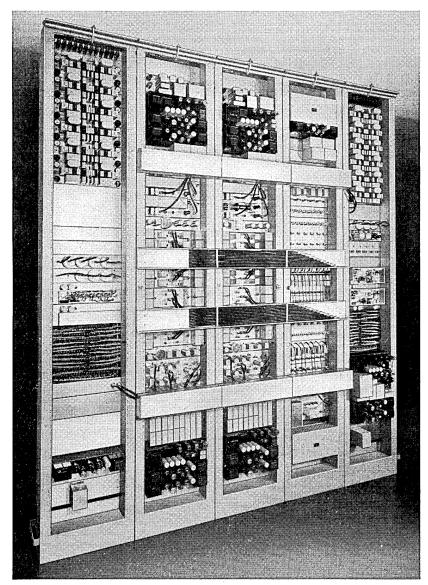
Fig. 2. Rear view. Cables in the horizontal ducts carry timing pulses leftward from the synchronizing bay.
