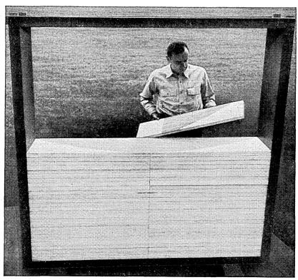
Fig. 8—A six-foot square strip lens half assembled.
