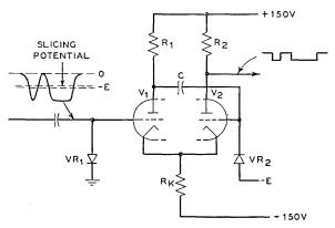
Fig. 15. Slicer circuit.
