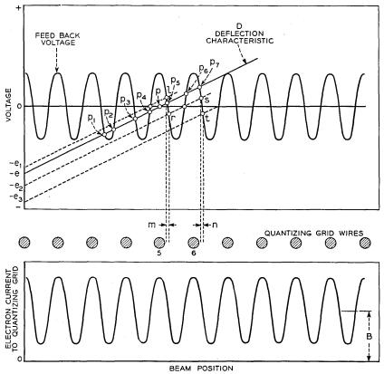
Fig. 3—Graphical representation of quantization.
