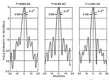
Fig. 9—Directional patterns of a 3-foot diameter lens at several frequencies.
