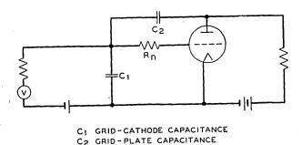
Fig. 6—Low-frequency noise in a triode can be ascribed to a fictitious noise resistance  $R_n$ , acting into an open circuit to cause voltage fluctuations on the grid.
