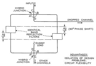
Fig. 3—Possible constant impedance channel dropping filter.
