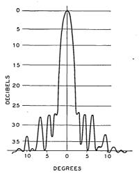
Fig. 20—Directional pattern of the lens of Figs. 8 and 16 when fed with a six-inch square electromagnetic horn.
