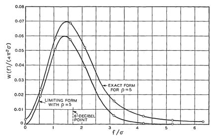
Fig. 9—Approach of W(f) to limiting form. As  $\rho \to \infty$ ,  $W(f) \to 4\pi^2 \sigma \ (\rho \sqrt{2\pi})^{-1} \ (f/\sigma)^2 \exp \left[-f^2/(2\sigma^2)\right]$ .
