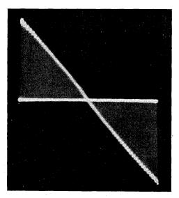
Fig. 25. Output of expandor (vertical) vs. input to compressor (horizontal).
