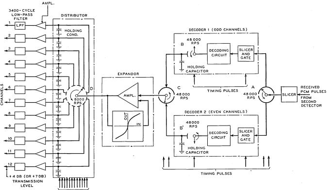
Fig. 10. PCM receiver for a 12-channel group.
