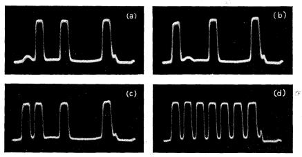
Fig. 9—Typical pulse code outputs.
