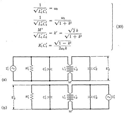
Fig. 5.—Mismatched transformer (a) fed by constant current generator, (b) with input and output reversed.
