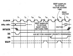
Figure 3. Interrupt Acknowledge Timing
