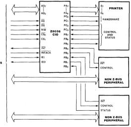
Figure 3. Functional Block Diagram
