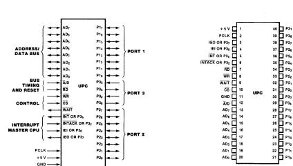
**Figure 1. Pin Functions**
