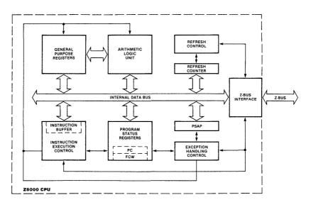
Figure 2-1. Z8000 CPU Functional Block Diagram
