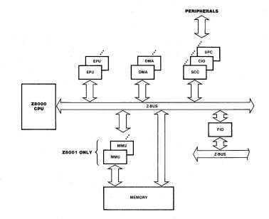
Figure 2-2. Z8000 System Configuration
