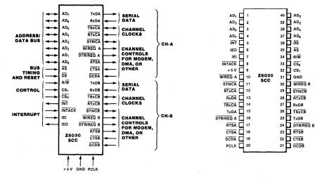
Figure 1. Pin Functions
