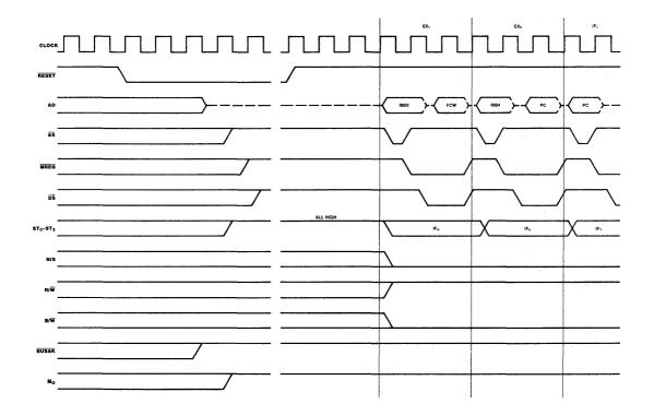
Figure 9-11. Reset Timing
