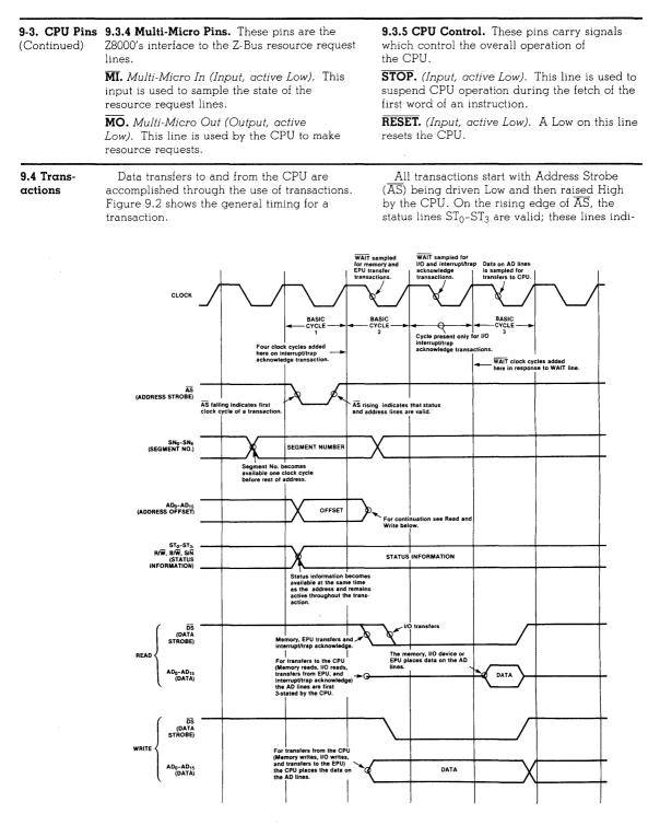
Figure 9-2. Transaction Timing
