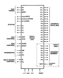
Figure 2-3. Z8000 Pin Functions
