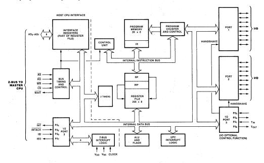
Figure 3. Z-UPC Functional Block Diagram
