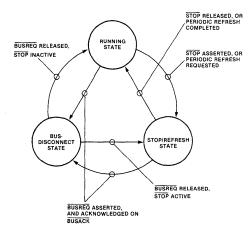
Figure 4-1. Operating States and Transistions
