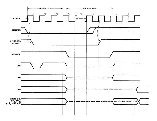
Figure 9-9. Bus Request/Acknowledge Timing
