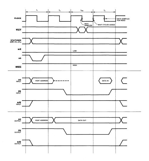
Figure 9-5. Input/Output Transaction
