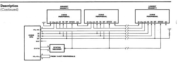
Figure 2. Interrupt Connections
