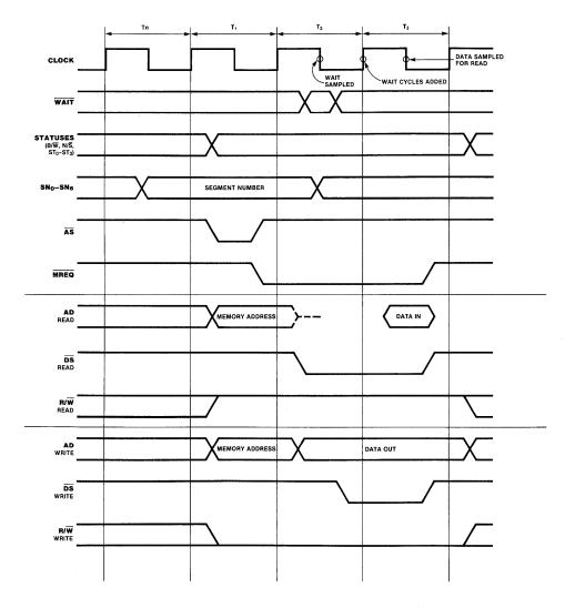
Figure 9-3. Memory Read and Write Transaction
