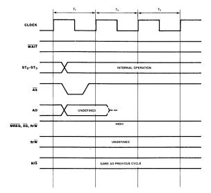
Figure 9-7. Internal Operation Timing
