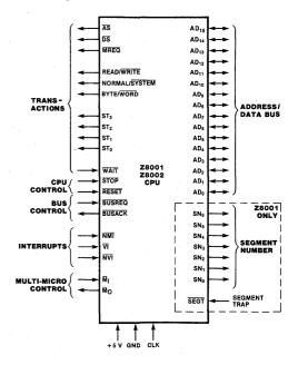
Figure 9-1. Pin Functions
