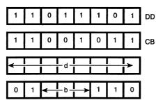
**Description:** This instruction tests bit b in the memory location specified by the contents of register pair IX combined with the two's complement displacement d and sets the Z flag accordingly. Operand b is specified as follows in the assembled object code.
