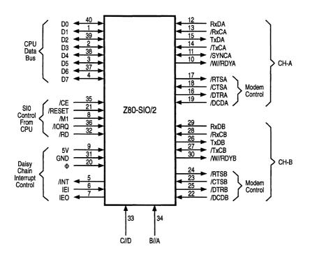
Figure 2-6. Z80-ZIO/2 Pin Assignments
