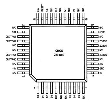
Figure 3-4. 44-pin Quad Flat Pack Pin Assignments
