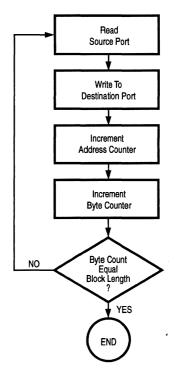
Figure 1-1. Typical CPU I/O Sequence
