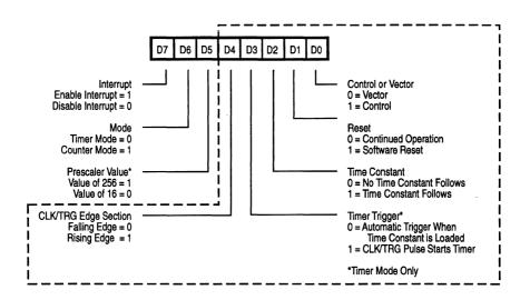
Figure 5-1. Channel Control Register
