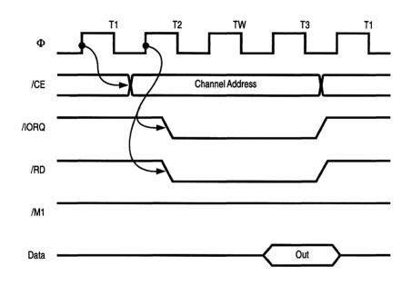
Figure 9-1. Read Cycle Timing
