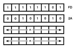
**Description:** The contents of address (nn) are loaded into the low order portion of Index Register IY, and the contents of the next highest memory address (nn+1) are loaded into the high order portion of IY. The first n operand after the opcode is the low order byte of nn.
