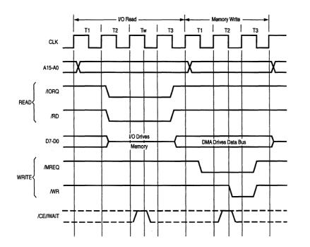
Figure 8-4. Sequential I/O-to-Memory Transfer, Standard Timing (Searching Is Optional)
