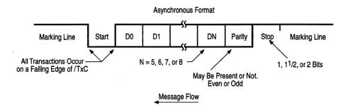
Figure 4-1. Asynchronous Message Format
