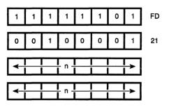
**Description:** Integer nn is loaded into the Index Register IY. The first n operand after the opcode is the low order byte.
