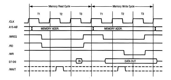
Figure 3-3. Memory Read or Write Cycle
