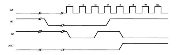
Figure 3-12. Power-Down Release Cycle No. 3
