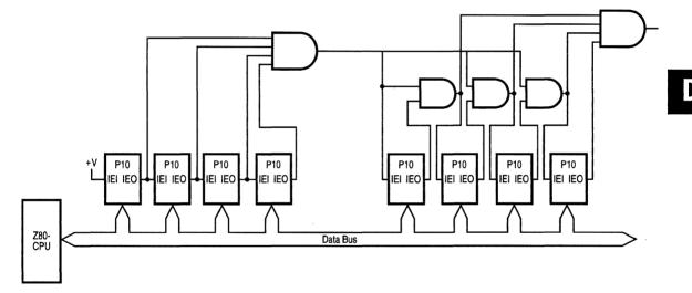
Figure 7-1. A Method of Extending the Interrupt Priority Daisy Chain
