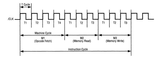
Figure 3-1. Basic CPU Timing Example
