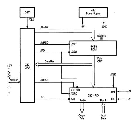
Figure 7-1. Minimum Z80 Computer System
