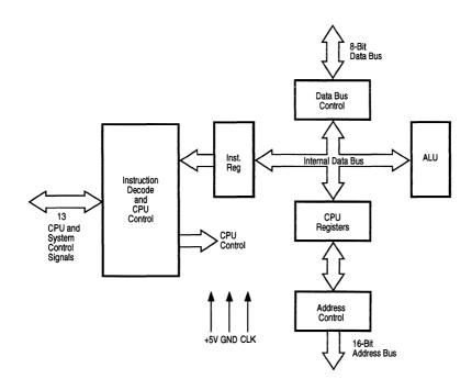
Figure 1-1. Z80 CPU Block Diagram
