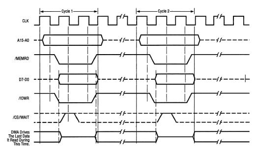
Figure 8-6. Simultaneous Memory-to-I/O Transfer (Byte Mode)
