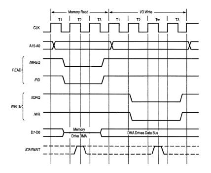
Figure 8-3. Sequential Memory-to-I/O Transfer, Standard Timing (Searching Is Optional)
