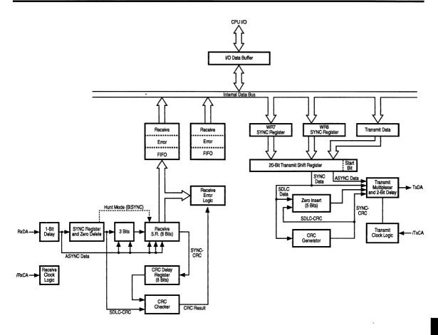
Figure 3-1. Transmit and Receive Data Path
