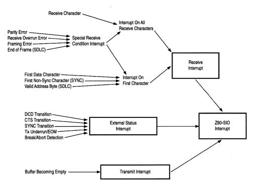
Figure 3-2. Interrupt Structure
