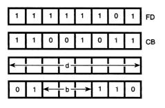
**Description:** This instruction tests bit b in the memory location specified by the content of register pair IY combined with the two's complement displacement d and sets the Z flag accordingly. Operand b is specified as follows in the assembled object code.
