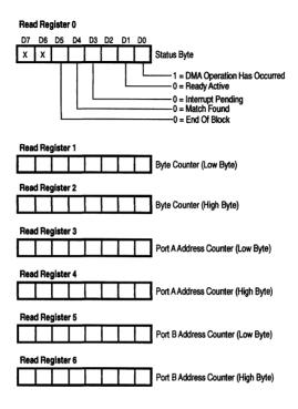
Figure A8. Read Register 0 Through 6 Bit Functions
