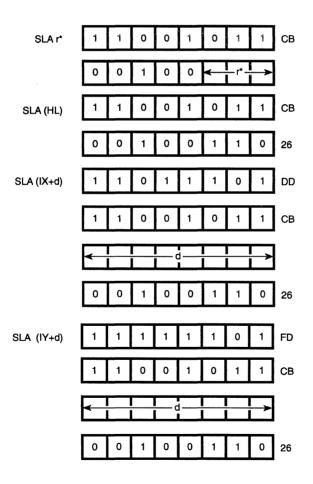
r identifies registers B, C, D, E, H, L, or A specified as follows in the assembled object code field above:
