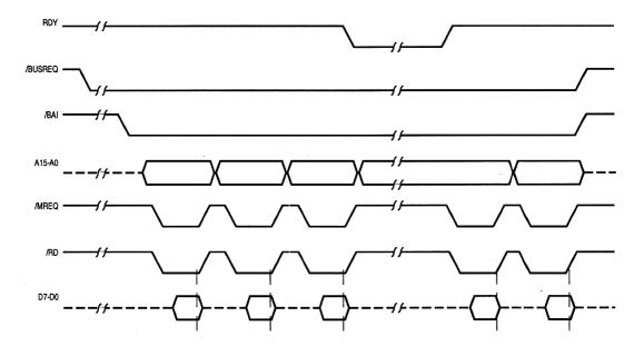
Figure 8-14. RDY Line in Continuous Mode
