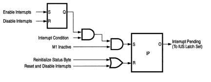
\*NOTE: Interrupt conditions can include end-or-block, byte match or active RDY line, depending on programming.
