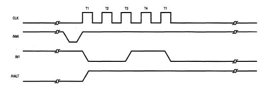
Figure 3-10. Power-Down Release Cycle No. 1
