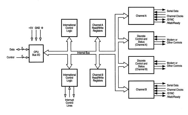
Figure 1-1. Z80-SIO Block Diagram
