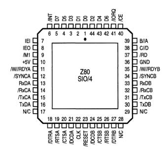
Figure 2-8. Z80-ZIO/4 Pin Assignments
