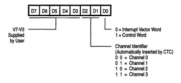
Figure 5-4. Interrupt Vector Register
