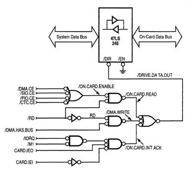
Figure 6-7. Data Bus Buffer Control Example
