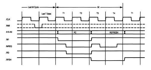
Figure 3-7. Non-Maskable Interrupt Request Operation
