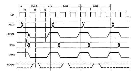
Figure 8-5. Simultaneous Memory-to-I/O Transfer (Burst and Continuous Mode)
