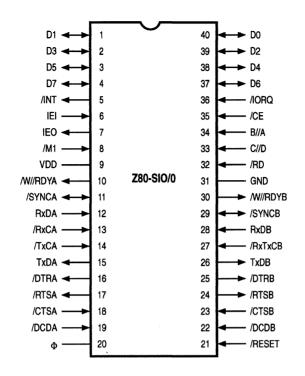
Figure 2-1. Z80-SIO/0 Pin Functions
