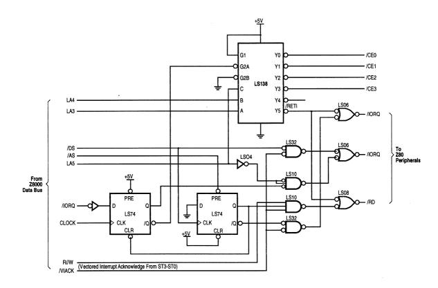
Figure 6-10. Z8000/Z80 Peripheral Interface
