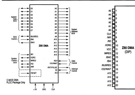
Figure 3-1. Pin Functions
