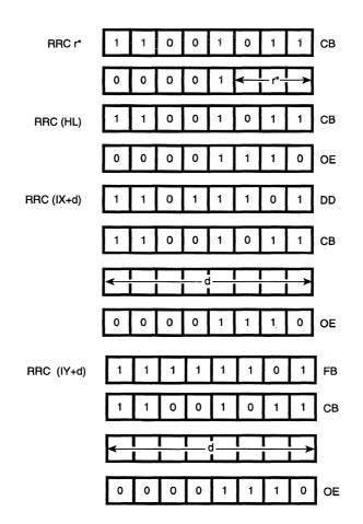
\*r identifies registers B, C, D, E, H, L, or A specified as follows in the assembled object code above:
