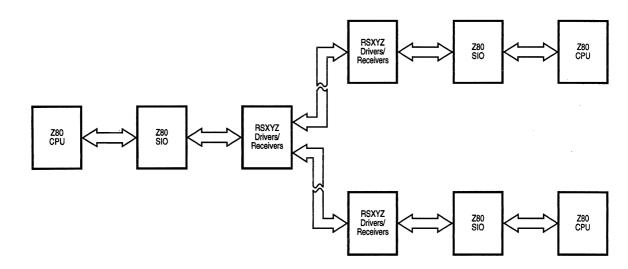
Figure 8-1. Synchronous/Asynchronous Processor-to-Processor Communication (Direct Wire to Two Remote Locations)
