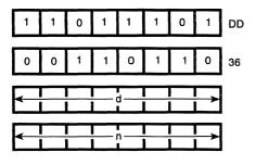
**Description:** The n operand is loaded into the memory address specified by the sum of the Index Register IX an the two's complement displacement operand d.
