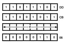
**Description:** The contents of the memory address specified by the sum of the contents of the Index Register IX and a two's complement displacement integer d, are rotated left 1-bit position. The content of bit 7 is copied into the Carry flag and also, into bit 0. Bit 0 is the least significant bit.
