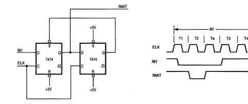
Figure 7-3. Adding One Wait State to an M1 Cycle
