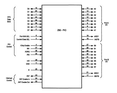
Figure 3-1. PIO Pin Functions
