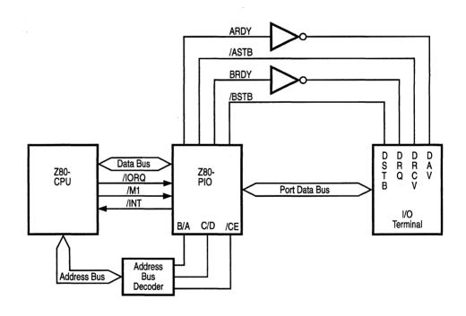
Figure 7-2. Example of I/O Interface
