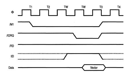
Figure 9-3. Interrupt Acknowledge Cycle Timing
