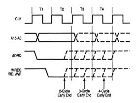
Figure 8-15. Variable-Cycle and Edge Timing
