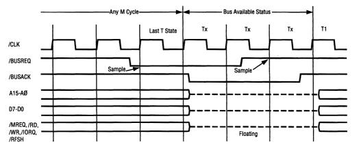
Figure 3-5. Bus Request/Acknowledge Cycle
