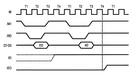
Figure 9-4. Return From Interrupt Cycle Timing
