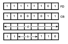
**Description:** Bit b in the memory location addressed by the sum of the contents of the IY register pair and the two's complement displacement d is set. Operand b is specified as follows in the assembled object code:
