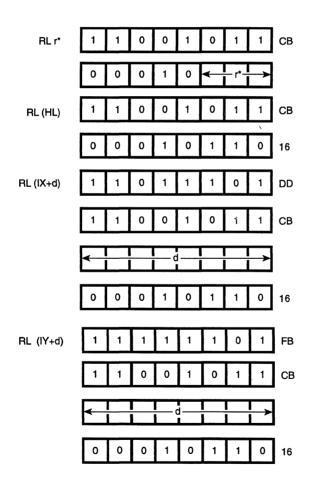
\*r identifies registers B, C, D, E, H, L, or A specified as follows in the assembled object code above:
