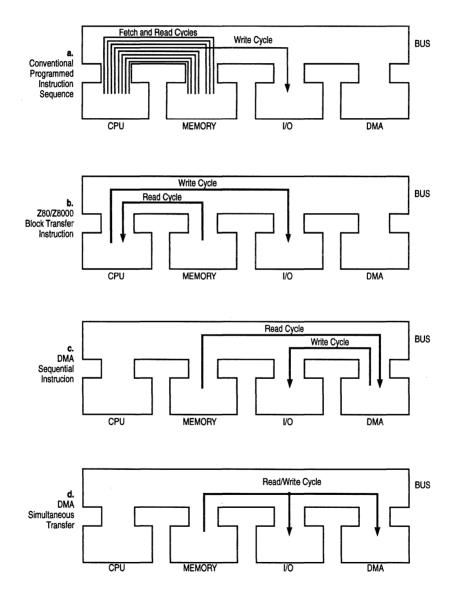
Figure 1-2. Conceptual Comparison of Various I/O Transfer Methods
