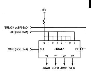
Figure 6-4. Simultaneous Transfer Multiplexer
