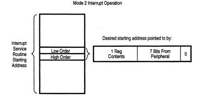
Figure 5-3. Mode 2 Interrupt Operation
