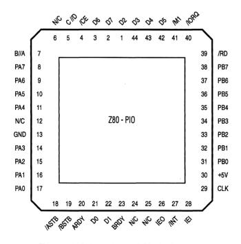
Figure 3-2. PIO 44-Pin PLCC Pin Assignments
