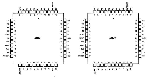
Figure 3-3. 44-Pin PLCC Pin Assignments (Z8410 NMOS)
