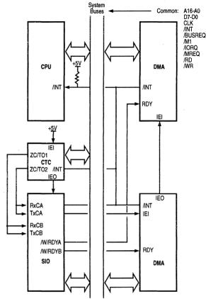
Figure 6-8. Z80 DMA-SIO Environment
