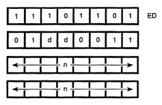
**Description:** The low order byte of register pair dd is loaded into memory address (nn); the upper byte is loaded into memory address (nn+1). Register pair dd defines either BC, DE, HL, or SP, assembled as follows in the object code:
