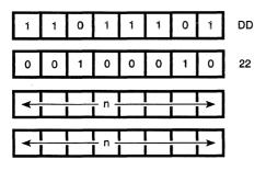
**Description:** The low order byte in Index Register IX is loaded into memory address (nn); the upper order byte is loaded into the next highest address (nn+1). The first n operand after the opcode is the low order byte of nn.
