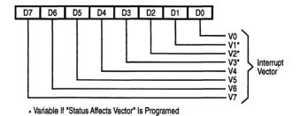
Figure 7-11. Read Register 2 (Channel B Only)
