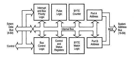
Figure 4-1. Z80 DMA Block Diagram
