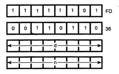
**Description:** Integer n is loaded into the memory location specified by the contents of the Index Register summed with the two's complement displacement integer d.
