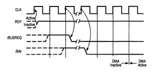
Figure 8-7. Bus Request and Acceptance Timing
