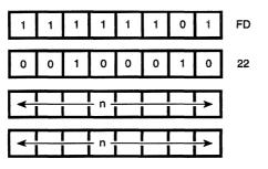
**Description:** The low order byte in Index Register IY is loaded into memory address (nn); the upper order byte is loaded into memory location (nn+1). The first n operand after the opcode is the low order byte of nn.
