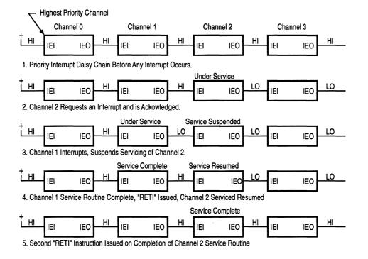
Figure 7-3. Daisy-Chain Interrupt Servicing
