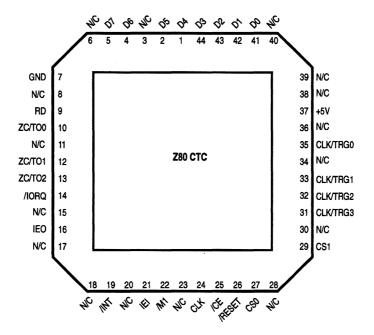
Figure 3-3. 44-pin Chip Carrier Pin Assignments
