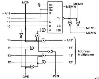
GPE is made to correspond to the 4K byte capacity of VRAM under MDA and is ANDed with A12 to A14. In case pages or graphics will be used with HGC, however, GPE will become '1' so that A12 to A14 will be enabled. In CGA mode, A12 and A13 are constantly being used. Therefore, when MON = '0' (for use with CGA), the OR operation on GPE and MON will cause the AND circuit to operate simply as a buffer.
