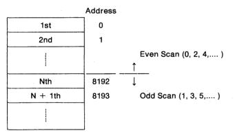
With Hercules software, the data is stored in separate banks in four-line cycles, then the banks are switched according to the Raster Address RA0, RA1 (4 Bank Mode). That is, the data of Lines 0, 4, 8, ... is placed in the first 8K bytes, the data of Lines 1, 5, 9, ... is placed in the next 8K bytes, the
