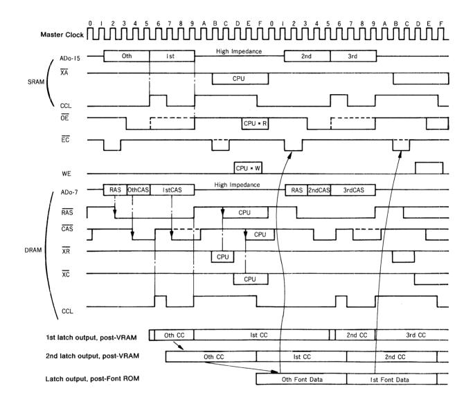
The above figure shows the timing of the various signals in High Resolution Text Mode (in case the horizontal font size is 8 PELs). The Character Codes are latched by an external circuit at the rising edge of CCL, then are latched again at the falling edge of CCL in order to provide leeway in the access time of the Font ROM. After the data from the Font ROM is latched at the falling edge of CCL, it is input to PCDC by EC via the RD bus.
