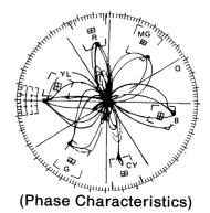
The preceding photographs depict the output of an NTSC-standard Composite signal and its phase characteristics in the case of a 14.318 MHz Master Clock frequency (when using the previously-shown circuit).
