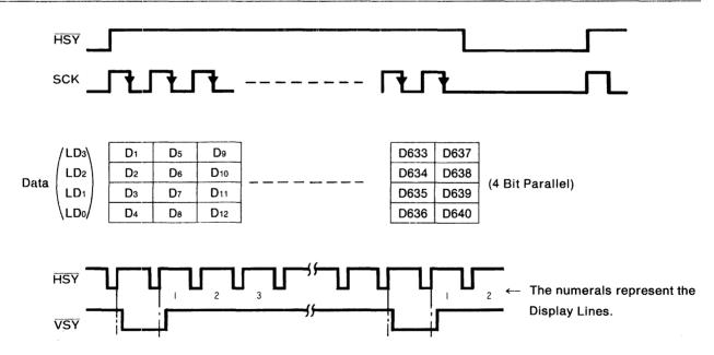
(Though the quantity of bits used for data transmission is varied, the above figure illustrates the case of 4Bit Parallel Mode.)
