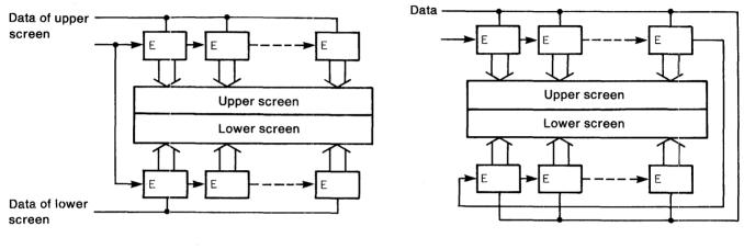
Dual-Drive Type Two-Screen LCD (Simultaneous transmission of data for upper/lower screens)
