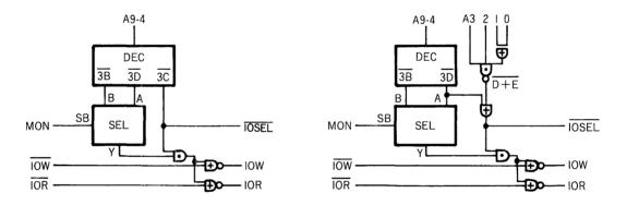
The other method utilizes the fact that the I/O Registers D and E are unused in CGA Mode and employs the same I/O ports as those of CGA for writing to the Register Bank, even with an MDA or HGC. A sample circuit for this method is shown at the above right. The MON signal therein is used by CGA, MDA, and HGC for switching the decode values for the I/O registers.
