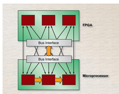
Figure 3 - FPGA-to-microprocessor without MPA support is too complicated.
