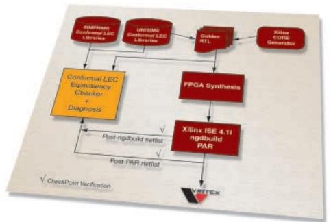
Figure 1 - FPGA equivalency checking flow with ISE 4.1i
