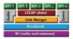
Figure 2 - Bluetooth architecture protocol stack
