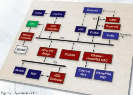
Figure 1 - Spartan-11 FPGAs provide interconnectivity in PCs to be HomePNA, Ethernet, and Bluetooth-enabled.
