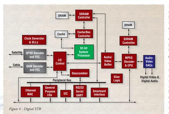
STBs usually have cable or satellite modem chips to bring broadband and TV signals to the home. Other ASSPs/ASICs handle and process digital video and audio services. These application-specific devices communicate with each other via buses on the system board. The CPU is responsible for coordinating the different
