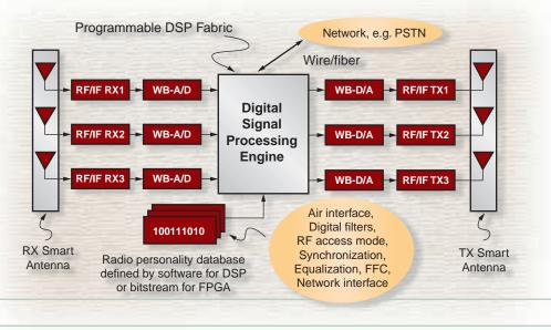
Figure 1 - SDR system diagram
