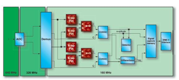
Figure 3 - Wideband down converter
