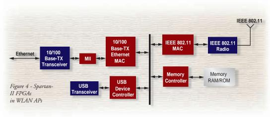
DMA engine, RAM packet buffer, host interface, configuration storage and MAC management), memory controller and as an interface to the PC.
