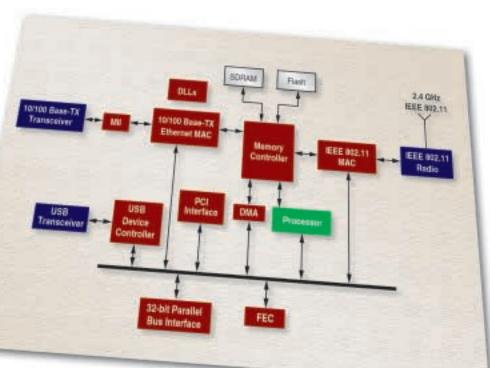
Figure 5 - Spartan-II FPGAs in (WLAN to Ethernet) technology bridges
