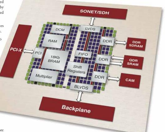
Figure 2 - A typical Virtex-II silicon block diagram
