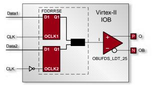
Figure 1 - Software implementation of HyperTransport and DDR implemented in a Virtex-II IOB
