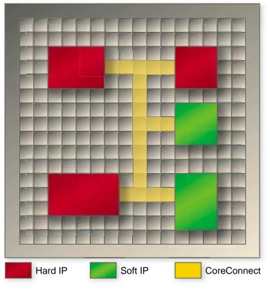
con area. The Virtex-II IP-Immersion architecture accommodates virtually any pre-defined rectilinear shape.
