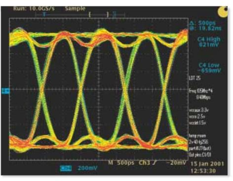
Figure 2 - Virtex-II HyperTransport I/O operating at 840 Mbps (420 MHz clock)
