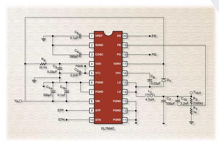
Figure 1 - EL7564C Board Circuit Schematic (VIN = 5V)
