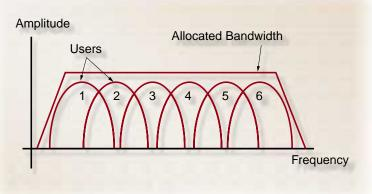
Figure 1 - OFDM allows for greater spectral efficiency
