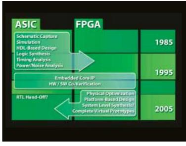
Figure 2. Evolution of ASIC and FPGA design methodologies
