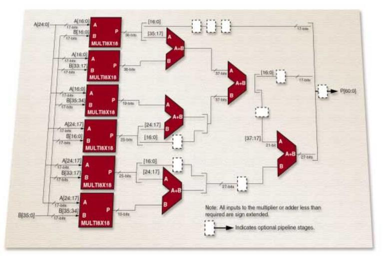
Figure 3 - Implementation produced by the Multiply Generator LogiCORE
