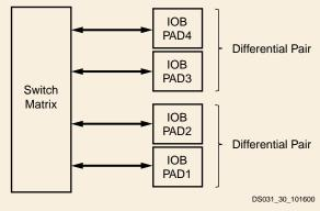
Figure 3: Virtex-II Input/Output Tile
