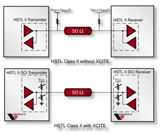
Figure 1 - Termination resistors on-chip
