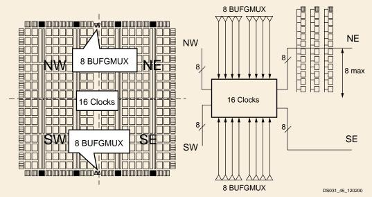
Figure 6: Virtex-II Clock Distribution
