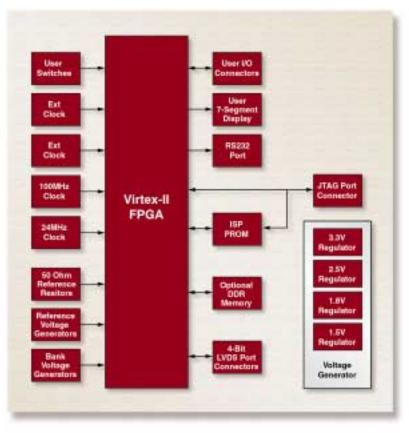
Figure 2 - Virtex-II development board block diagram
