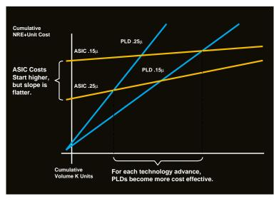
Figure 3. FPGA to ASIC crossover improves with process
