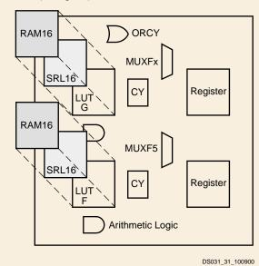
Figure 4: Virtex-II Slice Configuration
