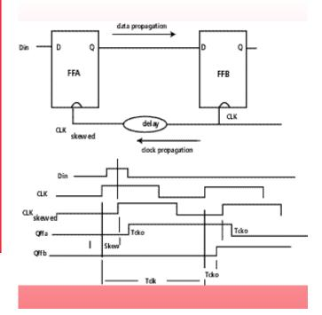
Figure 6 - Controlling the effects of clock skew through propagating the clock in the opposite direction.
