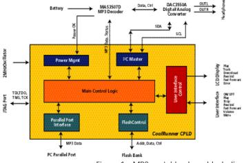
CoolRunner CPLD. All other blocks are external devices that can be obtained commercially.
