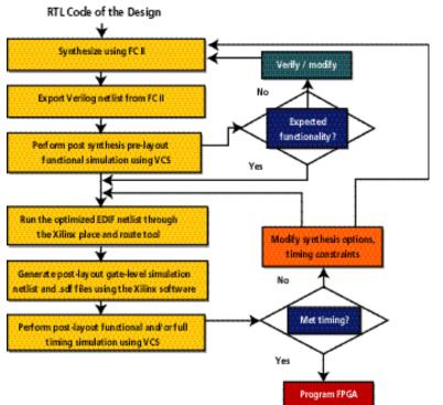
Figure 1 - Detailed design f.low for Xilinx FPGA's
