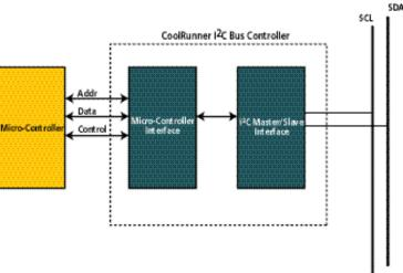
Figure 1 - CoolRunner I<sup>2</sup>C Bus Controller.
