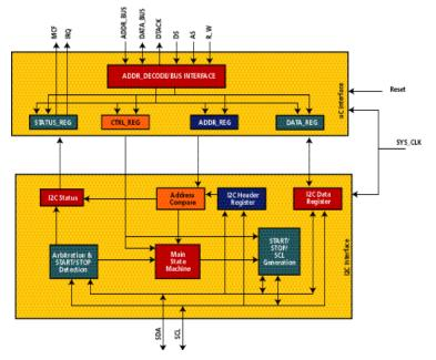
Figure 2 - CoolRunner I<sup>2</sup>C Controller block diagram.
