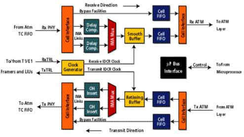
Figure 4 - Functional block diagram.
