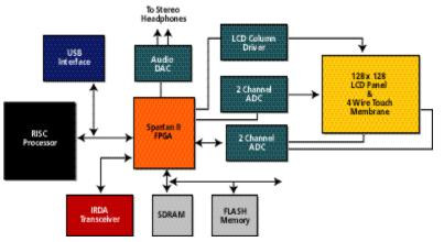
Figure 1: MP3 system block diagram.
