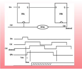
Figure 4 - Synchronous circuit with clock skew.
