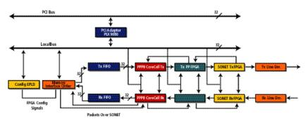
Figure 2 - Application of HDLC cores. (courtesy: CoreEL MicroSystems) packet with an FCS or invalid packet on packet interface error.
