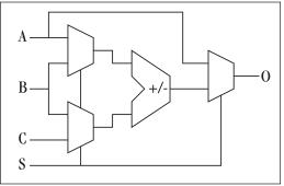
*Figure 2. Intelligent Resource Sharing Results in Efficient Arithmetic Implementations*
