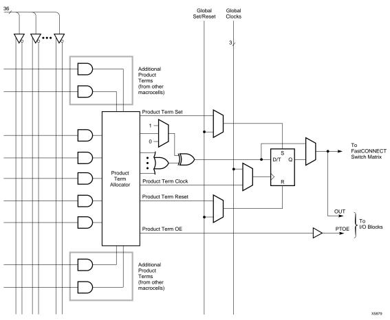
Figure 11: XC9500 Macrocell Within Function Block
