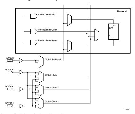
Figure 12: Macrocell Clock and Set/Reset Capability
