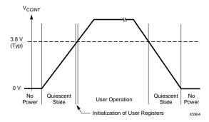
Figure 24: Device Behavior During Power-up
