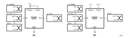
Figure 20: XC9500 Devices in (a) 5 V Systems and (b) Mixed 3.3 V/5 V Systems
