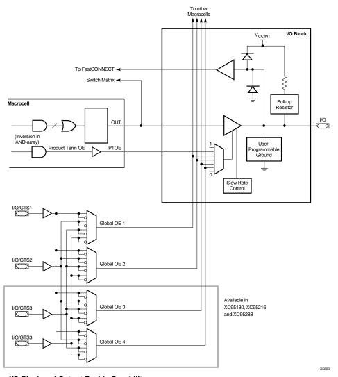
Figure 18: I/O Block and Output Enable Capability
