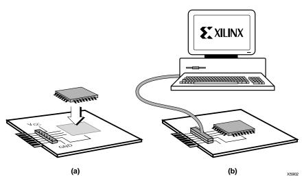
Figure 21: In-System Programming Operation (a) Solder Device to PCB and (b) Program Using Download Cable
