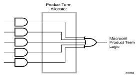
Figure 13: Macrocell Logic Using Direct Product
