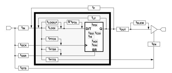
Figure 23: Detailed Timing Model
