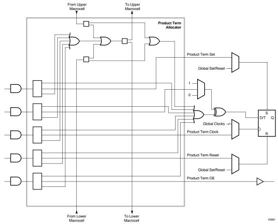
Figure 16: Product Term Allocator Logic
