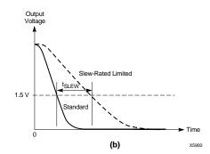
Figure 19: Output Slew-Rate Control For (a) Rising and (b) Falling Outputs
