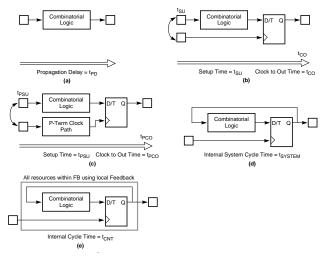
Figure 22: Basic Timing Model
