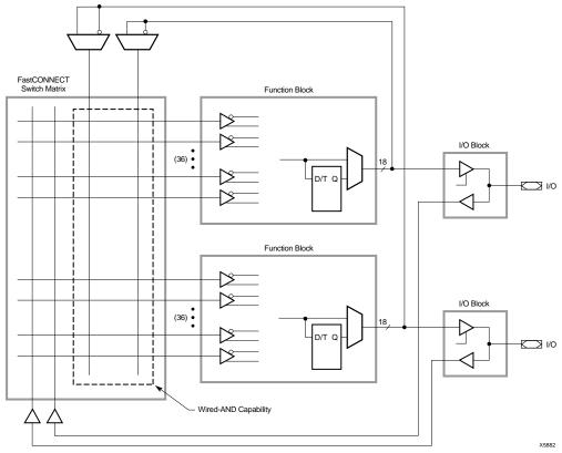
Figure 17: FastCONNECT Switch Matrix
