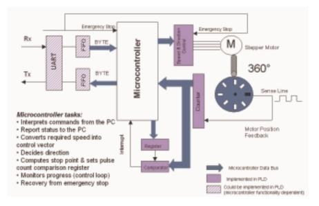
Figure 7-7 shows how we can use a microcontroller and a CPLD in a partitioned design to achieve the greatest control over a stepper motor.
