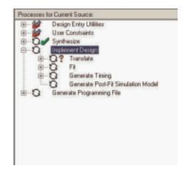
FIGURE 6-10: PROCESS WINDOW SHOWING IMPLEMENT DESIGN
