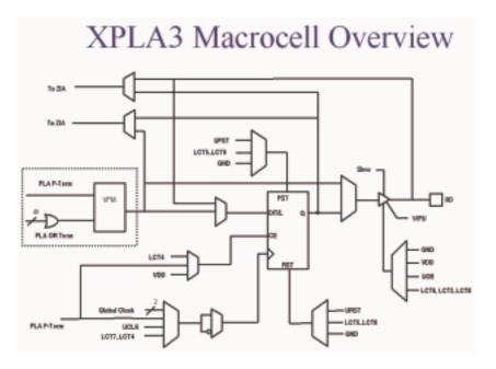
FIGURE 2-25: COOLRUNNER XPLA3 MACROCELL DIAGRAM
