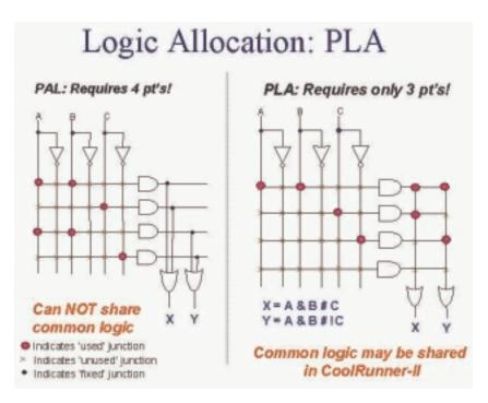
FIGURE 2-31: LOGIC ALLOCATION - TYPICAL PAL VS. PLA
