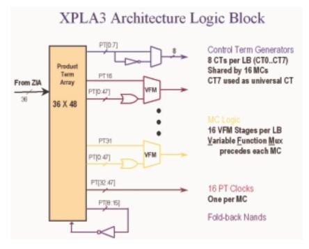
FIGURE 2-24: COOLRUNNER XPLA3 LOGIC BLOCK
