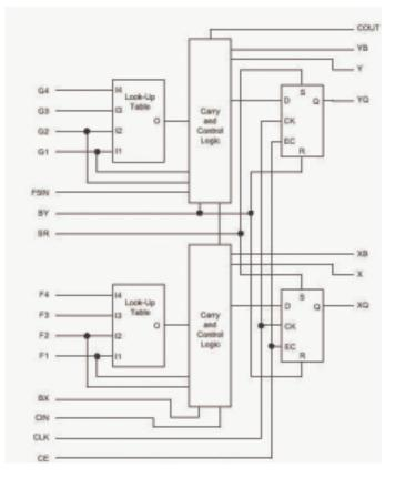
FIGURE 2-12: SPARTAN-IIE LOGIC CELL
