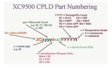
FIGURE 2-20: XC9500 PART NUMBERING SYSTEM
