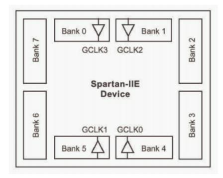
FIGURE 2-11: SPARTAN-IIE BANKING OF I/O STANDARDS
