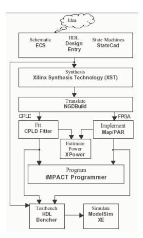
The flow diagram below shows the similarities and differences between CPLD and FPGA software flows.
