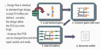
FIGURE 1-7: PLD DESIGN FLOW
