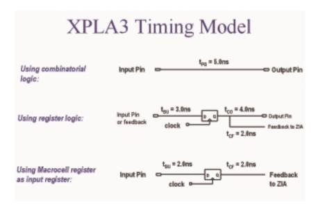
FIGURE 2-26: COOLRUNNER XPLA3 SIMPLE TIMING MODEL
