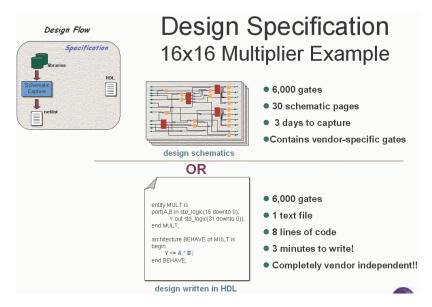
FIGURE 1-9: DESIGN SPECIFICATION - MULTIPLIER
