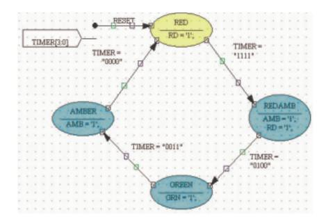
FIGURE 4-22: STATE MACHINE DRAWING
