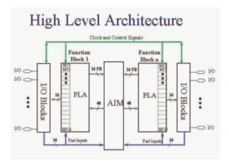
FIGURE 2-30: COOLRUNNER-II HIGH-LEVEL ARCHITECTURE
