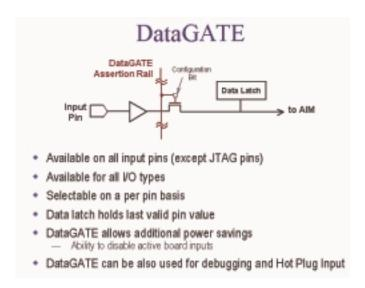
FIGURE 2-34: DATAGATE FUNCTION IN COOLRUNNER-II CPLDS
