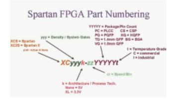
FIGURE 2-18: SPARTAN FPGA PART NUMBERING GUIDE
