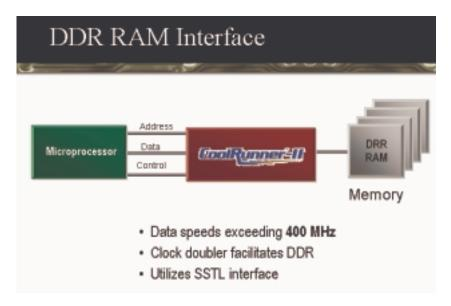
FIGURE 2-39: DDR RAM INTERFACE EXAMPLE
