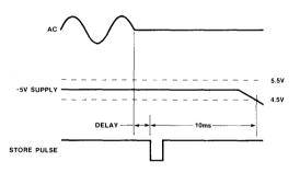
Figure 2) Missing ac must trigger a STORE pulse at least 10ms prior to the regulated dc dropping below specification.
