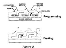
Data is stored and erased in the nonvolatile E<sup>2</sup>PROM via Fowler-Nordheim electron tunneling between these layers. An erase leaves Poly 2 positively charged; programming leaves Poly 2 negatively charged.
