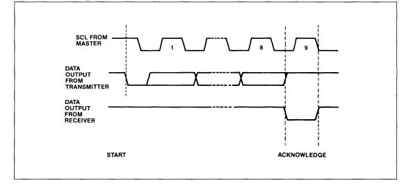
In the read mode the X2404 will transmit eight bits of data, release the SDA line and monitor the line for an acknowledge. If an acknowledge is detected and no stop condition is generated by the master, the X2404 will continue to transmit data. If an acknowledge is not detected, the X2404 will terminate further data transmissions and await the stop condition.
