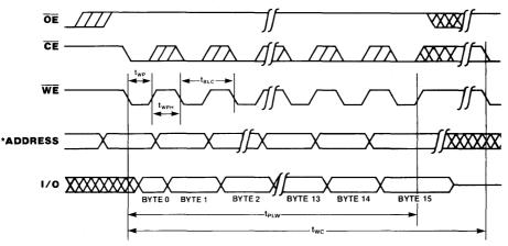
The page address, addresses  $A_4-A_{12}$ , must remain the same throughout the page write cycle ( $t_{PLW}$ ). If a page violation occurs, writes to an unknown address could result.
