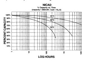
Figure 2: Nicad-Capacity vs. Time with Varying Temperatures
