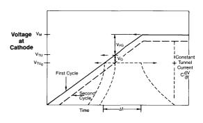
Figure 4: Voltage vs. Time Relationships at Floating Gate
