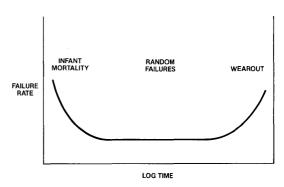
Figure 18: Illustration of bathtub curve of failure rates showing regions in which infant mortality, random failures, and wearout mechanisms dominate the failure rate.
