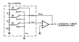
Figure 7) A simplified 3-switch CMOS DAC.
