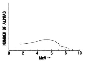
Figure 5: Spectrum of alpha particle emission rate vs. particle energy from an alumina lid. (Data from Meieran et al, ref. 23).
