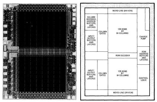
1. All aboard. This 16-K electrically erasable programmable read-only memory integrates all its support circuits. A charge pump generates the programming voltage from a 5-V supply; latches hold addresses and data during the internally timed write cycle.
