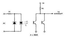
Figure 7) Two optoelectronic isolators are connected with their diodes back to back to provide an interupt signal.
