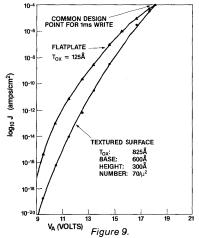
This figure illustrates that the two surface types do achieve a common design point at the higher current levels where programming occurs.
