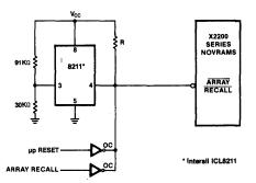
Figure 3: Power-up/Power-down Write Protection Circuit
