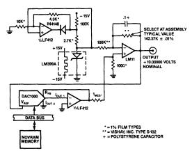
Figure 12) Software programmable voltage reference.
