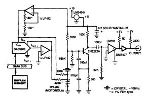
Figure 10) Tuneable crystal oscillator.
