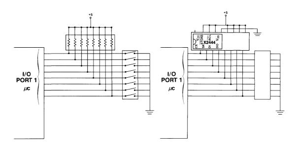
Figure 2. Microcomputer without Internal Pullups
