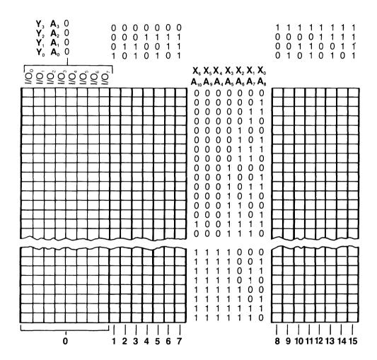
Figure 5: X2816A physical bit map. The arrangement of bits within each byte are displayed for column  $\not 0$  and suppressed for the other columns.
