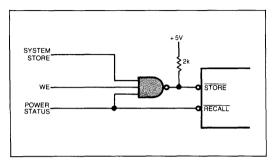
Fig 9—By NANDing the store, WE, and power-status signals you can protect the NOVRAM from false store commands. In this configuration, all three inputs must be true for a store operation to occur.
