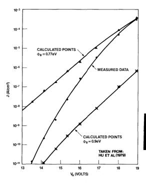
Figure 9: Current vs. applied voltage for current from textured poly surface emitted through 1760 Å of thermal SiO<sub>2</sub> compared with calculations based on previously available theory.
