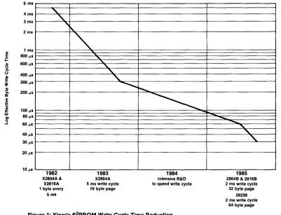
Figure 1: Xicor's E<sup>2</sup>PROM Write Cycle Time Reduction. Effective byte write cycle time is calculated by dividing the device's internal write cycle time by the number of bytes per page.
