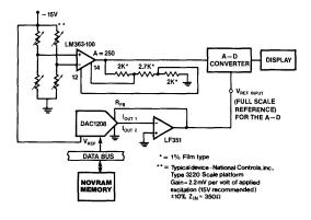
Figure 14) Automatic scale calibration.
