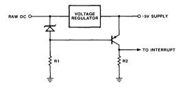
Figure 15) A dropping unregulated dc turns on the PNP transistor.
