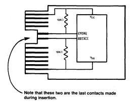
Figure 5: Typical Cartridge Write Protect Scheme
