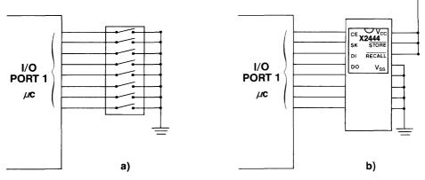
Figure 1. Microcomputer with Internal Pullups
