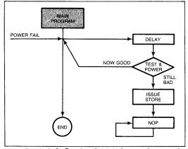
Fig 3—In a typical  $\mu P$  system that tests for power loss, once the processor receives an interrupt indicating a power loss, the system initiates a subroutine that tests for a true power loss. The subroutine first produces a delay of about 2 msec; then the system looks again at the power detector's output. If that output is still asserted, the system decides that the power loss is real and sends a store pulse to the nonvolatile RAM.
