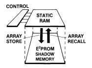
Figure 1: Xicor NOVRAM SRAM Functionality with Nonvolatile E<sup>2</sup>PROM
