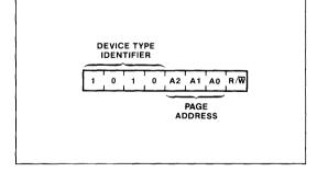
The next three bits of the slave address field are the page select bits. They are used by the master device to select which of the eight 256 word pages of memory are to be accessed. It should be noted, the protocol limits the size of memory to eight pages of 256 words; therefore, the protocol can support only one X24C16 per system.
