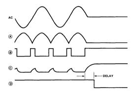
Figure 13) The delay established by R3 and C1 must be longer than the pulsewidth out of the first gate.
