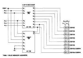
Figure 4. 74LS138 Decode Wiring Option
