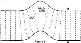
Fowler-Nordheim tunneling current increases exponentially with increasing electric field applied to the emitting surface area. Research done at Xicor has established an equation that characterizes tunneling current as a function of the amount of texture on the programming surface. The current comparison of flatplate (125 Å) and textured (825 Å) surfaces is shown in Figure 9 below.
