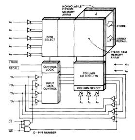
Figure 2: Functional diagram of X2212 memory
