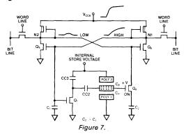
Again, VCCA goes low momentarily to equalize N1, and N2 is then allowed tdo rise. In this instance (Figure 7), the bit cell is erased (positively charged) and Q8 is on. With Q8 on, C2 and N2 are connected. N1 is then able to rise more quickly to VCCA than N2 and the latch is set with N1 high and N2 low.
