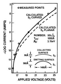
Figure 13: Forward tunneling characteristic comparing the measured data with curves calculated for a concave and a planar collecting surface.
