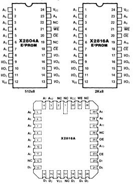
Figure 1. Pinouts for X2804A and X2816A in DIP and LCC.
