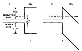
Figure 8: Energy band diagrams of the  $Si/SiO_2$  system in the neutral state (a), and during the store operation (b).
