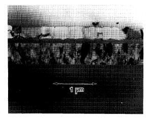
Figure 11: Transmission electron microscope (TEM) photograph of a cross-section through a textured tunneling structure. The one micron-long arrow shows the scale.
