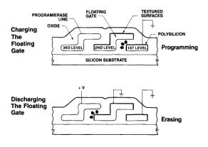
Figure 1: TPFG Cell Operation
