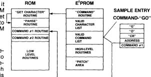
Figure 8a. Address Map for Hybrid-Initial Configuration.
