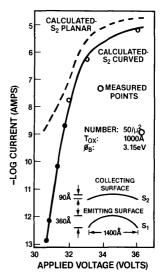
Figure 14: Reverse tunneling characteristic comparing the measured data with curves calculated for a concave and planar emitting surface.
