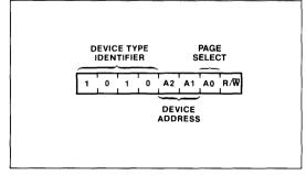
The next two significant bits address a particular device. A system could have up to four X24C04 devices on the bus (see Figure 10). The four addresses are defined by the state of the  $A_1$  and  $A_2$  inputs.
