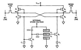
Figure 7: Schematic diagram of a NOVRAM memory cell showing how a standard six-transistor static RAM cell is merged with a floating gate E<sup>2</sup>PROM cell.
