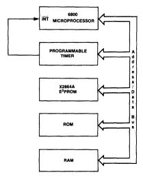
Figure 1: Hardware Configuration of a Typical System with the E<sup>2</sup>PROM and the Programmable Timer on the Bus
