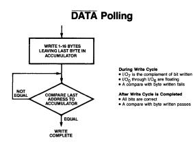
Prior to nonvolatile Write Cycle completion, the comparison test will continue. When the Write Cycle is complete, the comparison test will succeed and control will fall out of the loop. The user may then access the memory for the next read or write operation.
