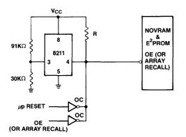
The Intersil<sup>4</sup> ICL 8211 programmable voltage reference is an inexpensive 8-pin mini DIP which will sense a selected voltage threshold and output a logic "0" when the supply is below that threshold. Conversely, as the sensed voltage rises above the selected threshold, the 8211 outputs a logic "1" following its supply voltage level.
