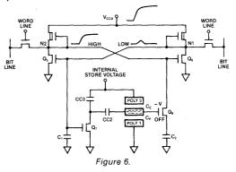
As shown in Figure 6, when recalling a programmed cell, the memory array voltage VCC<sub>A</sub> goes low momentarily to equalize the voltages at nodes N1 and N2. Then, VCC<sub>A</sub> is allowed to rise. If the floating gate on a particular bit cell is programmed (negatively charged), Q8 is off. This allows N2 to rise more rapidly than N1 to the VCC<sub>A</sub> level and the "latch" (the static RAM) is set with N2 high and N1 low.
