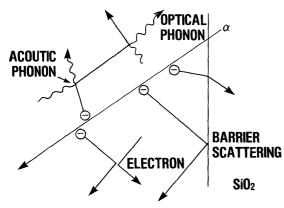
Figure 2: Schematic illustration of scattering process which contributes to small escape depth of electrons from Si.
