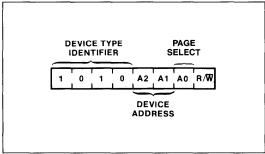
The next two significant bits address a particular device. A system could have up to four X2404 devices on the bus (see Figure 10). The four addresses are defined by the state of the  $A_1$  and  $A_2$  inputs.
