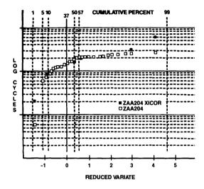
Figure 3. Correlation between endurance data obtained by Xicor and by one of Xicor's customers for Lot ZAA204. Each test is based on 28 data points. Most of Xicor's points are coincident with the customer's so that they are hidden.
