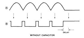
Figure 5) Waveforms in the circuit of Figure 4 without the capacitor. The microprocessor is interupted every 8.3ms and must check 2ms later to determine if the power loss is real.
