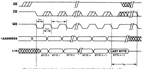
\*The page address, addresses A<sub>5</sub>-A<sub>12</sub>, must remain the same throughout the page write cycle (tpLW). If a page violation occurs, writes to an unknown address could result.
