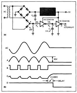
Fig 6—When you use two Schmitt triggers to detect ac loss (a), the delay produced by  $R_{s}$  and  $C_{s}$  must be longer than the first gate's output pulse width. The timing diagram (b) shows the circuit waveforms.
