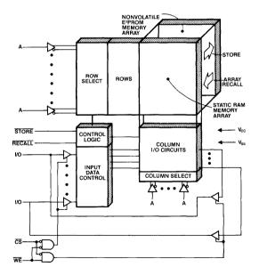
Figure 1) NOVRAM memory block diagram.
