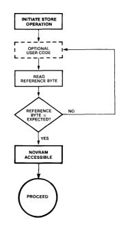
Figure 2: Early Write Completion Flowchart
