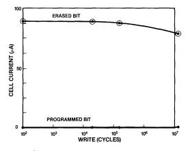
Figure 1. E<sup>2</sup>PROM cell current vs. write/erase cycles. 50  $\mu$ A is the trip point of the cell.
