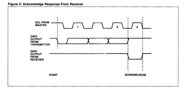
In the read mode the X2404 will transmit eight bits of data, release the SDA line and monitor the line for an acknowledge. If an acknowledge is detected and no stop condition is generated by the master, the X2404 will continue to transmit data. If an acknowledge is not detected, the X2404 will terminate further data transmissions and await the stop condition.
