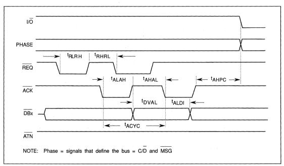
FIG. 6-28. TIMING-RECEIVE SYNCHRONOUS TRANSFER OUT AS TARGET
