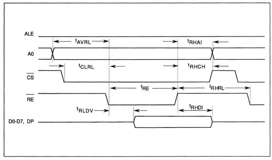
FIGURE 6-4. PROCESSOR READ TIMING
