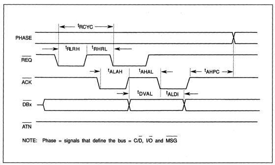
FIG. 6-27. TIMING-SEND SYNCHRONOUS TRANSFER OUT AS INITIATOR
