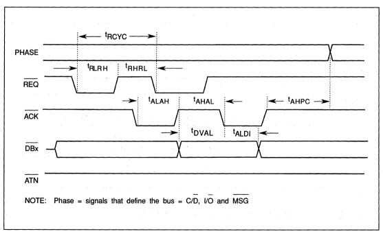
FIG. 6-26. TIMING-SEND SYNCHRONOUS TRANSFER OUT AS INITIATOR
