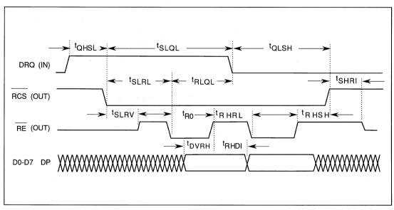
FIGURE 6-10. WD BUS BUFFER READ TIMING
