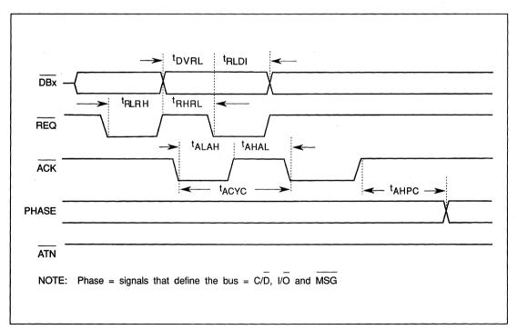
FIGURE 6-25. TIMING-SEND SYNCHRONOUS TRANSFER IN AS TARGET
