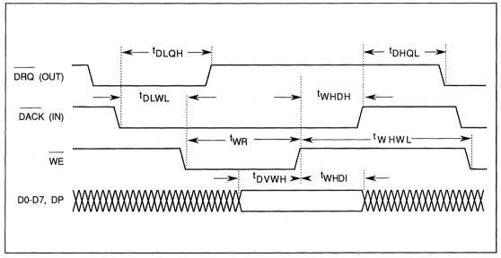
FIGURE 6-7. DMA WRITE TIMING
