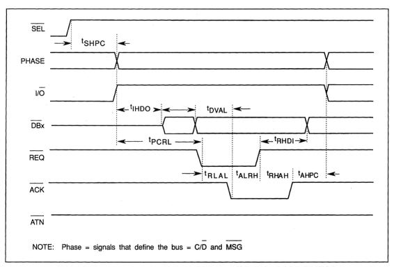
FIGURE 6-21. TIMING-ASYNCHRONOUS TRANSFER OUT AS INITIATOR
