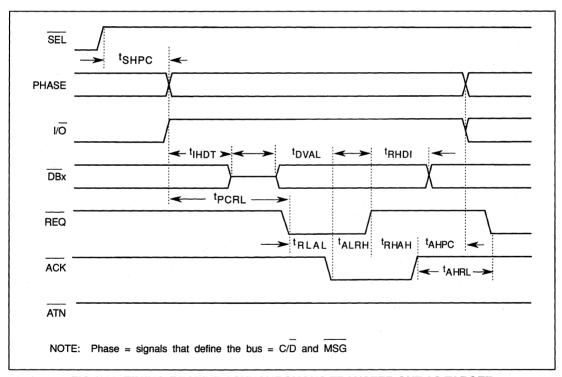
FIG.6-22. TIMING-RECEIVE ASYNCHRONOUS TRANSFER OUT AS TARGET
