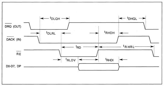
FIGURE 6-8. DMA READ TIMING
