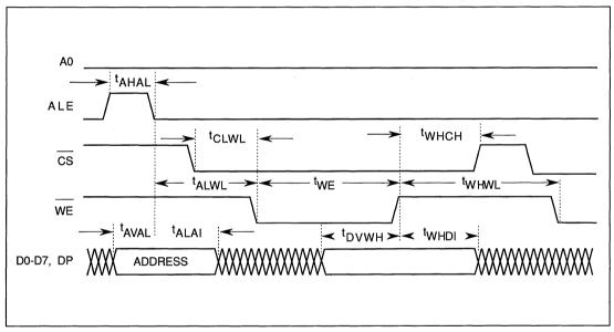
FIGURE 6-5. PROCESSOR WRITE (DIRECT) TIMING
