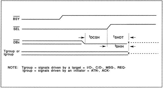
FIGURE 6-30. TIMING-SELECTION TO BUS FREE
