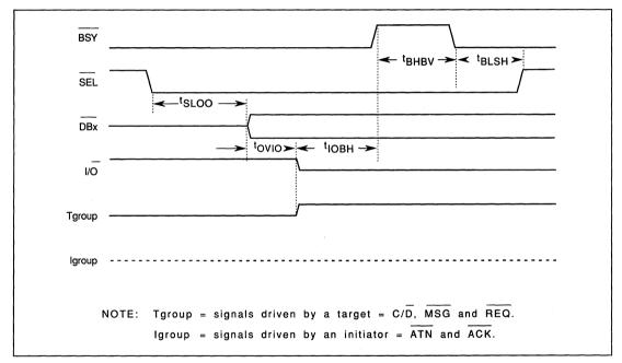
FIGURE 6-17. TIMING-RESELECTING A TARGET
