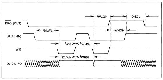
FIGURE 6-11. BURST DMA WRITE TIMING
