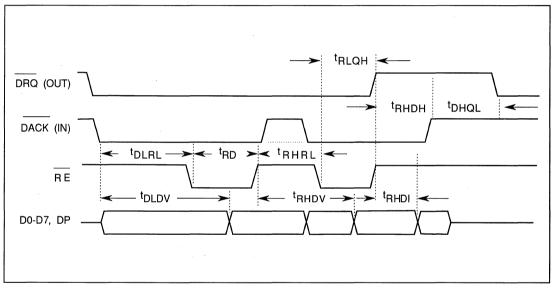
FIGURE 6-12. BURST DMA READ TIMING
