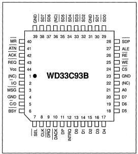
FIGURE 2-1. 44-PIN CHIP CARRIER
