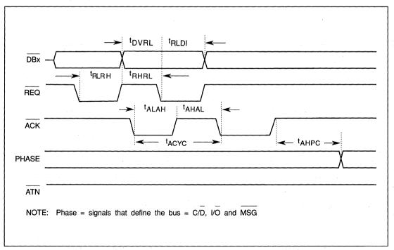
FIGURE 6-24. TIMING-SEND SYNCHRONOUS TRANSFER IN AS TARGET
