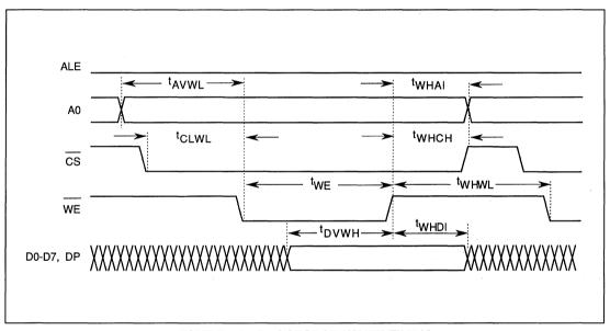
FIGURE 6-3. PROCESSOR WRITE TIMING
