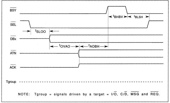
FIGURE 6-15. TIMING-INITIATOR SELECTING A TARGET
