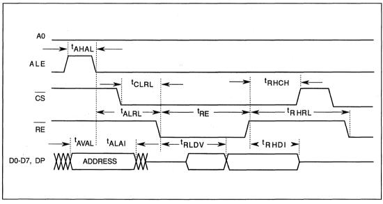
FIGURE 6-6. PROCESSOR READ (DIRECT) TIMING
