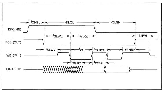
FIGURE 6-9. WD BUS BUFFER WRITE TIMING
