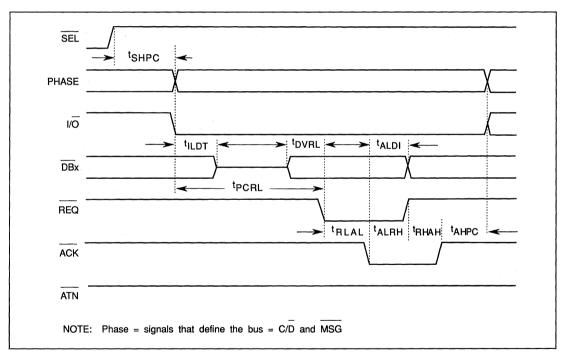
FIGURE 6-19. TIMING-ASYNCHRONOUS TRANSFER IN AS INITIATOR
