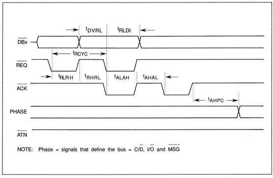
FIG.6-23.TIMING-RECEIVE SYNCHRONOUS TRANSFER IS AN INITIATOR
