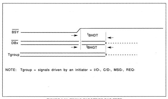
FIGURE 6-32. TIMING-TARGET TO BUS FREE
