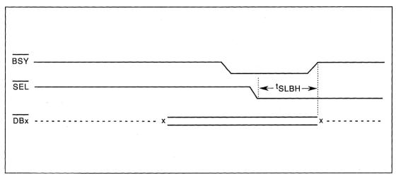
FIGURE 6-29. ARBITRATION TO BUS FREE TIMING
