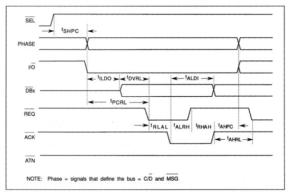
FIGURE 6-20. TIMING-ASYNCHRONOUS TRANSFER IN AS TARGET
