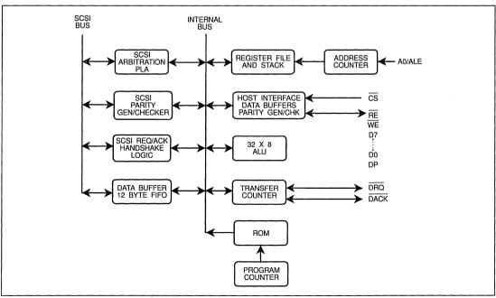
FIGURE 2-3. WD33C93B BLOCK DIAGRAM
