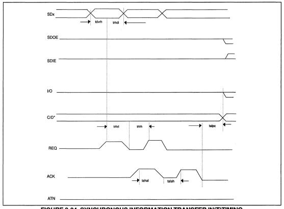
FIGURE 9-24. SYNCHRONOUS INFORMATION TRANSFER IN(T)TIMING
