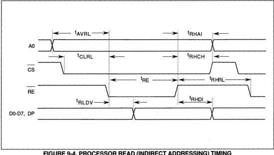
FIGURE 9-4. PROCESSOR READ (INDIRECT ADDRESSING) TIMING
