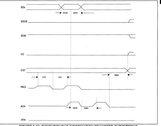
FIGURE 9-26. SYNCHRONOUS INFORMATION TRANSFER OUT(T)TIMING
