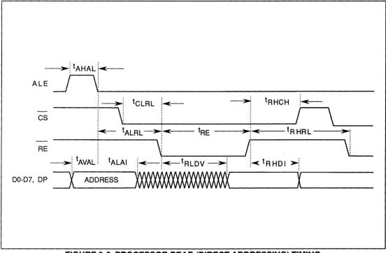
FIGURE 9-6. PROCESSOR READ (DIRECT ADDRESSING) TIMING
