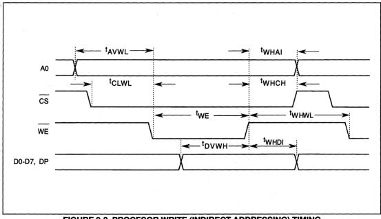
FIGURE 9-3. PROCESOR WRITE (INDIRECT ADDRESSING) TIMING
