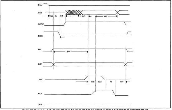
FIGURE 9-20. ASYNCHRONOUS INFORMATION TRANSFER IN(T)TIMING
