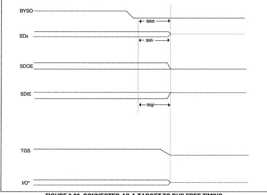
FIGURE 9-30. CONNECTED-AS-A-TARGET TO BUS FREE TIMING
