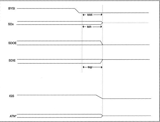
FIGURE 9-29. CONNECTED-AS AN-INITIATOR TO BUS FREE TIMING
