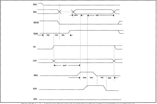
FIGURE 9-19. ASYNCHRONOUS INFORMATION TRANSFER IN(I)TIMING
