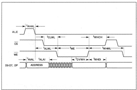
FIGURE 9-5. PROCESSOR WRITE (DIRECT ADDRESSING) TIMING
