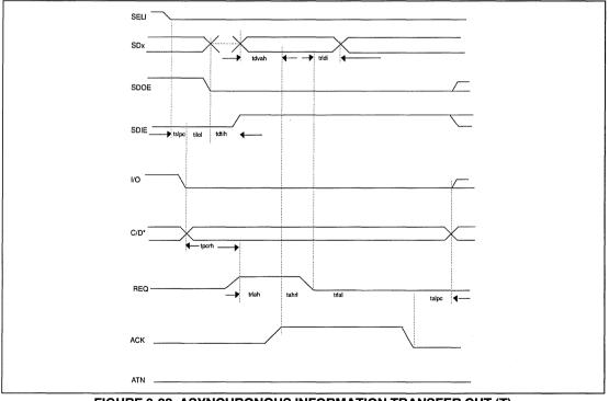
FIGURE 9-22. ASYNCHRONOUS INFORMATION TRANSFER OUT (T)
