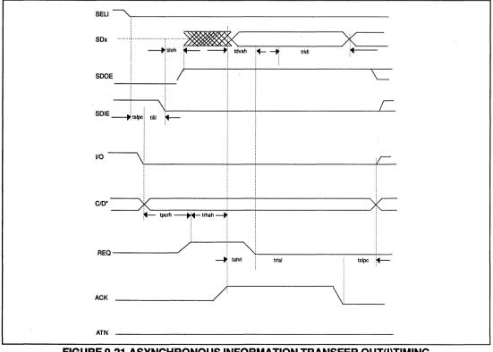
FIGURE 9-21.ASYNCHRONOUS INFORMATION TRANSFER OUT(I)TIMING
