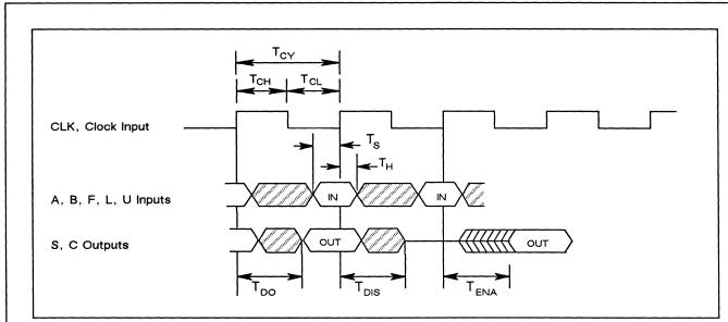
Figure 8. Switching Characteristics
