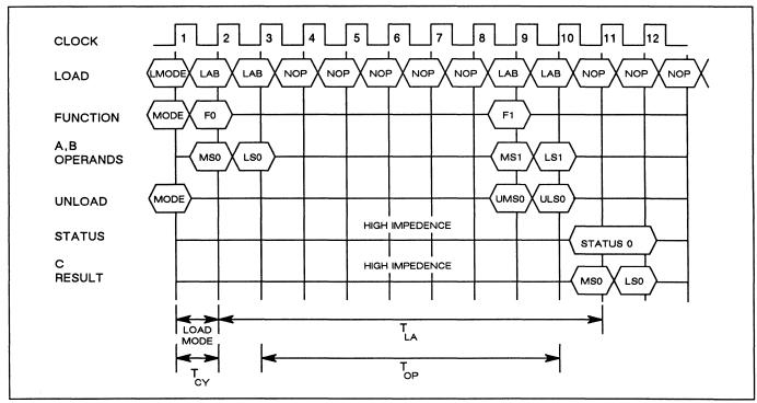
Figure 11. Flowthrough Mode Timing Diagram
