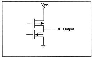
Figure 5. WTL 1232 Output Equivalent Circuit
