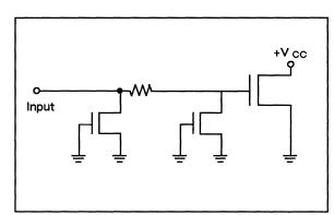
Figure 2. WTL 1233 Input Equivalent Circuit
