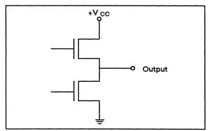
Figure 3. WTL 1233 Output Equivalent Circuit
