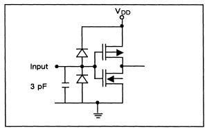
Figure 4. WTL 1232 Input Equivalent Circuit
