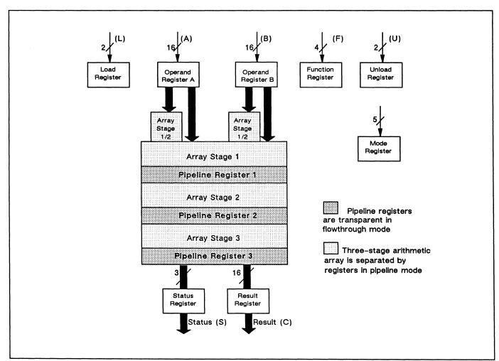
Figure 1. WTL 1232 Multiplier and 1233 ALU Data Path Architecture
