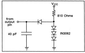
Figure 6. Test Load for Delay Measurement
