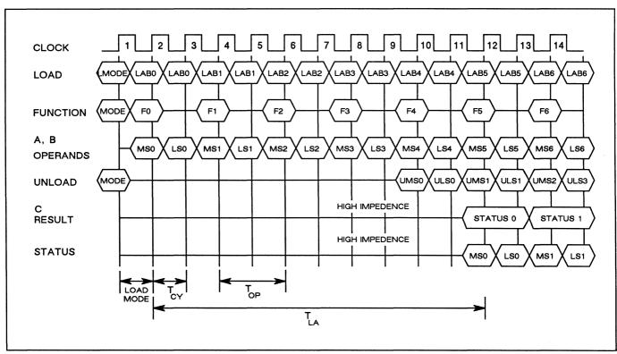
Figure 12. Pipeline Mode Timing Diagram
