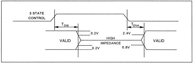
Figure 9. Tri-State Enable/Disable Timing Diagram
