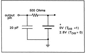
Figure 7. Test Load for Tri-State Delay Measurement
