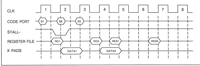
Figure 32. STALL- timing (including fstore)
