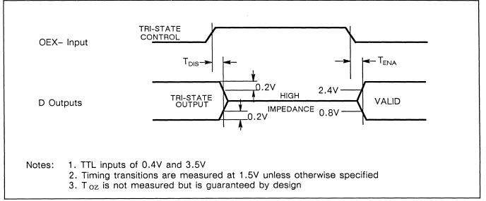
Figure 50. Tri-state timing
