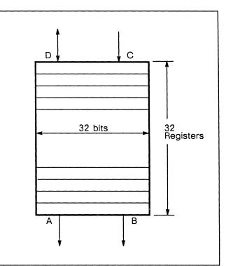
Figure 9. The four-port register file
