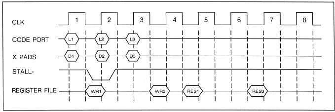
Figure 31. STALL- timing (including fload)
