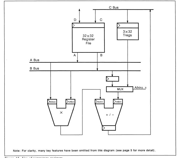
Figure 15. Use of temporary registers
