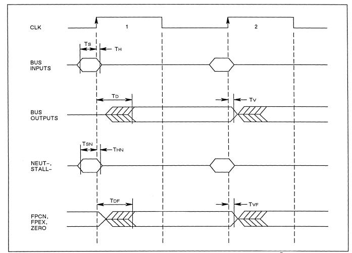
Figure 52. Signal timing diagram
