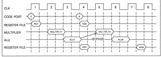
Figure 22. The timing of Internal Bypass Mode
