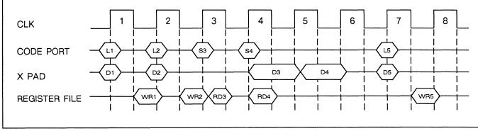
Figure 25. Normal X port I/O timing
