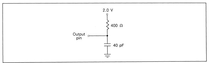
Figure 51. Test load for delay measurement
