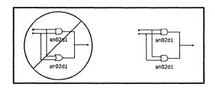
If a signal is driven by macros in parallel but whose input signals are not common, the VLSI netlist screener produces an error message unless the macros are three-state. This restriction prevents contention:
