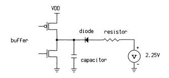
The resistor and voltage network causes the output buffers to sink or source the appropriate amount of current during AC performance simulations. For sourcing current, the diode in the above figure points the opposite direction.
