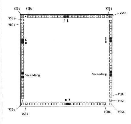
If you choose the recommended split power bus arrangement, place a PCVDD1 macro in the A position and a PCVSS1 macro in the B position. Use PCVDD2 and PCVSS2 on the vertical sides of the array, as shown, in locations C and D respectively. Additionally, for VGT100 arrays, place PCVDD1 and PCVDD2 macros in the two indicated corners of the array.
