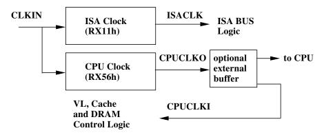
Figure 3. VT82C496G Clock Processor
