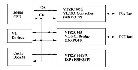
Figure 2. VT82C496G Based 80486 PCI/VL/ISA System
