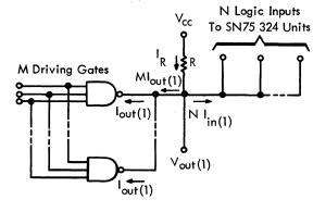
Voltage across  $R = V_R = V_{cc}$  (min) -  $V_{out}(1)$ Current through  $R = I_R = M I_{out(1)} + N I_{in(1)}$ V (···-V
