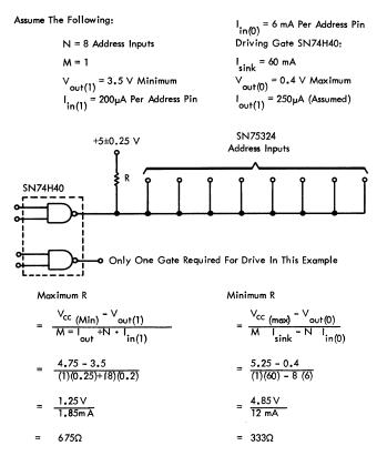
FIGURE 8. Sample Calculation of Pull-Up Resistor Value for SN74H40
