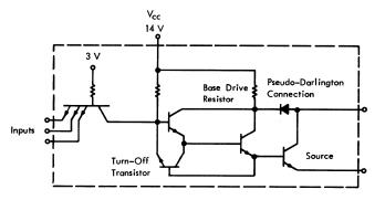
FIGURE 11. An Individual Source Circuit
