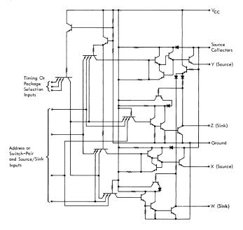
FIGURE 9. Schematic Circuit of SN75 324
