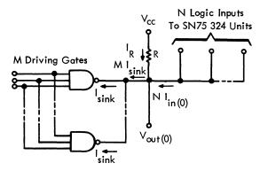
Current in resistor =  $I_R = M I_{sink} - N I_{in(0)}$ Voltage across resistor =  $V_R = V_{CC} - V_{out}(0)$
