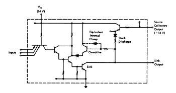
FIGURE 10. An Individual Sink Circuit
