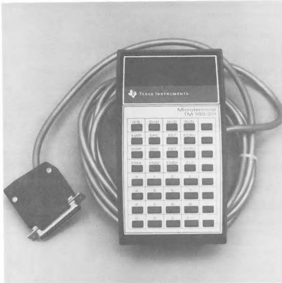
FIGURE I-1. TM 990/301 MICROTERMINAL
