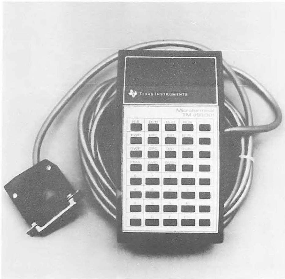
Figure 7-10. TM 990/301 Microterminal
