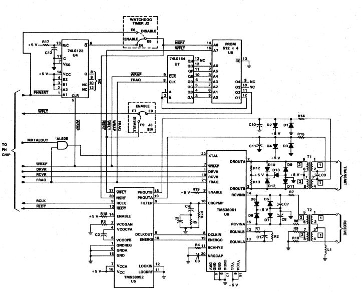
FIGURE 4-69. RING INTERFACE SCHEMATIC
