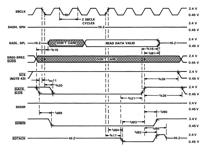
NOTE 43: The "inactive" chip select is SIACK in DIO read and DIO write cycles, and SCS in interrupt acknowledge cycles.
