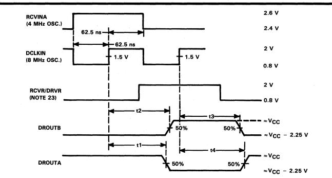
NOTE 23: For this test the RCVR output is tied directly to the DRVR input to test the asymmetry of the transmitter in a repeater configuration.
