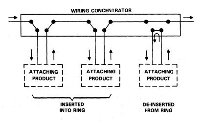
FIGURE 1-5. TOKEN RING WIRING CONCENTRATOR
