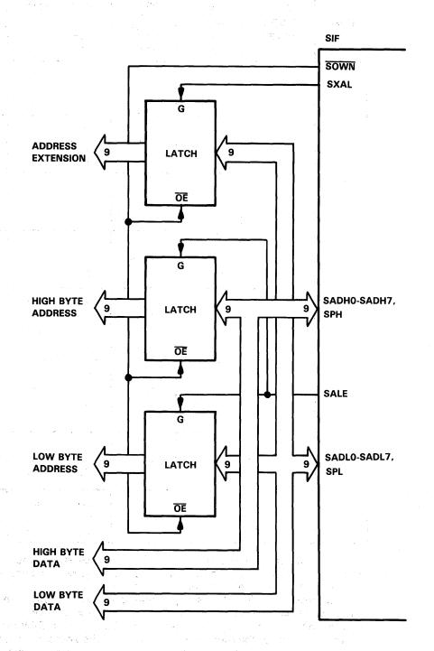
FIGURE 4-15. EXTERNAL TTL LATCHES DEMULTIPLEX ADDRESS/DATA BUS
