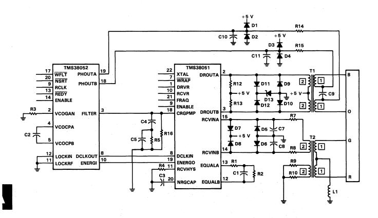
FIGURE 1. TOKEN RING INTERFACE CIRCUIT
