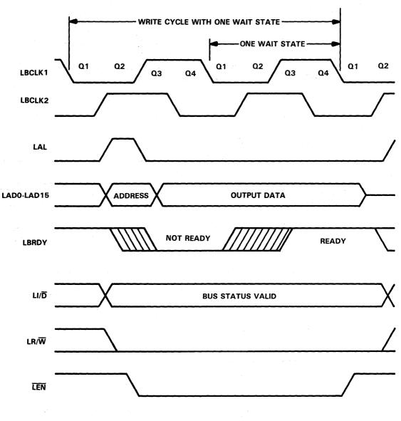
(b) LAN ADAPTER BUS WRITE CYCLE WITH WAIT STATE
