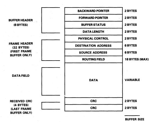
FIGURE 4-43. ADAPTER INTERNAL BUFFER FORMAT
