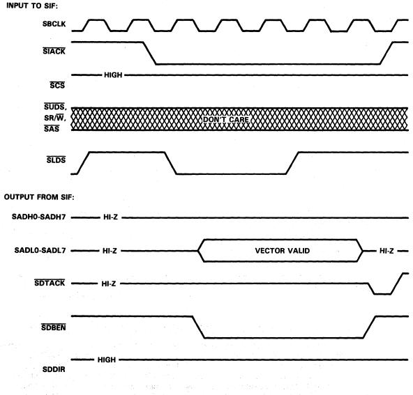
FIGURE 4-27. INTERRUPT ACKNOWLEDGE TIMING FOR 680XX MODE
