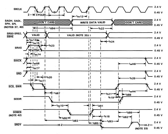
NOTES: 33. Internal logic will drive SRDY/SDTACK high and verify that it has reached a valid high level before tristating the signal. 35. In 808X Mode, SRAS may be used to strobe the values of SBHE, SRS0-SRS2 and SCS. When used to do so, SRAS must meet parameter t<sub>su14</sub> and SBHE, SRS0-SRS2, and SCS must meet parameter t<sub>su13</sub>. If SRAS is strapped high, then parameters t<sub>su14</sub> and t<sub>su13</sub> are irrelevant.
