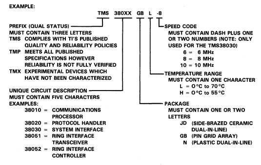
NOTE: The TMS38020 will include a ROM code level designator. (RC \_ \_ \_ \_ ).
