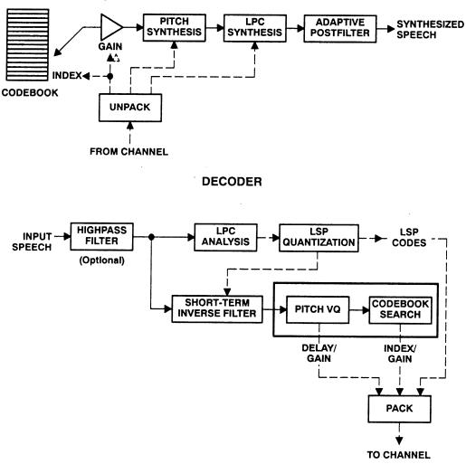
Figure 1. USFS CELP Decoder and Encoder Structures
