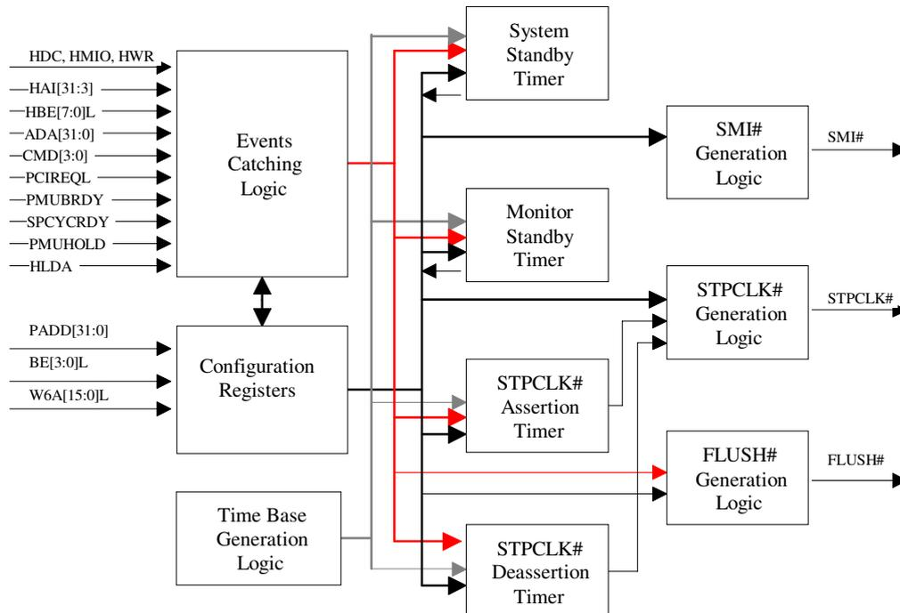
*Figure 3-6 Legacy PMU Block Diagram*
