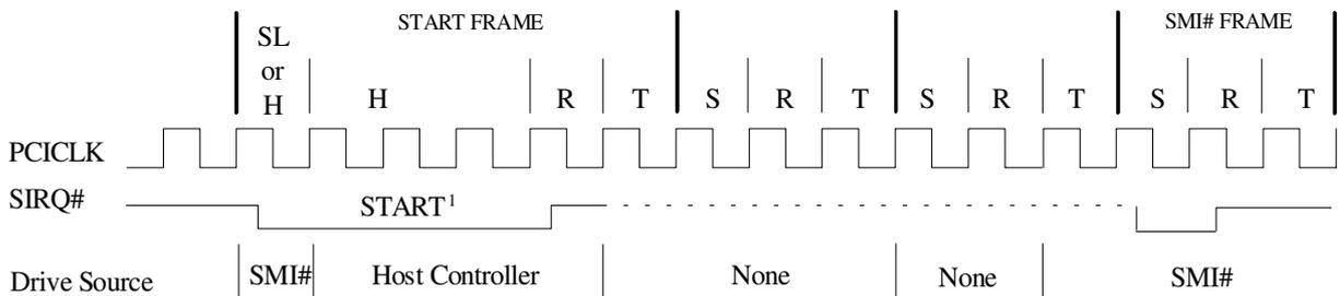
H=Host Control SL=Slave Control R=Recovery T=Turn-around S=Sample
