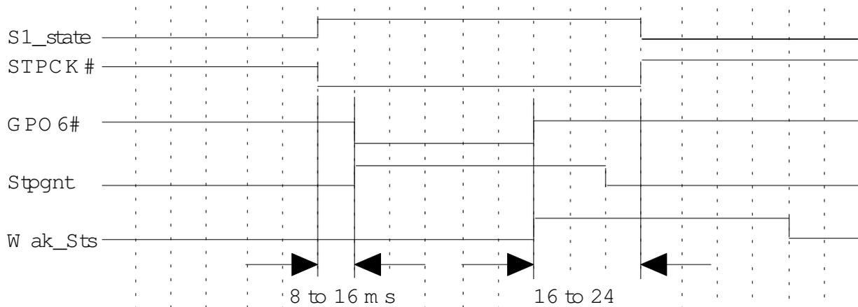
1. Programming SLP\_EN in SMI or SCI would put the PC in the system power state S1.
