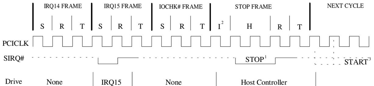
H=Host Control R=Recovery T=Turn-around S=Sample I=Idle
