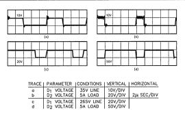
Figure 4. Output Circuit Waveforms. The Upper Traces Show the Voltage Waveform Appearing Across D1, While the Lower Covers Rectifier D2. In Both Cases, Load is at 5A; (a) with the Input Voltage at 85V and (b) at 265V.
