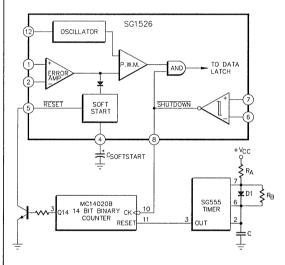
Figure 21. Using CMOS Logic as a Fault Counter to Control Transition from Pulse-by-Pulse Current Limiting to "Hiccup" Mode Current Limiting Obviously this technique can be extended even further. A second counter could accumulate "hiccup" cycles and shut the supply off until manual reset or power re-cycle. This is easily accomplished with the SG1526 since the SHUTDOWN and RESET terminals are compatible with both TTL and CMOS logic.
