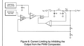
A voltage comparator with fixed input offset voltage switches from a logical HIGH state to a LOW state when the selected current threshold is exceeded. Since both logic inputs to the AND gate must be HIGH to enable the output pulse, the pulse width can be narrowed by the current limit comparator independently of the voltage control loop.
