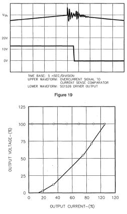
Figure 20. Measured Output Characteristics of the 100KHz Switching Supply in Figure 17.
