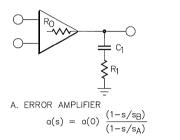
WHERE s<sub>A</sub> IS A POLE AT s =  $-\frac{1}{R_0C_1}$ WHERE s<sub>B</sub> IS A ZERO AT s =  $-\frac{1}{R_1C_1}$
