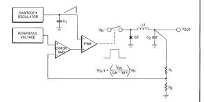
Figure 1. Basic Architecture of a Constant Voltage Switching Power Supply.
